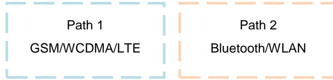
Fig.15.1 Simultaneous Transmission Paths
