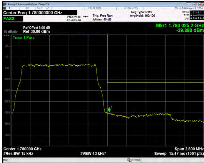
Band66 QPSK BW=10MHz Channel=132022 RB Size=1 Position=#0
