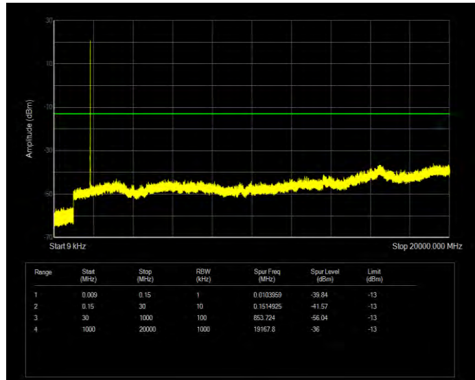
Band2 QPSK BW=3MHz Channel=18900 RB Size=15 Position=#0
