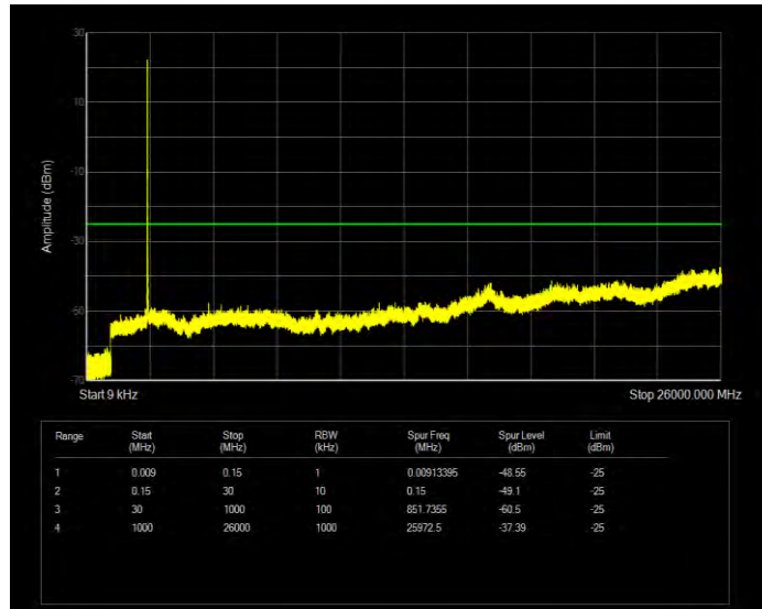
Band7 16QAM BW=5MHz Channel=21100 RB Size=25 Position=#0
