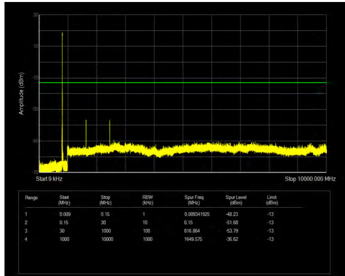
Band5 QPSK BW=1.4MHz Channel=20525 RB Size=6 Position=#0
