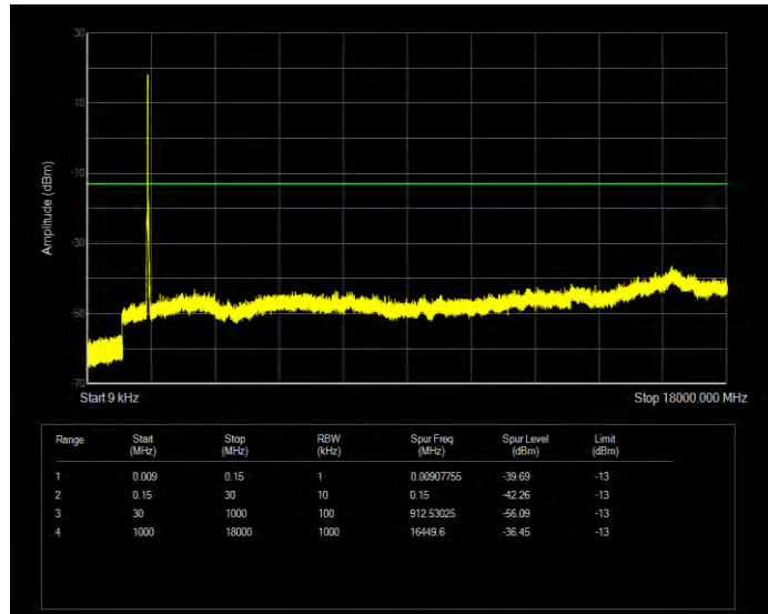
Band4 QPSK BW=20MHz Channel=20175 RB Size=100 Position=#0
