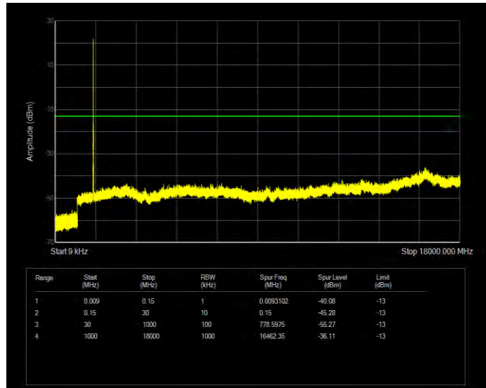
Band4 QPSK BW=5MHz Channel=20175 RB Size=25 Position=#0
