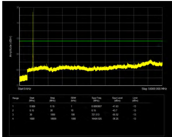
Band4 16QAM BW=3MHz Channel=20175 RB Size=15 Position=#0
