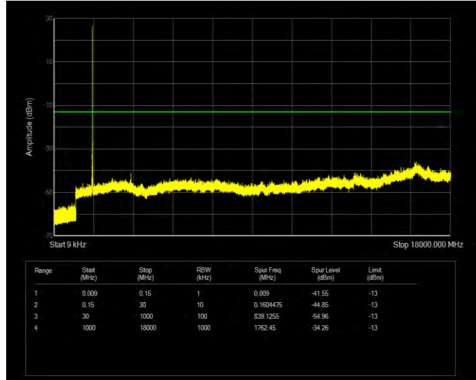
Band4 QPSK BW=10MHz Channel=20000 RB Size=50 Position=#0
