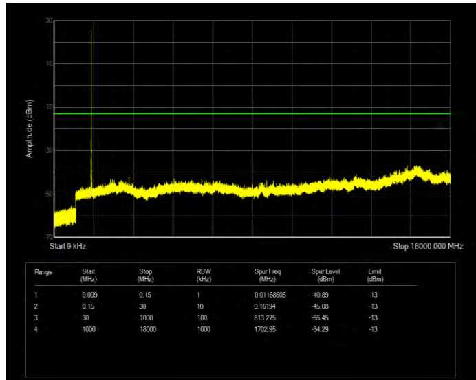
Band4 QPSK BW=1.4MHz Channel=20175 RB Size=6 Position=#0
