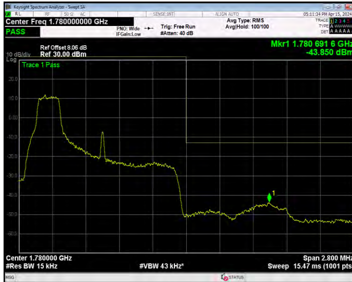
Band66 QPSK BW=1.4MHz Channel=132665 RB Size=6 Position=#0
