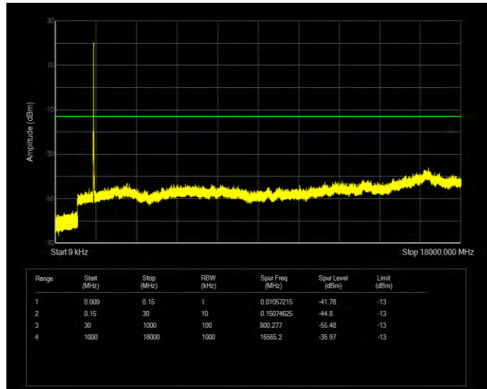
Band4 QPSK BW=10MHz Channel=20175 RB Size=50 Position=#0
