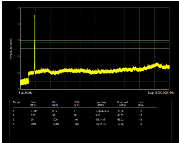
Band4 16QAM BW=10MHz Channel=20175 RB Size=50 Position=#0
