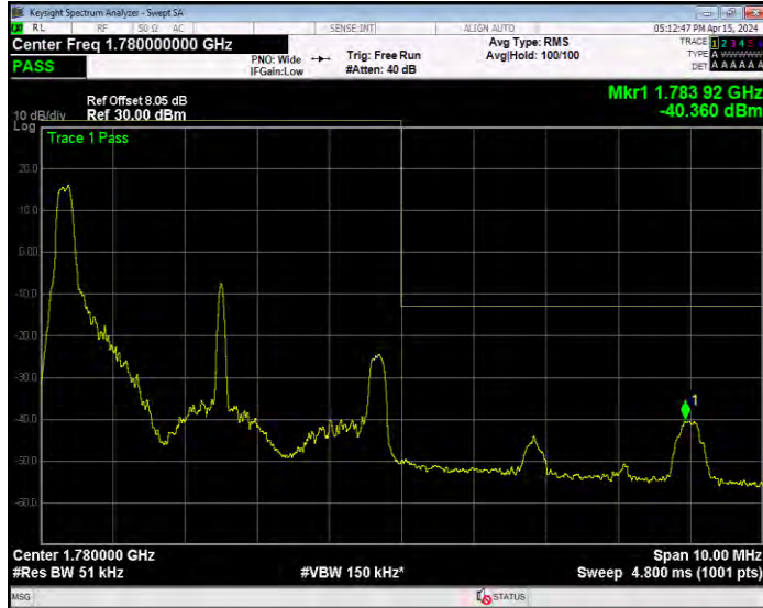
Band66 QPSK BW=5MHz Channel=132647 RB Size=25 Position=#0
