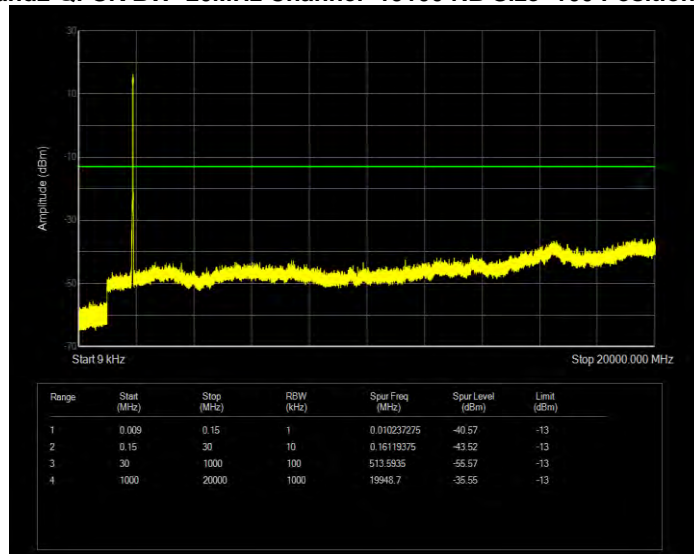
Band2 QPSK BW=3MHz Channel=18615 RB Size=15 Position=#0
