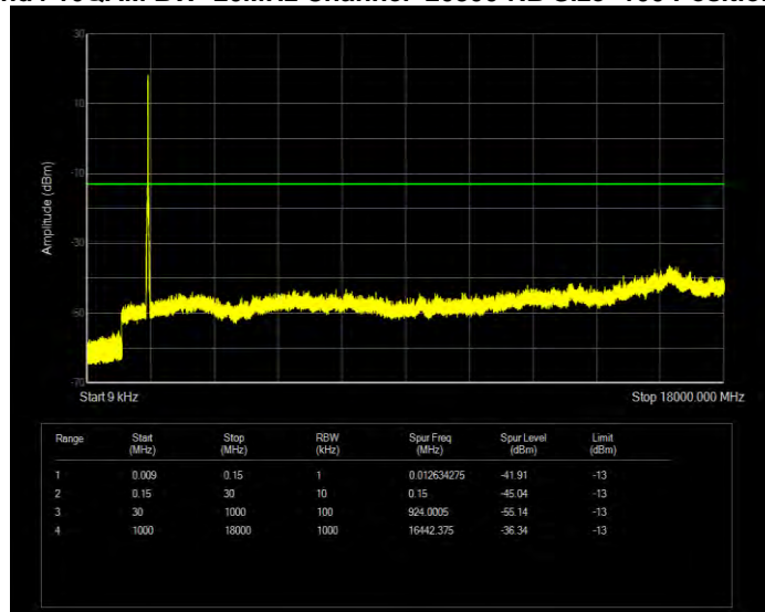
Band4 16QAM BW=3MHz Channel=19965 RB Size=15 Position=#0
