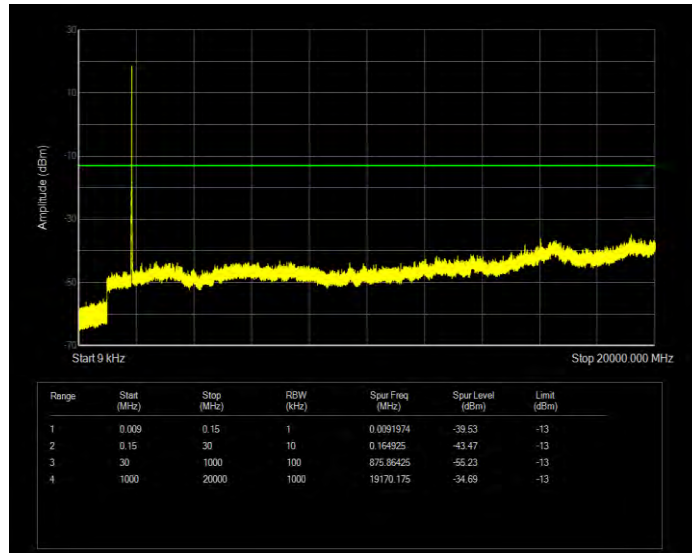
Band2 16QAM BW=10MHz Channel=18900 RB Size=50 Position=#0
