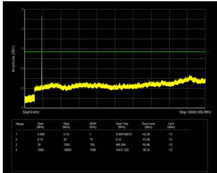
Band4 QPSK BW=3MHz Channel=20175 RB Size=15 Position=#0
