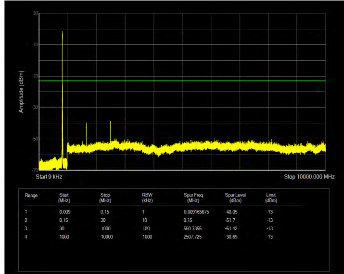
Band5 QPSK BW=3MHz Channel=20635 RB Size=15 Position=#0
