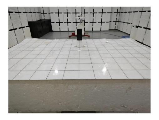
Set-up for Radiated Spurious Emission, Above 1GHz
