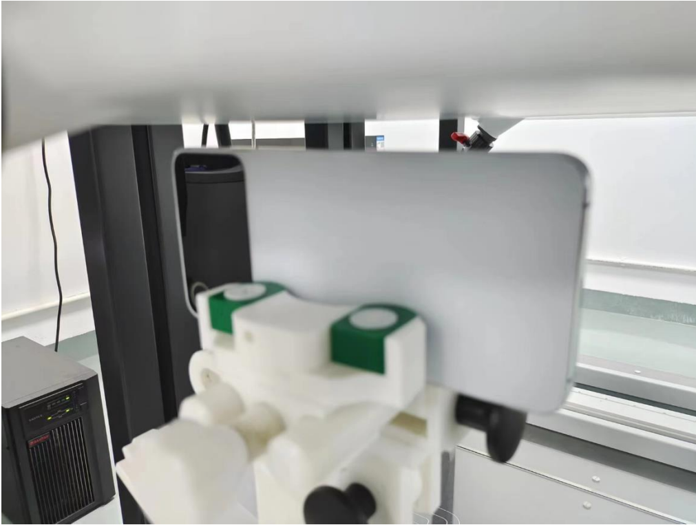
Body Left side (separation distance is 10mm)
