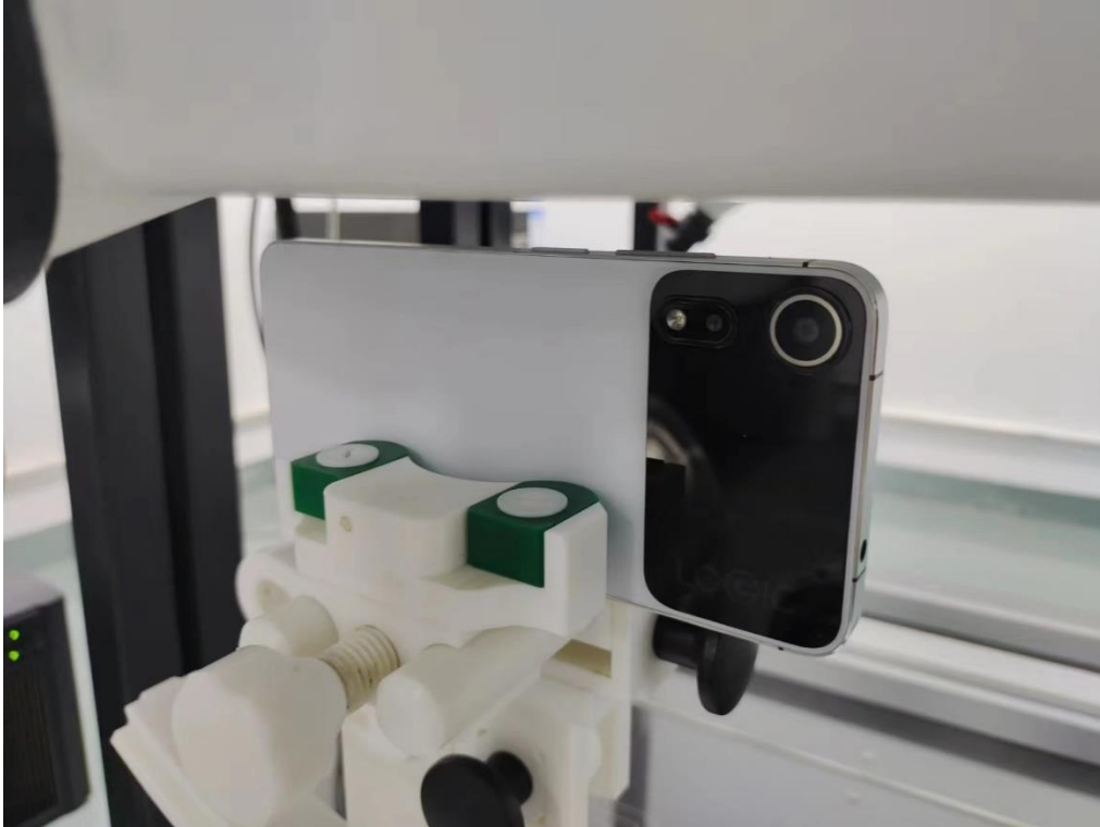
Body Right side (separation distance is 10mm)
