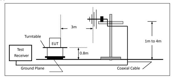
(c) For radiated emissions above 1000MHz
