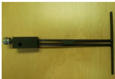
Figure 1 – MVG COMOSAR Validation Dipole
