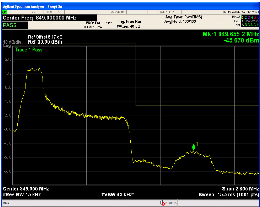
Band5 QPSK BW=1.4MHz Channel=20643 RB Size=1 Position=#Max
