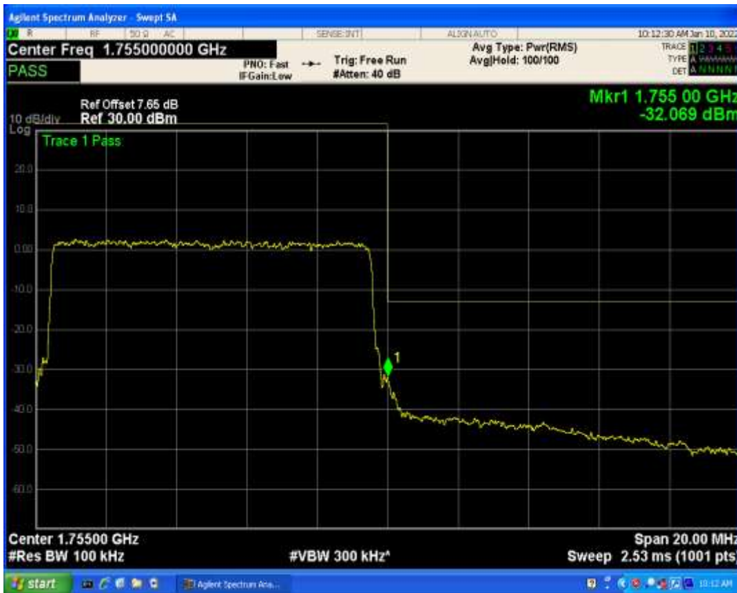
Band4 QAM16 BW=15MHz Channel=20025 RB Size=1 Position=#0
