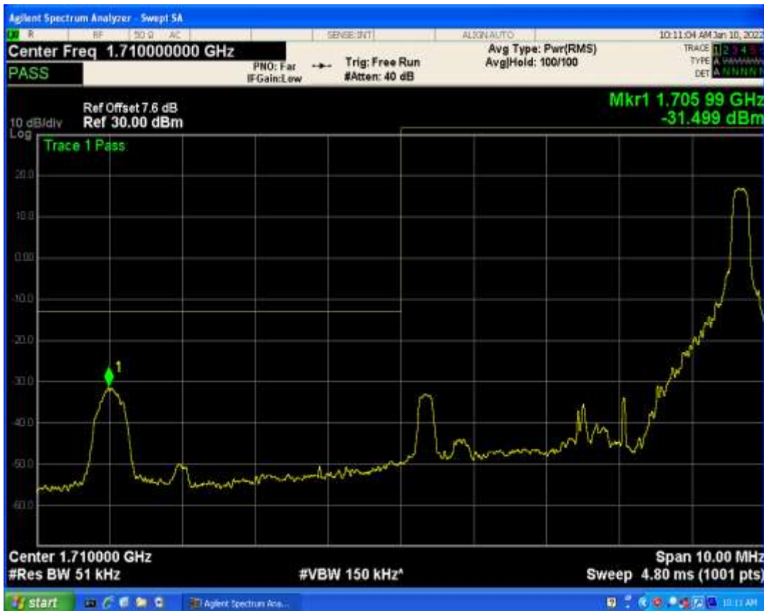
Band4 QPSK BW=3MHz Channel=20385 RB Size=1 Position=#Max
