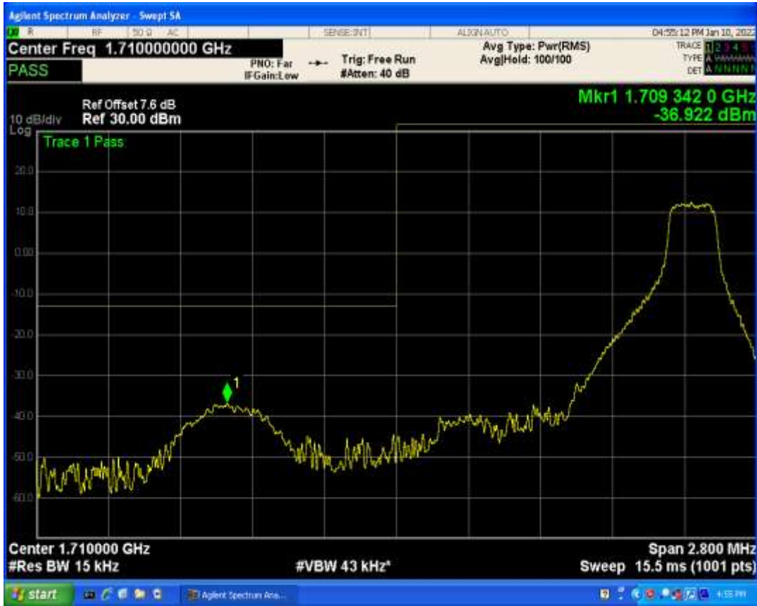
Band66 QPSK BW=1.4MHz Channel=132665 RB Size=1 Position=#0
