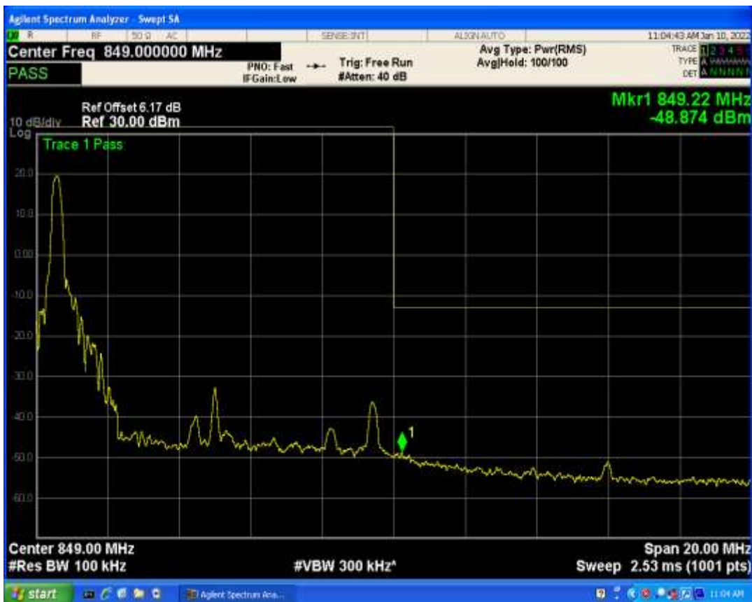
Band5 QPSK BW=5MHz Channel=20625 RB Size=1 Position=#0
