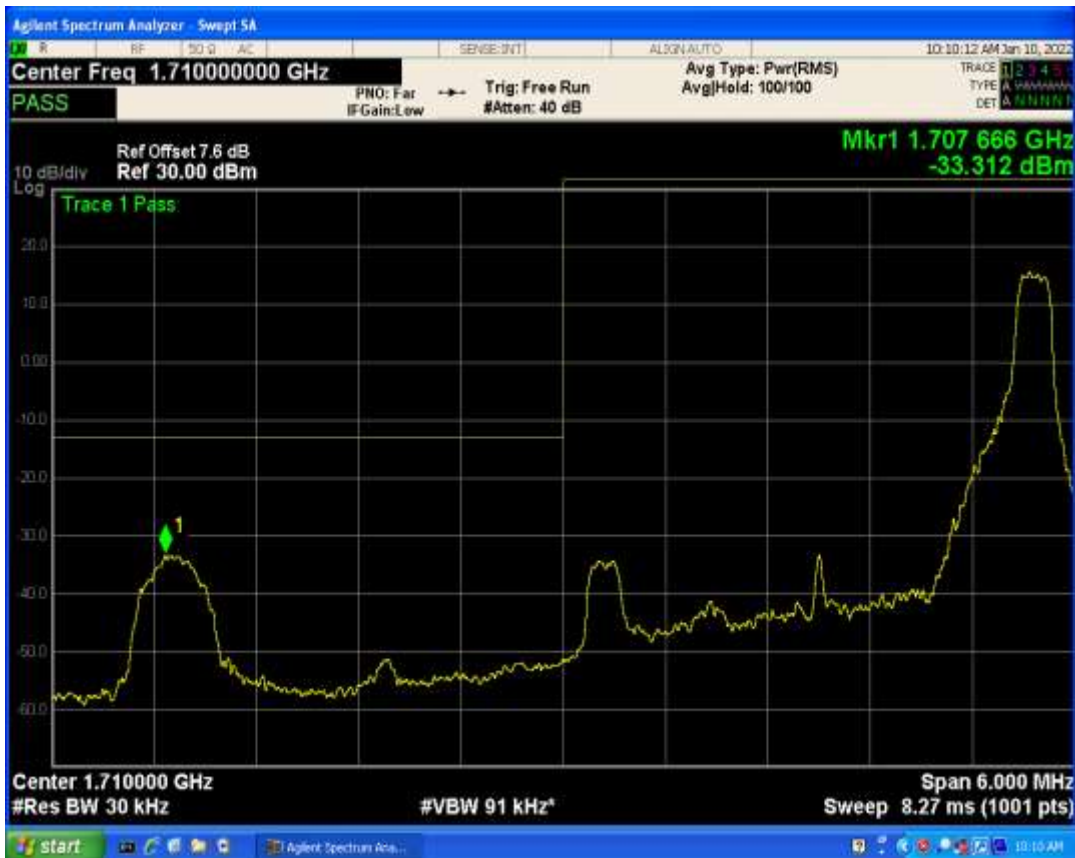
Band4 QPSK BW=20MHz Channel=20050 RB Size=1 Position=#0
