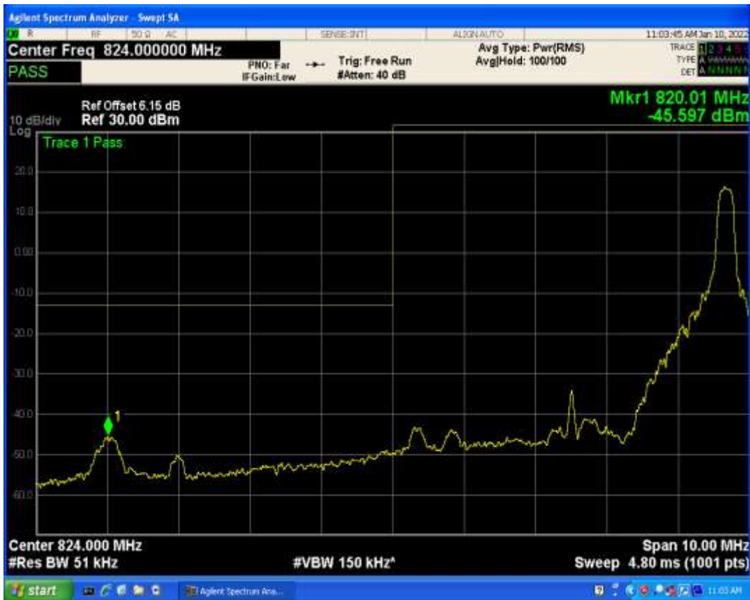
Band5 QAM16 BW=5MHz Channel=20625 RB Size=1 Position=#0
