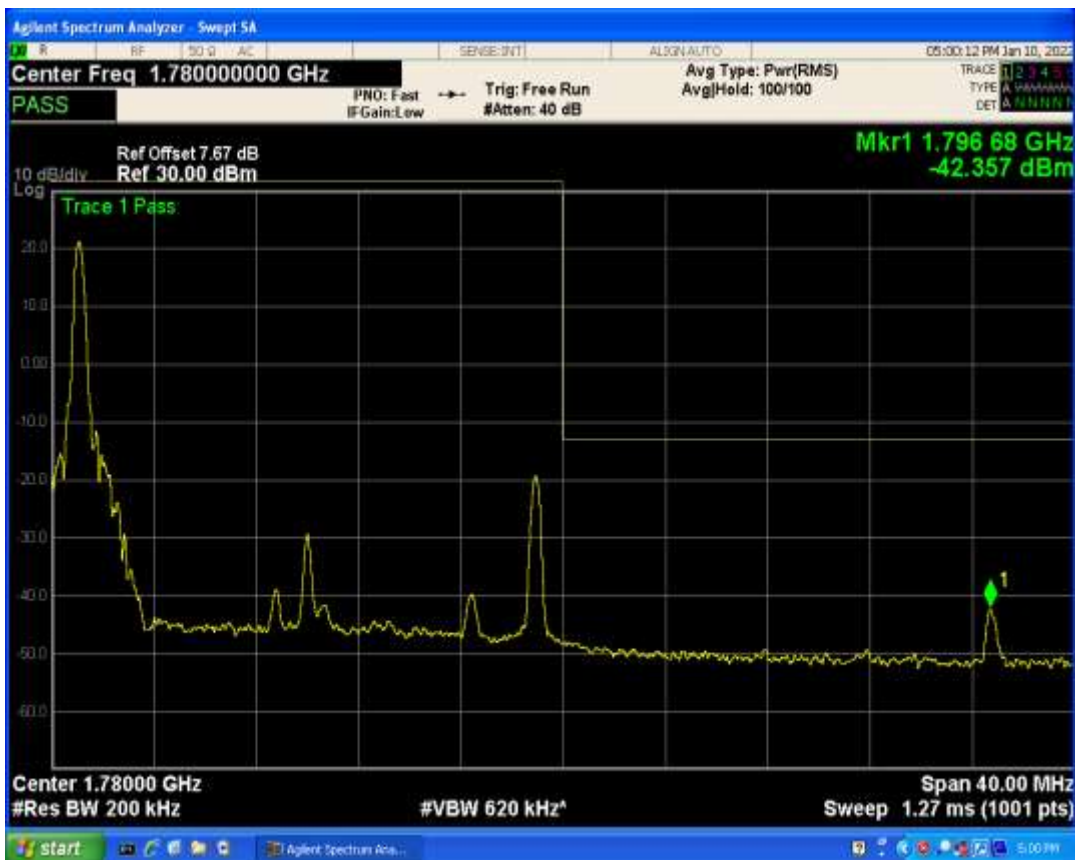
Band66 QAM16 BW=20MHz Channel=132572 RB Size=100 Position=#0
