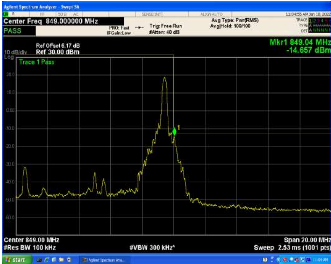
Band5 QAM16 BW=3MHz Channel=20415 RB Size=1 Position=#Max
