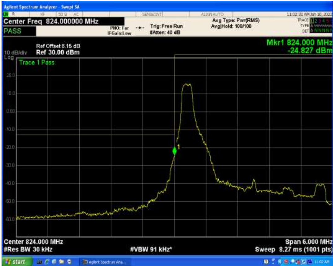
Band5 QPSK BW=10MHz Channel=20600 RB Size=50 Position=#0
