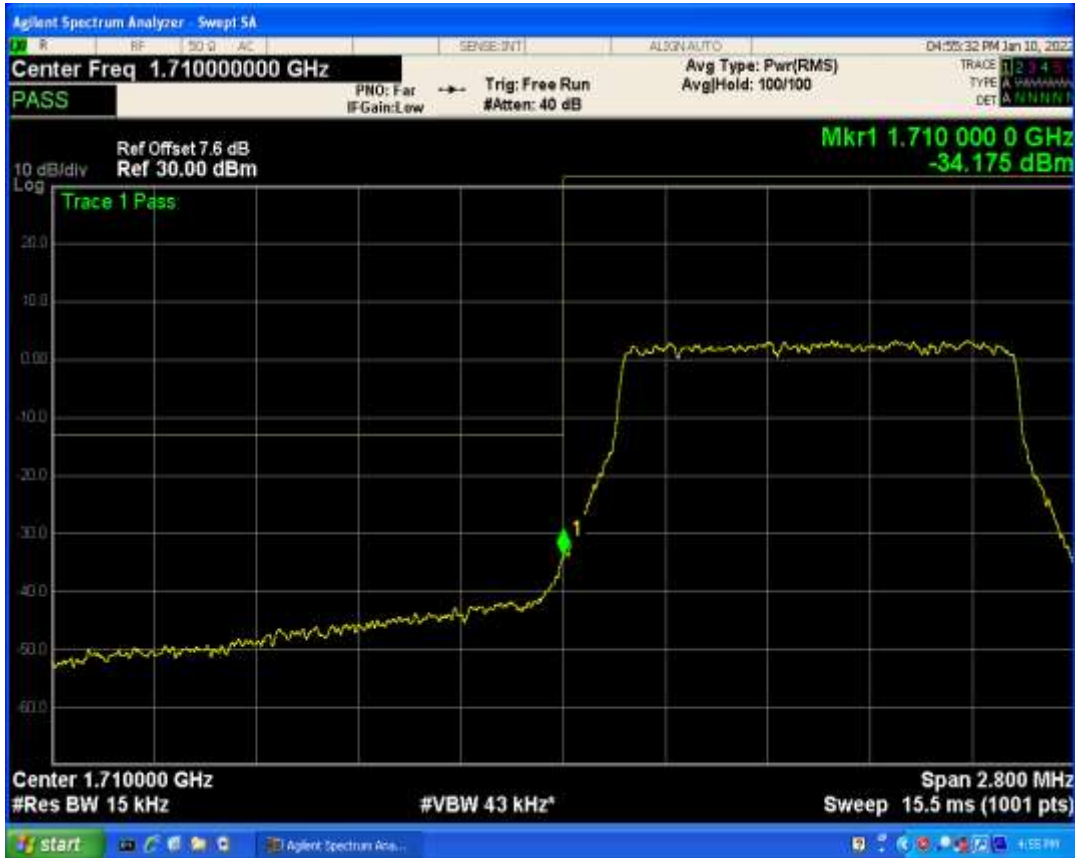
Band66 QAM16 BW=1.4MHz Channel=131979 RB Size=1 Position=#Max
