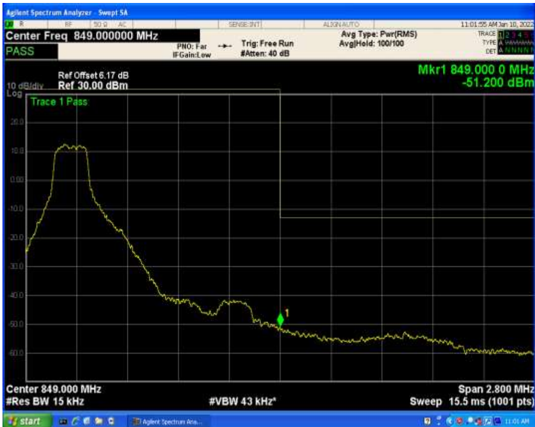
Band5 QPSK BW=1.4MHz Channel=20643 RB Size=6 Position=#0
