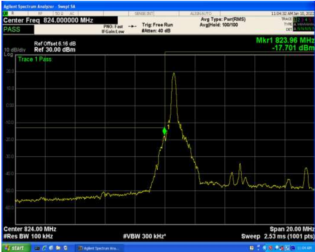
Band5 QAM16 BW=10MHz Channel=20600 RB Size=1 Position=#0
