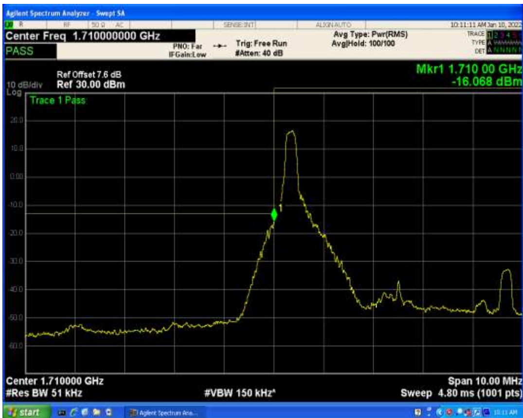
Band4 QAM16 BW=3MHz Channel=20385 RB Size=15 Position=#0
