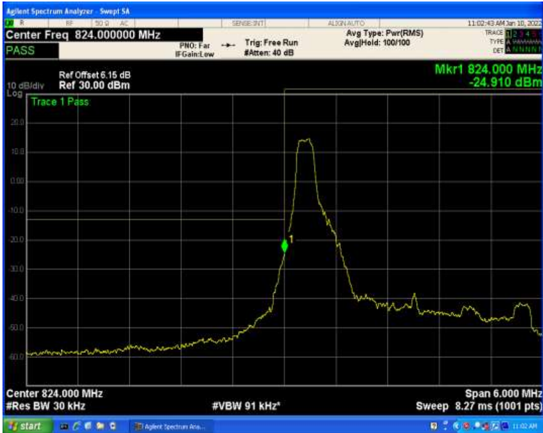
Band5 QPSK BW=1.4MHz Channel=20407 RB Size=6 Position=#0
