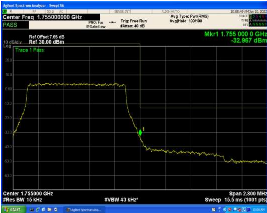
Band4 QPSK BW=10MHz Channel=20000 RB Size=1 Position=#Max
