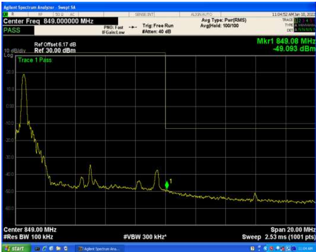
Band5 QAM16 BW=10MHz Channel=20450 RB Size=50 Position=#0
