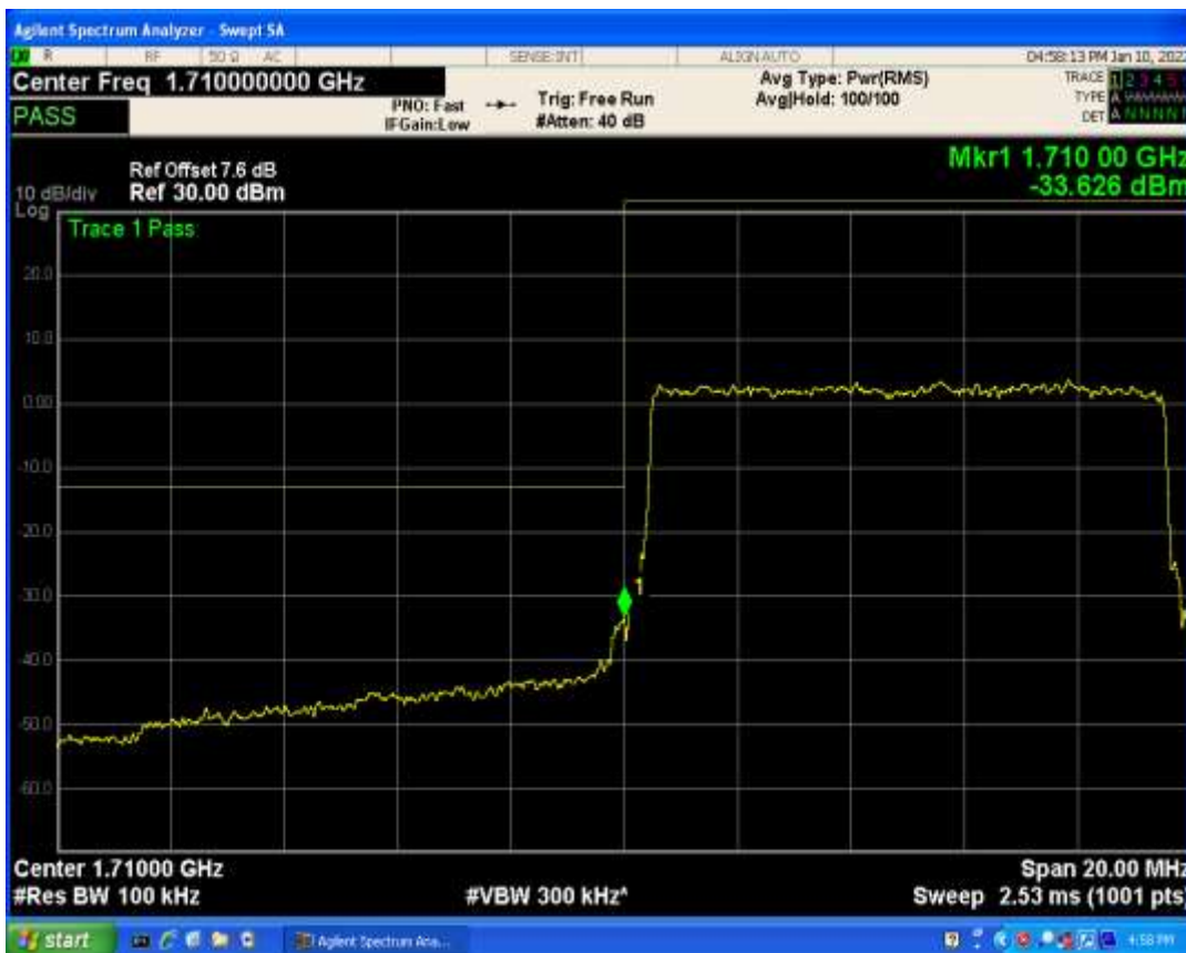
Band66 QPSK BW=10MHz Channel=132622 RB Size=1 Position=#Max
