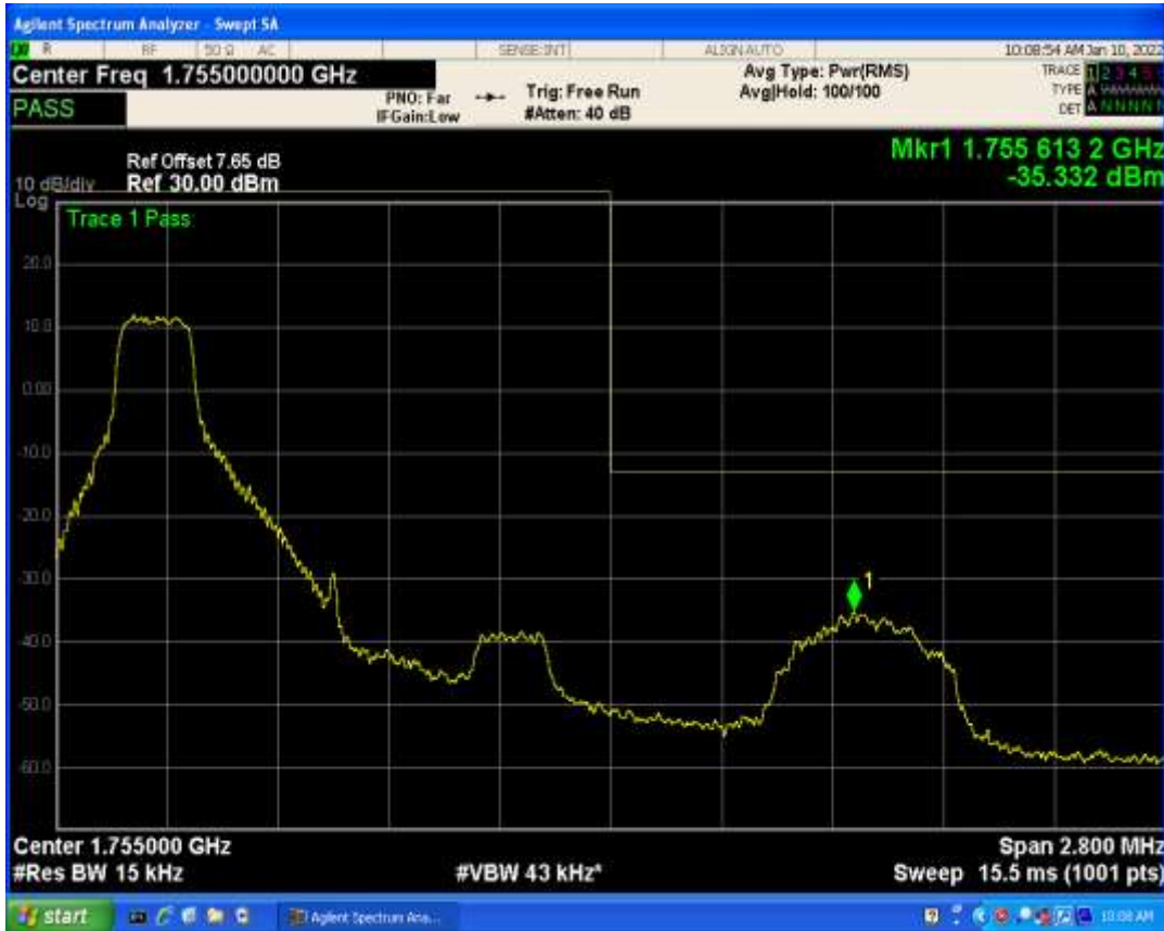
Band4 QAM16 BW=1.4MHz Channel=19957 RB Size=6 Position=#0
