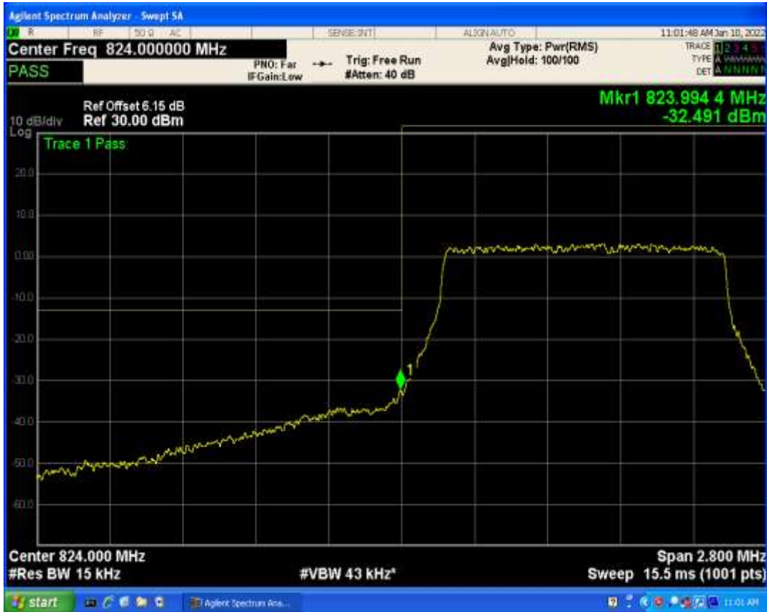
Band5 QAM16 BW=1.4MHz Channel=20407 RB Size=1 Position=#Max
