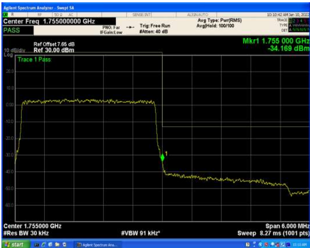
Band5 QAM16 BW=1.4MHz Channel=20407 RB Size=1 Position=#0
