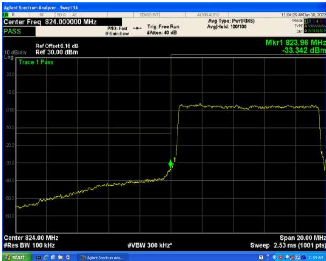
Band5 QPSK BW=10MHz Channel=20600 RB Size=1 Position=#Max
