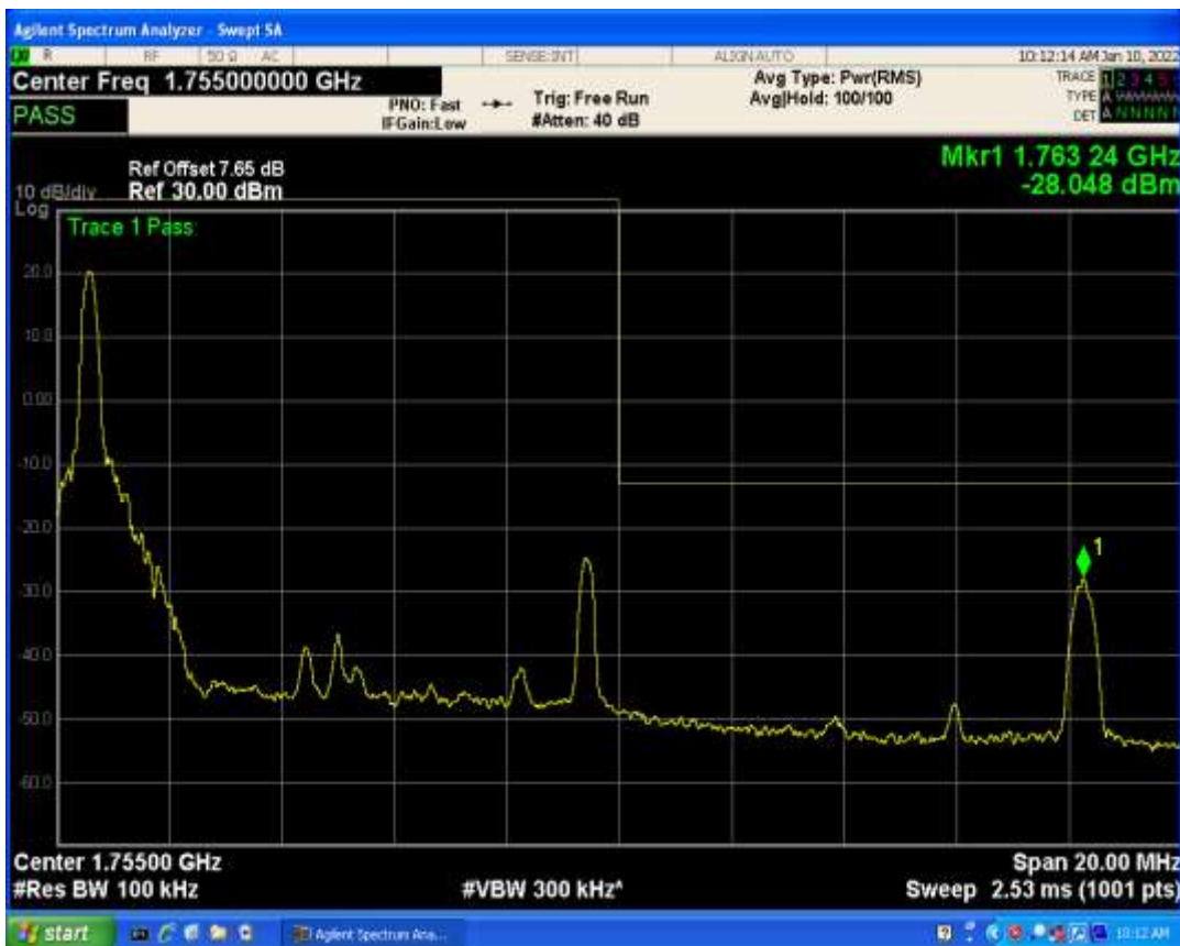
Band4 QPSK BW=10MHz Channel=20000 RB Size=50 Position=#0
