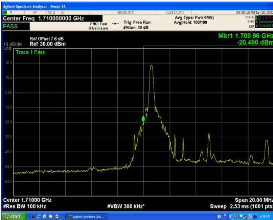
Band66 QAM16 BW=10MHz Channel=132022 RB Size=50 Position=#0
