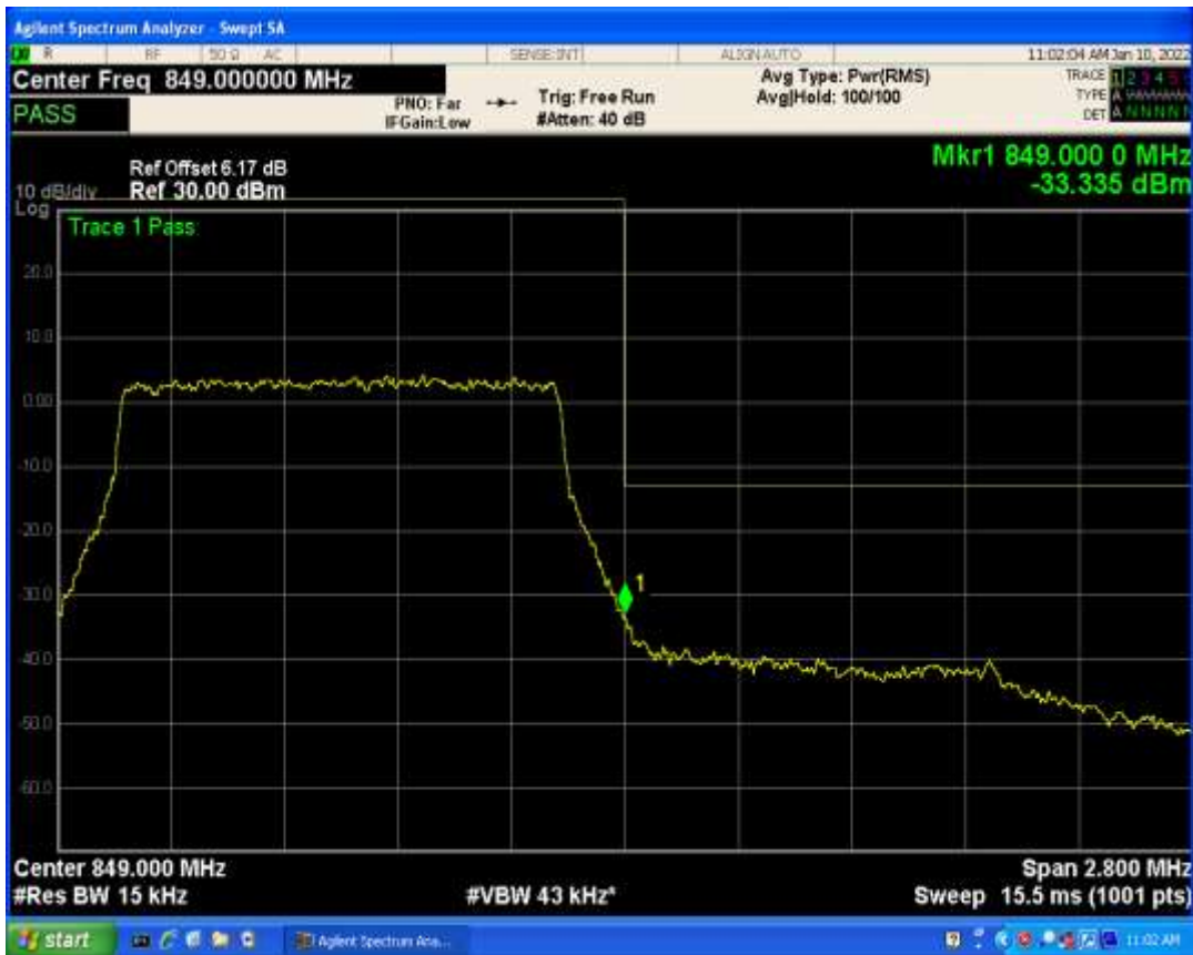
Band5 QPSK BW=1.4MHz Channel=20643 RB Size=1 Position=#Max
