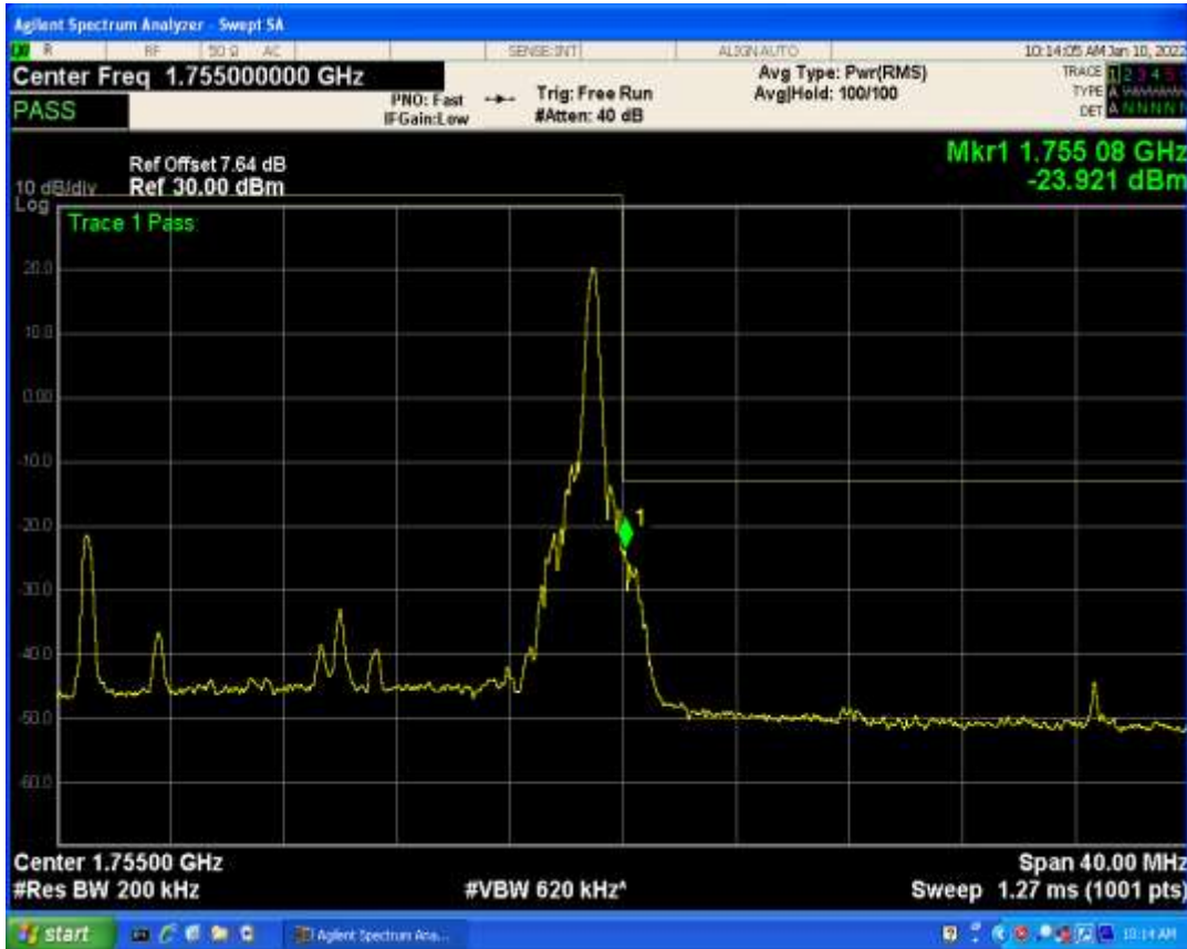
Band4 QAM16 BW=20MHz Channel=20300 RB Size=1 Position=#0
