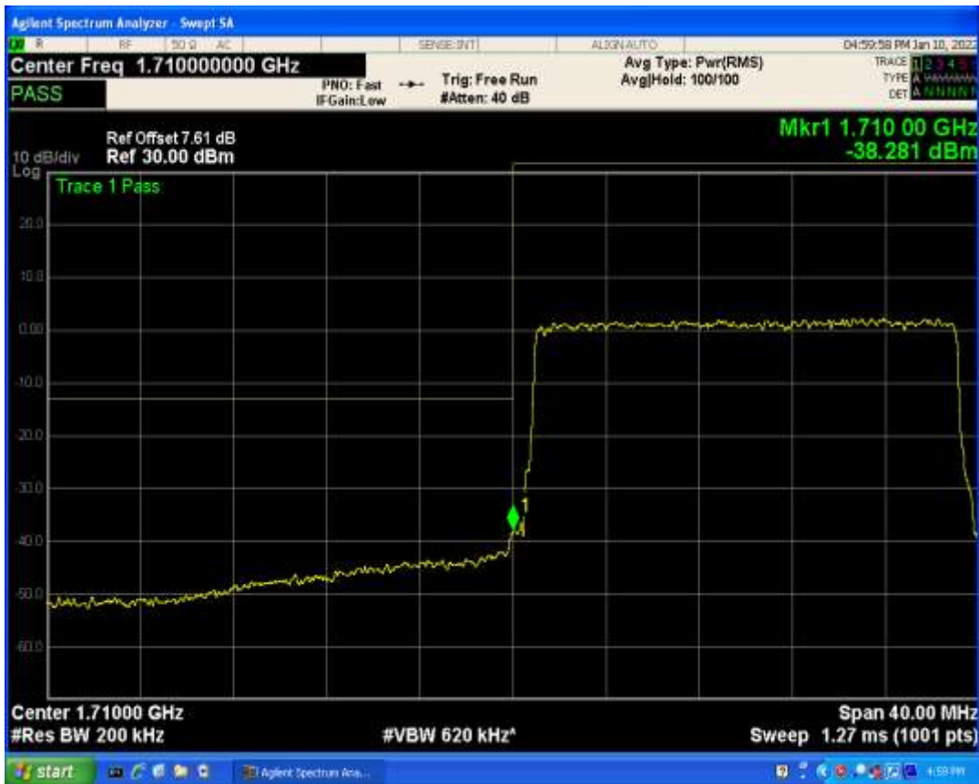
Band66 QAM16 BW=20MHz Channel=132072 RB Size=1 Position=#Max
