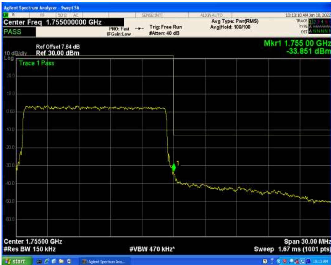
Band4 QPSK BW=20MHz Channel=20050 RB Size=1 Position=#Max
