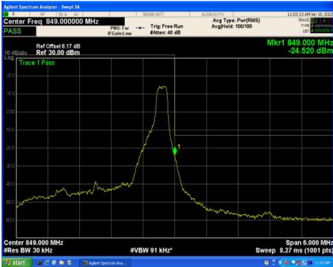
Band5 QAM16 BW=3MHz Channel=20635 RB Size=1 Position=#0
