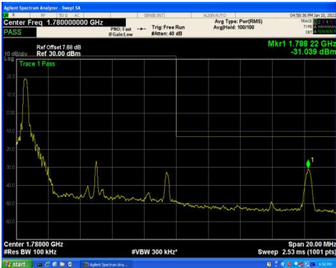
Band66 QAM16 BW=1.4MHz Channel=131979 RB Size=6 Position=#0
