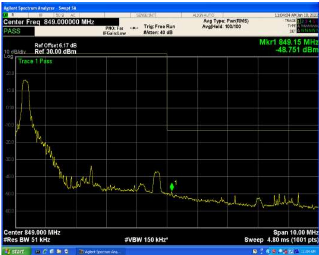
Band5 QAM16 BW=5MHz Channel=20625 RB Size=25 Position=#0
