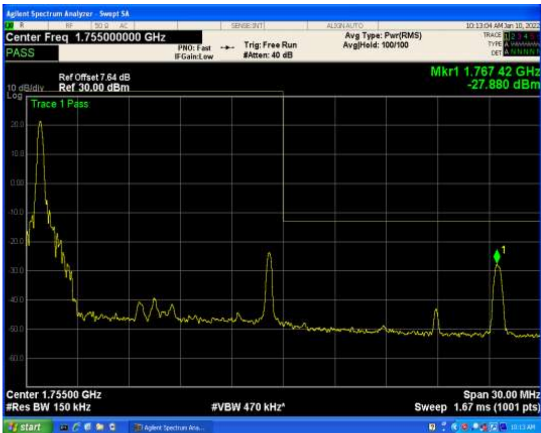
Band4 QPSK BW=15MHz Channel=20025 RB Size=1 Position=#0
