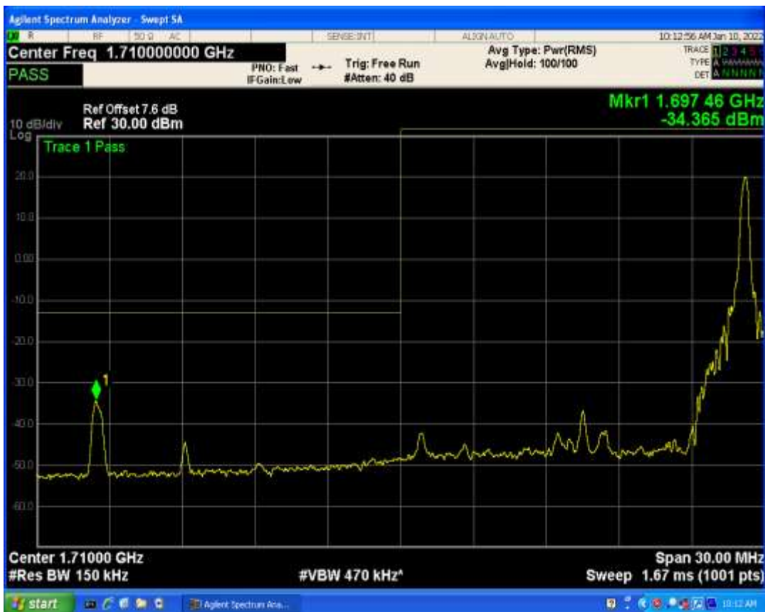
Band4 QAM16 BW=15MHz Channel=20325 RB Size=1 Position=#0
