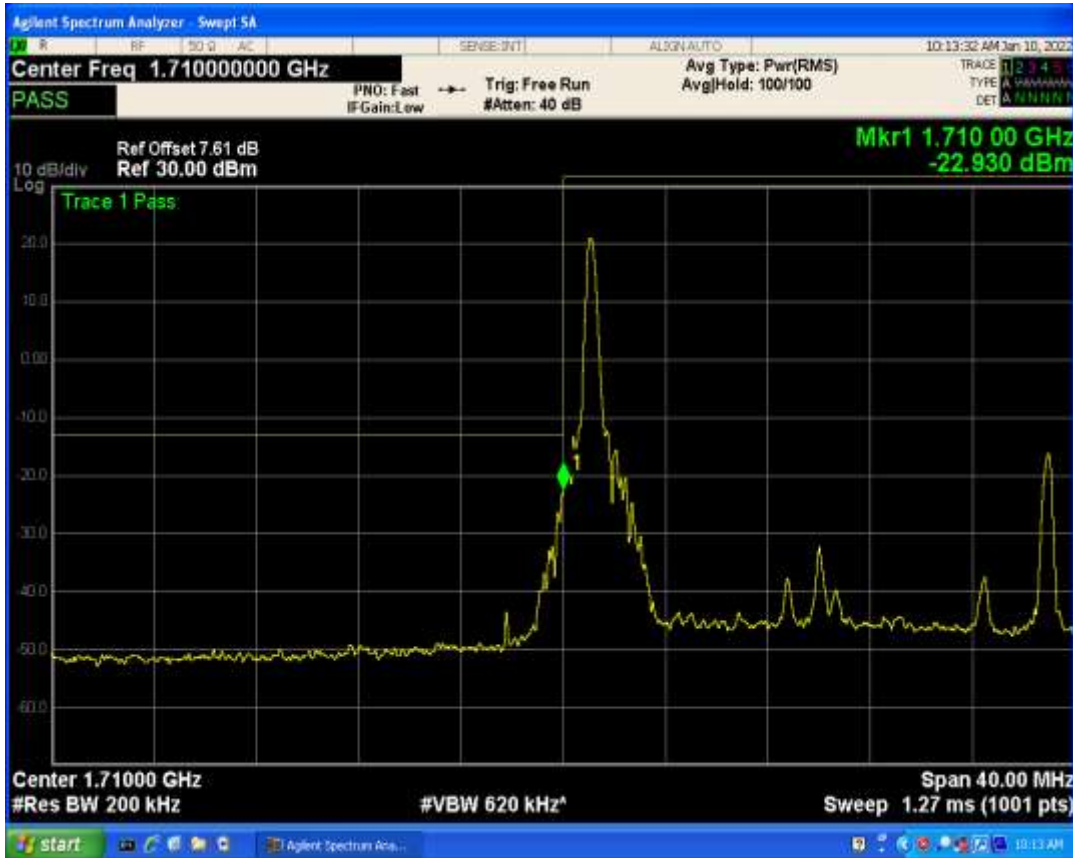
Band4 QPSK BW=15MHz Channel=20325 RB Size=75 Position=#0
