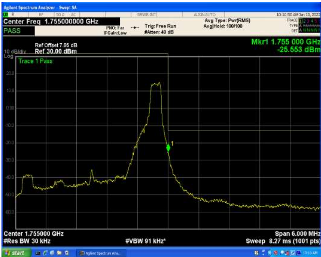
Band4 QAM16 BW=3MHz Channel=19965 RB Size=1 Position=#0
