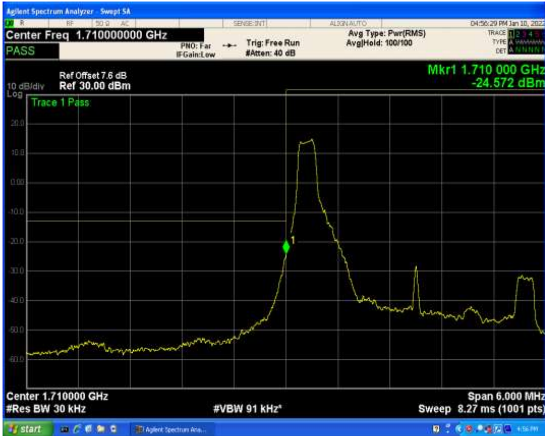
Band66 QPSK BW=1.4MHz Channel=131979 RB Size=6 Position=#0
