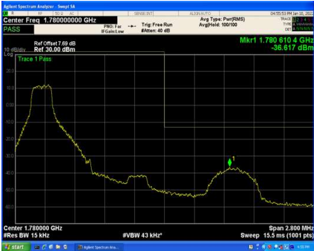
Band66 QAM16 BW=1.4MHz Channel=132665 RB Size=6 Position=#0
