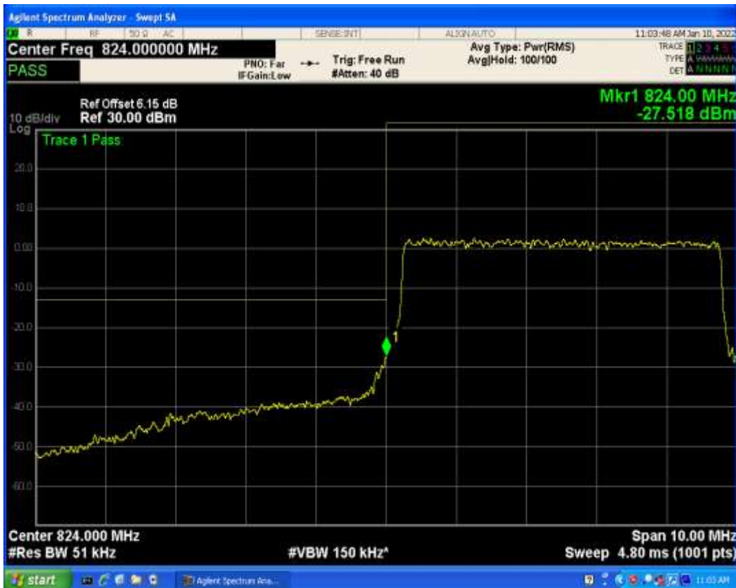
Band5 QAM16 BW=5MHz Channel=20425 RB Size=1 Position=#Max
