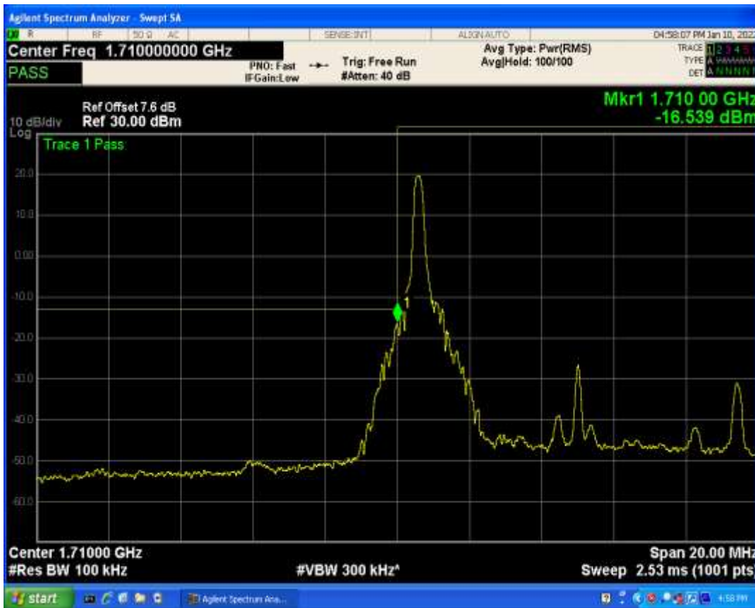
Band66 QPSK BW=10MHz Channel=132022 RB Size=50 Position=#0
