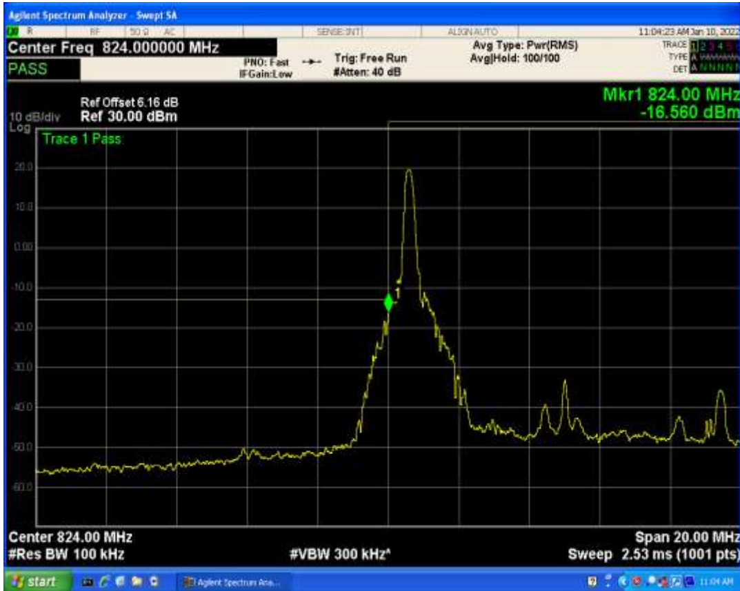
Band5 QPSK BW=10MHz Channel=20450 RB Size=50 Position=#0
