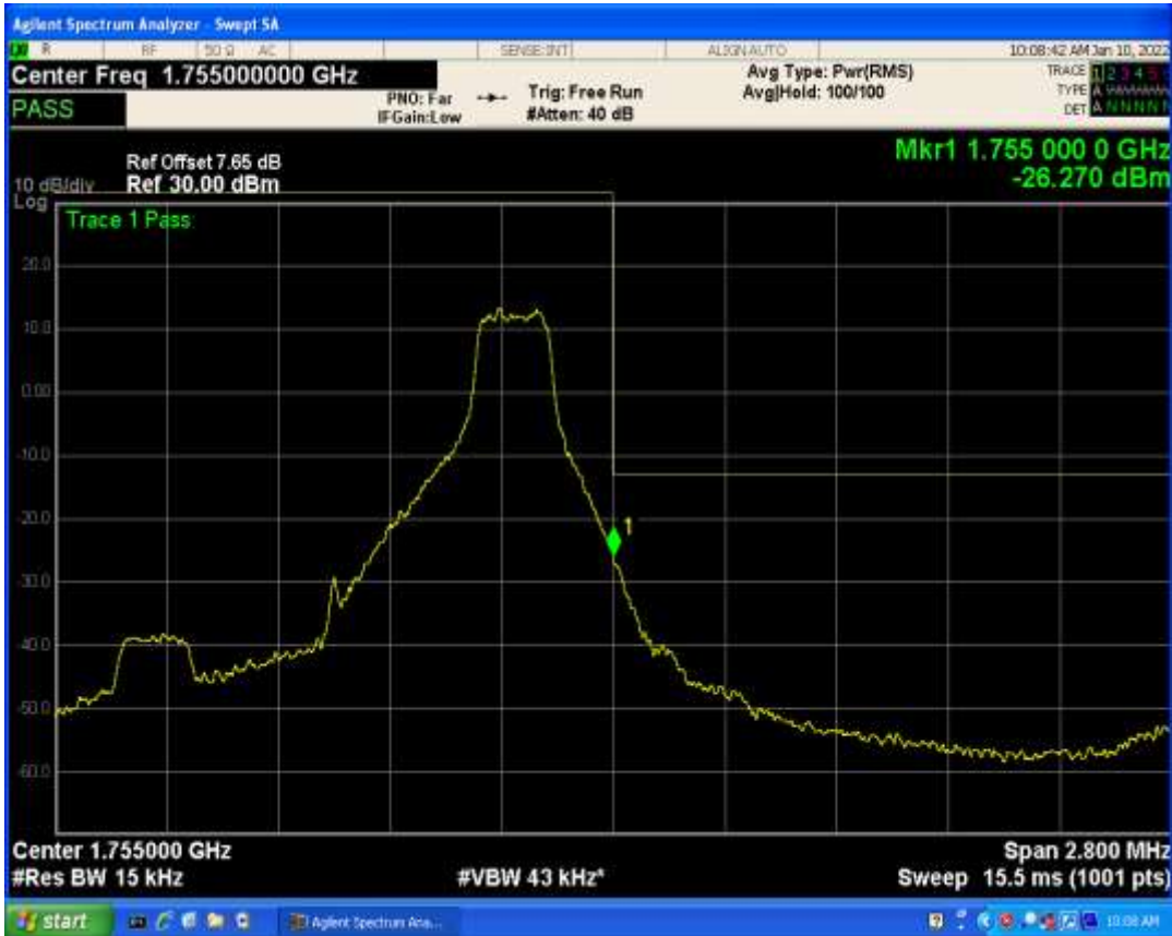
Band4 QPSK BW=1.4MHz Channel=20393 RB Size=1 Position=#0
