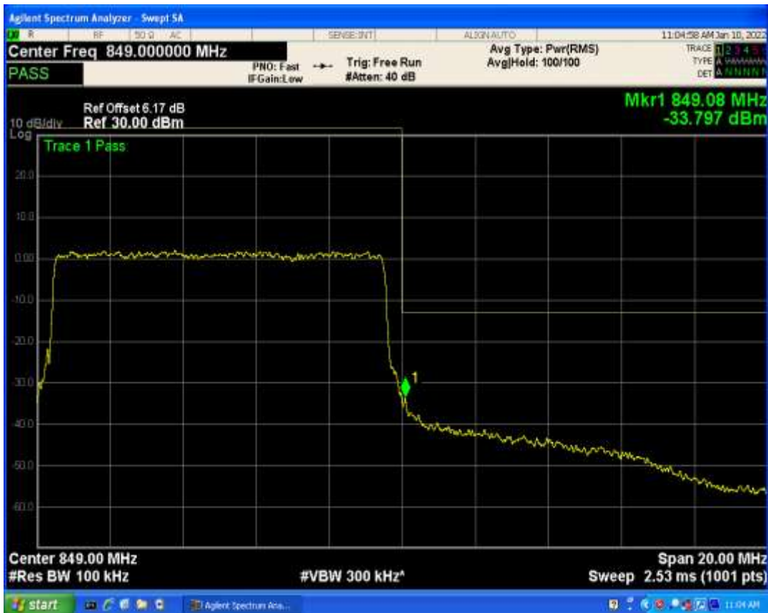
Band5 QAM16 BW=10MHz Channel=20600 RB Size=1 Position=#Max
