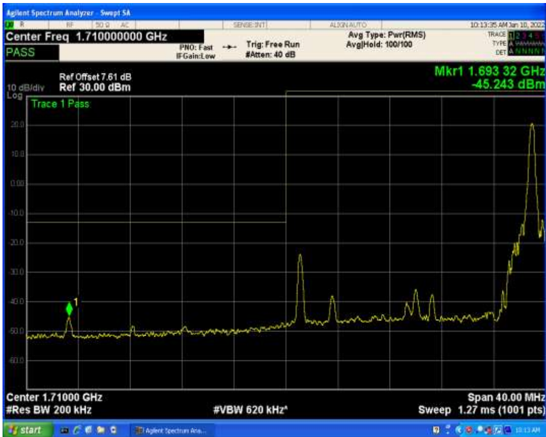
Band4 QPSK BW=20MHz Channel=20300 RB Size=1 Position=#0
