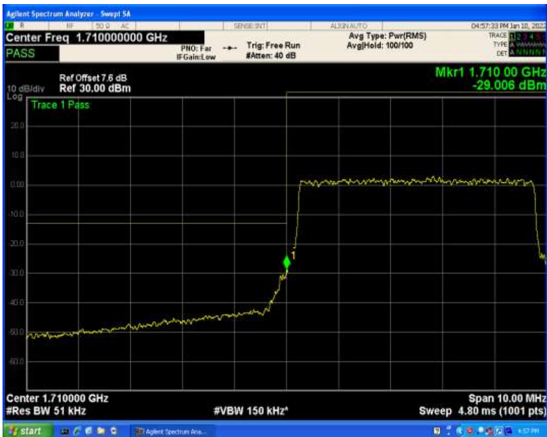
Band66 QAM16 BW=5MHz Channel=131997 RB Size=1 Position=#Max
