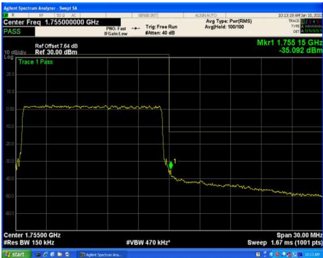
Band4 QAM16 BW=15MHz Channel=20325 RB Size=1 Position=#Max
