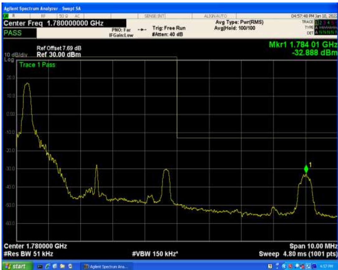
Band66 QAM16 BW=5MHz Channel=132647 RB Size=25 Position=#0
