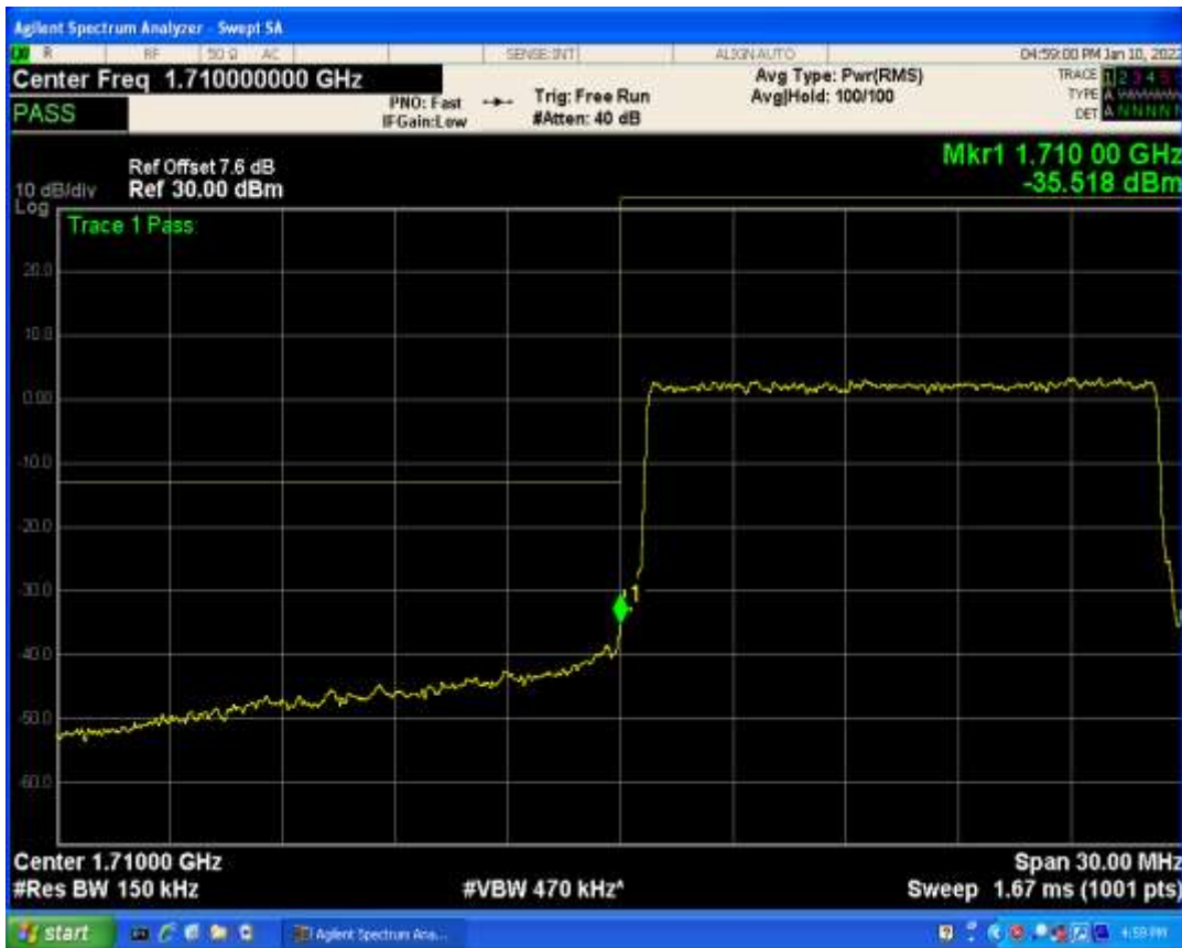
Band66 QPSK BW=10MHz Channel=132022 RB Size=1 Position=#Max
