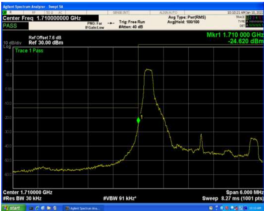
Band4 QAM16 BW=20MHz Channel=20300 RB Size=100 Position=#0
