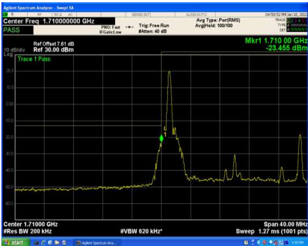
Band66 QAM16 BW=20MHz Channel=132072 RB Size=100 Position=#0
