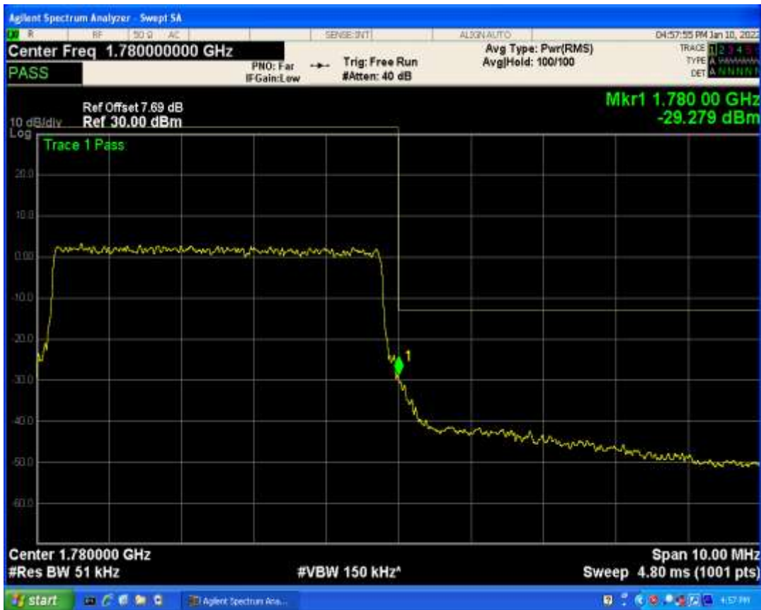
Band66 QAM16 BW=5MHz Channel=132647 RB Size=1 Position=#Max
