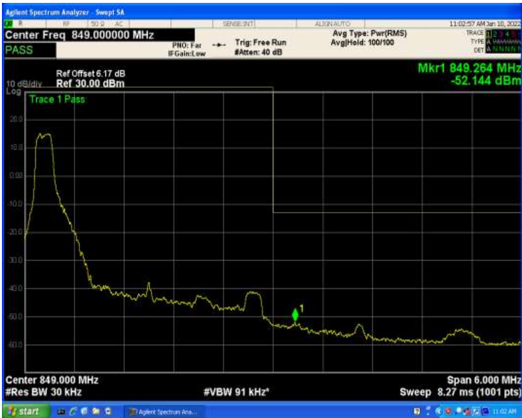
Band5 QPSK BW=3MHz Channel=20415 RB Size=15 Position=#0
