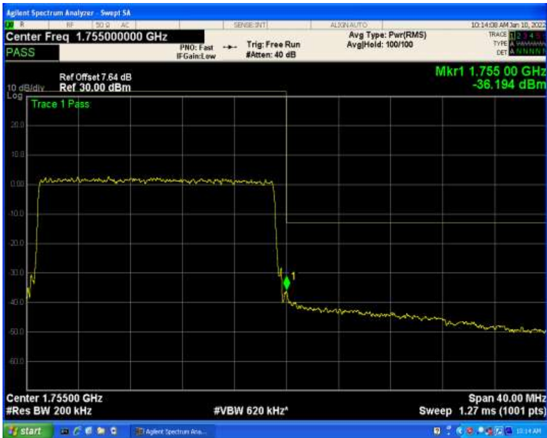
Band4 QAM16 BW=3MHz Channel=19965 RB Size=1 Position=#Max
