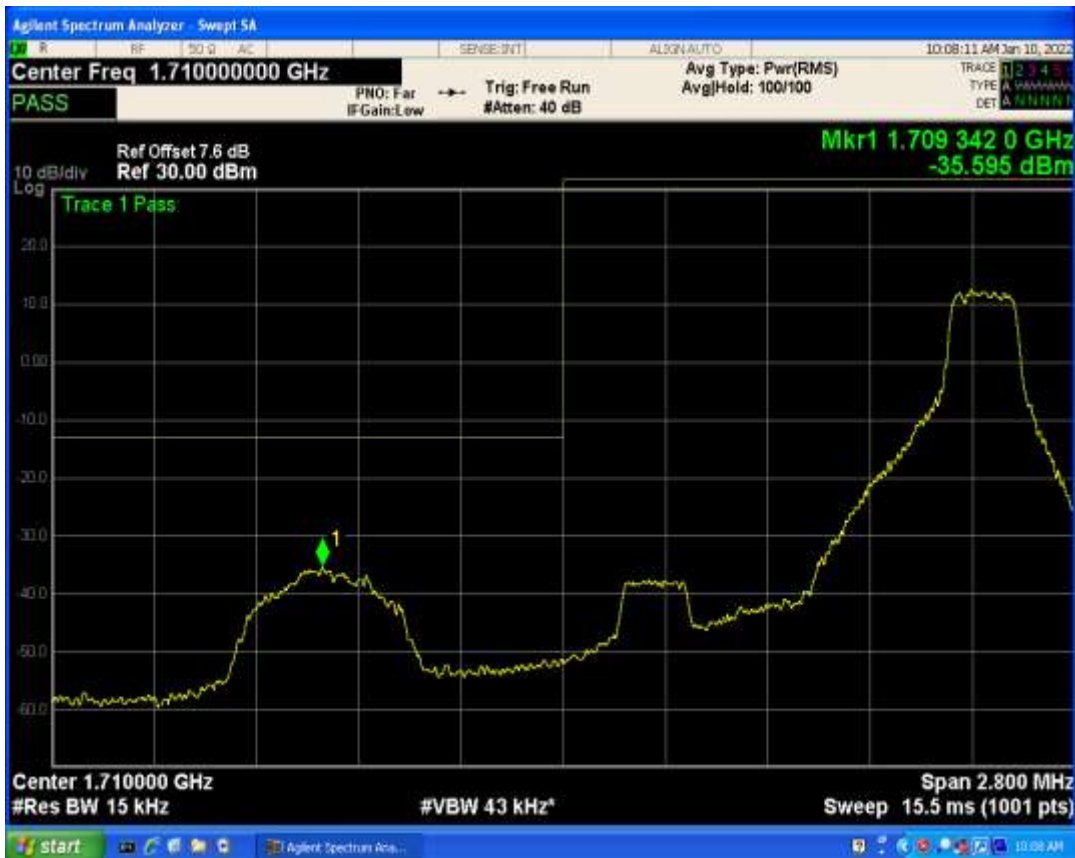
Band4 QPSK BW=15MHz Channel=20025 RB Size=75 Position=#0
