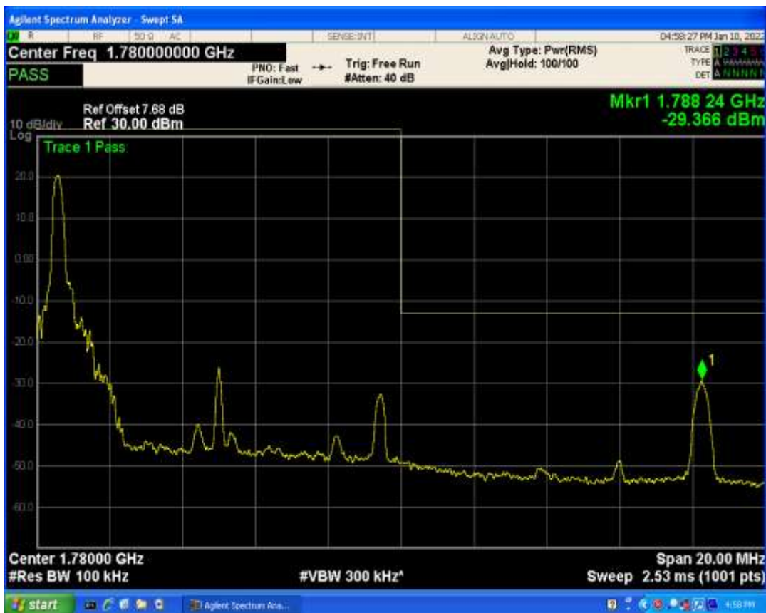
Band66 QPSK BW=20MHz Channel=132572 RB Size=1 Position=#Max
