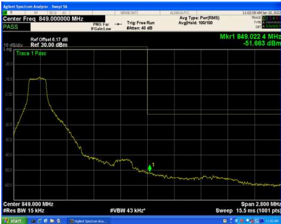
Band5 QAM16 BW=3MHz Channel=20635 RB Size=1 Position=#Max
