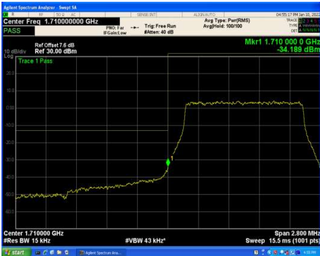
Band66 QPSK BW=1.4MHz Channel=131979 RB Size=1 Position=#Max
