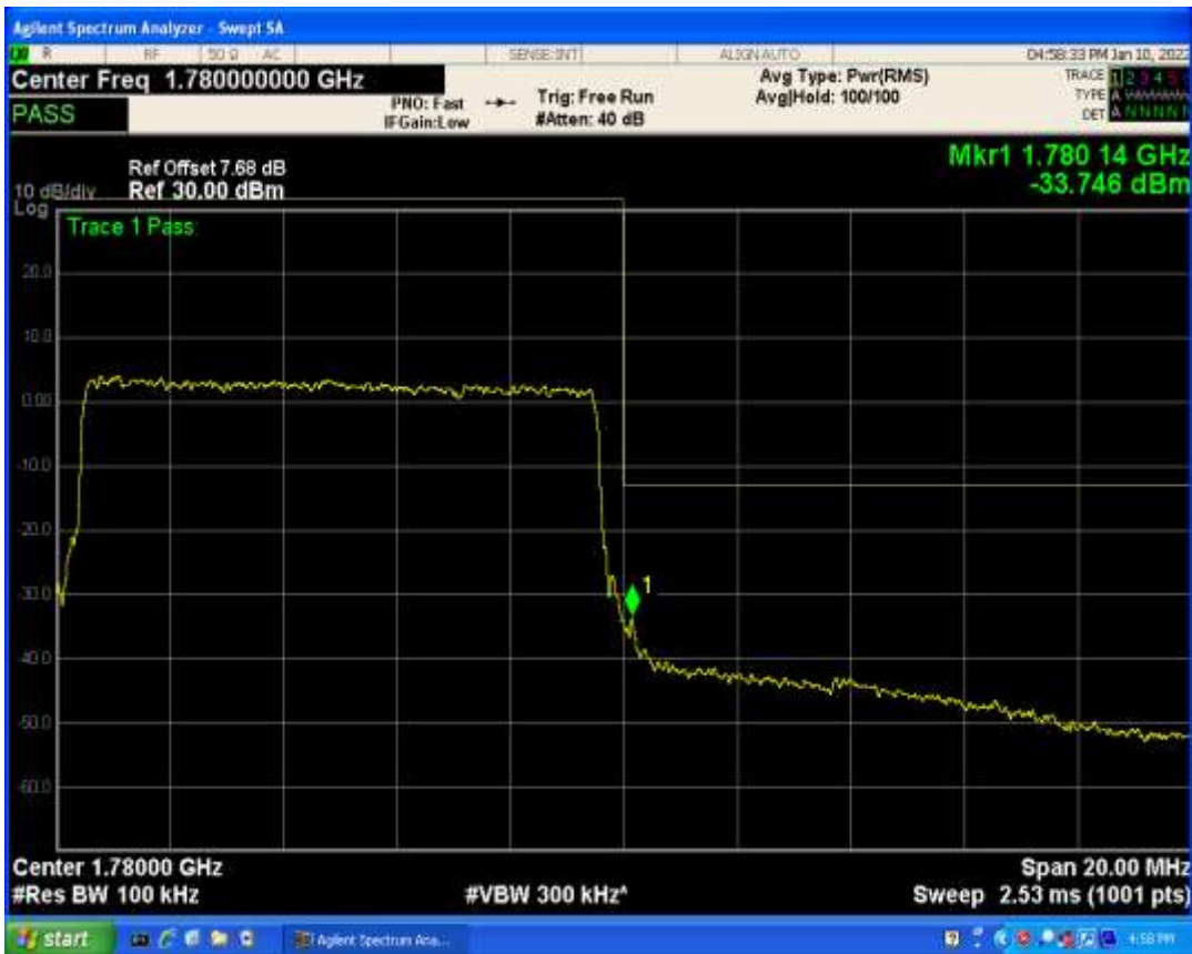
Band66 QPSK BW=15MHz Channel=132047 RB Size=1 Position=#Max
