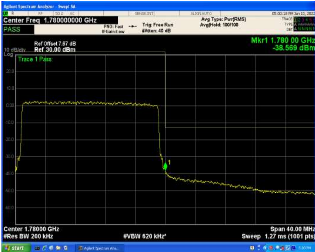
Band66 QAM16 BW=3MHz Channel=131987 RB Size=1 Position=#Max
