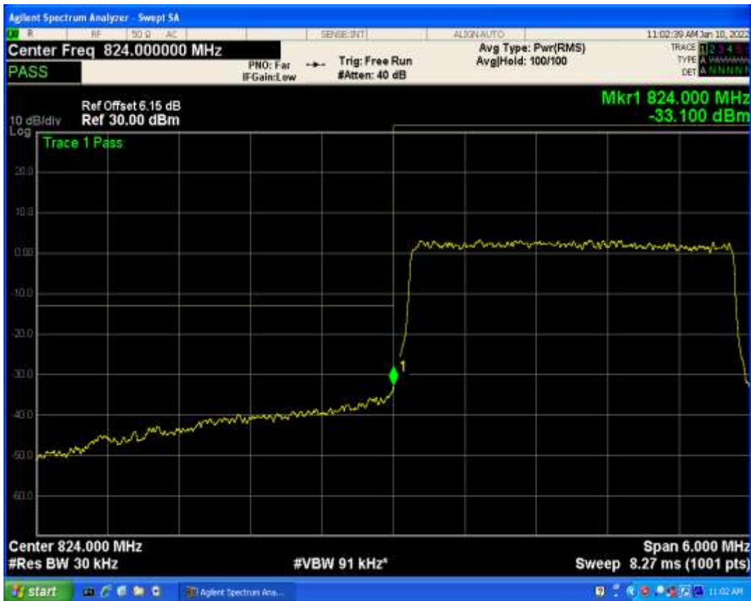
Band5 QPSK BW=10MHz Channel=20450 RB Size=1 Position=#Max
