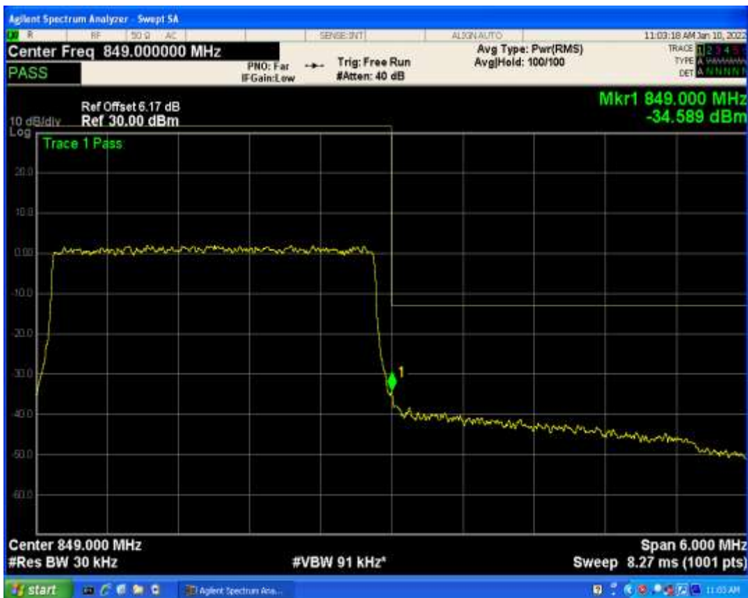
Band5 QAM16 BW=3MHz Channel=20415 RB Size=15 Position=#0
