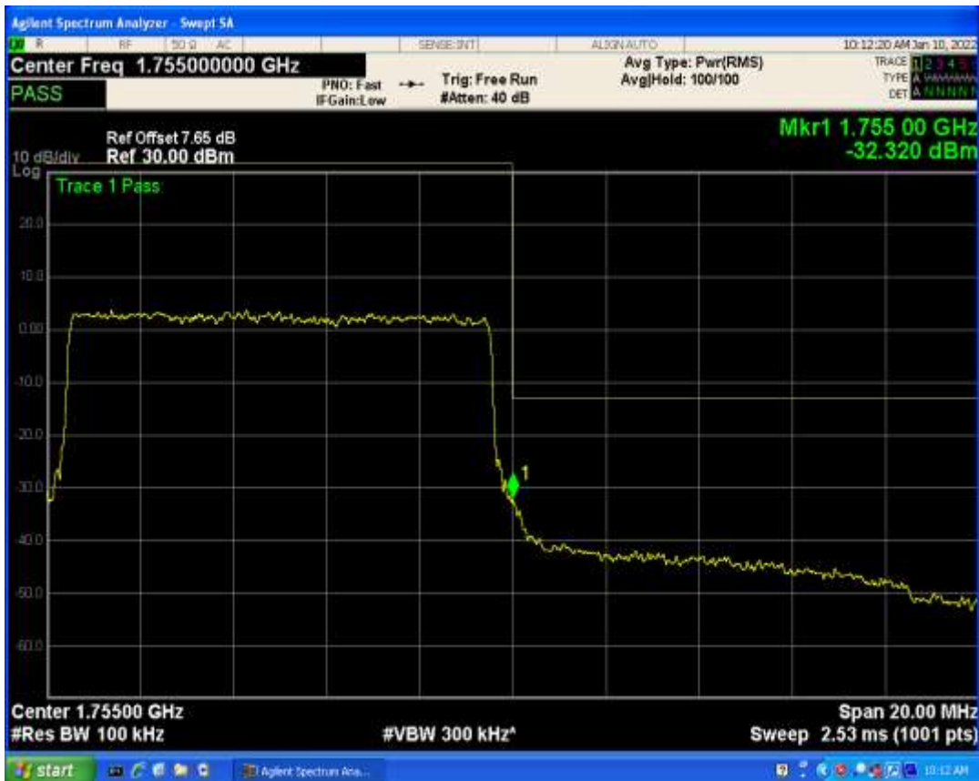
Band4 QPSK BW=10MHz Channel=20350 RB Size=1 Position=#Max
