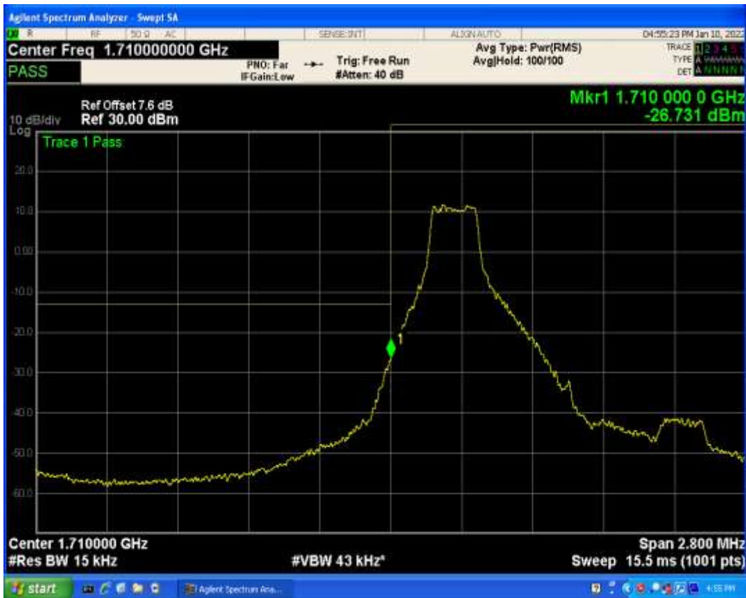
Band66 QAM16 BW=10MHz Channel=132022 RB Size=1 Position=#Max
