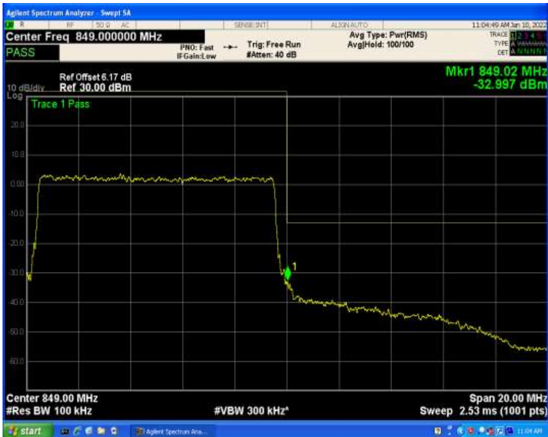
Band5 QPSK BW=3MHz Channel=20415 RB Size=1 Position=#Max
