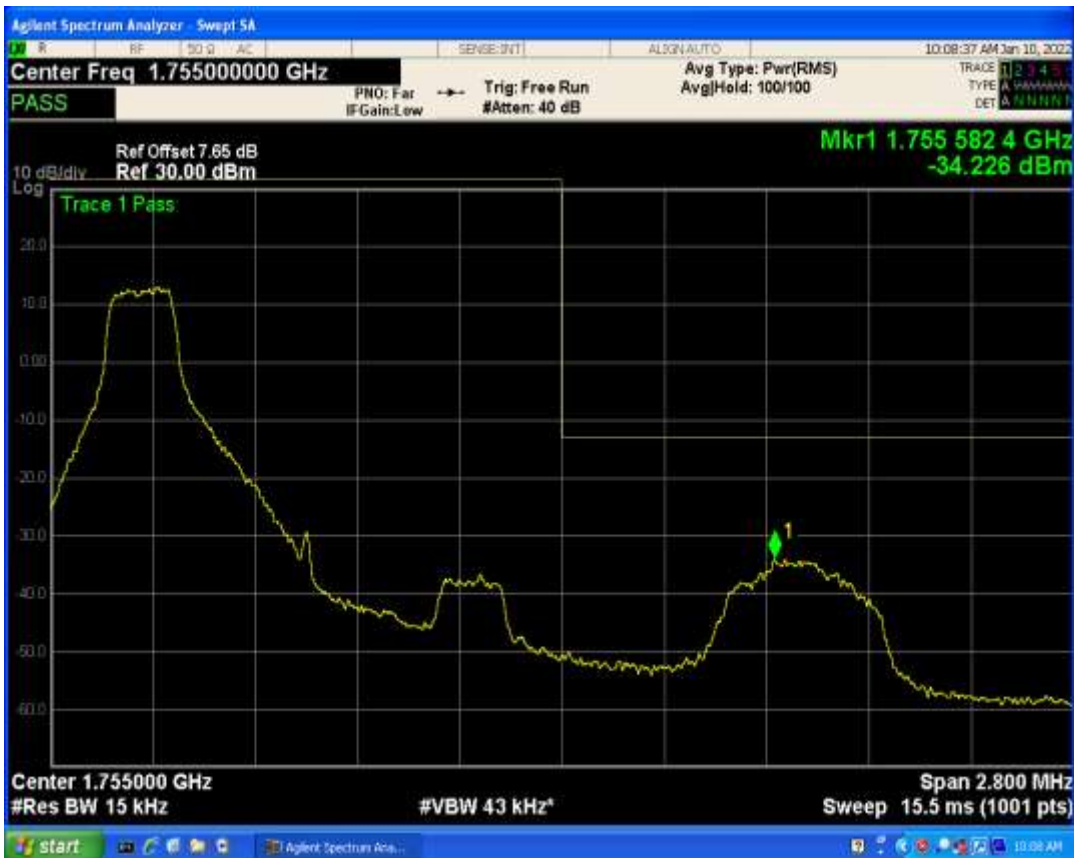
Band4 QPSK BW=1.4MHz Channel=20393 RB Size=6 Position=#0
