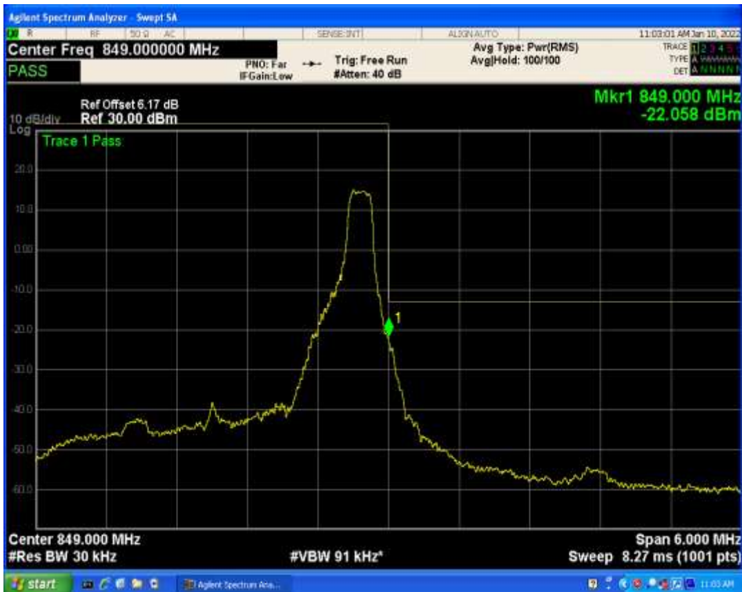
Band5 QPSK BW=5MHz Channel=20425 RB Size=1 Position=#Max
