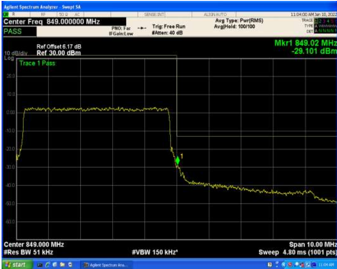
Band5 QPSK BW=5MHz Channel=20625 RB Size=1 Position=#Max
