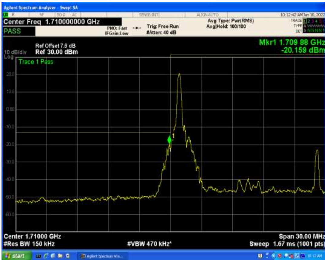
Band4 QPSK BW=10MHz Channel=20350 RB Size=1 Position=#0
