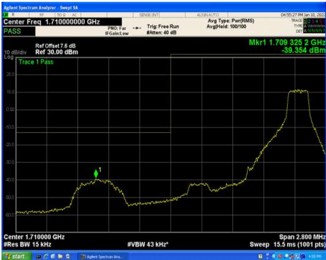
Band66 QAM16 BW=1.4MHz Channel=132665 RB Size=1 Position=#0
