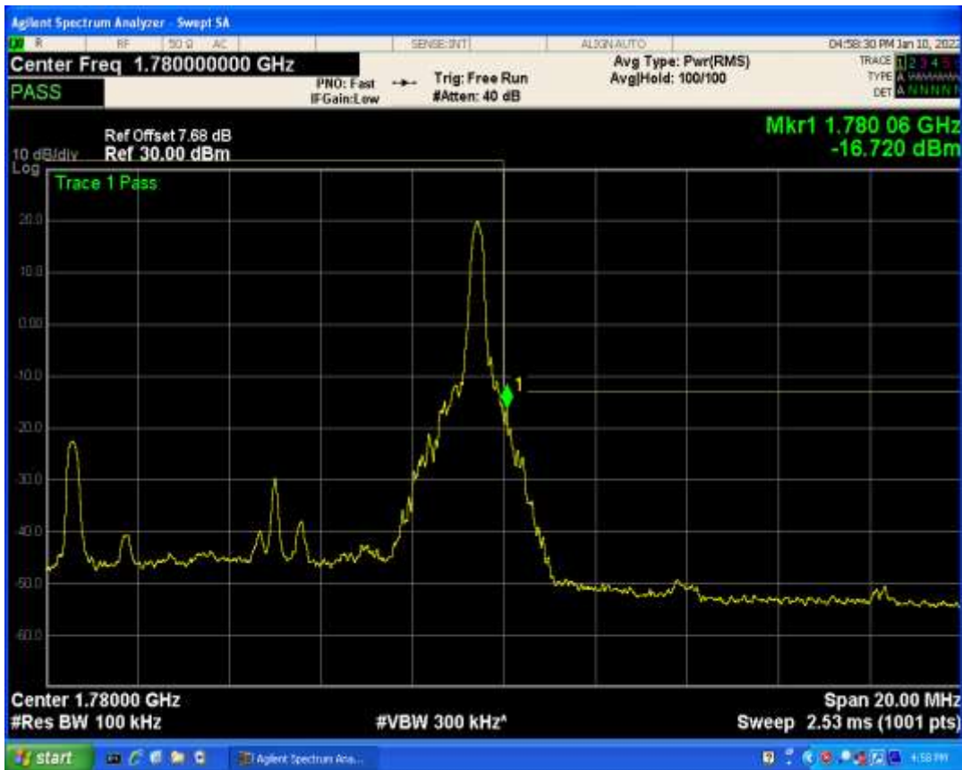
Band66 QPSK BW=10MHz Channel=132622 RB Size=1 Position=#0
