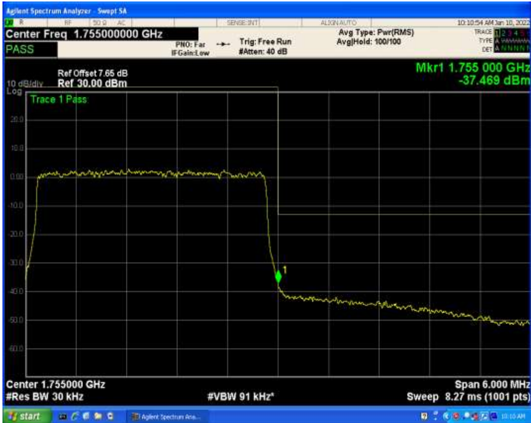
Band4 QAM16 BW=5MHz Channel=19975 RB Size=1 Position=#Max
