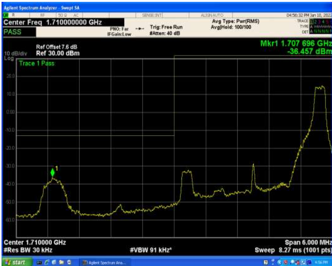
Band66 QAM16 BW=3MHz Channel=131987 RB Size=1 Position=#0
