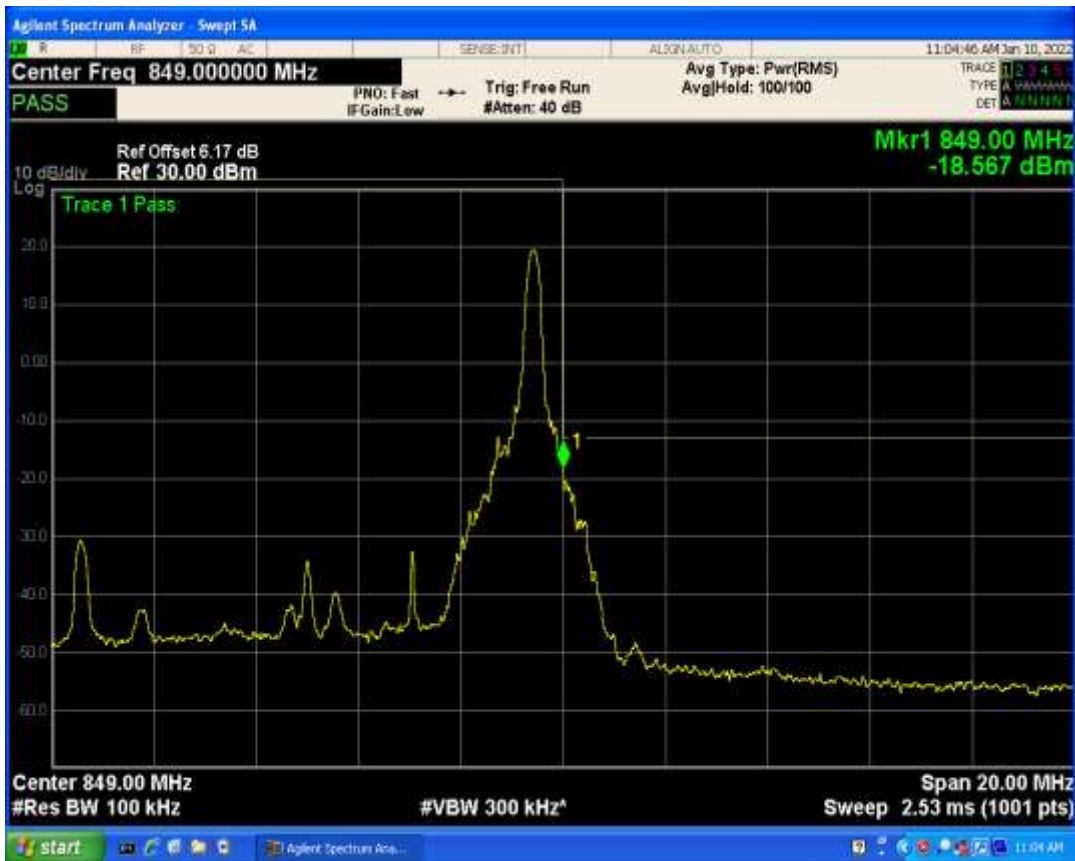
Band5 QPSK BW=10MHz Channel=20600 RB Size=1 Position=#0
