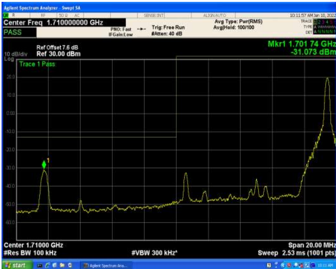
Band4 QPSK BW=10MHz Channel=20000 RB Size=1 Position=#0
