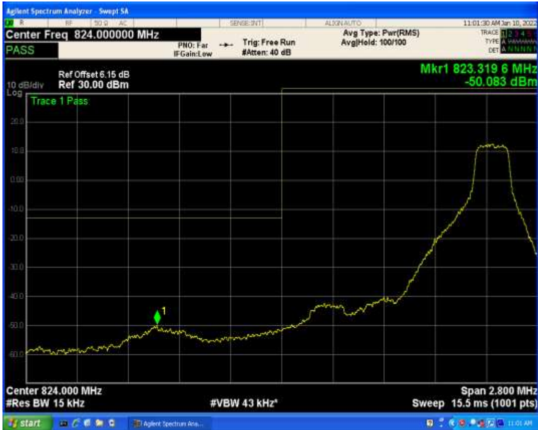
Band5 QPSK BW=1.4MHz Channel=20643 RB Size=1 Position=#0
