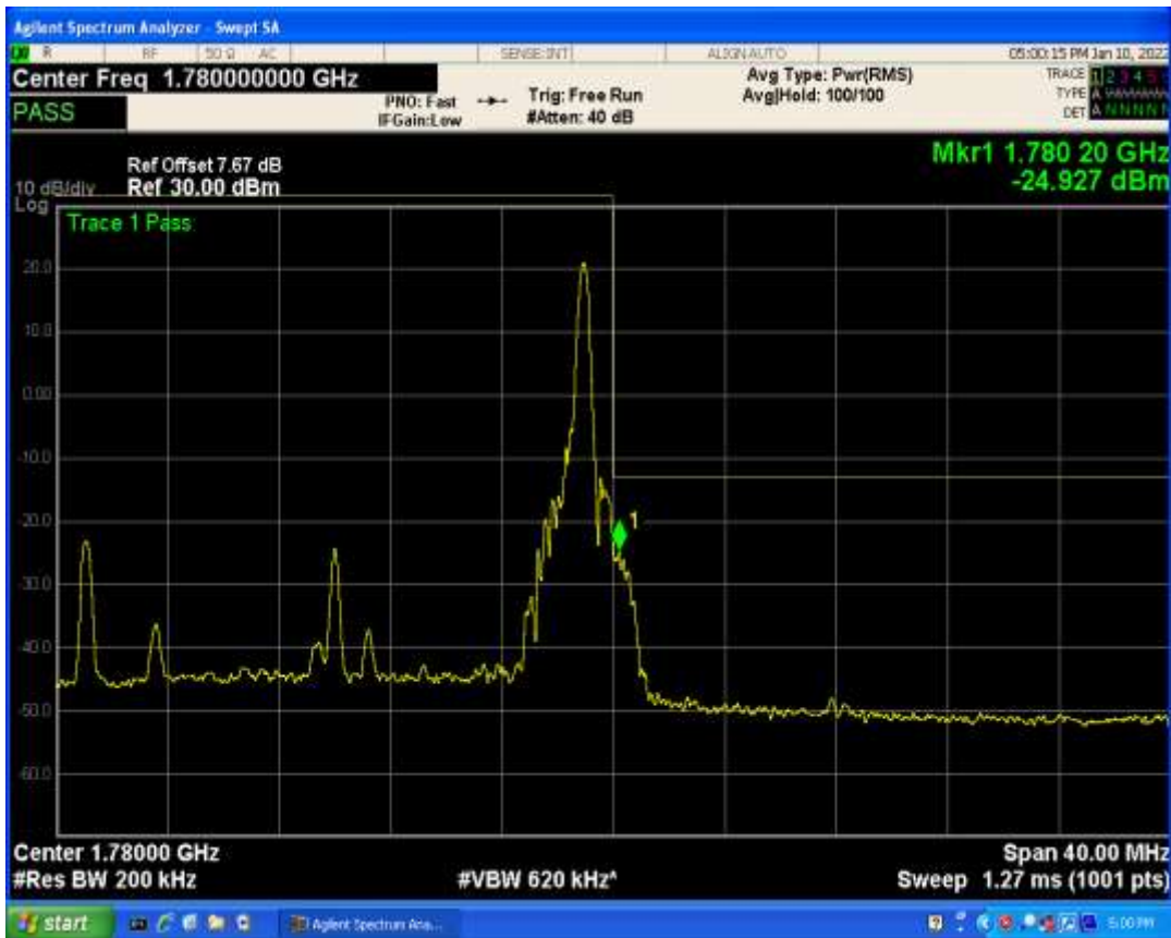
Band66 QAM16 BW=20MHz Channel=132572 RB Size=1 Position=#0
