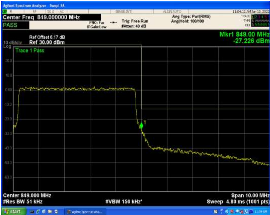
Band5 QAM16 BW=5MHz Channel=20625 RB Size=1 Position=#Max
