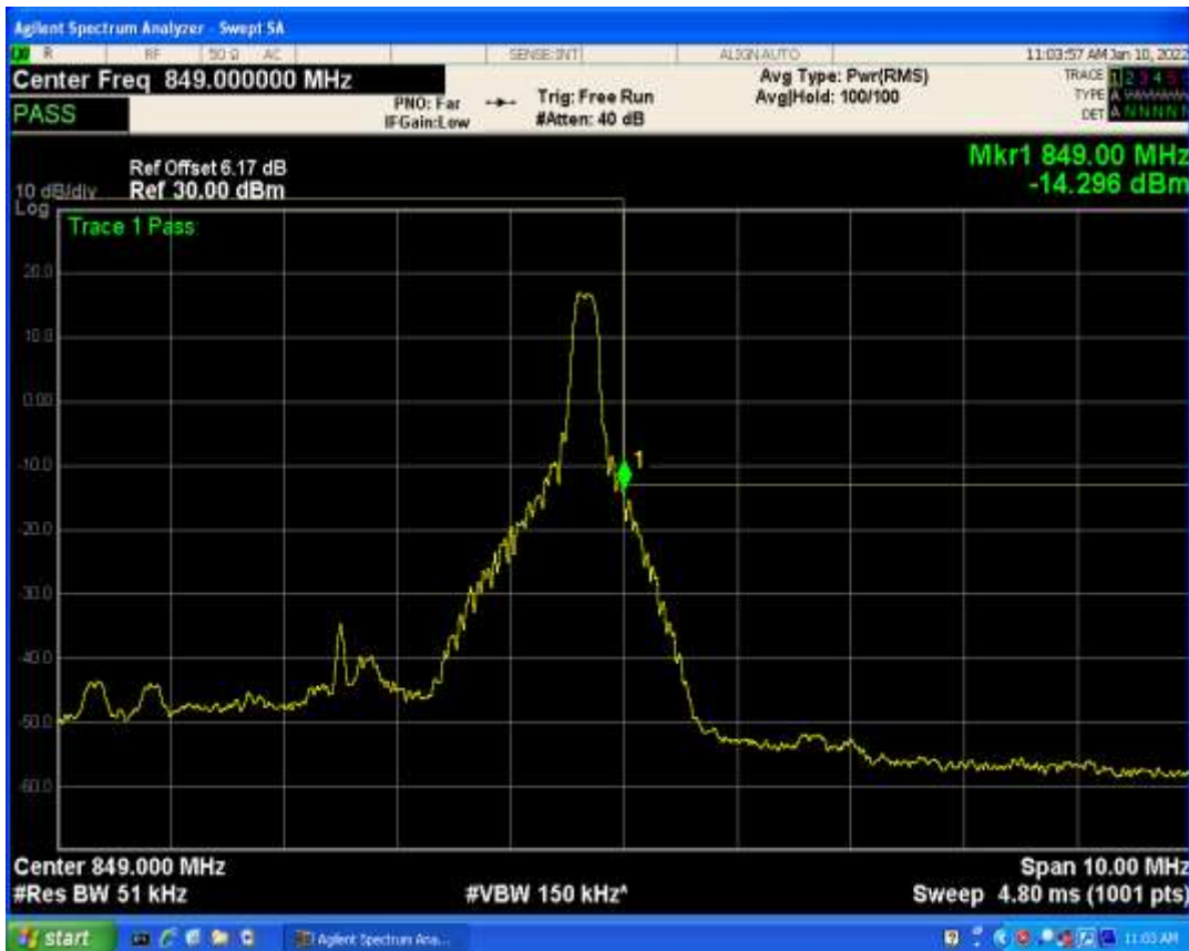
Band5 QPSK BW=3MHz Channel=20635 RB Size=15 Position=#0
