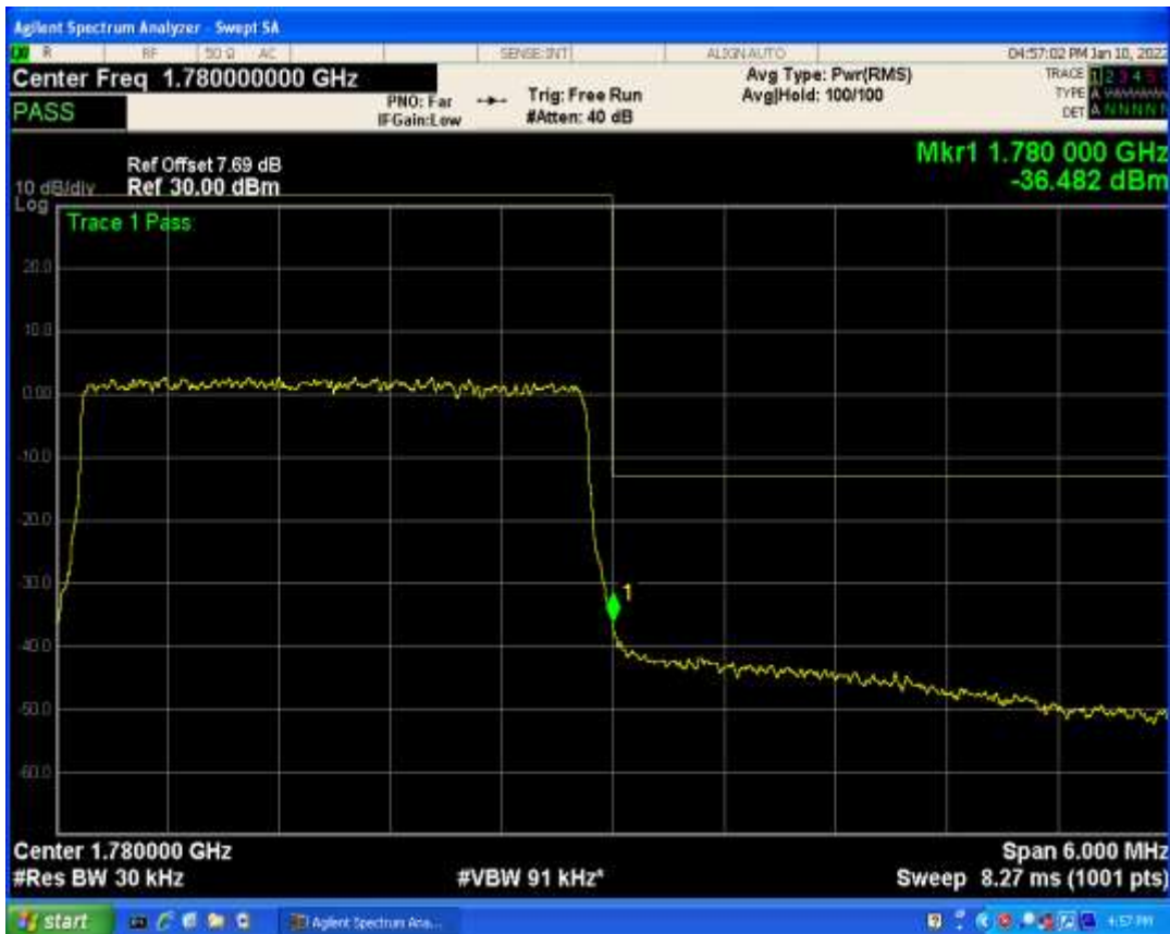
Band66 QAM16 BW=20MHz Channel=132572 RB Size=1 Position=#Max
