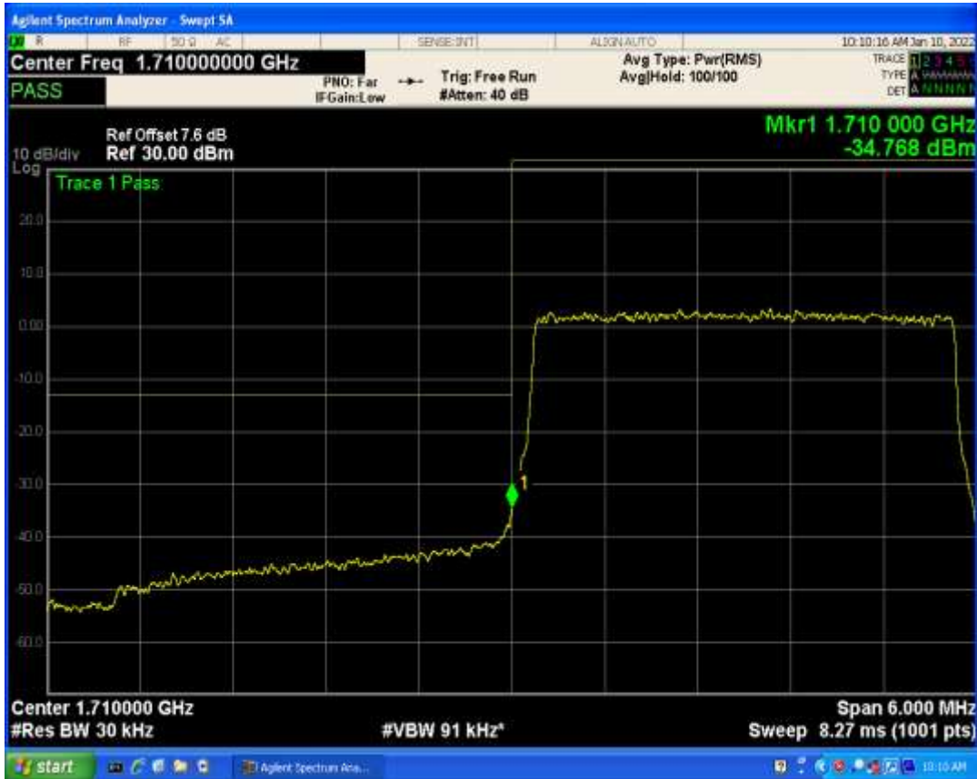
Band4 QPSK BW=3MHz Channel=19965 RB Size=1 Position=#Max
