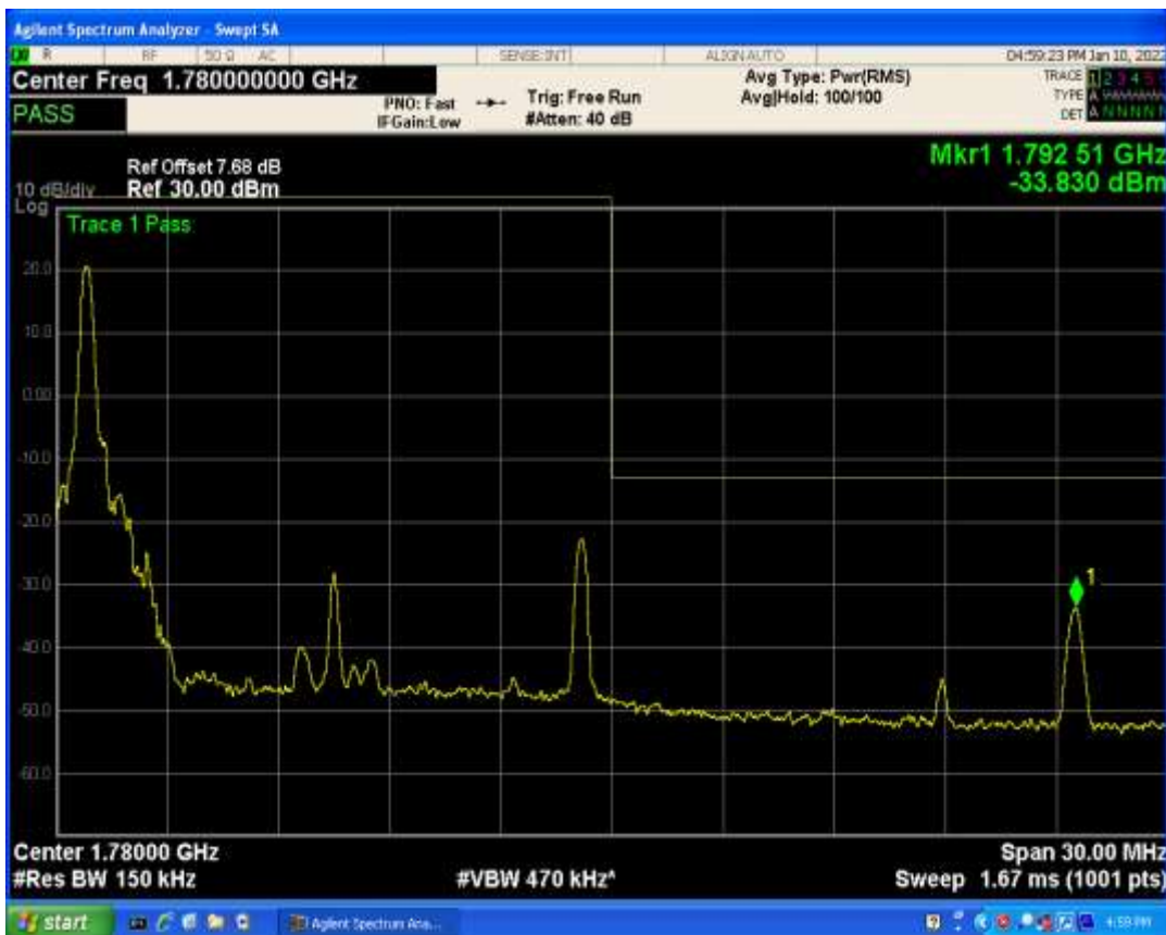
Band66 QAM16 BW=15MHz Channel=132047 RB Size=75 Position=#0
