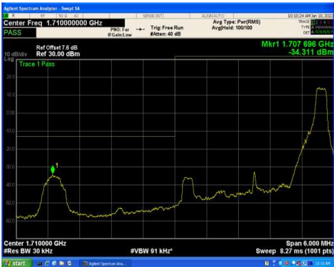
Band4 QAM16 BW=3MHz Channel=20385 RB Size=1 Position=#0
