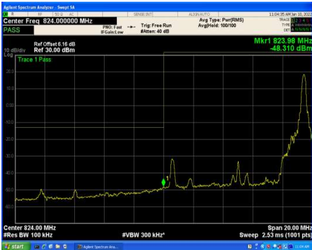
Band5 QAM16 BW=10MHz Channel=20450 RB Size=1 Position=#0
