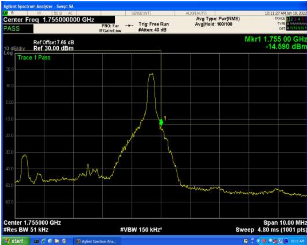
Band4 QPSK BW=5MHz Channel=19975 RB Size=1 Position=#Max
