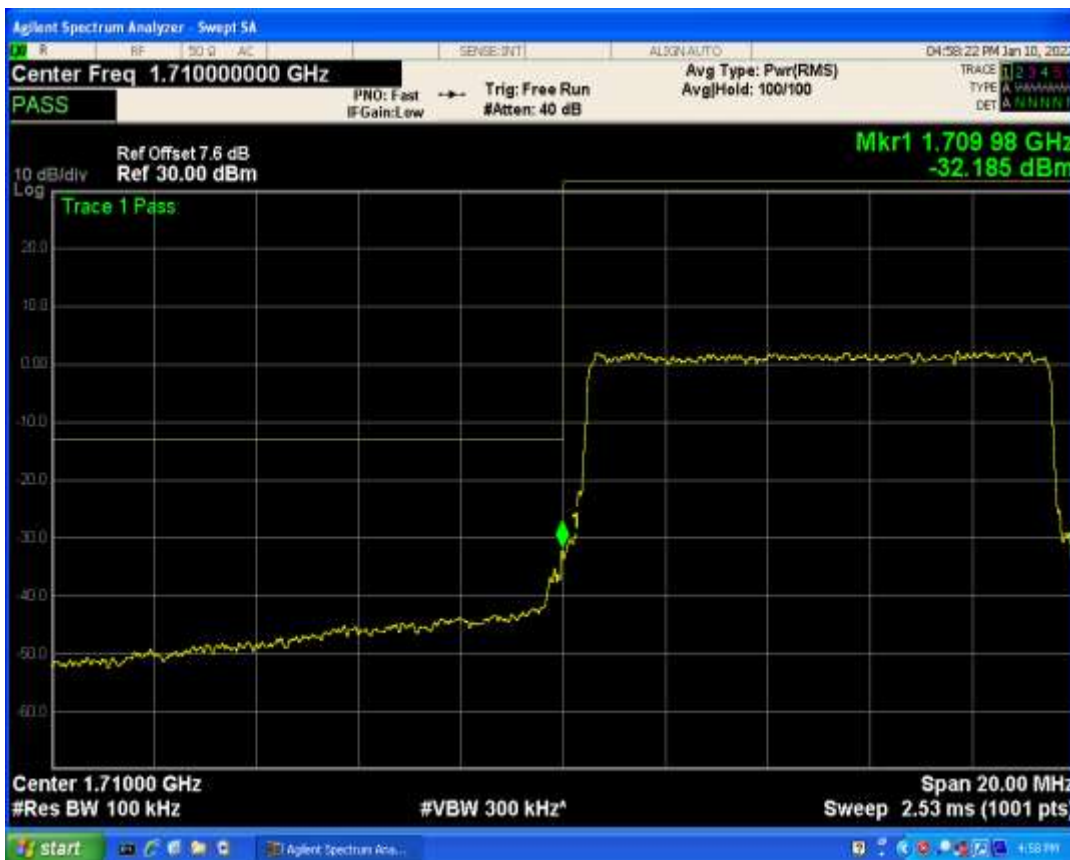
Band66 QAM16 BW=10MHz Channel=132622 RB Size=1 Position=#Max
