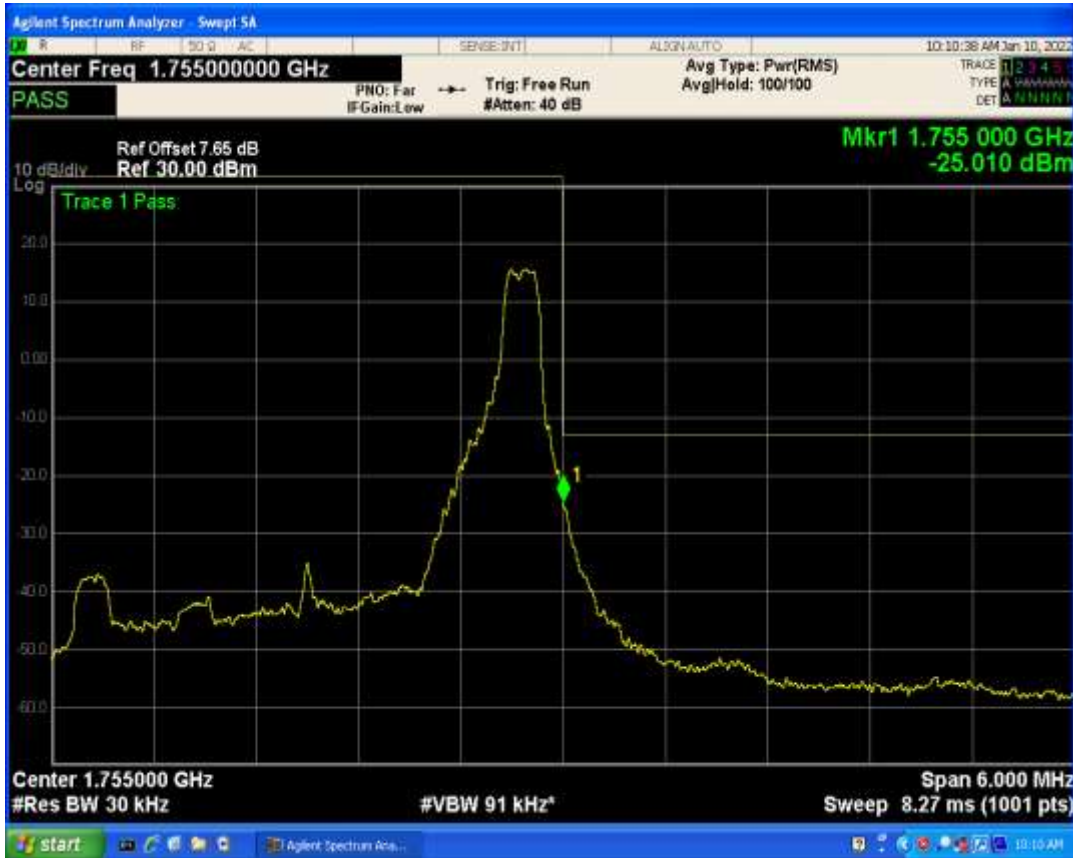
Band4 QPSK BW=3MHz Channel=20385 RB Size=1 Position=#0
