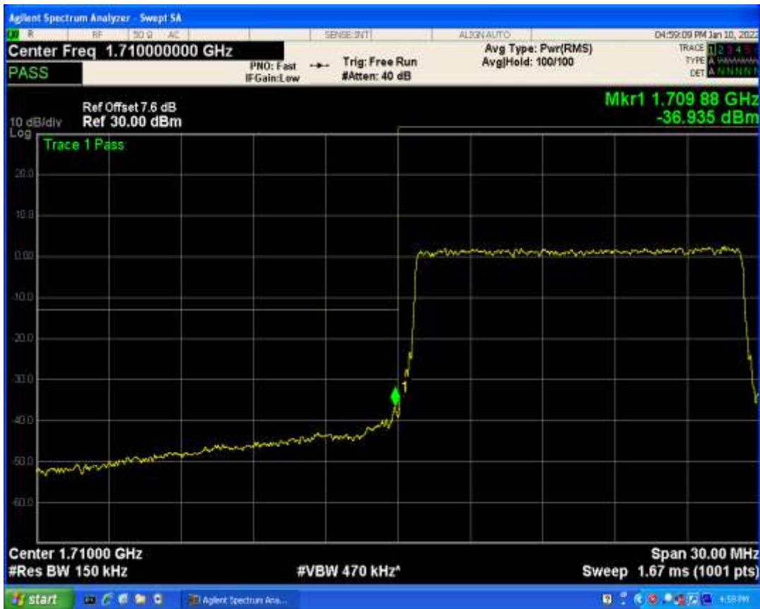
Band66 QAM16 BW=3MHz Channel=132657 RB Size=1 Position=#0
