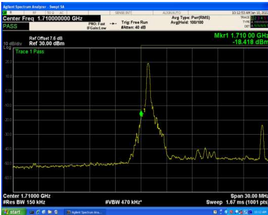
Band4 QAM16 BW=10MHz Channel=20350 RB Size=1 Position=#Max
