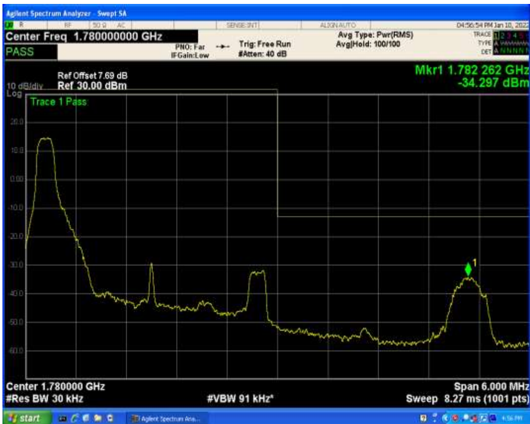
Band66 QAM16 BW=3MHz Channel=131987 RB Size=15 Position=#0
