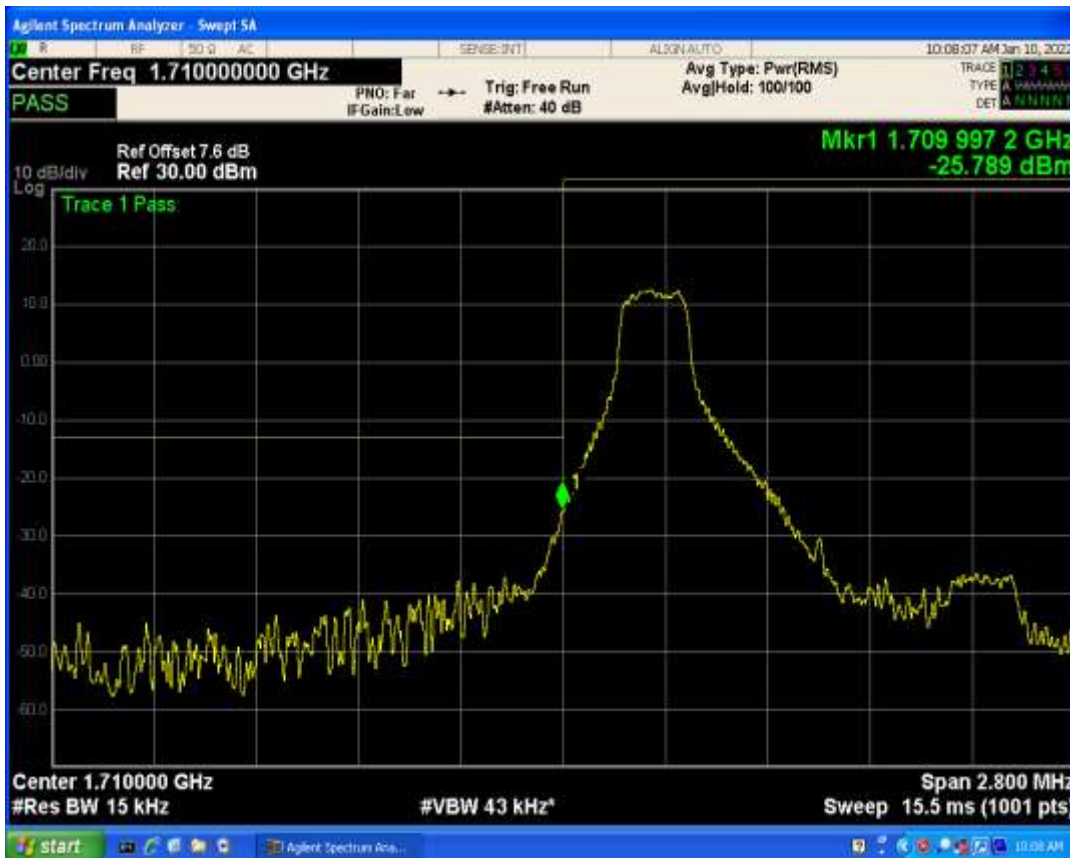
Band4 QPSK BW=1.4MHz Channel=19957 RB Size=6 Position=#0
