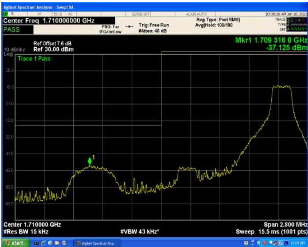
Band4 QAM16 BW=1.4MHz Channel=19957 RB Size=1 Position=#0
