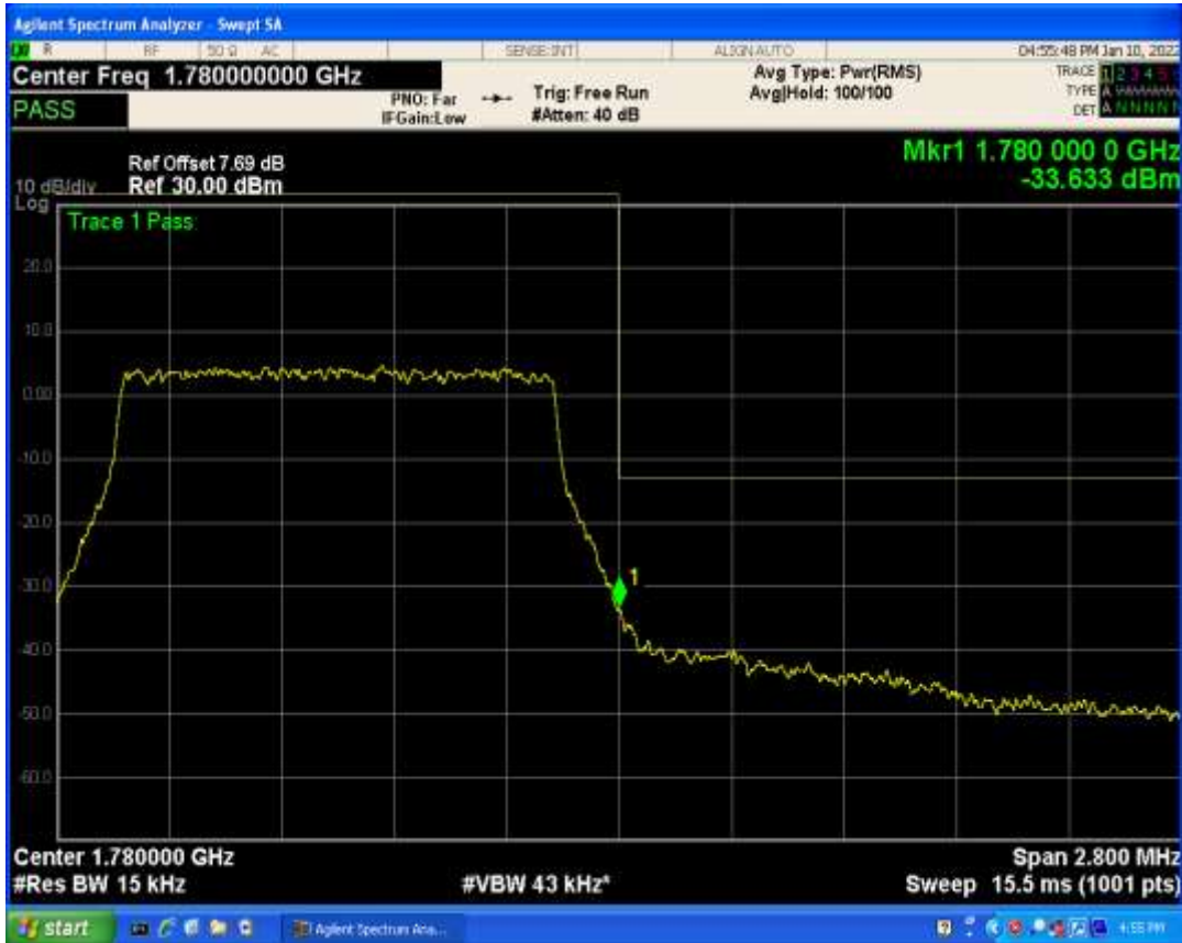
Band66 QPSK BW=1.4MHz Channel=132665 RB Size=1 Position=#Max
