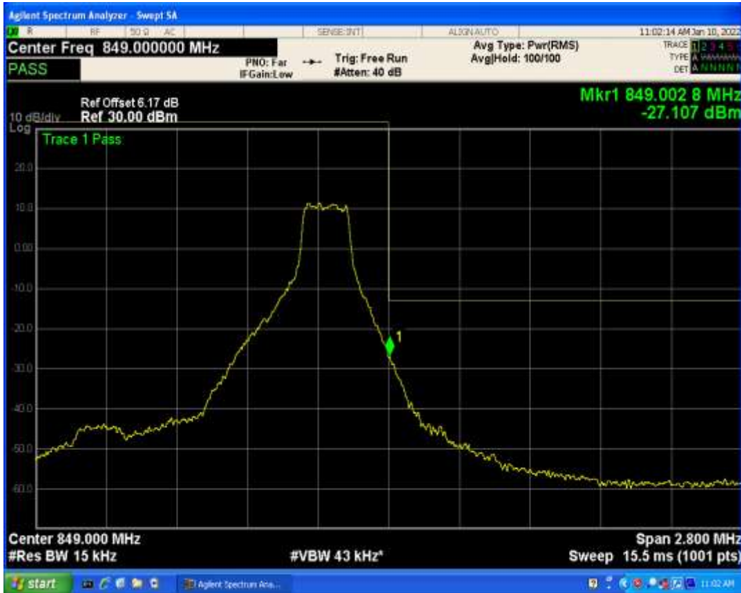
Band5 QAM16 BW=1.4MHz Channel=20643 RB Size=1 Position=#0
