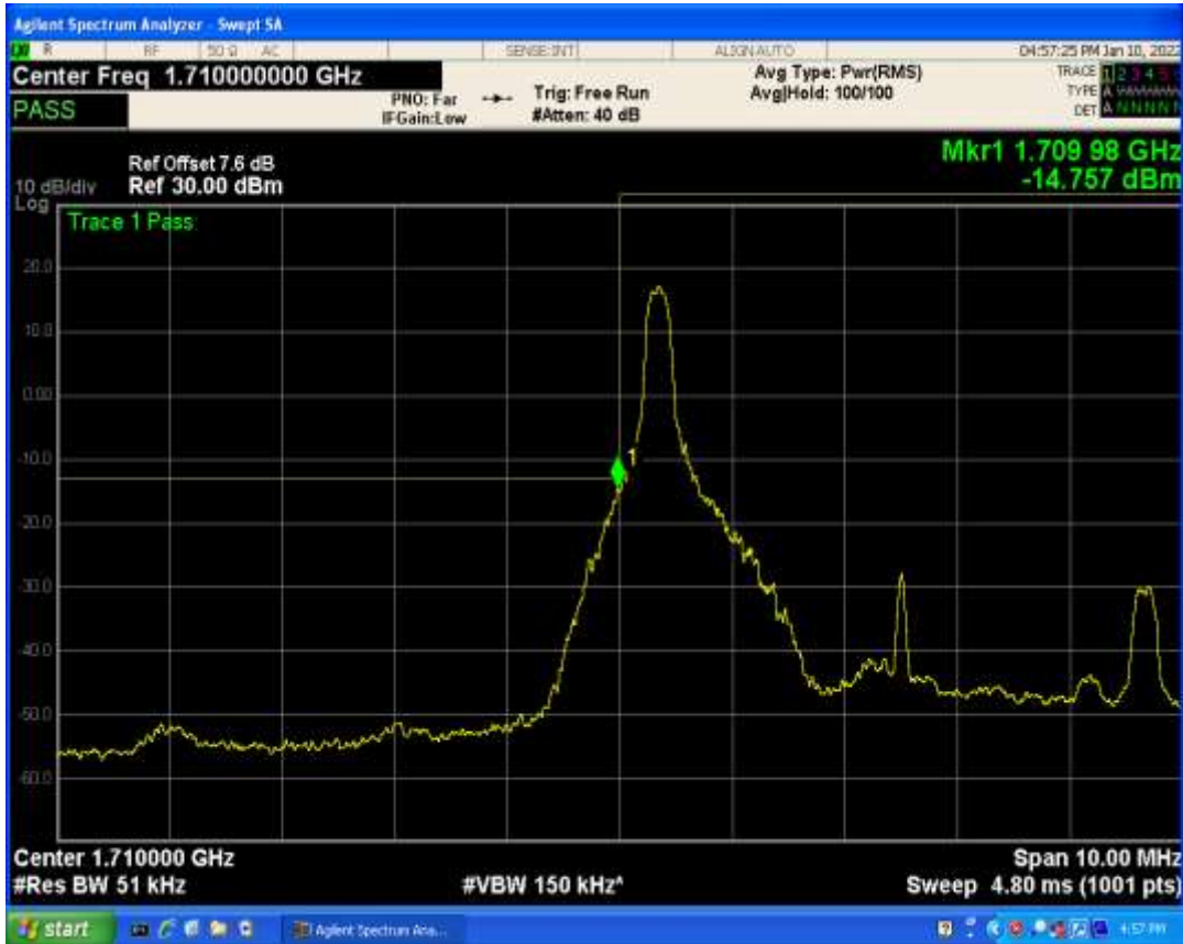
Band66 QAM16 BW=3MHz Channel=132657 RB Size=15 Position=#0
