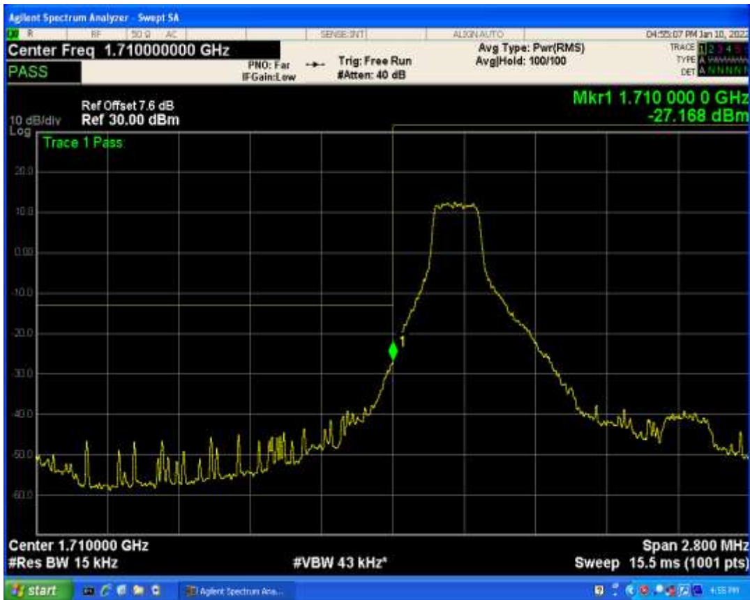
Band66 QAM16 BW=5MHz Channel=131997 RB Size=25 Position=#0
