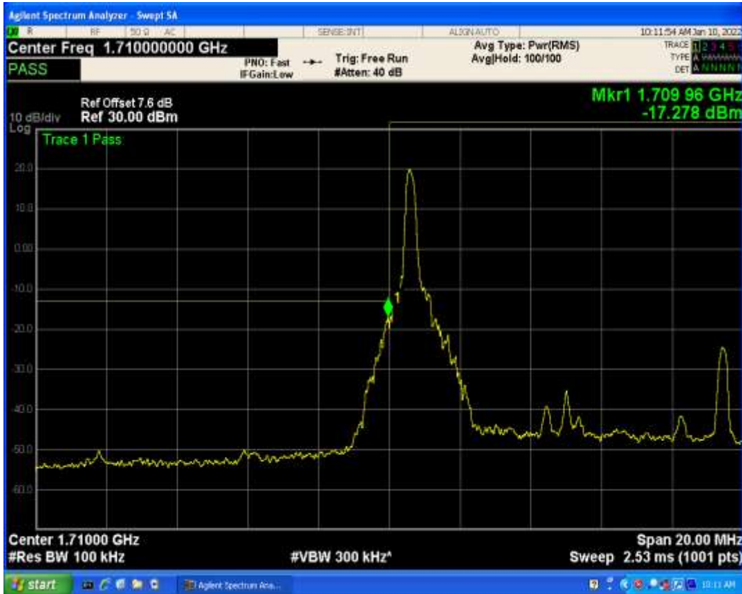
Band4 QAM16 BW=5MHz Channel=20375 RB Size=25 Position=#0
