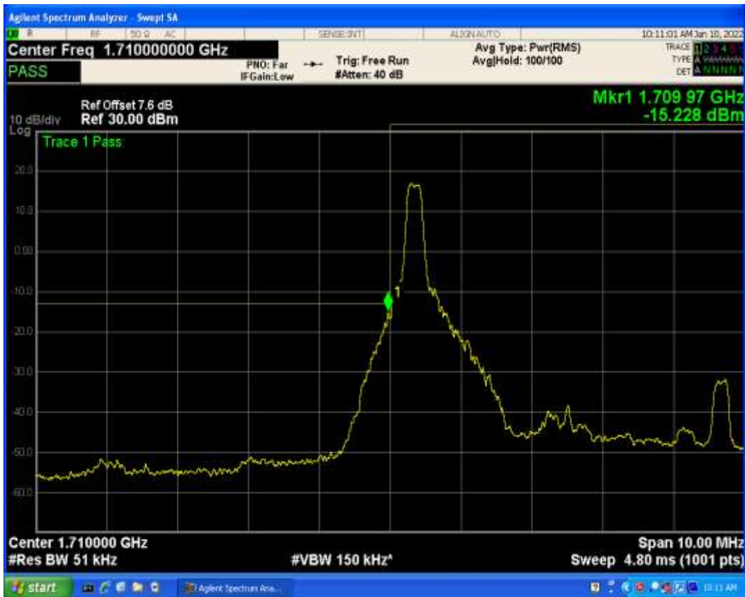
Band4 QPSK BW=3MHz Channel=20385 RB Size=15 Position=#0
