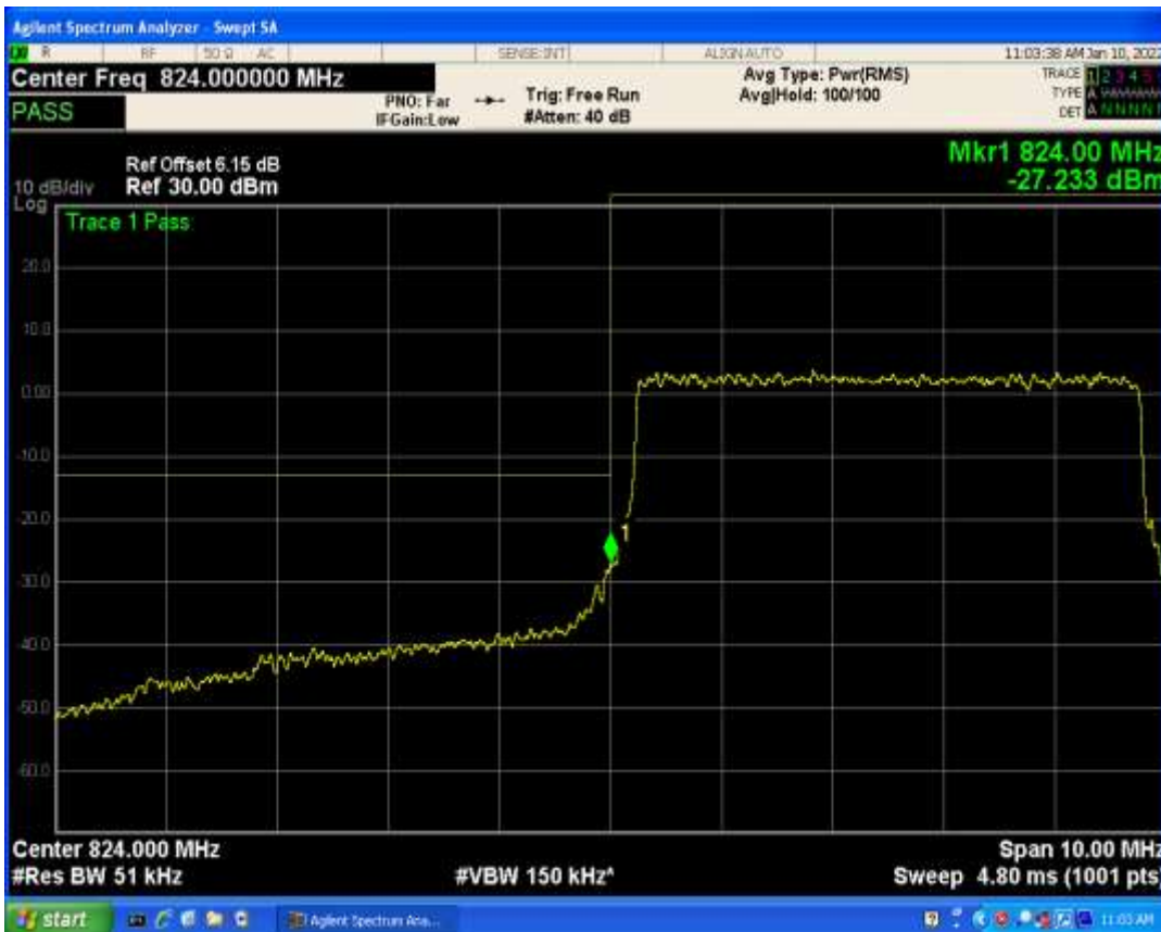
Band5 QPSK BW=5MHz Channel=20625 RB Size=25 Position=#0
