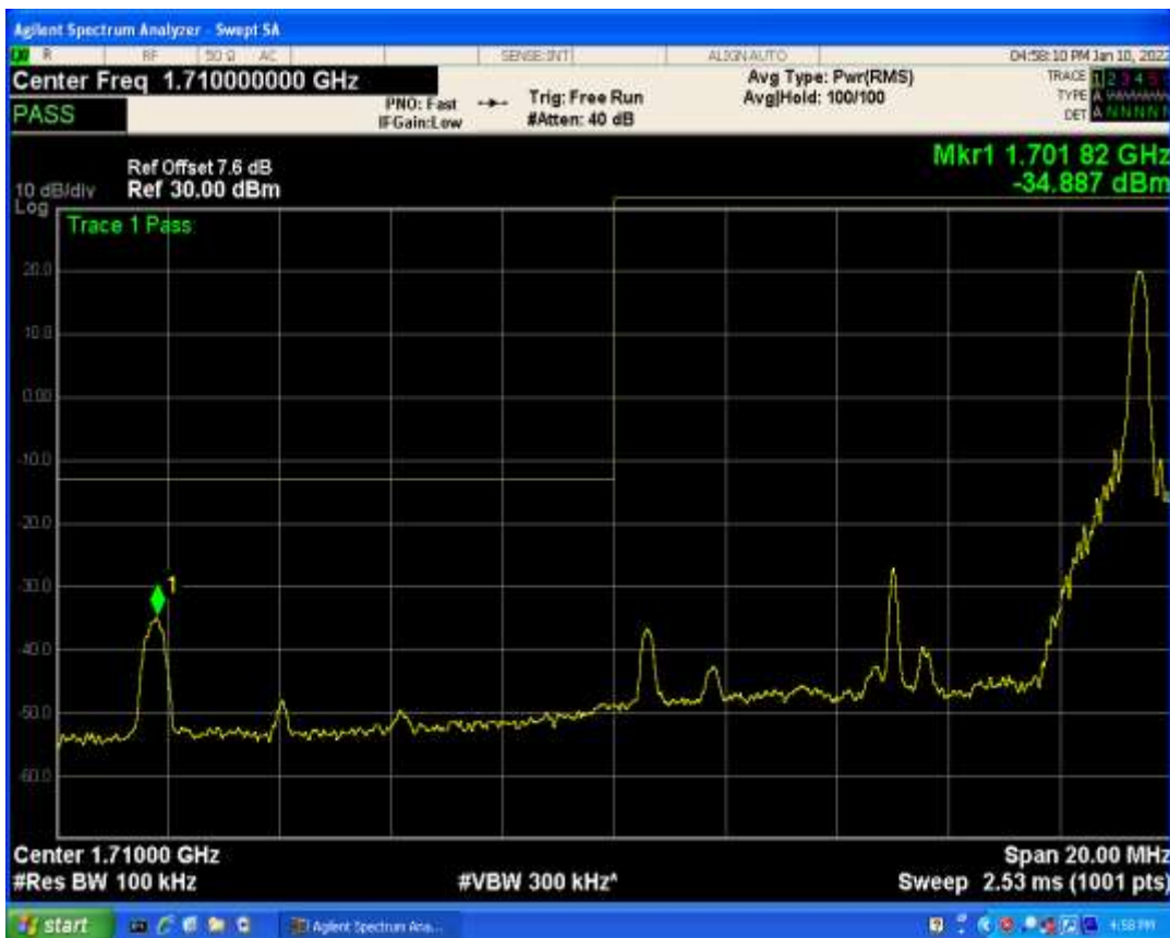
Band66 QPSK BW=10MHz Channel=132022 RB Size=1 Position=#0
