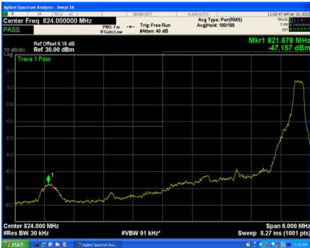
Band5 QAM16 BW=3MHz Channel=20415 RB Size=1 Position=#0
