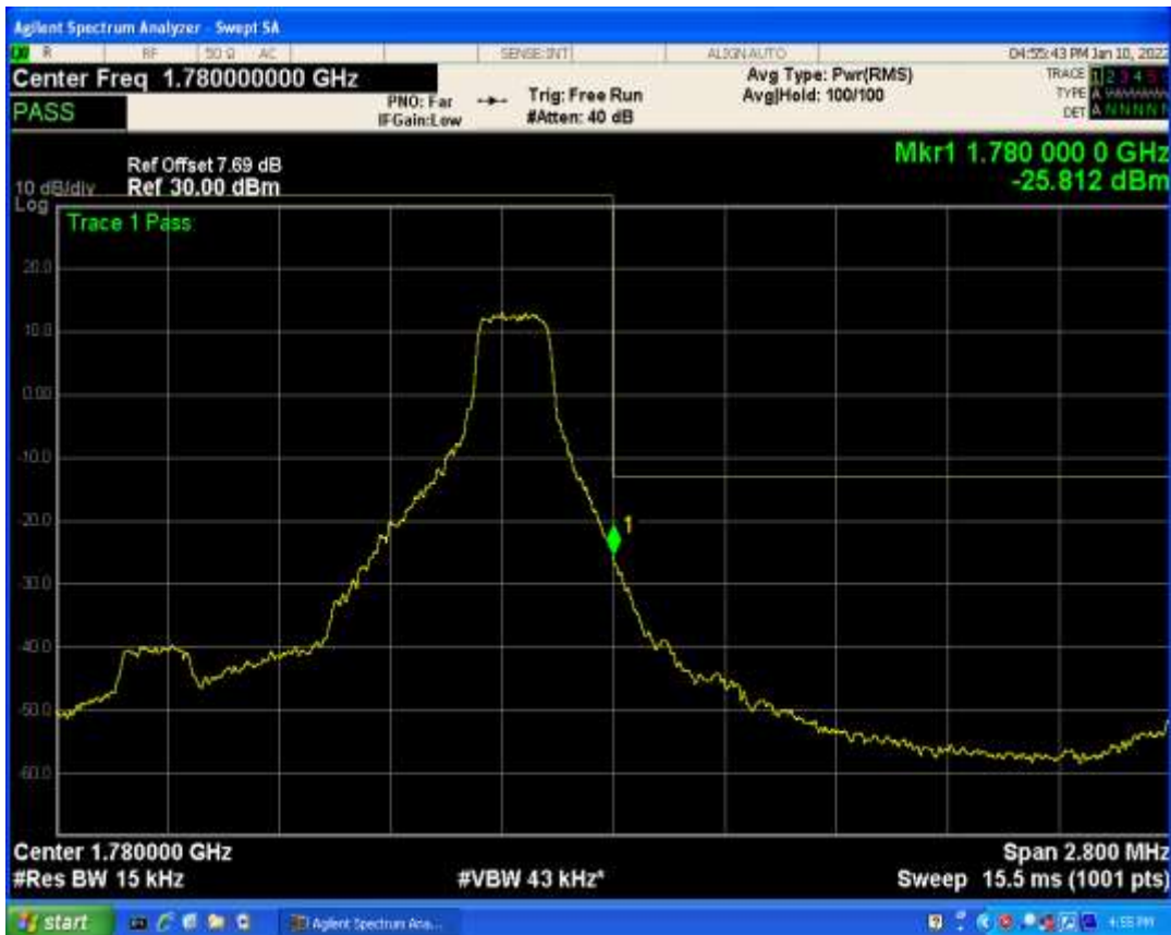
Band66 QPSK BW=1.4MHz Channel=131979 RB Size=1 Position=#0
