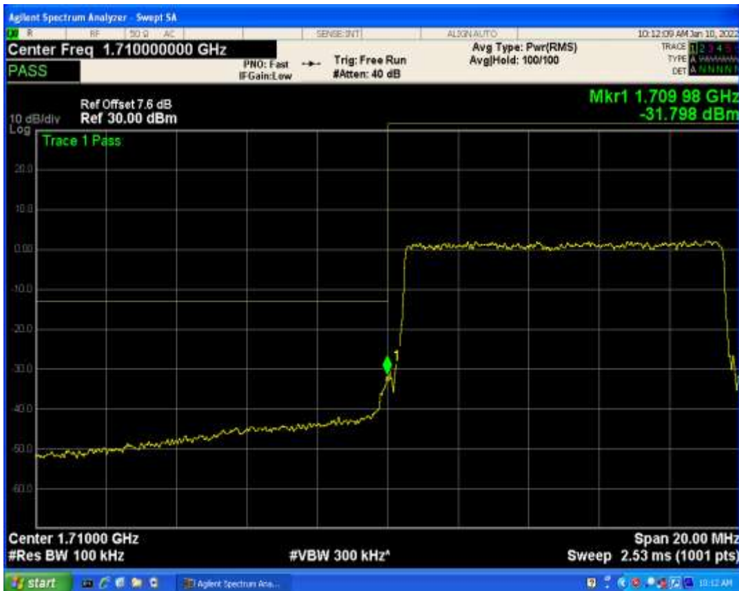
Band4 QAM16 BW=10MHz Channel=20350 RB Size=1 Position=#0
