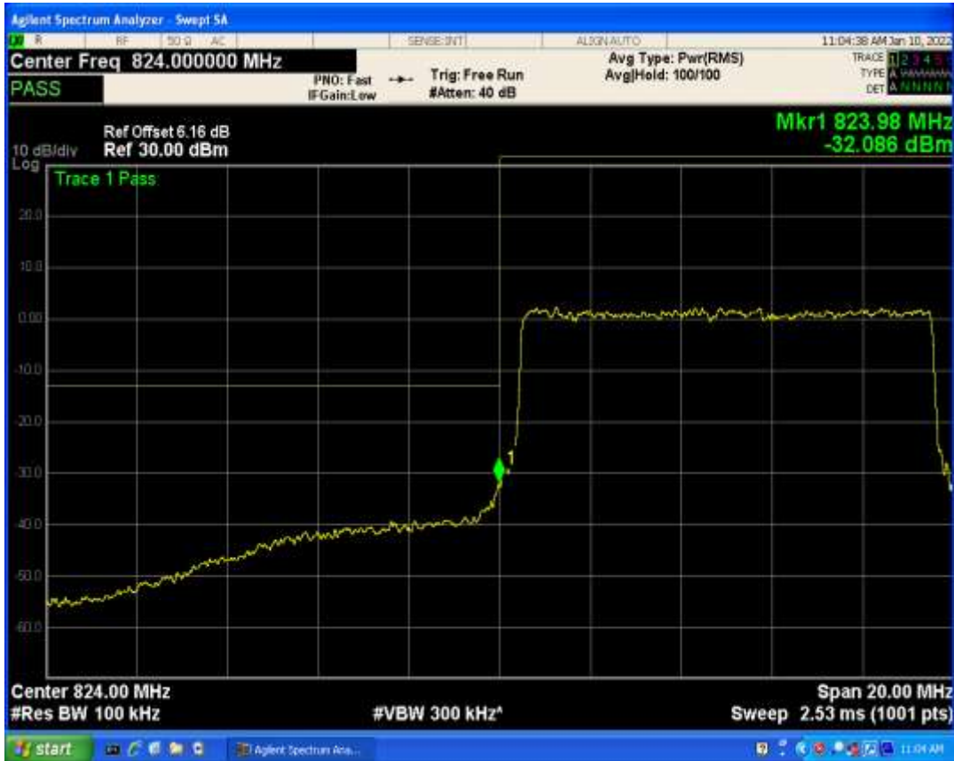
Band5 QAM16 BW=1.4MHz Channel=20643 RB Size=6 Position=#0
