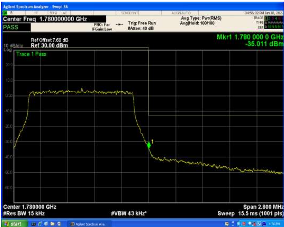
Band66 QAM16 BW=1.4MHz Channel=132665 RB Size=1 Position=#Max
