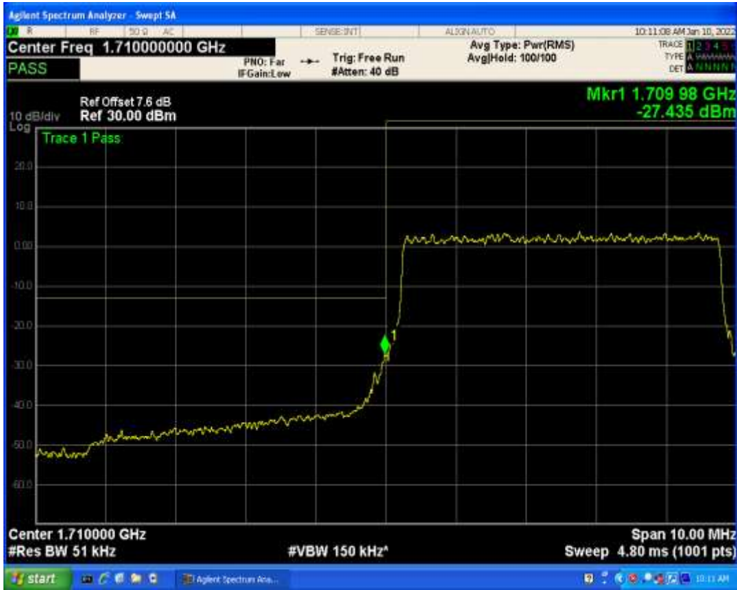
Band4 QPSK BW=5MHz Channel=20375 RB Size=25 Position=#0
