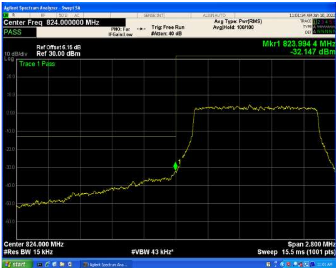
Band5 QPSK BW=1.4MHz Channel=20407 RB Size=1 Position=#Max
