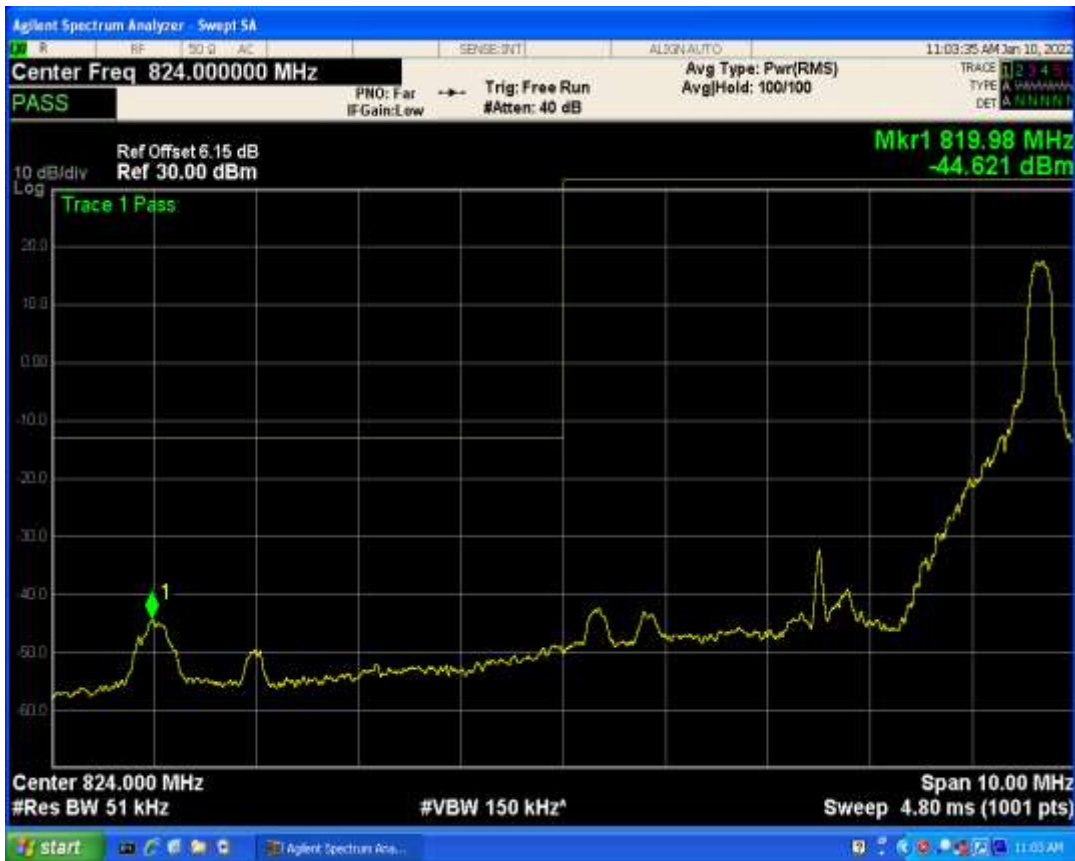
Band5 QPSK BW=5MHz Channel=20425 RB Size=1 Position=#0
