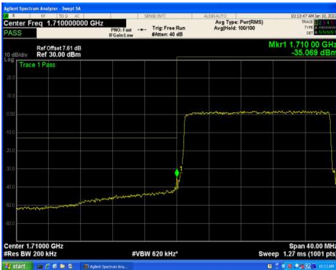
Band4 QAM16 BW=20MHz Channel=20300 RB Size=1 Position=#Max
