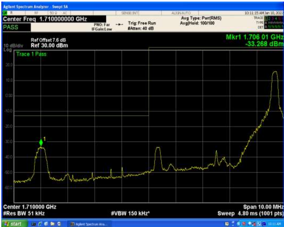
Band4 QAM16 BW=5MHz Channel=20375 RB Size=1 Position=#0
