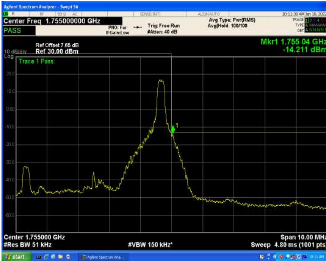
Band4 QPSK BW=1.4MHz Channel=19957 RB Size=1 Position=#0
