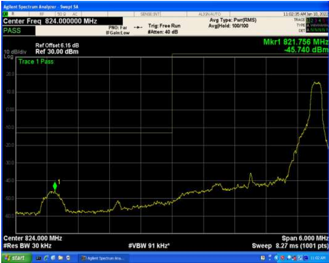
Band5 QPSK BW=3MHz Channel=20635 RB Size=1 Position=#0
