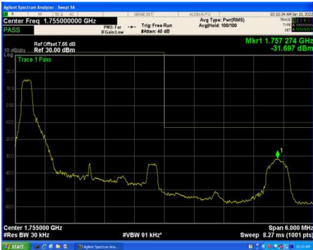
Band4 QPSK BW=5MHz Channel=19975 RB Size=1 Position=#0
