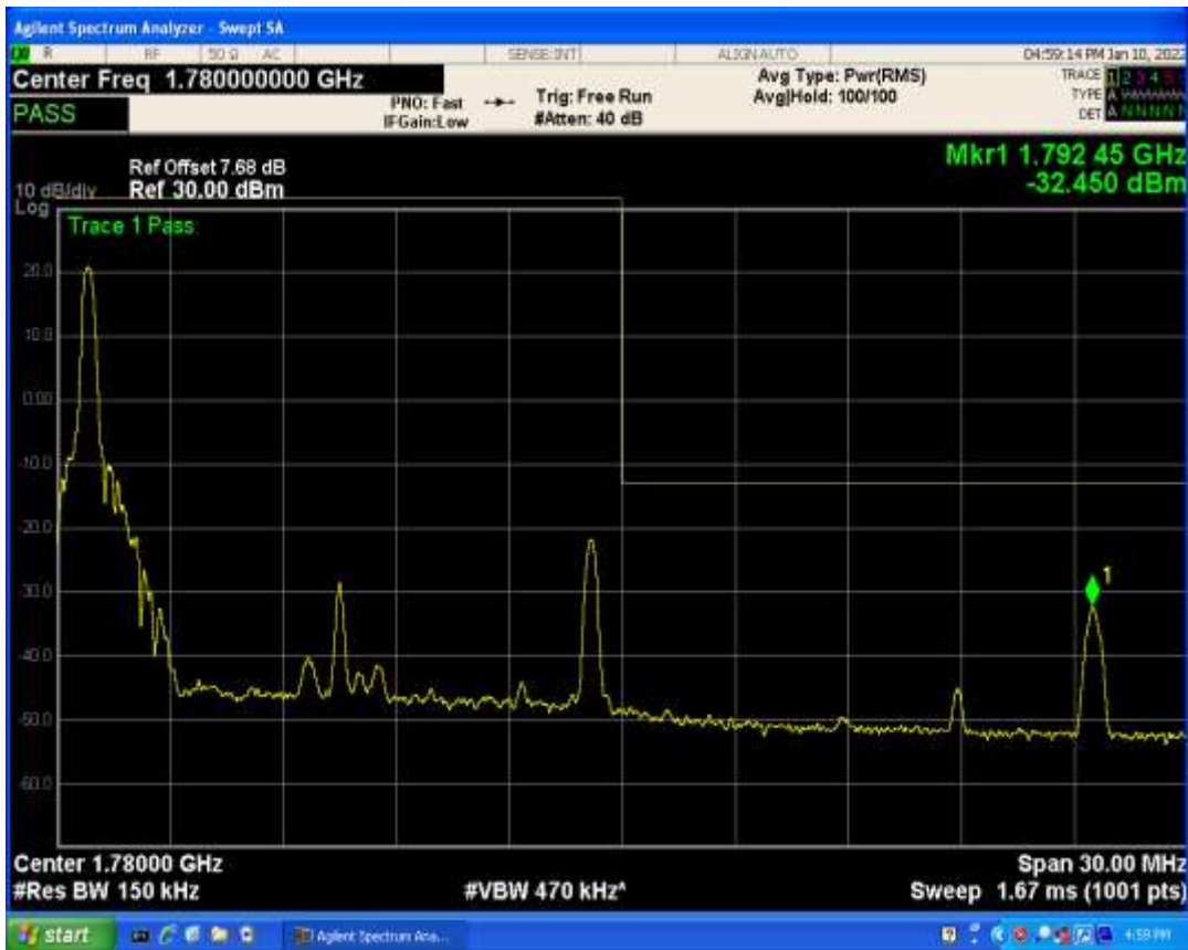
Band66 QPSK BW=15MHz Channel=132047 RB Size=75 Position=#0
