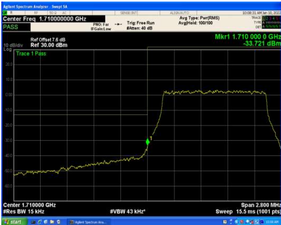
Band4 QAM16 BW=10MHz Channel=20350 RB Size=50 Position=#0
