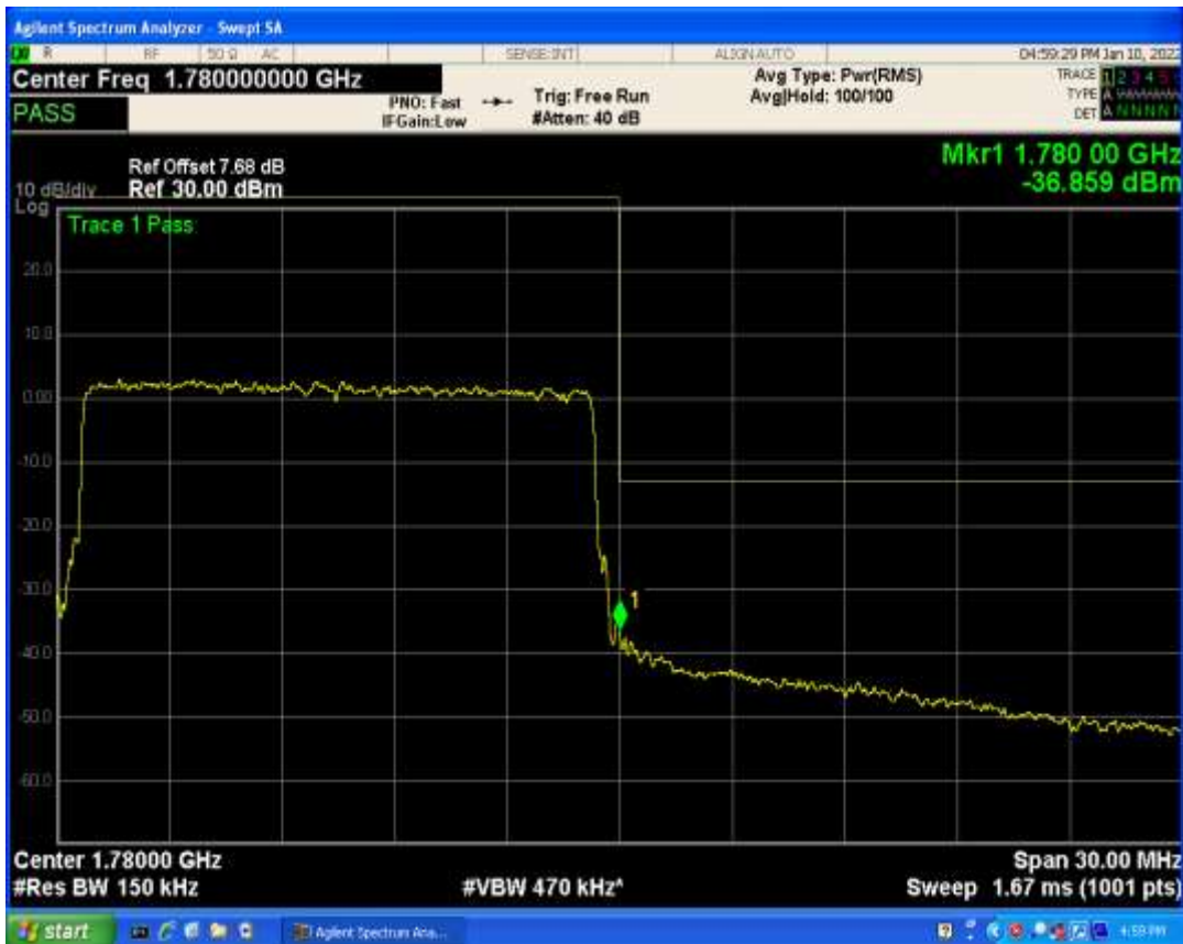
Band66 QAM16 BW=15MHz Channel=132597 RB Size=1 Position=#Max
