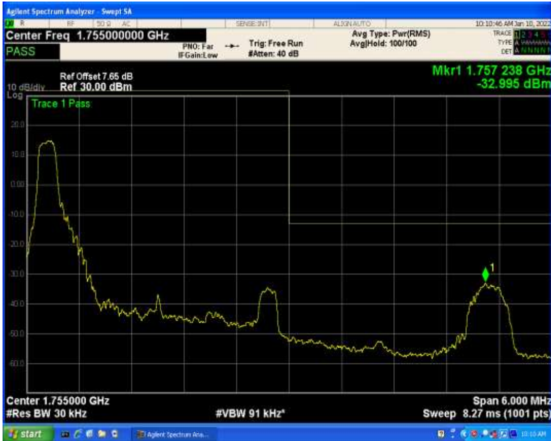
Band4 QAM16 BW=3MHz Channel=19965 RB Size=15 Position=#0
