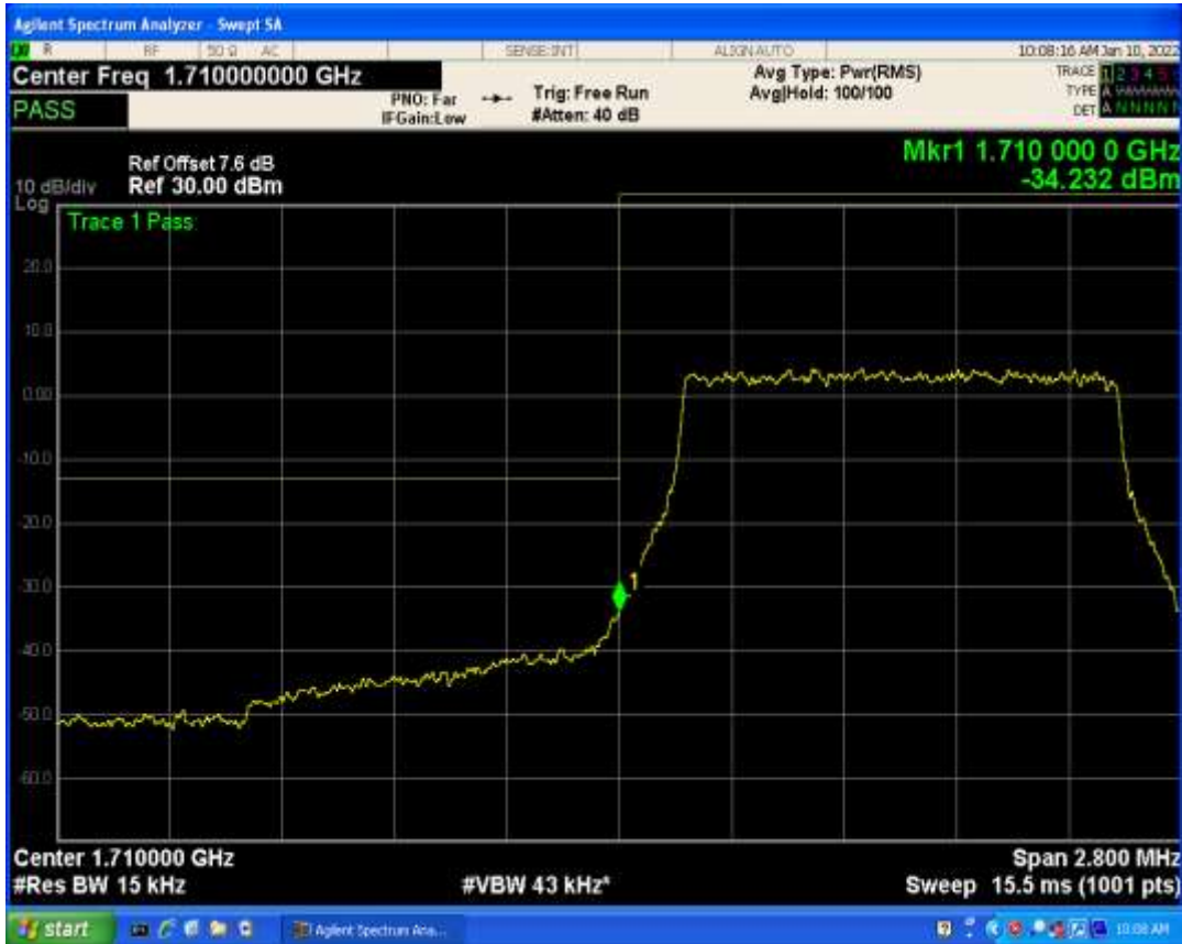
Band4 QPSK BW=1.4MHz Channel=19957 RB Size=1 Position=#Max
