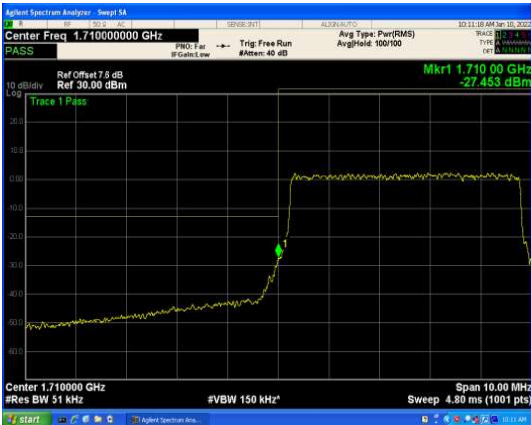
Band4 QAM16 BW=3MHz Channel=20385 RB Size=1 Position=#Max
