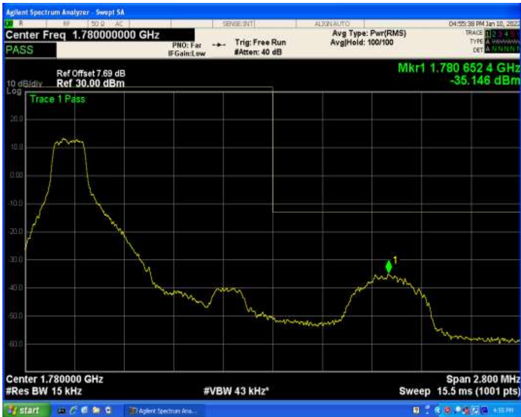
Band66 QPSK BW=1.4MHz Channel=132665 RB Size=6 Position=#0
