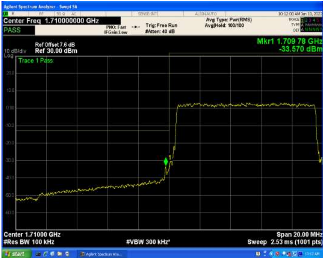
Band4 QPSK BW=10MHz Channel=20350 RB Size=50 Position=#0
