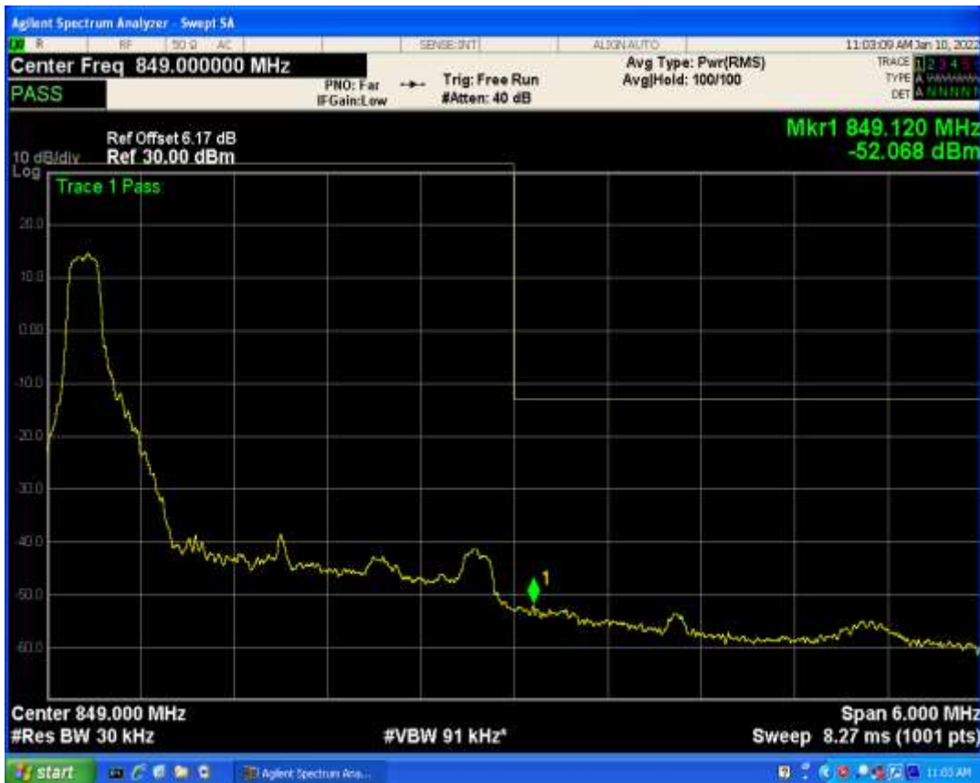
Band5 QAM16 BW=5MHz Channel=20425 RB Size=1 Position=#0
