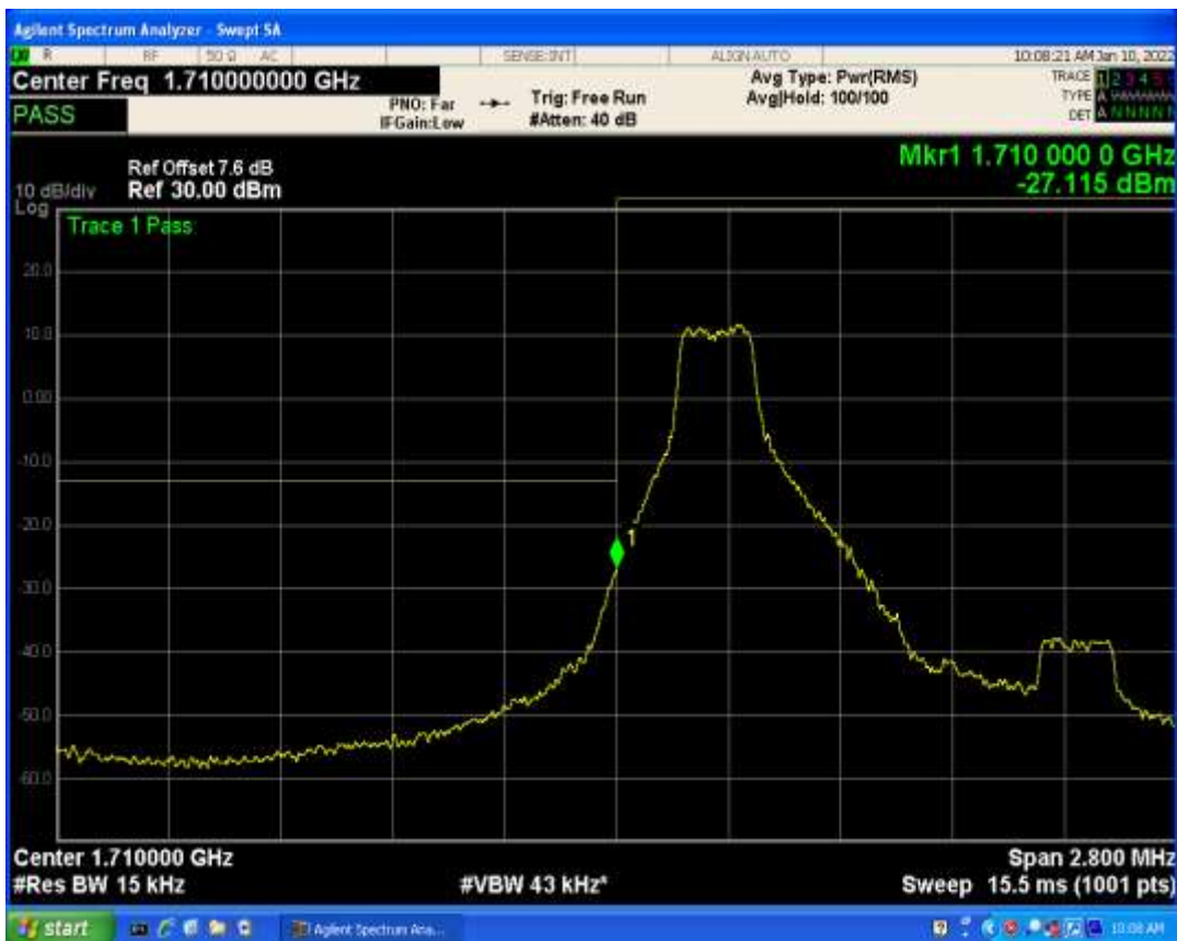
Band4 QAM16 BW=1.4MHz Channel=20393 RB Size=1 Position=#0
