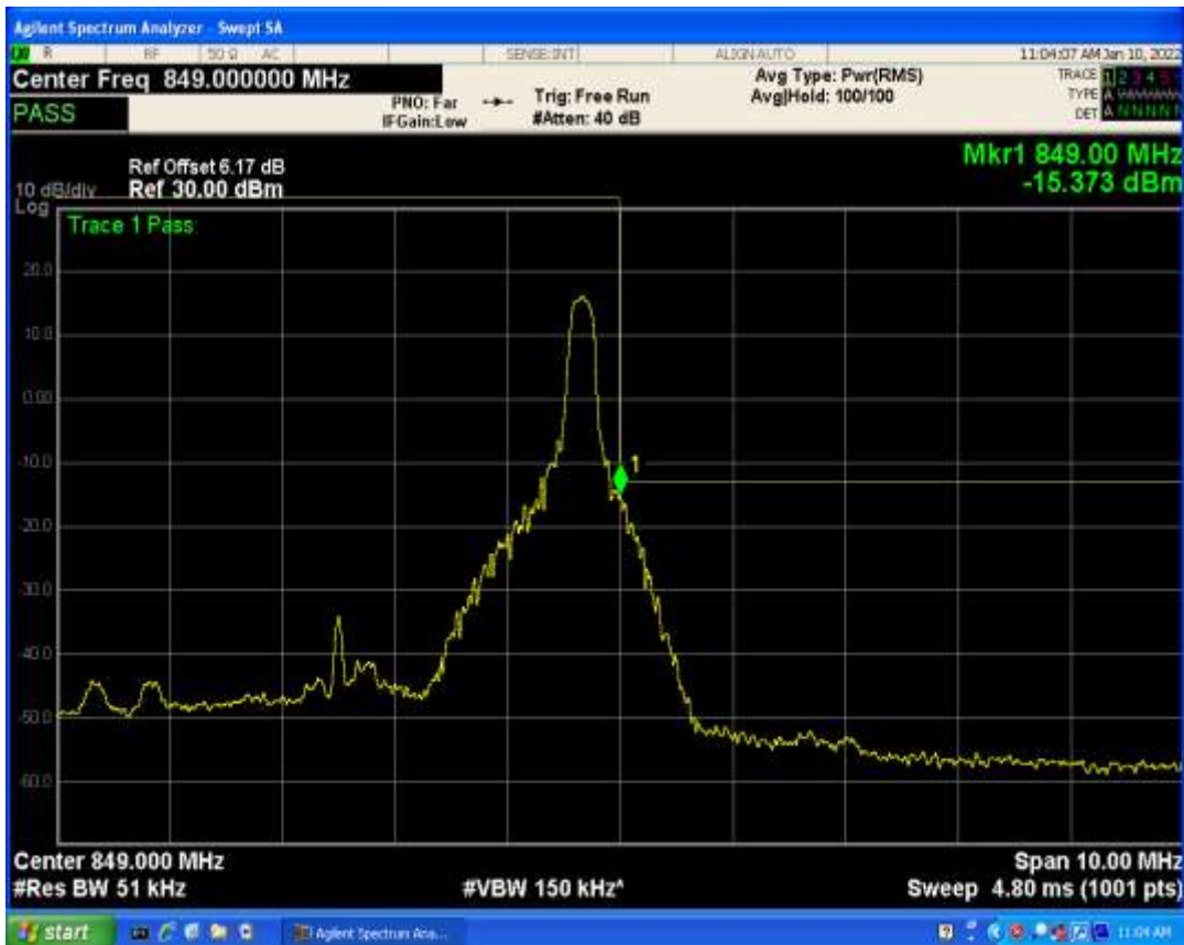
Band5 QPSK BW=3MHz Channel=20415 RB Size=1 Position=#0
