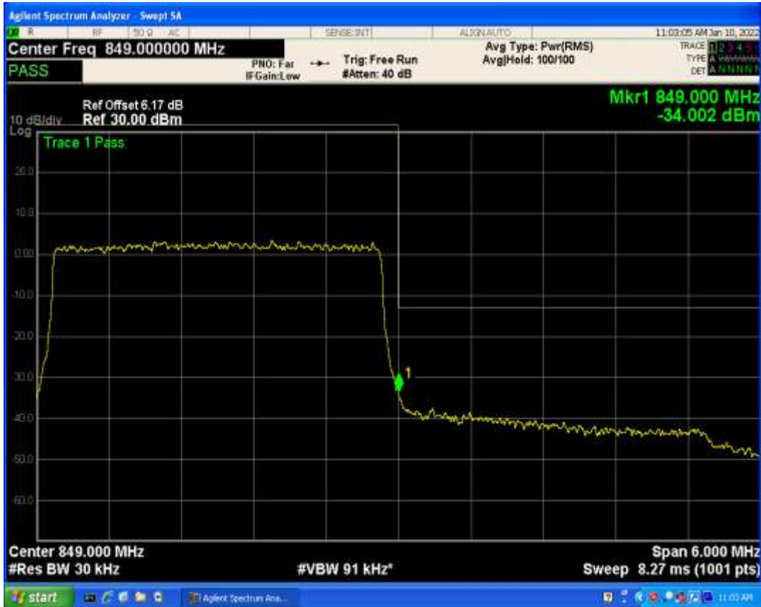
Band5 QPSK BW=3MHz Channel=20635 RB Size=1 Position=#Max
