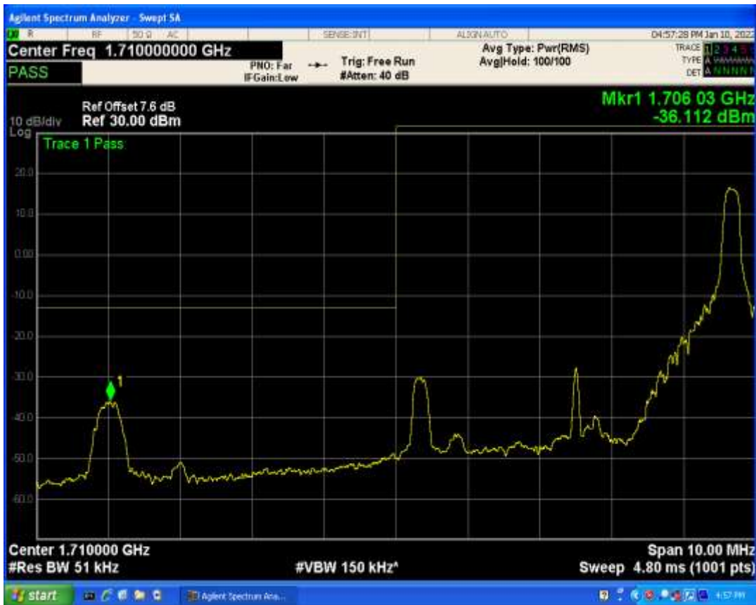
Band66 QAM16 BW=5MHz Channel=132647 RB Size=1 Position=#0
