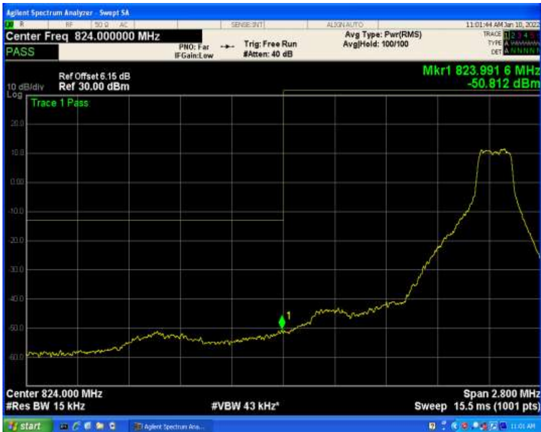
Band5 QAM16 BW=1.4MHz Channel=20643 RB Size=1 Position=#Max
