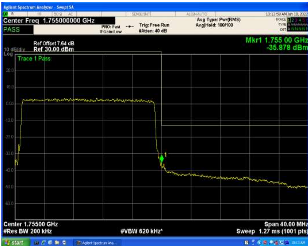
Band4 QPSK BW=20MHz Channel=20300 RB Size=1 Position=#Max
