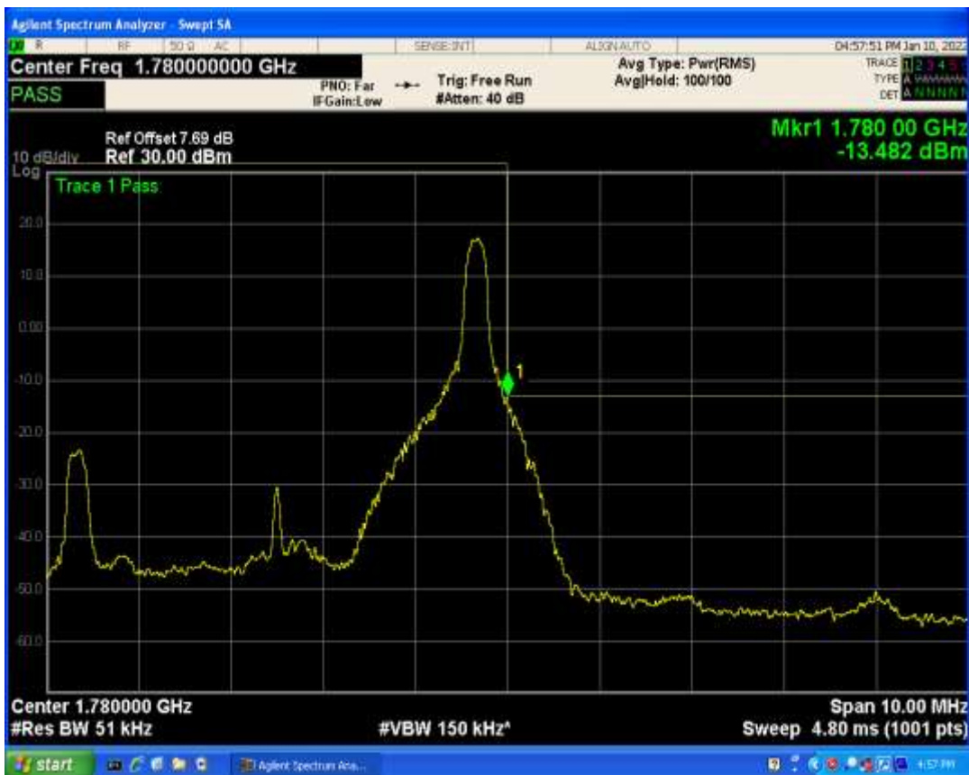
Band66 QPSK BW=15MHz Channel=132047 RB Size=1 Position=#0
