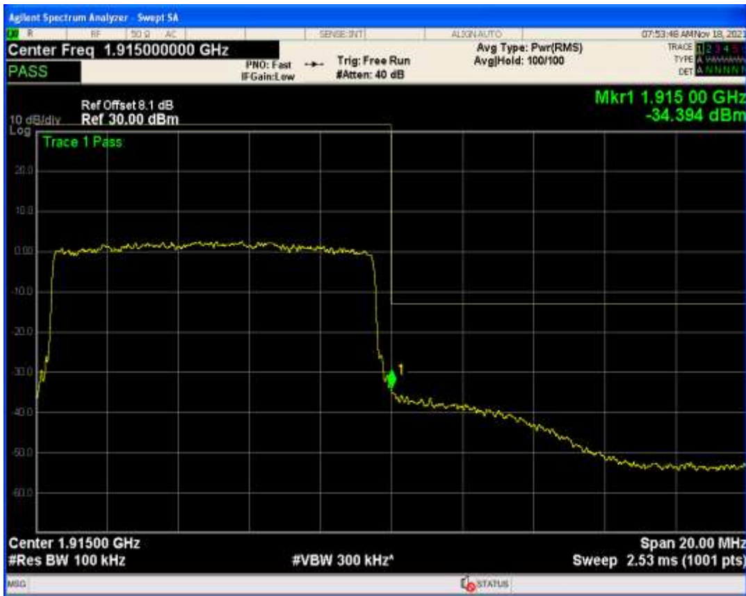
Band25 QAM16 BW=10MHz Channel=26640 RB Size=1 Position=#Max
