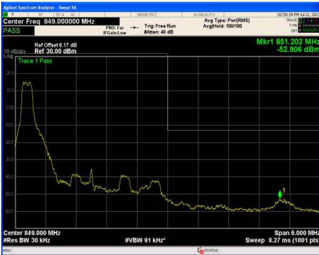
Band26b QAM16 BW=5MHz Channel=26815 RB Size=1 Position=#0
