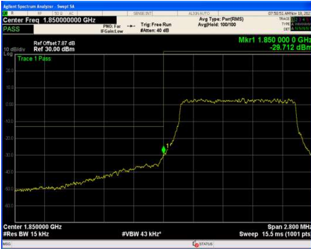
Band25 QAM16 BW=1.4MHz Channel=26047 RB Size=1 Position=#0
