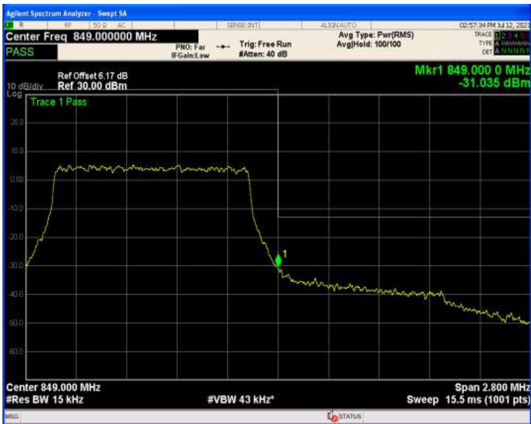
Band26b QPSK BW=1.4MHz Channel=26797 RB Size=6 Position=#0
