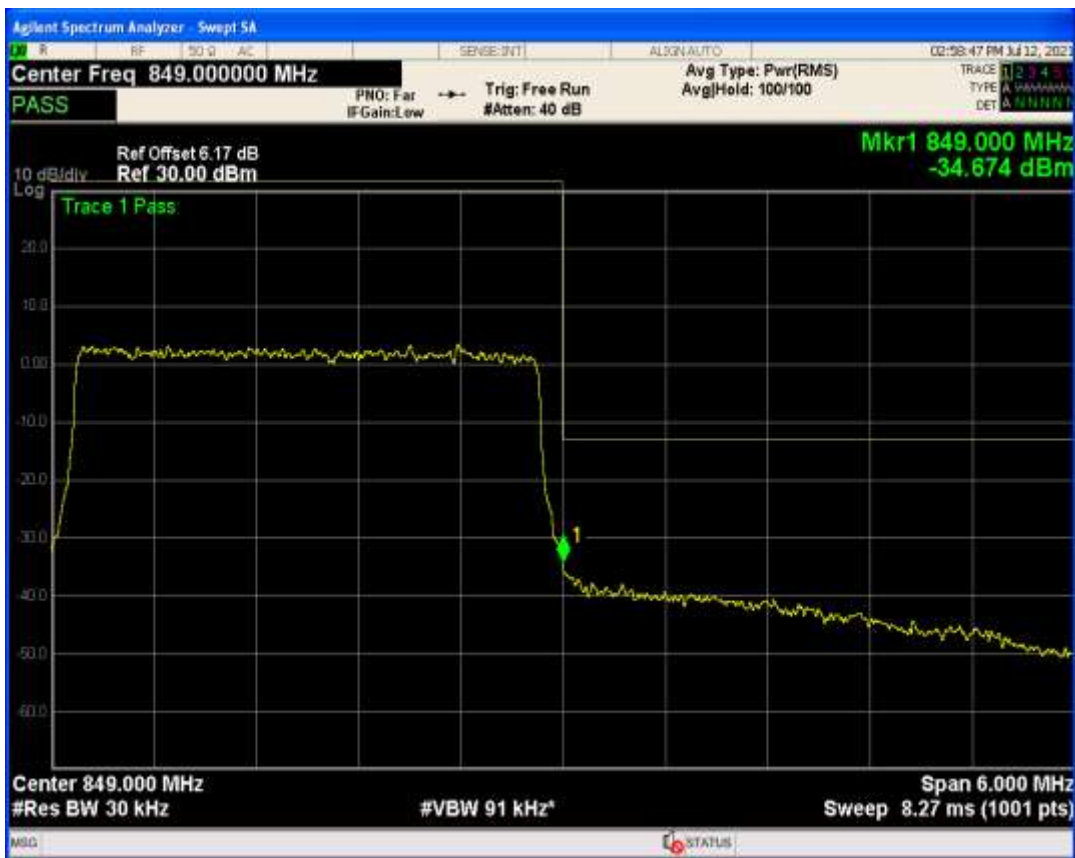
Band26b QAM16 BW=3MHz Channel=27025 RB Size=1 Position=#Max
