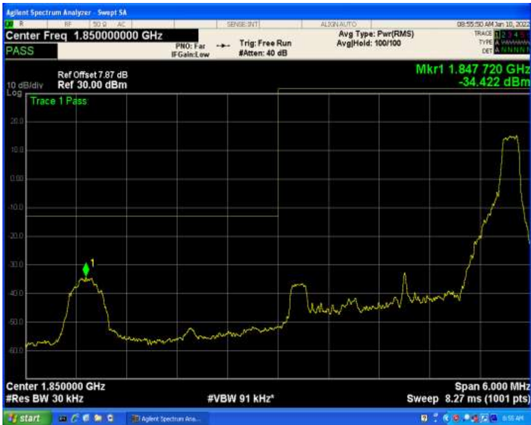
Band2 QPSK BW=3MHz Channel=19185 RB Size=1 Position=#0
