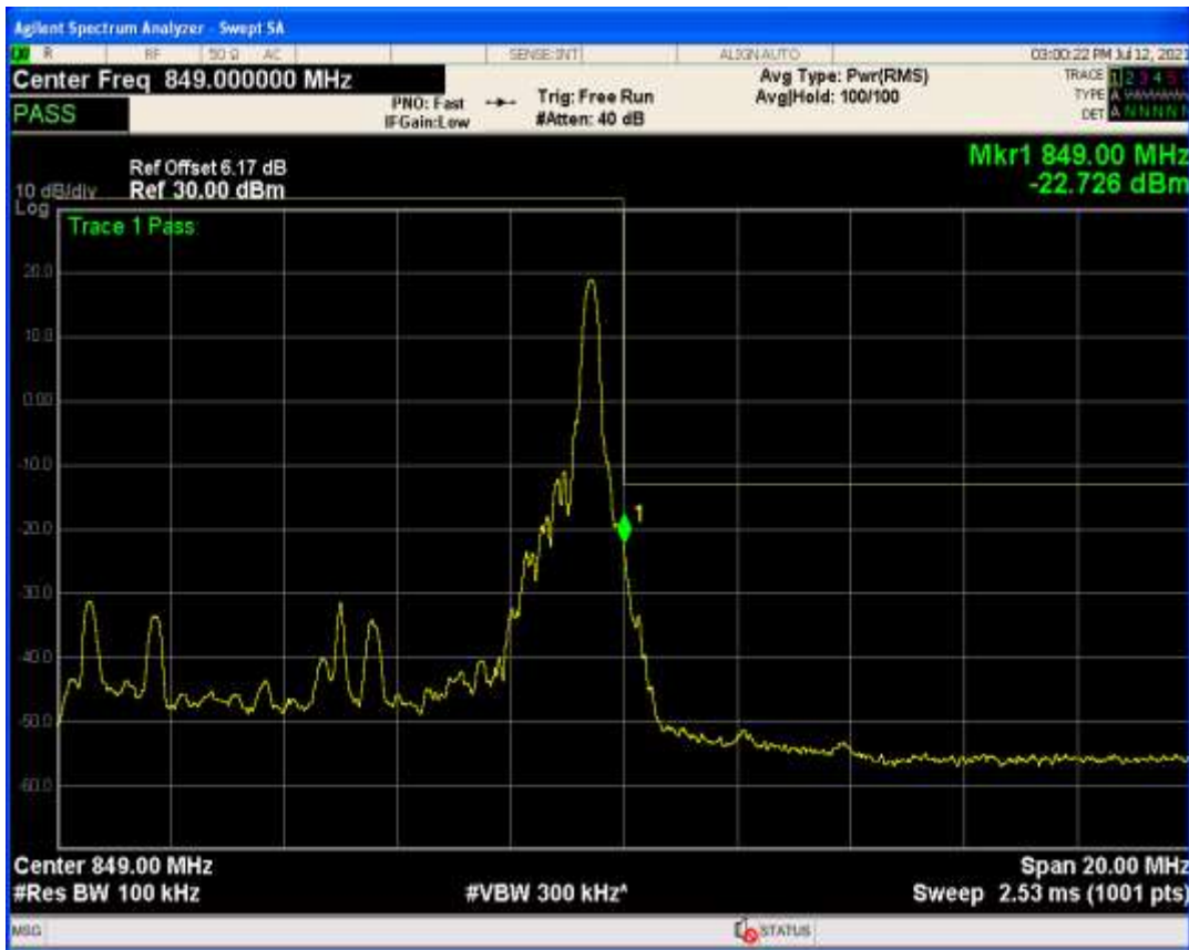
Band26b QAM16 BW=10MHz Channel=26840 RB Size=1 Position=#0
