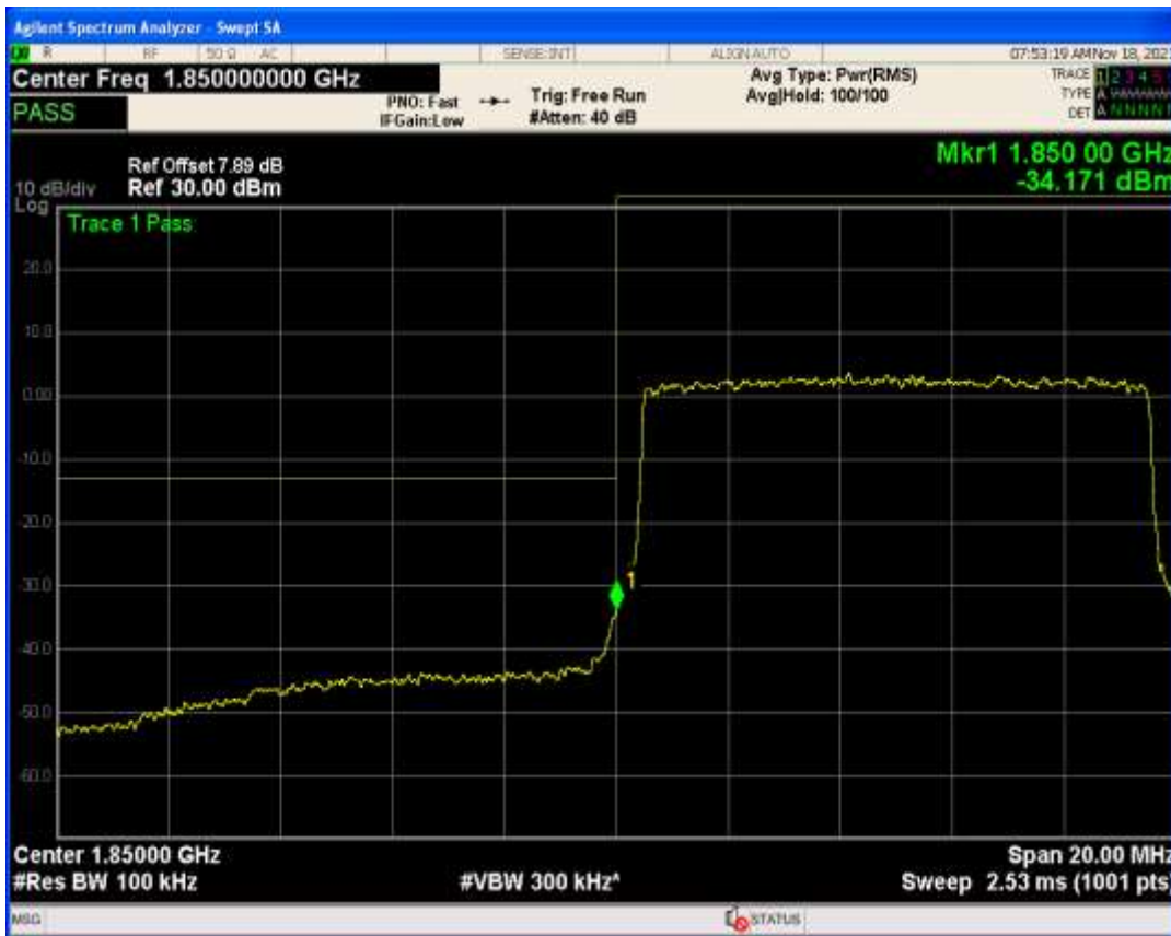
Band25 QPSK BW=10MHz Channel=26090 RB Size=1 Position=#Max
