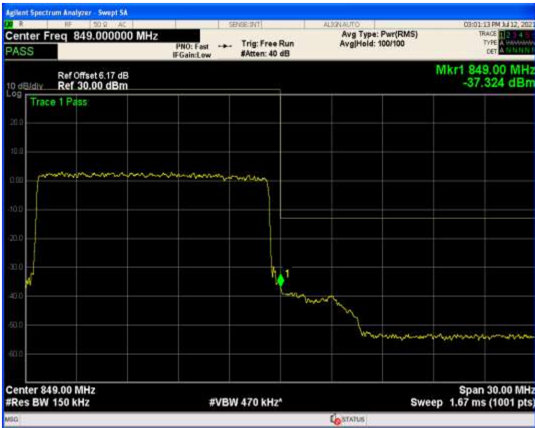
Band26b QPSK BW=10MHz Channel=26840 RB Size=50 Position=#0
