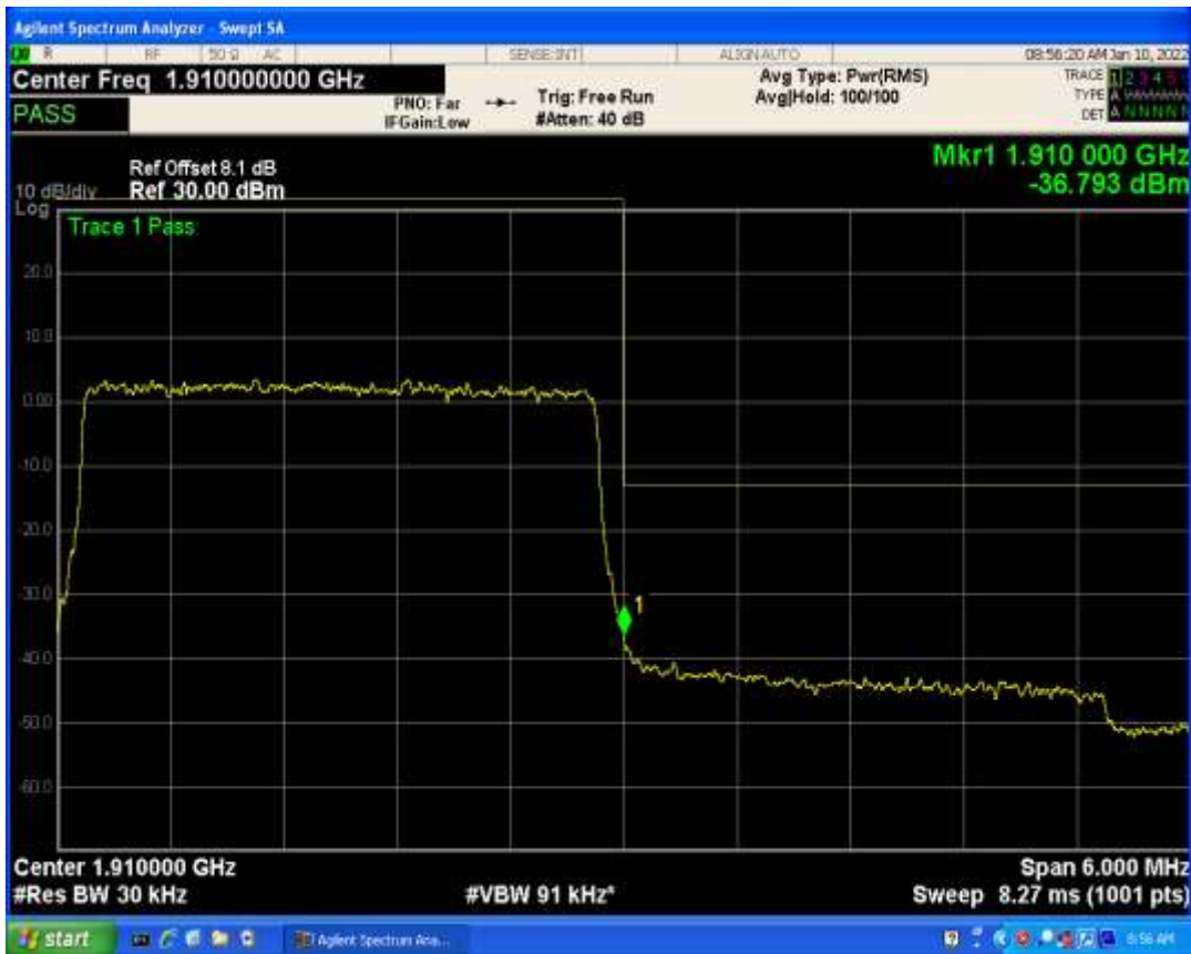
Band2 QPSK BW=3MHz Channel=19185 RB Size=1 Position=#Max
