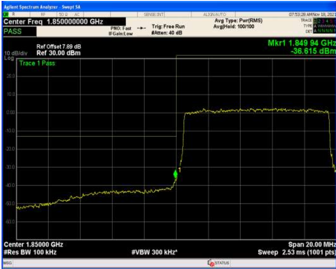
Band25 QAM16 BW=10MHz Channel=26640 RB Size=50 Position=#0
