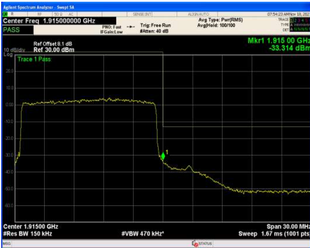
Band25 QPSK BW=5MHz Channel=26665 RB Size=1 Position=#0
