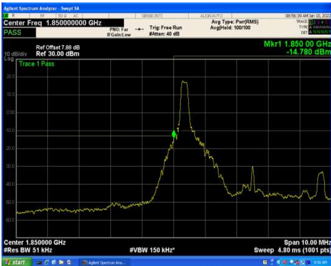
Band2 QPSK BW=5MHz Channel=18625 RB Size=1 Position=#Max
