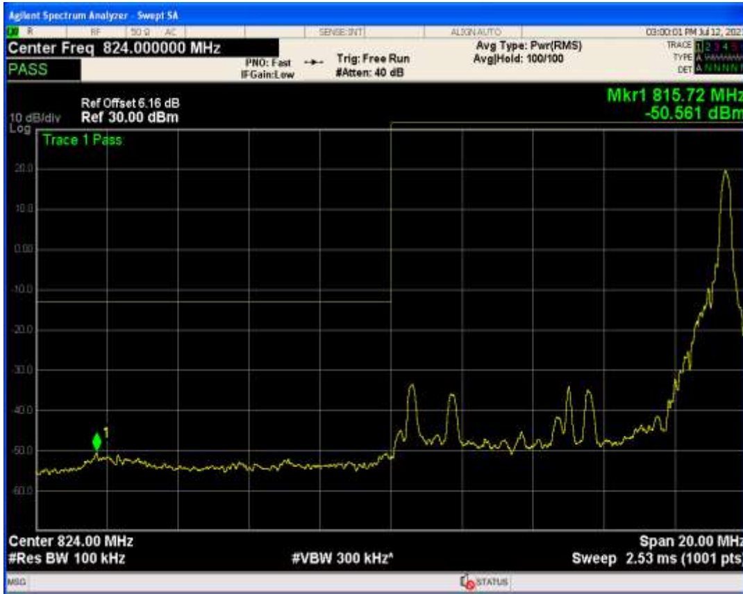
Band26b QAM16 BW=15MHz Channel=26865 RB Size=1 Position=#0
