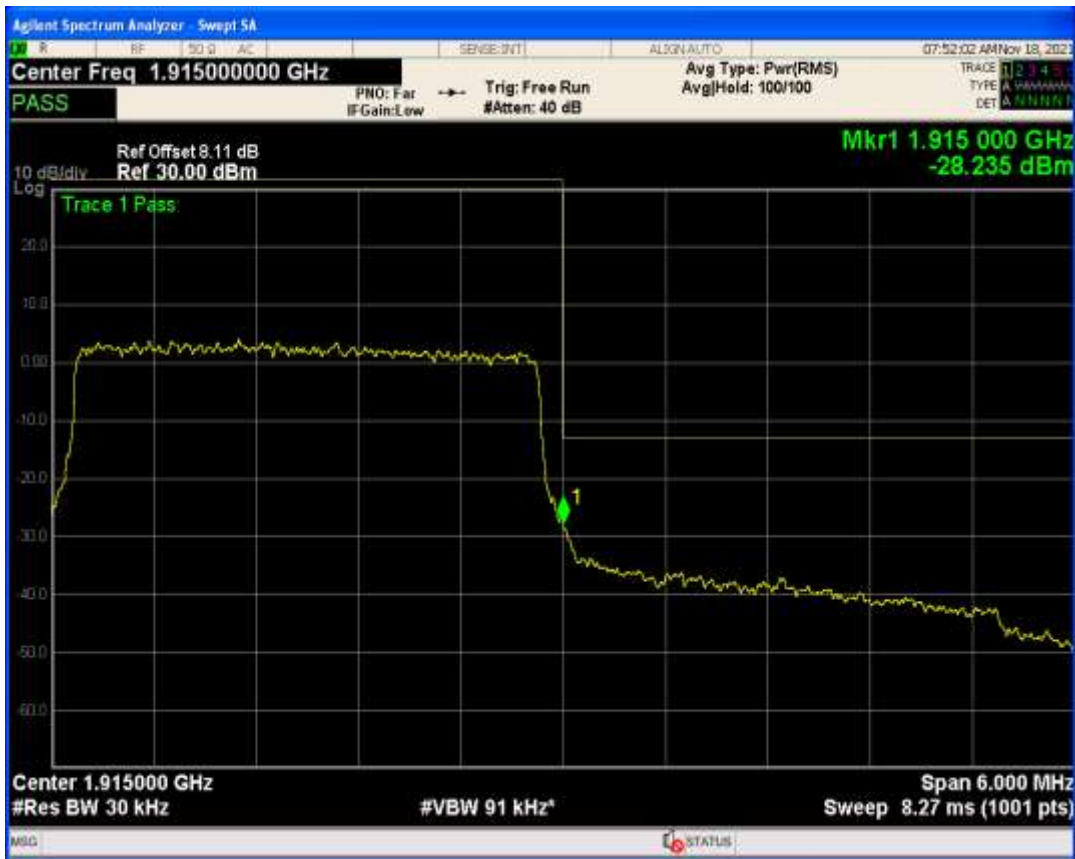
Band25 QPSK BW=3MHz Channel=26675 RB Size=1 Position=#Max
