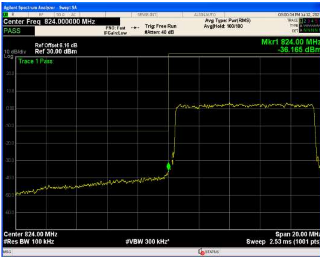
Band26b QAM16 BW=10MHz Channel=26840 RB Size=1 Position=#Max
