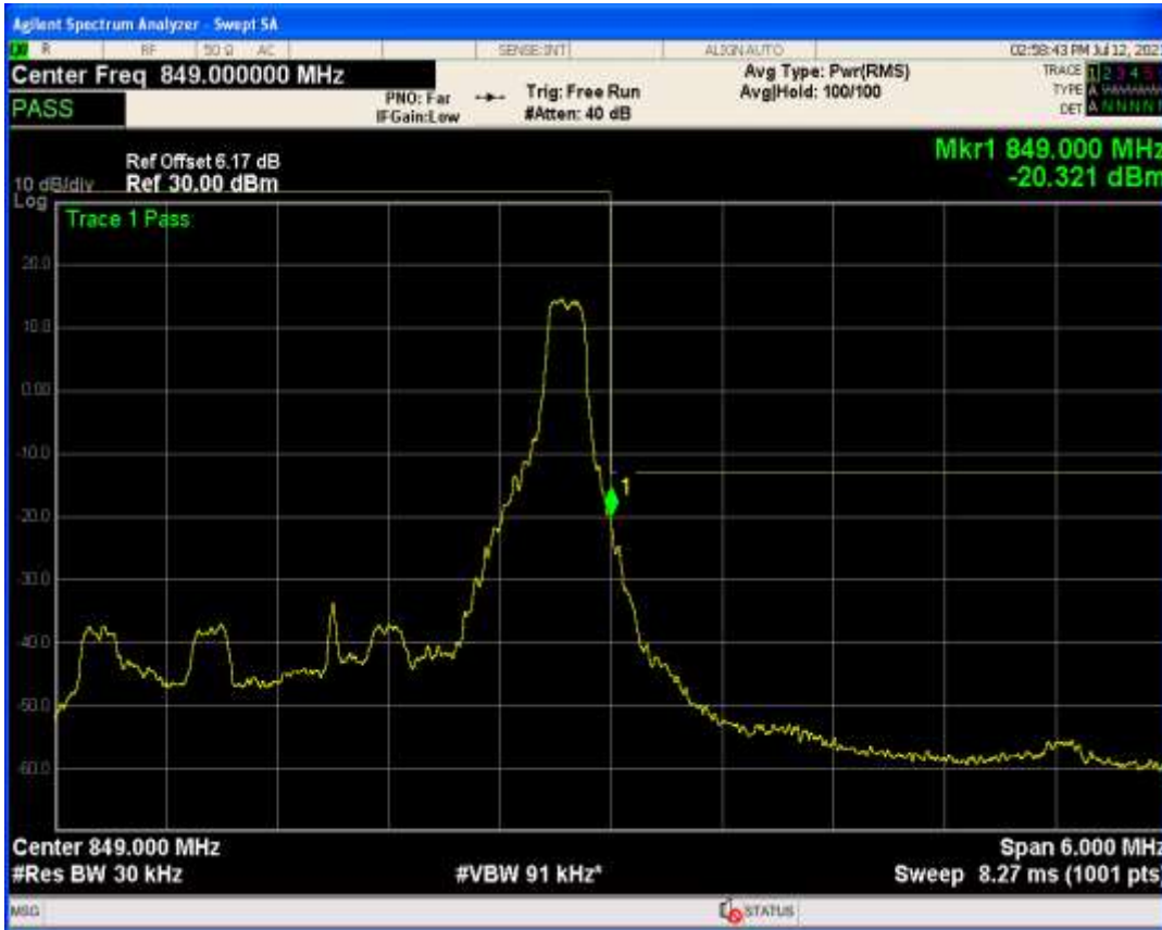
Band26b QAM16 BW=3MHz Channel=27025 RB Size=1 Position=#0
