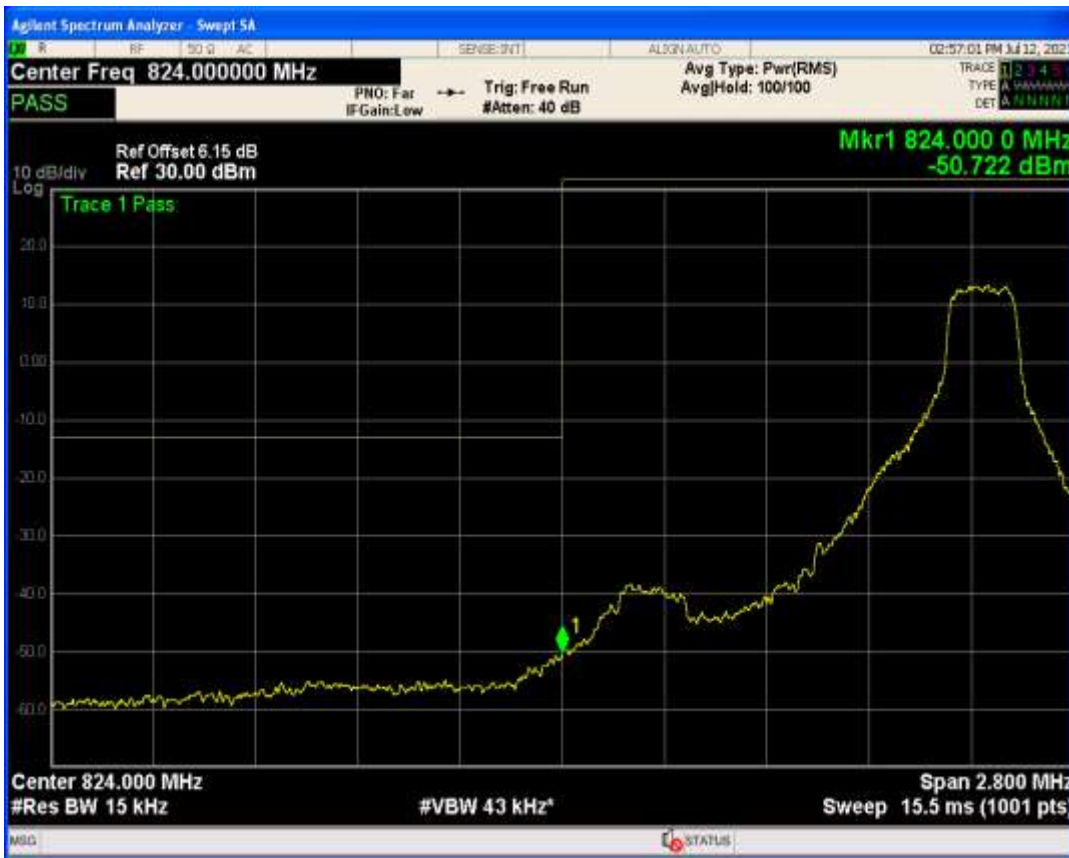
Band26b QAM16 BW=5MHz Channel=27015 RB Size=1 Position=#Max
