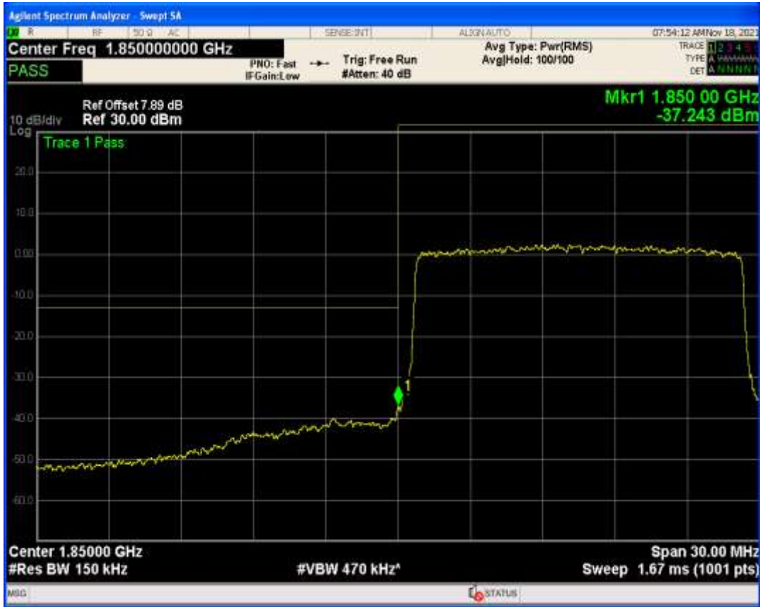
Band25 QAM16 BW=15MHz Channel=26115 RB Size=1 Position=#Max
