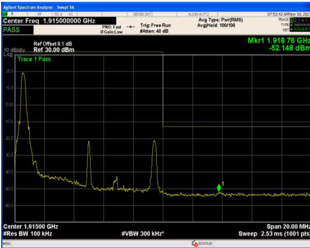
Band25 QAM16 BW=5MHz Channel=26065 RB Size=1 Position=#0
