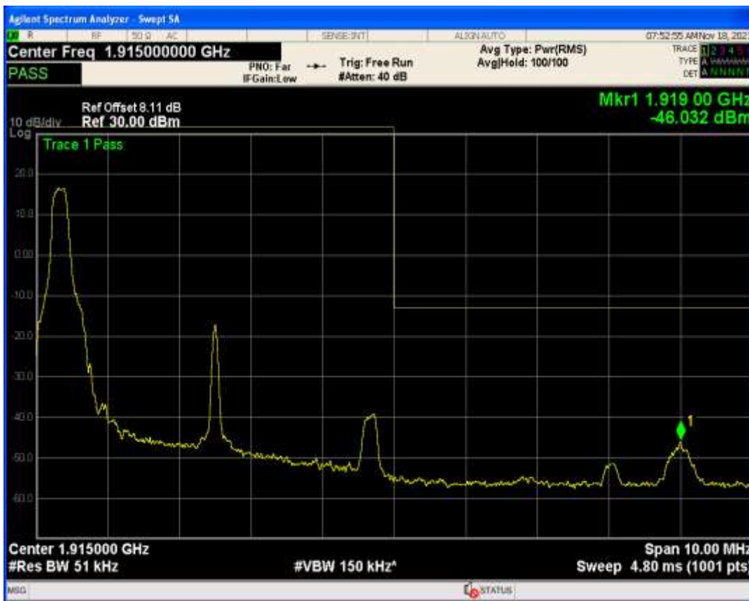
Band25 QAM16 BW=5MHz Channel=26065 RB Size=25 Position=#0
