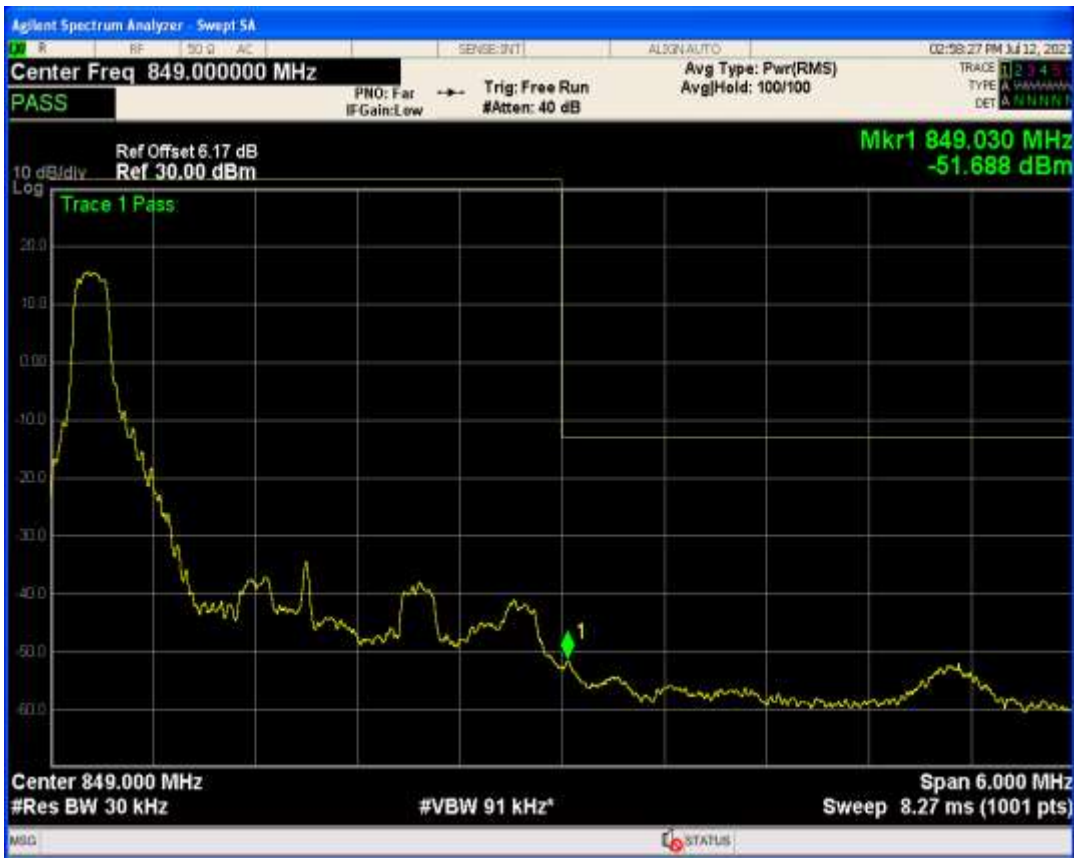
Band26b QPSK BW=3MHz Channel=26805 RB Size=1 Position=#0
