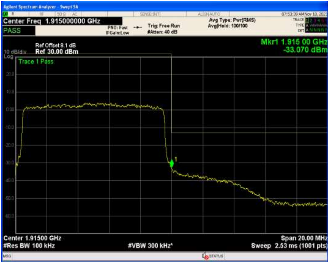
Band25 QPSK BW=10MHz Channel=26640 RB Size=1 Position=#Max
