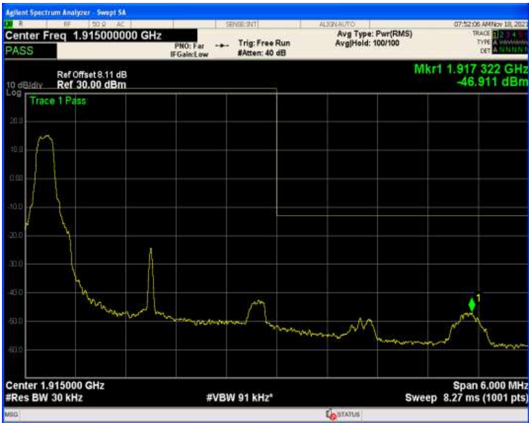
Band25 QAM16 BW=20MHz Channel=26590 RB Size=1 Position=#Max
