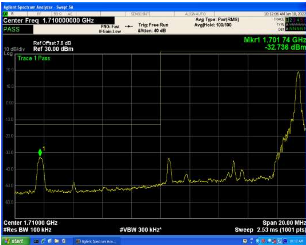
Band4 QAM16 BW=10MHz Channel=20000 RB Size=1 Position=#0
