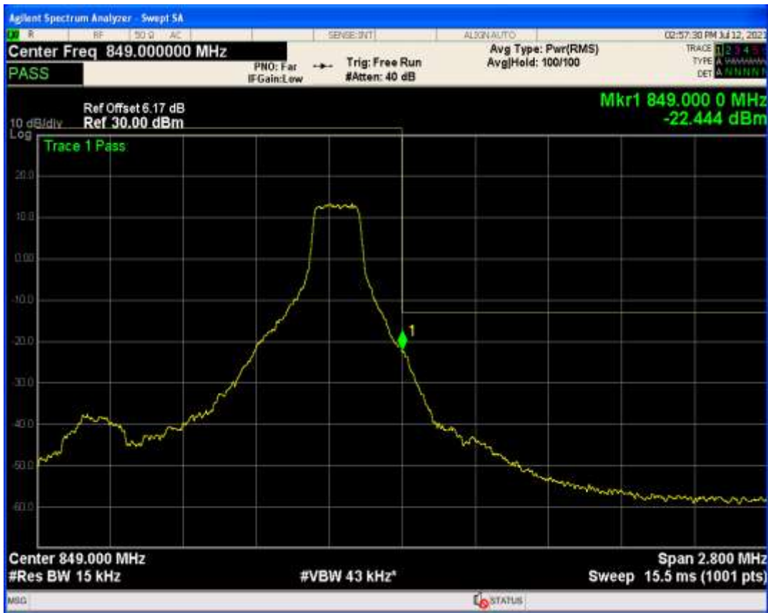
Band26b QPSK BW=1.4MHz Channel=27033 RB Size=6 Position=#0
