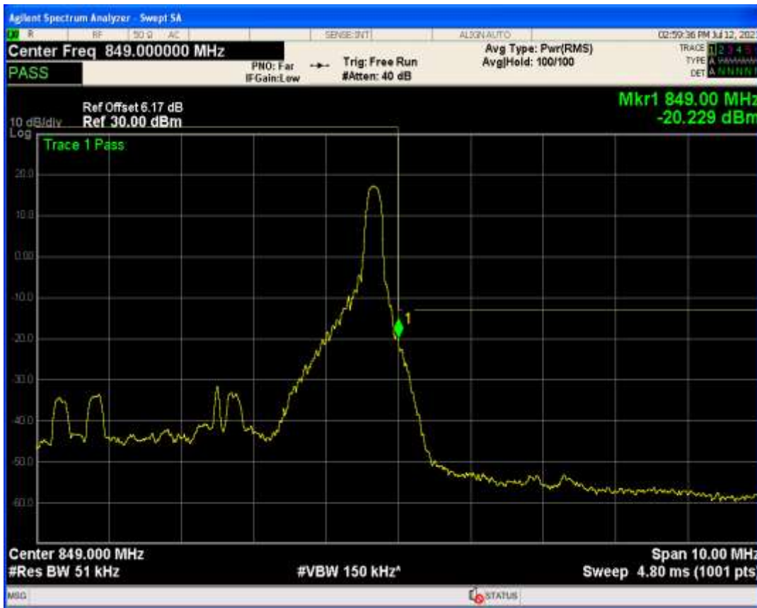
Band26b QAM16 BW=5MHz Channel=27015 RB Size=25 Position=#0
