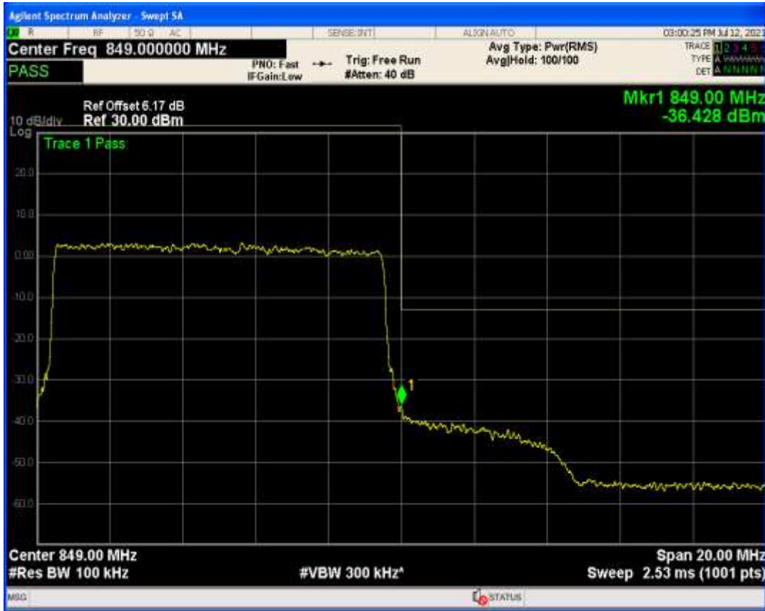
Band26b QAM16 BW=10MHz Channel=26990 RB Size=1 Position=#Max
