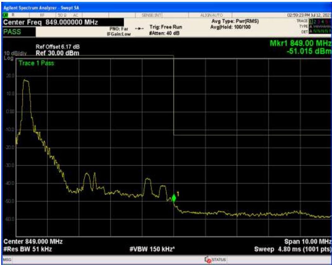
Band26b QPSK BW=15MHz Channel=26965 RB Size=1 Position=#Max
