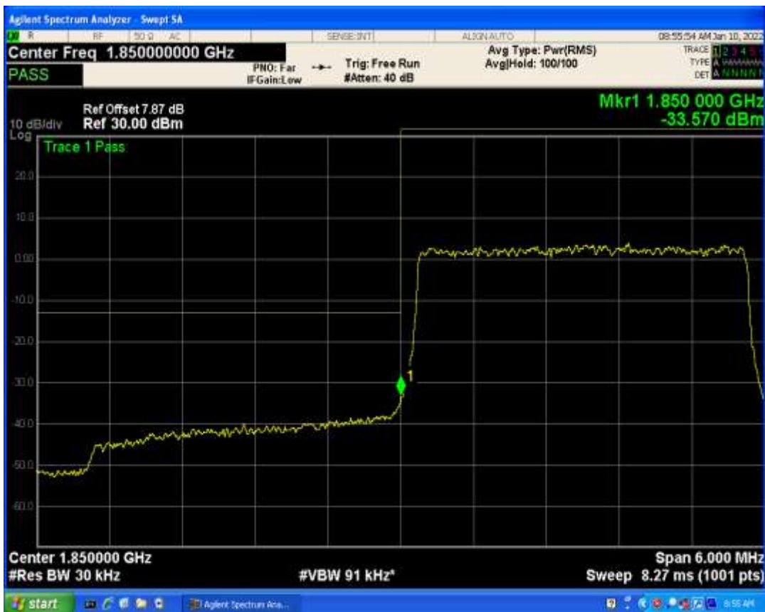
Band2 QPSK BW=3MHz Channel=18615 RB Size=1 Position=#Max
