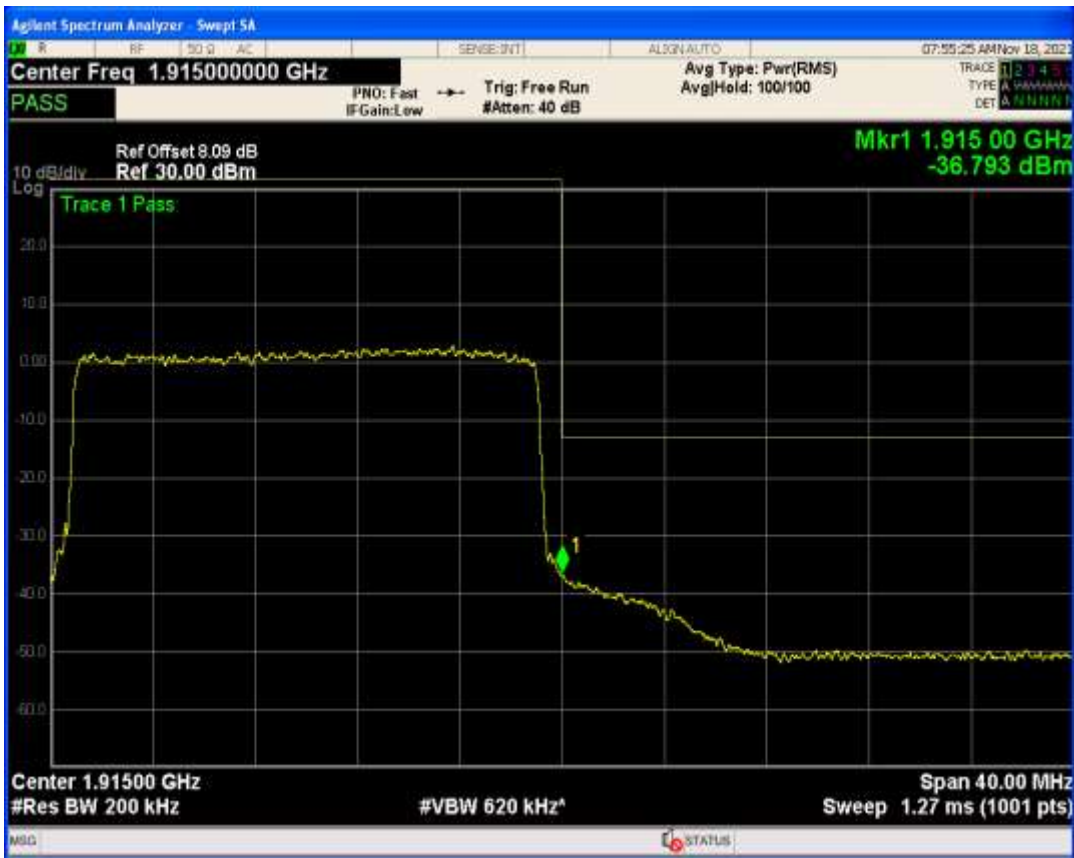
Band25 QAM16 BW=3MHz Channel=26055 RB Size=15 Position=#0
