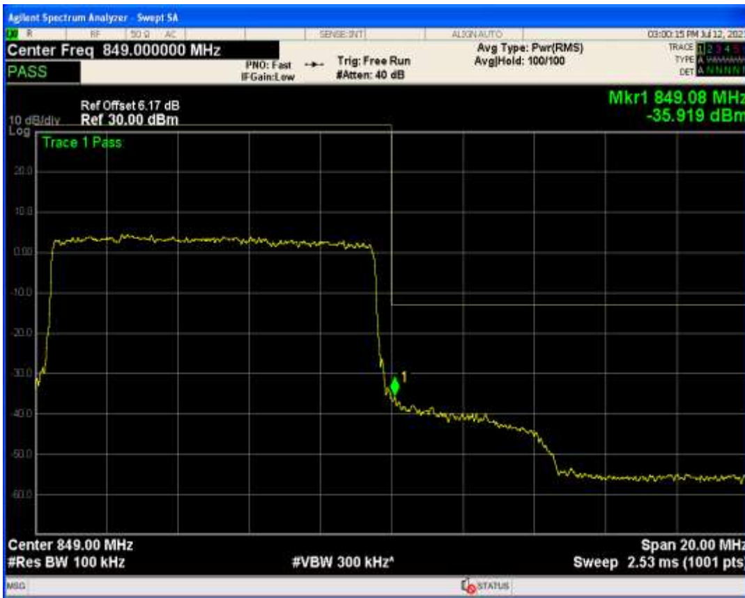
Band26b QPSK BW=1.4MHz Channel=26797 RB Size=1 Position=#0
