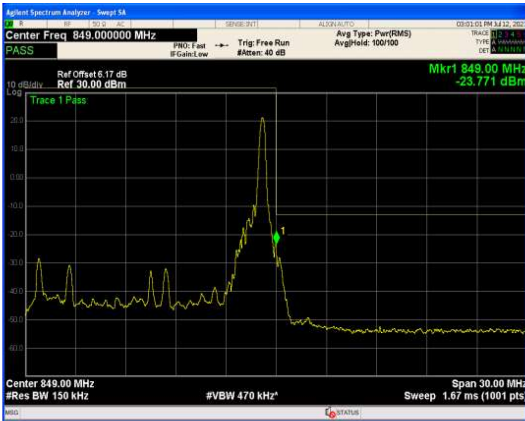
Band26b QPSK BW=15MHz Channel=26965 RB Size=75 Position=#0
