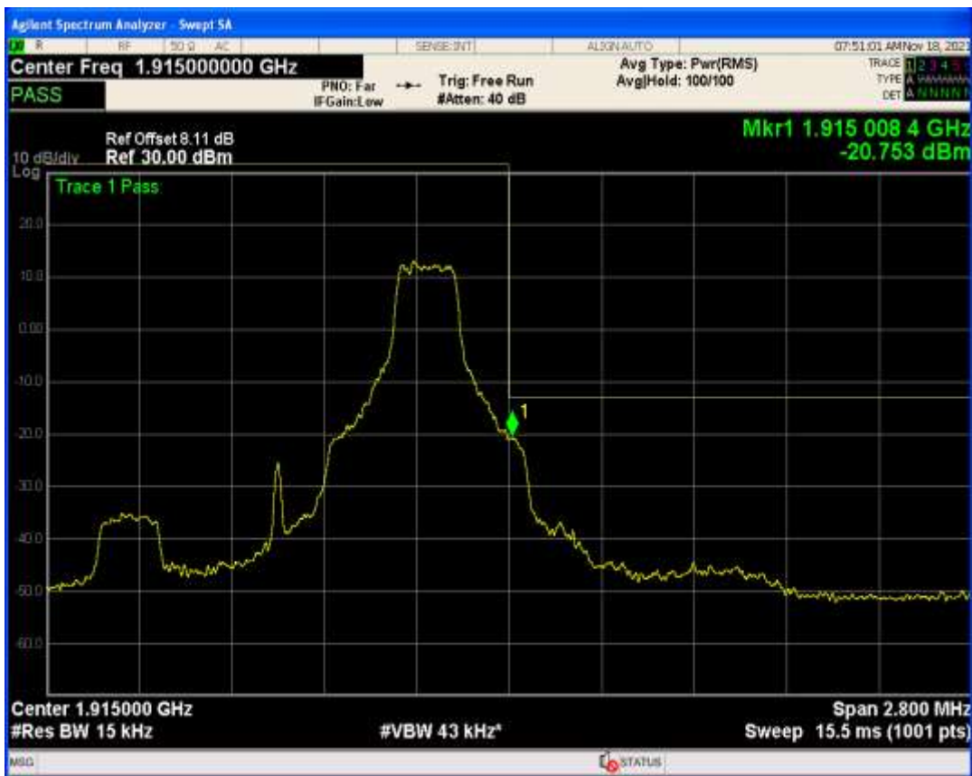
Band25 QPSK BW=1.4MHz Channel=26683 RB Size=1 Position=#0
