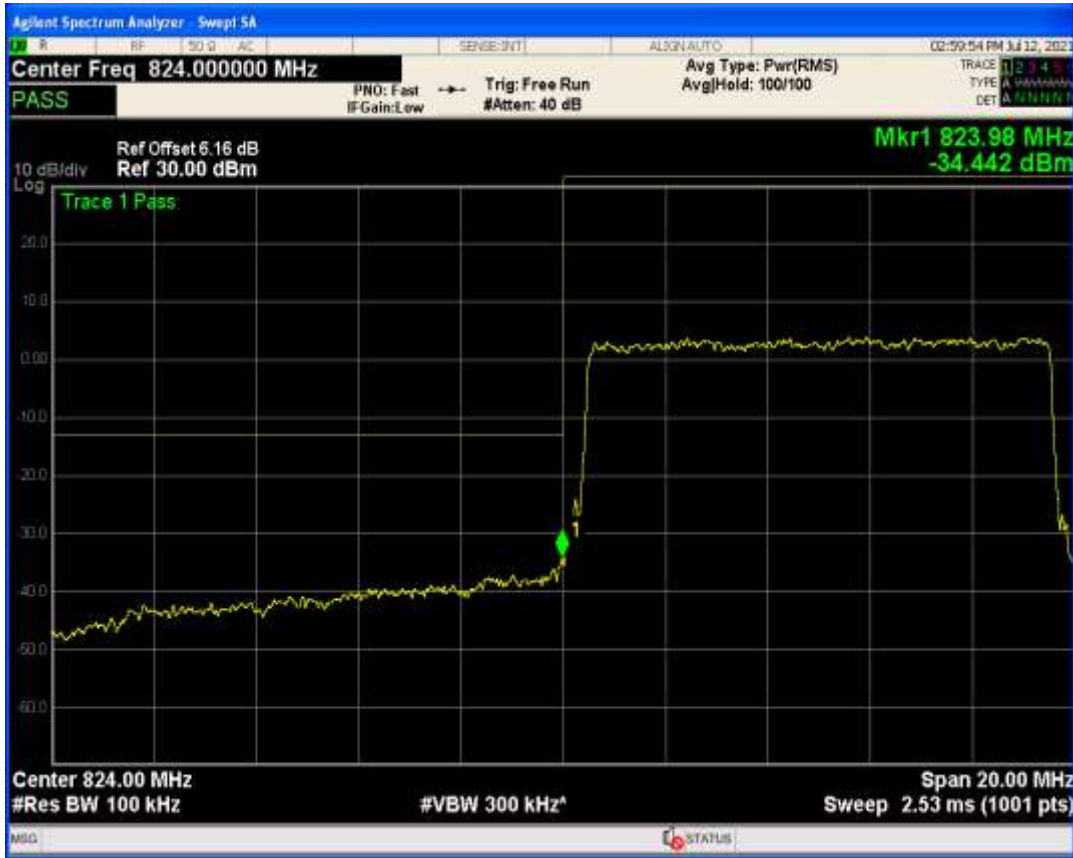
Band26b QPSK BW=10MHz Channel=26990 RB Size=1 Position=#0
