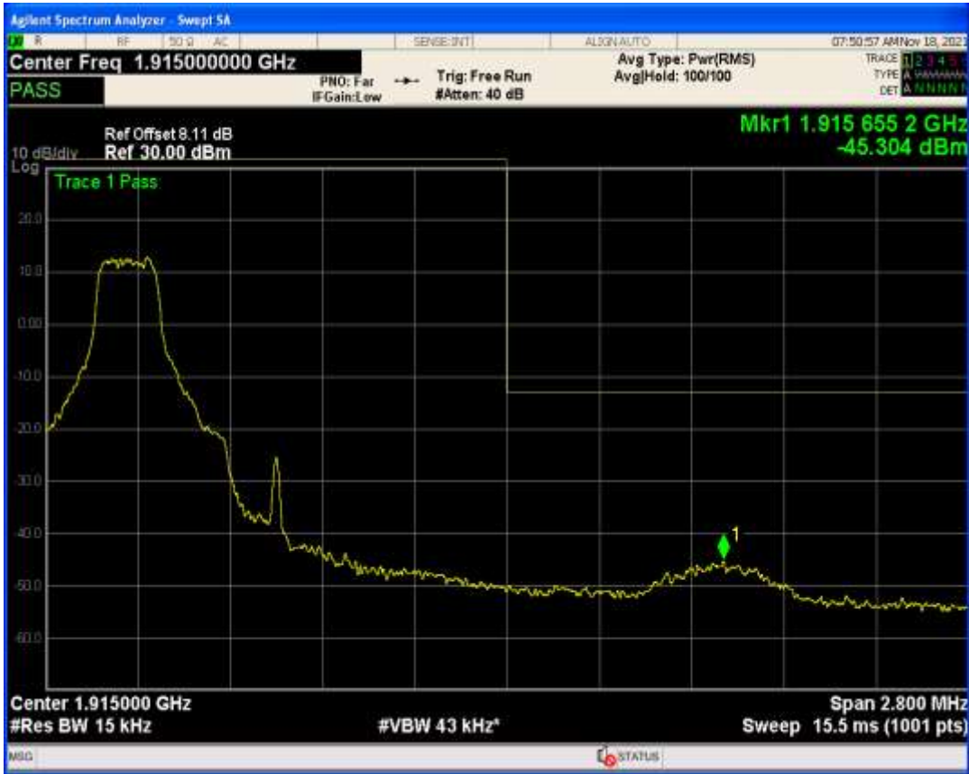
Band25 QPSK BW=20MHz Channel=26590 RB Size=100 Position=#0
