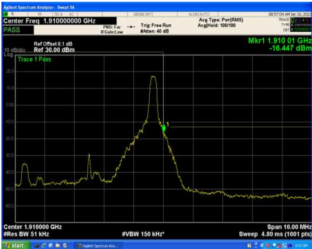
Band2 QPSK BW=5MHz Channel=19175 RB Size=25 Position=#0
