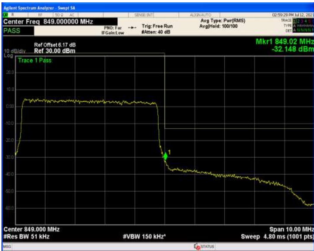
Band26b QPSK BW=5MHz Channel=26815 RB Size=25 Position=#0
