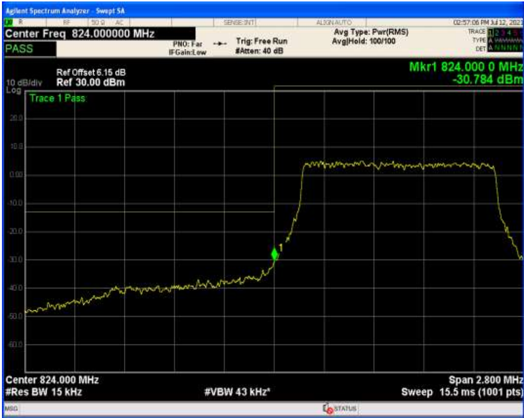
Band26b QPSK BW=1.4MHz Channel=27033 RB Size=1 Position=#0
