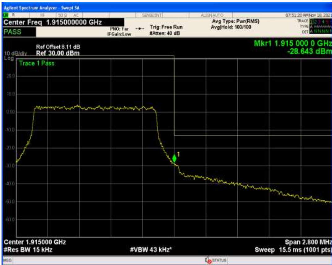
Band25 QAM16 BW=10MHz Channel=26090 RB Size=50 Position=#0
