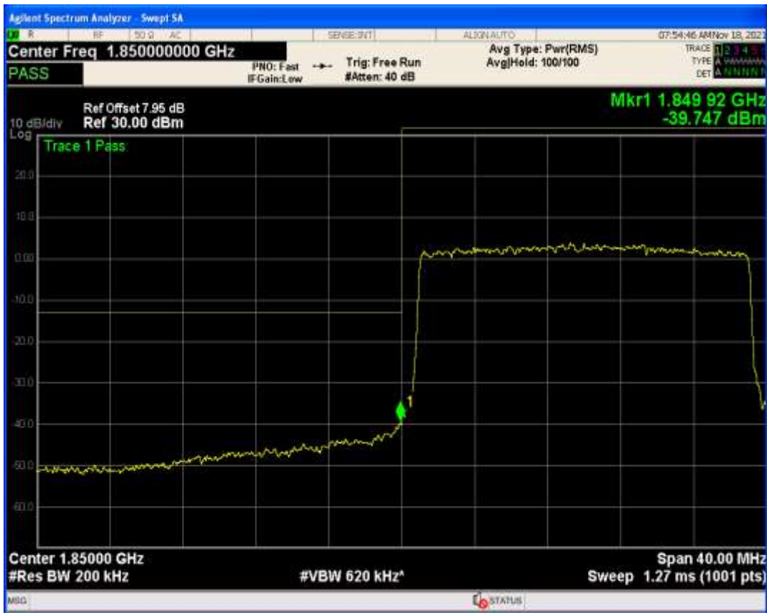
Band25 QPSK BW=15MHz Channel=26615 RB Size=1 Position=#0
