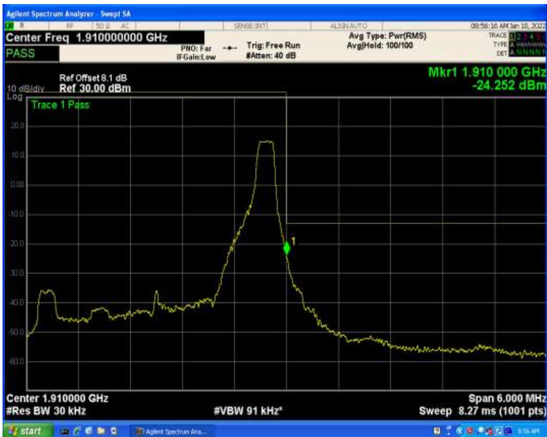
Band2 QPSK BW=3MHz Channel=18615 RB Size=1 Position=#0
