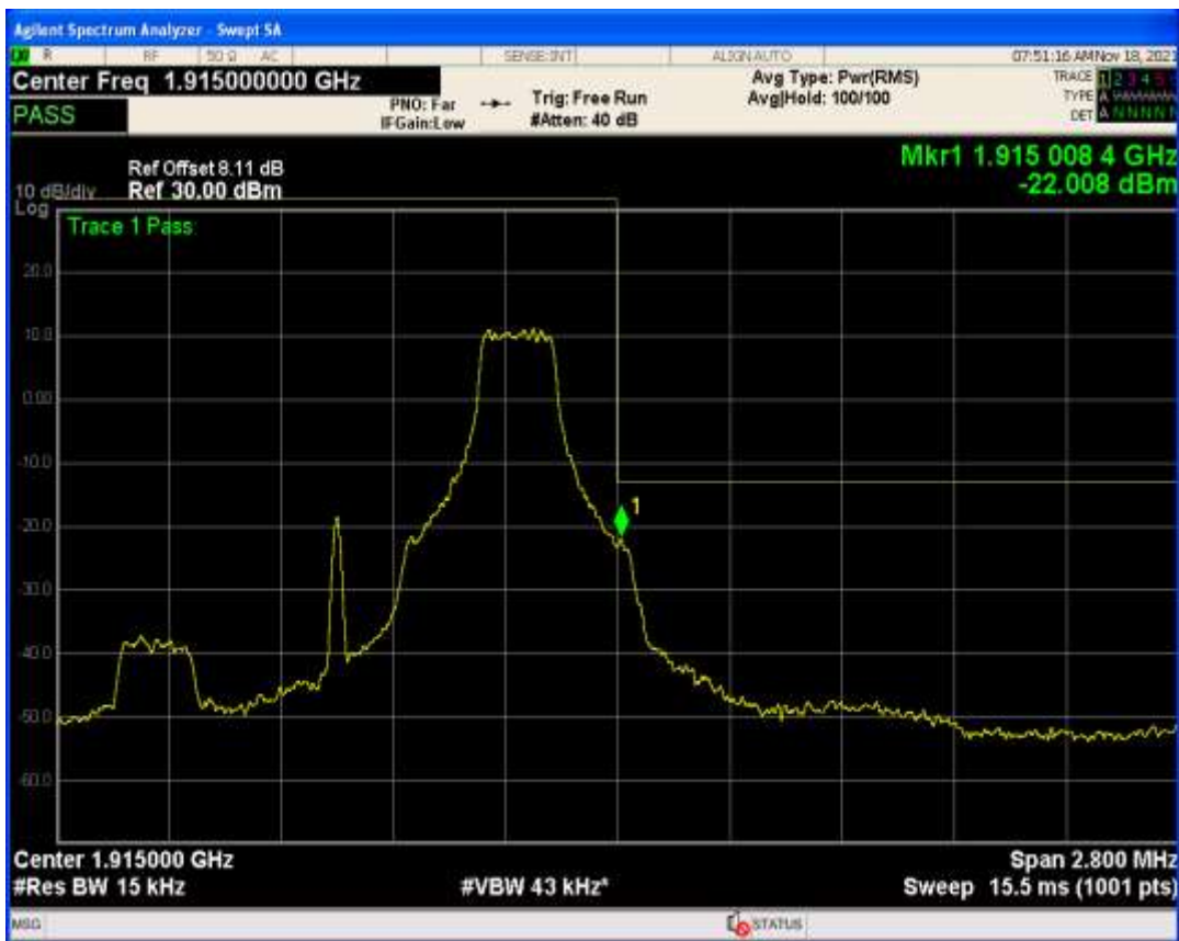
Band25 QAM16 BW=1.4MHz Channel=26047 RB Size=6 Position=#0
