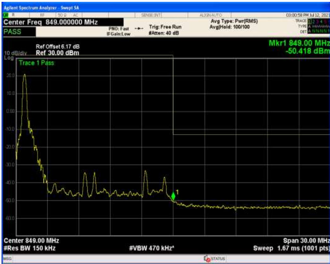
Band26b QPSK BW=3MHz Channel=26805 RB Size=15 Position=#0
