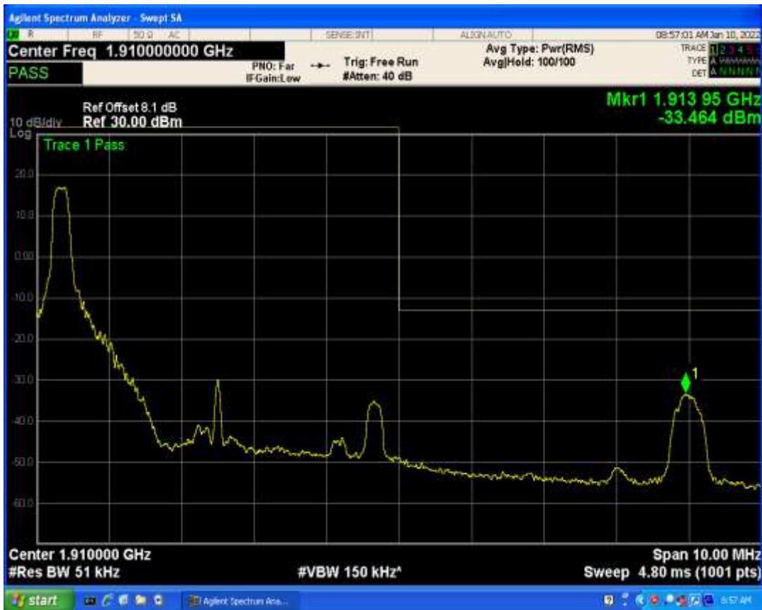
Band2 QPSK BW=5MHz Channel=19175 RB Size=1 Position=#Max
