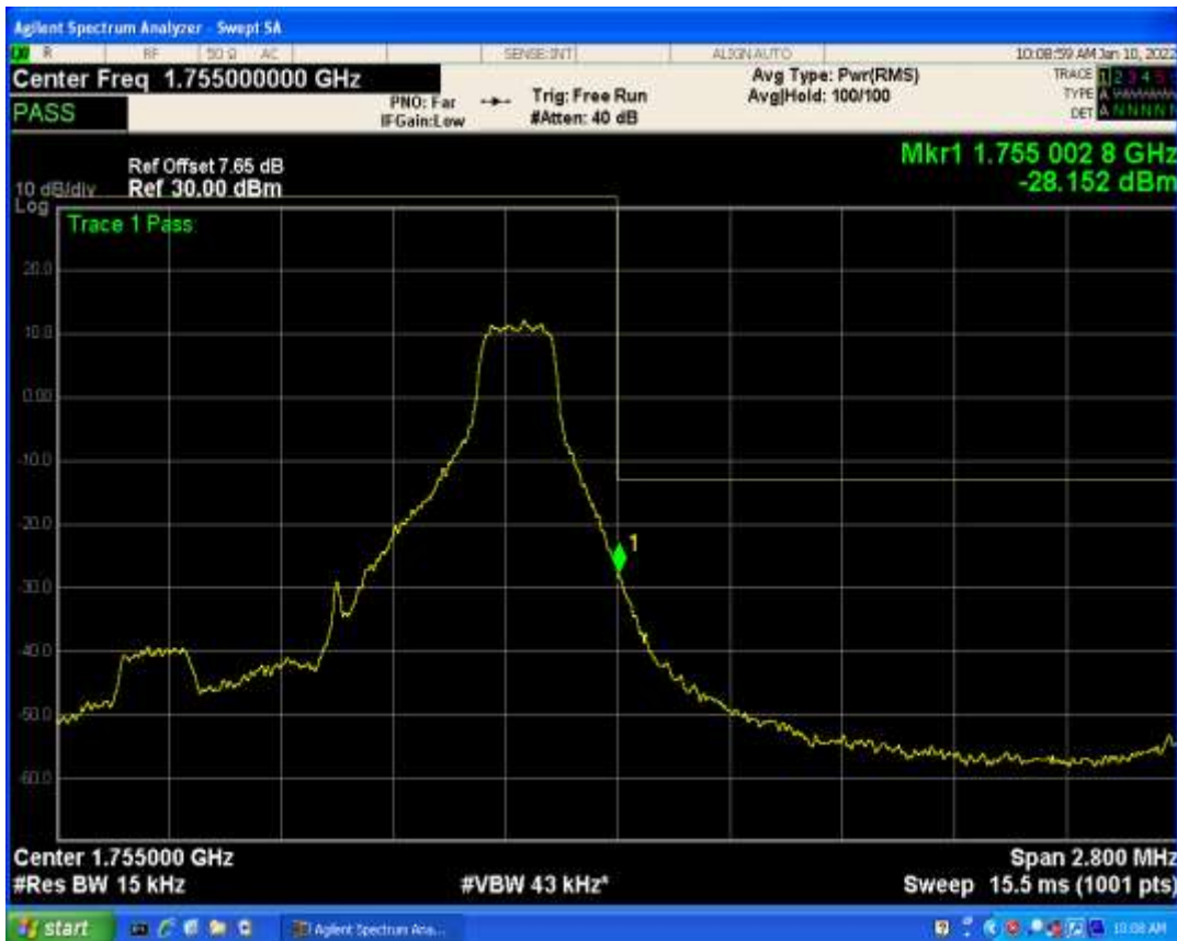
Band4 QAM16 BW=10MHz Channel=20000 RB Size=1 Position=#Max
