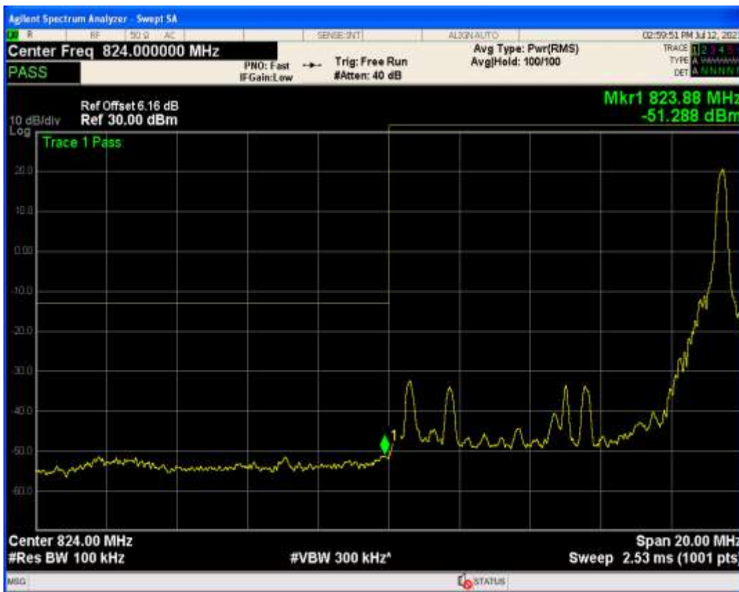
Band26b QPSK BW=15MHz Channel=26865 RB Size=1 Position=#0
