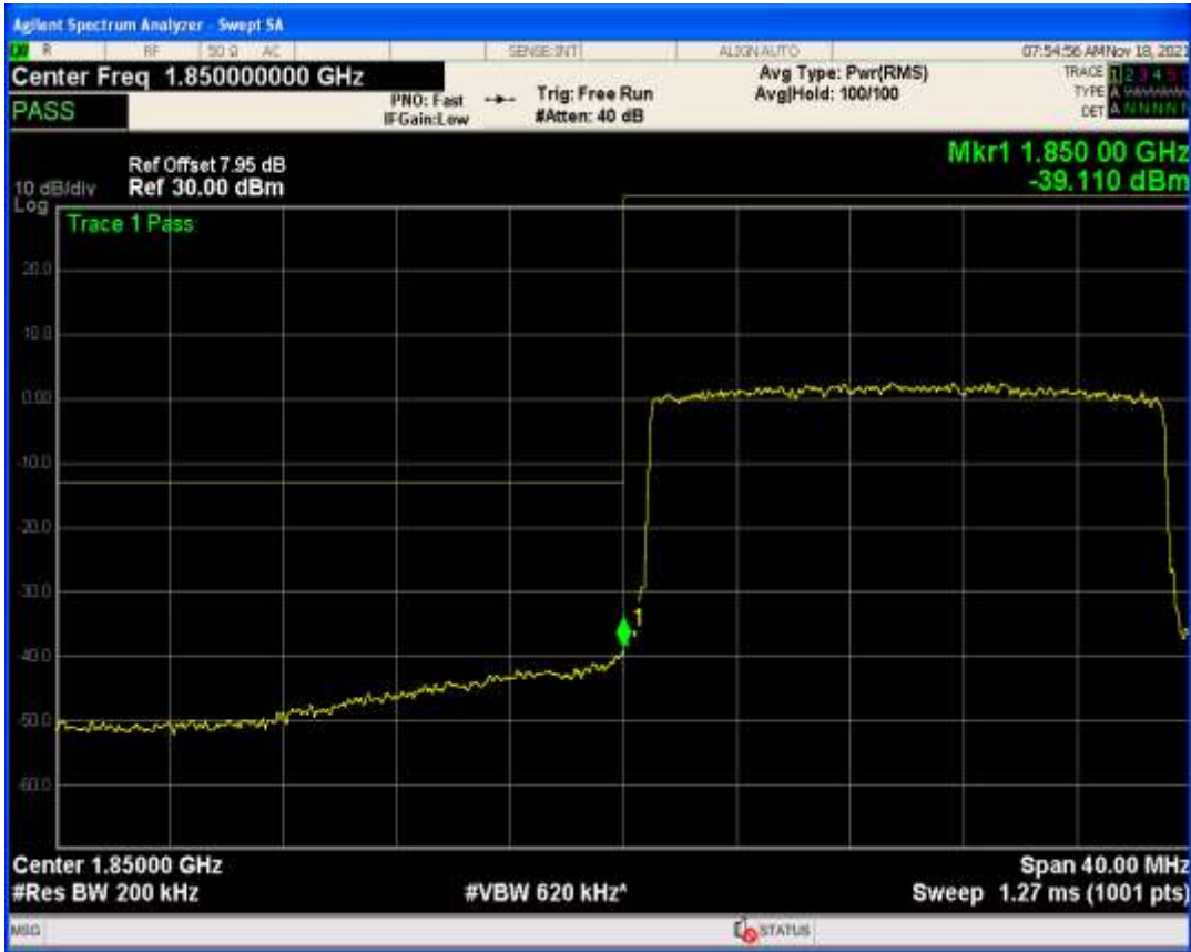
Band25 QAM16 BW=20MHz Channel=26590 RB Size=100 Position=#0
