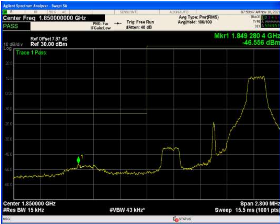
Band25 QAM16 BW=15MHz Channel=26615 RB Size=1 Position=#0
