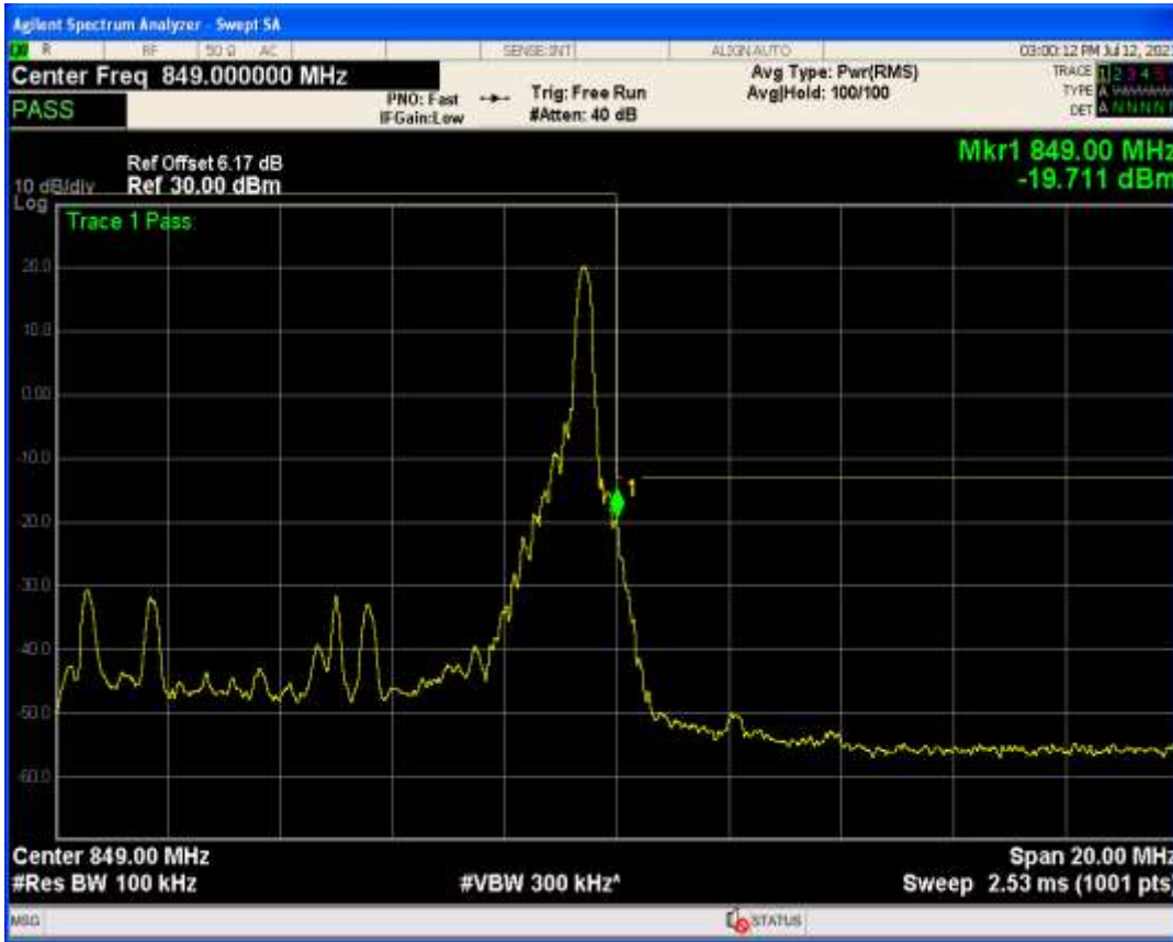
Band26b QPSK BW=10MHz Channel=26990 RB Size=50 Position=#0
