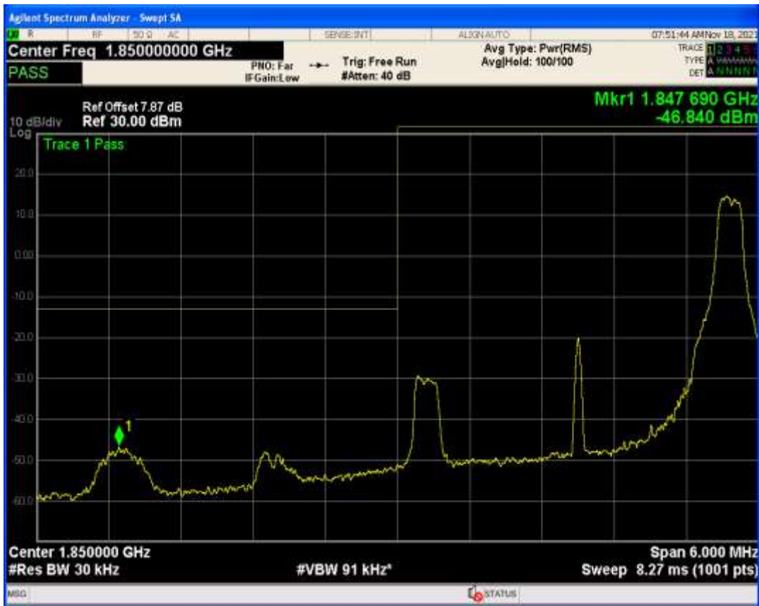
Band25 QAM16 BW=3MHz Channel=26055 RB Size=1 Position=#0
