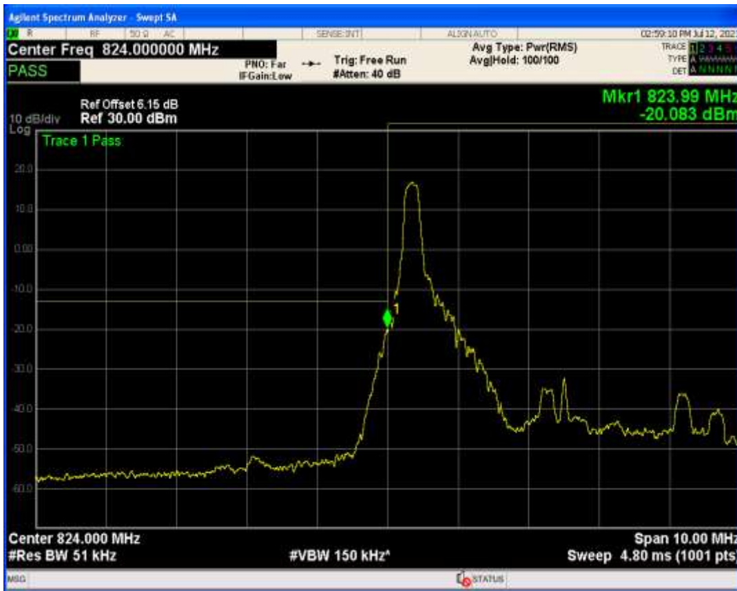
Band26b QAM16 BW=5MHz Channel=27015 RB Size=1 Position=#0
