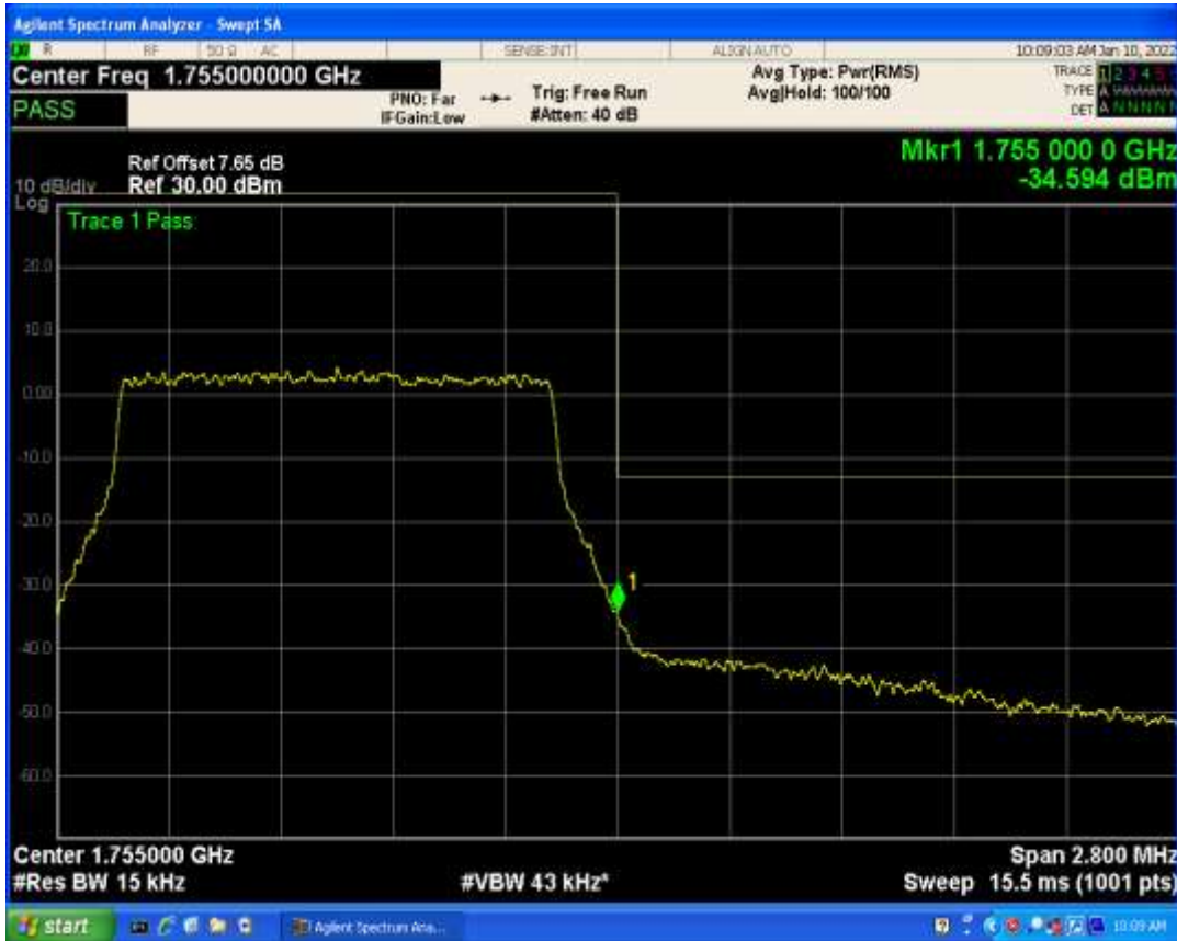
Band4 QAM16 BW=1.4MHz Channel=20393 RB Size=1 Position=#Max
