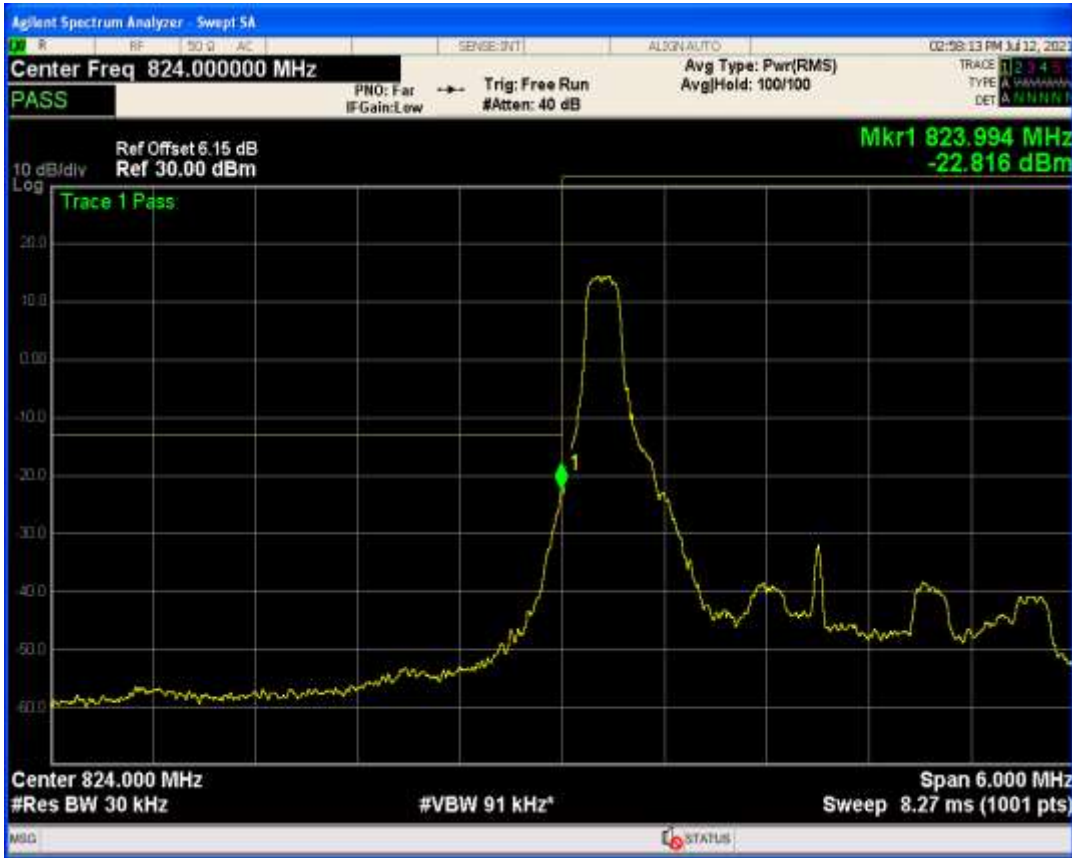
Band26b QAM16 BW=15MHz Channel=26965 RB Size=75 Position=#0
