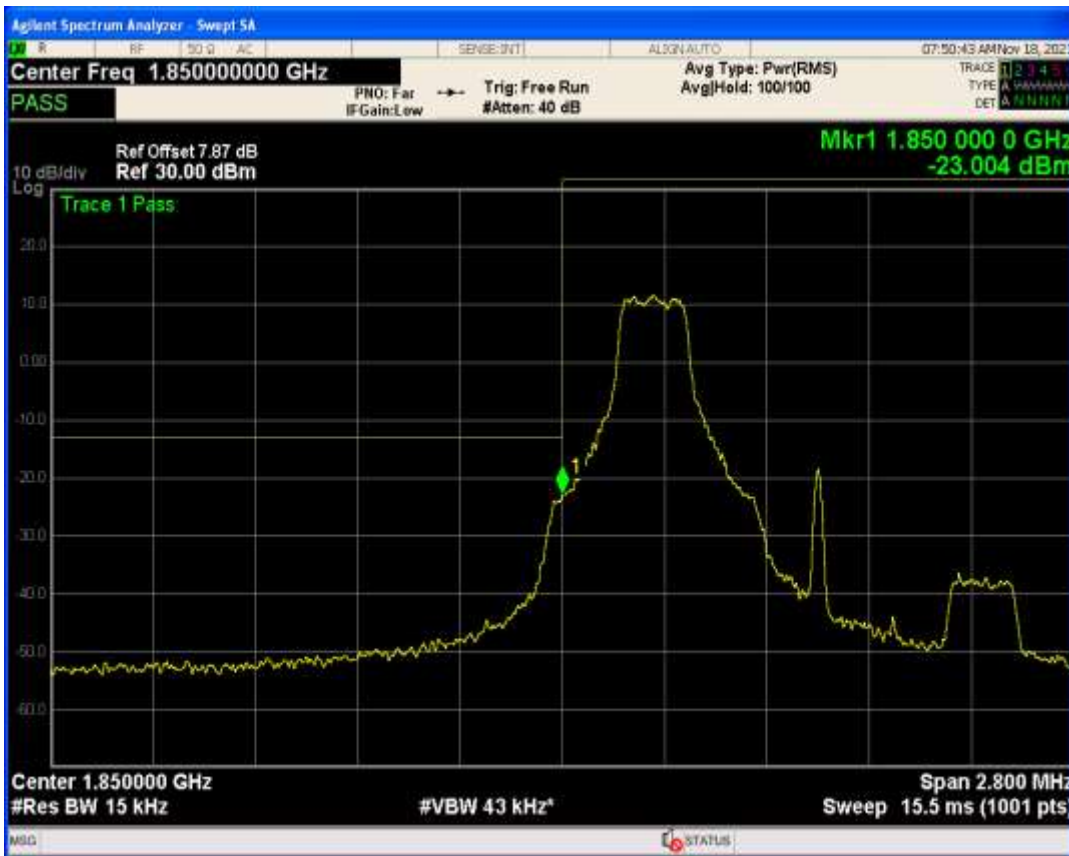
Band25 QAM16 BW=1.4MHz Channel=26047 RB Size=1 Position=#Max
