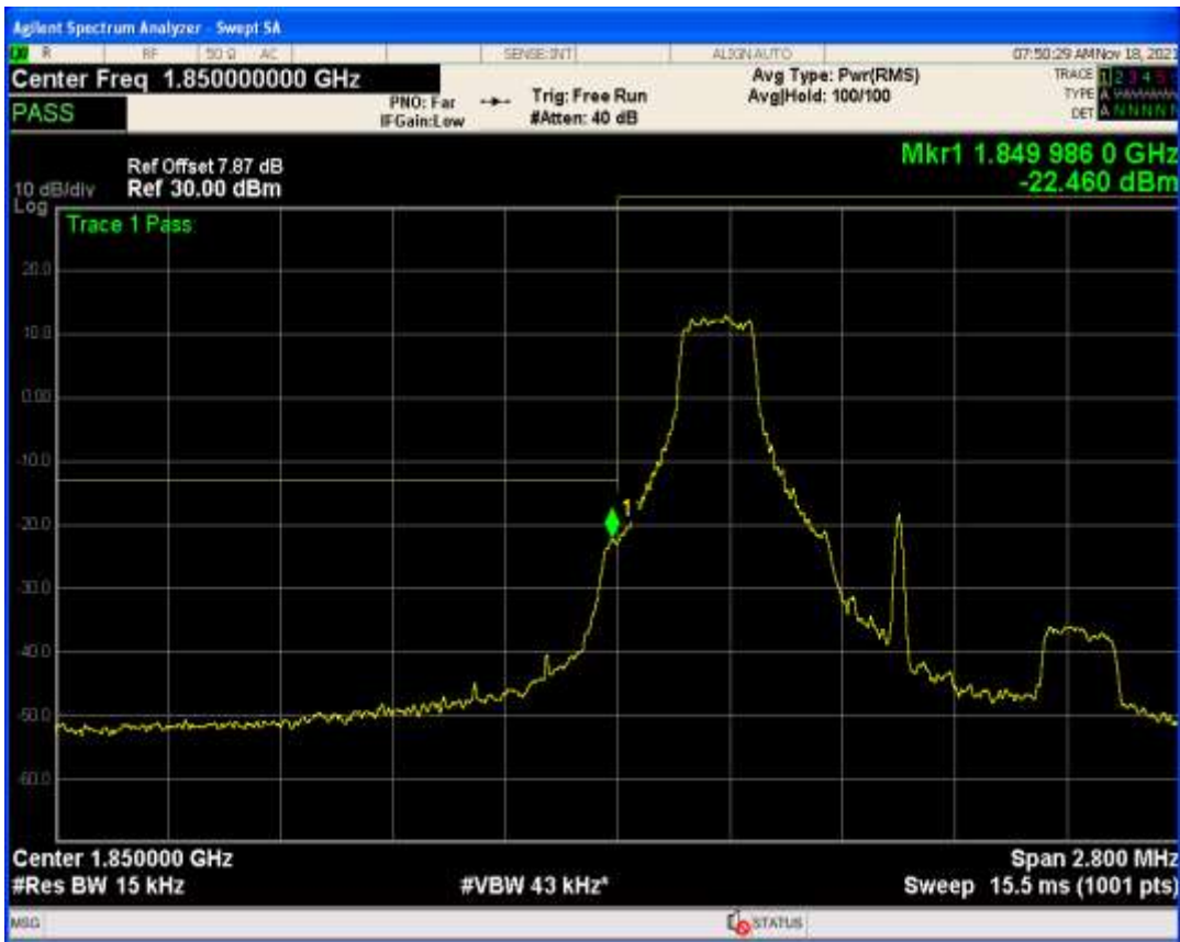
Band25 QAM16 BW=5MHz Channel=26665 RB Size=25 Position=#0
