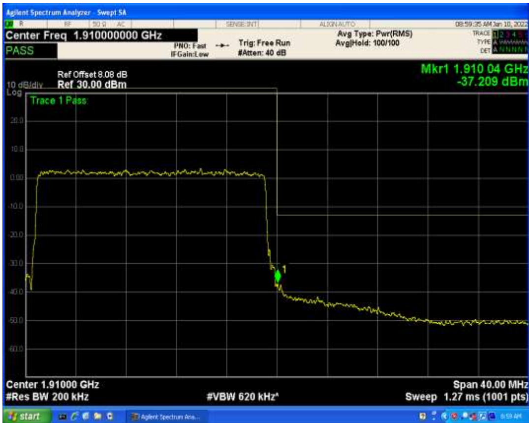
Band2 QPSK BW=20MHz Channel=19100 RB Size=1 Position=#Max
