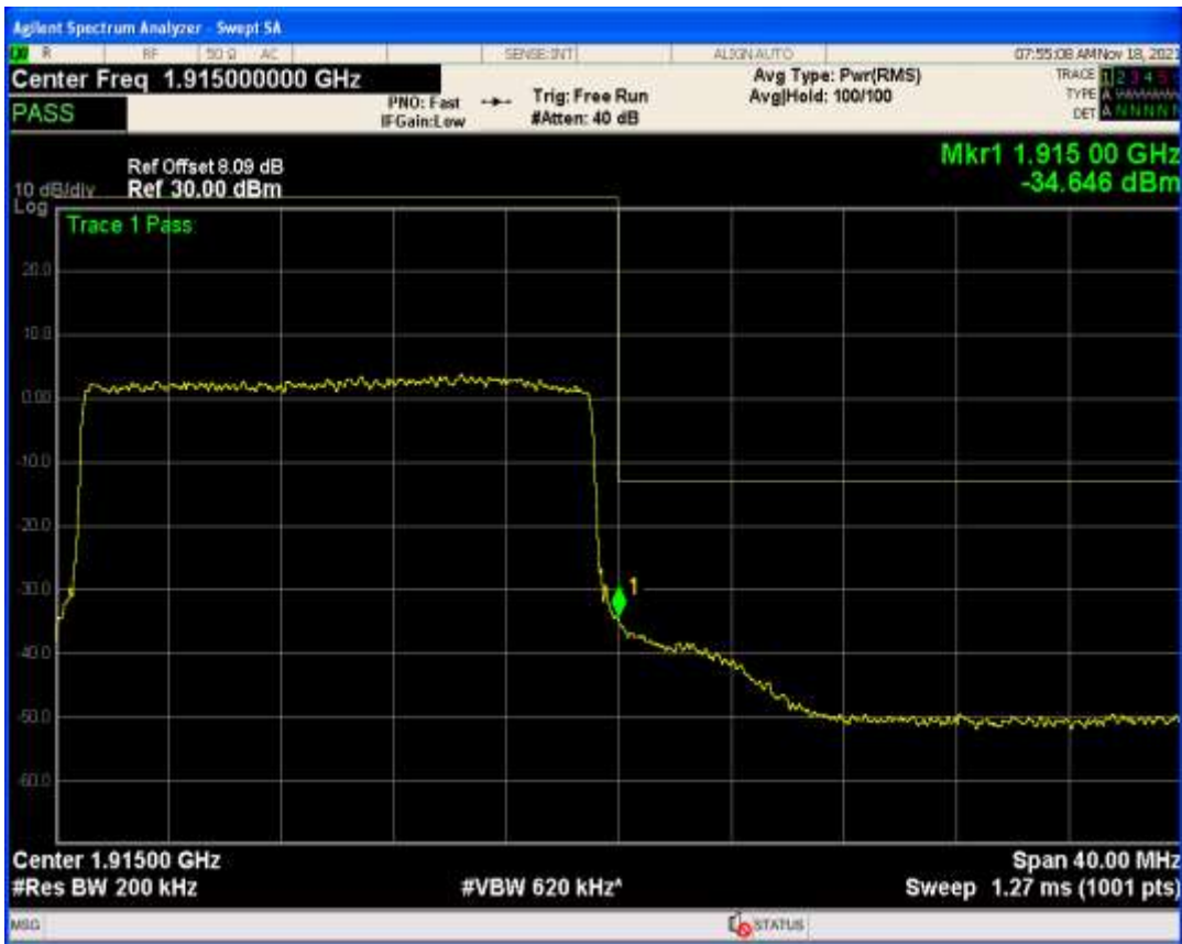
Band25 QPSK BW=20MHz Channel=26590 RB Size=1 Position=#Max
