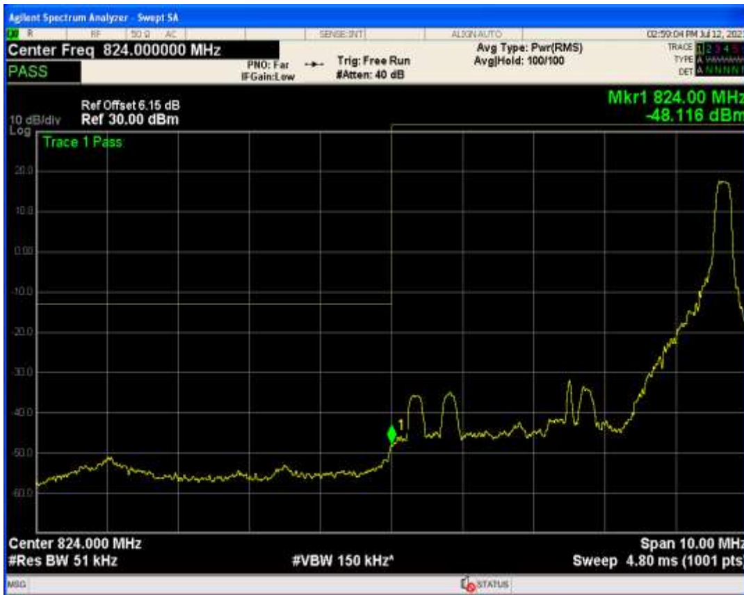
Band26b QPSK BW=3MHz Channel=27025 RB Size=1 Position=#Max
