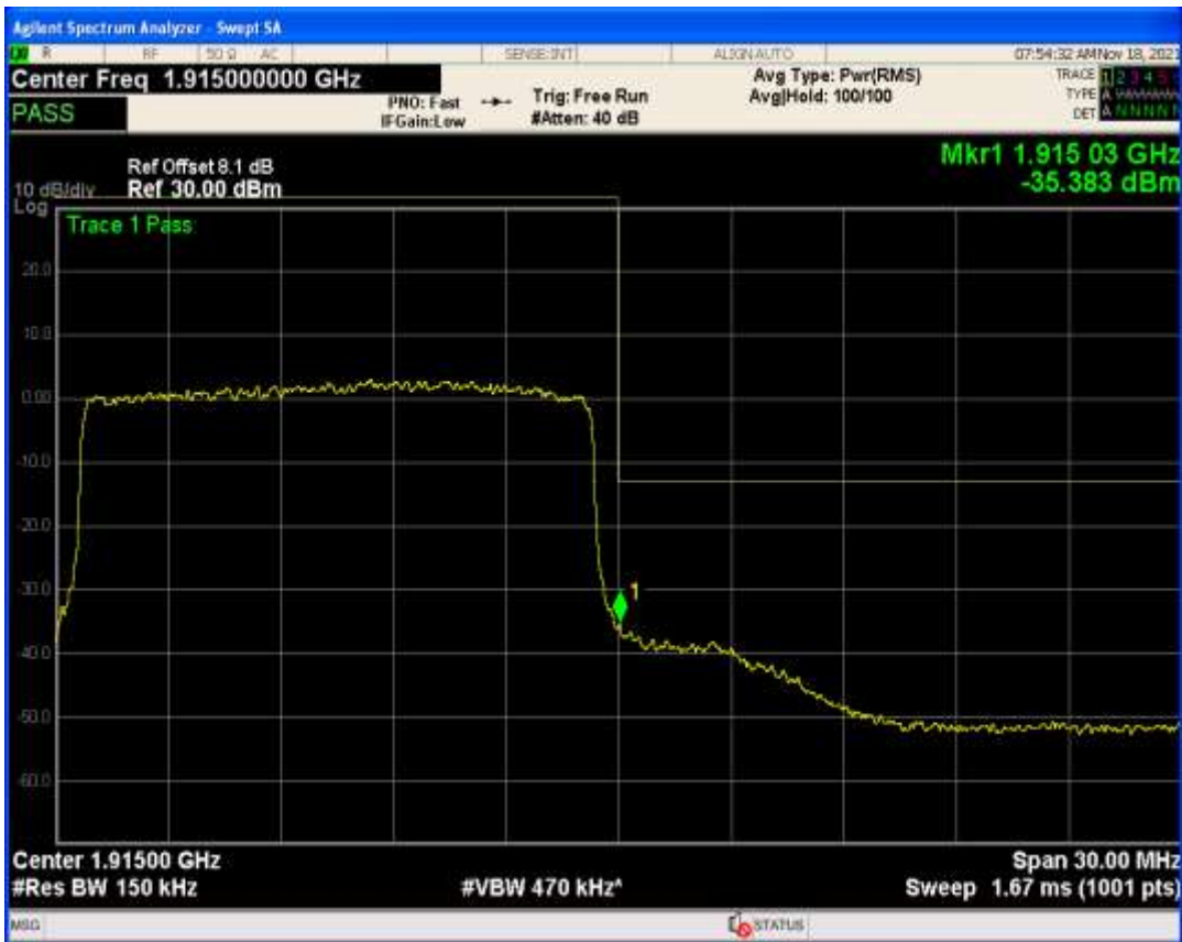
Band25 QAM16 BW=15MHz Channel=26115 RB Size=1 Position=#0
