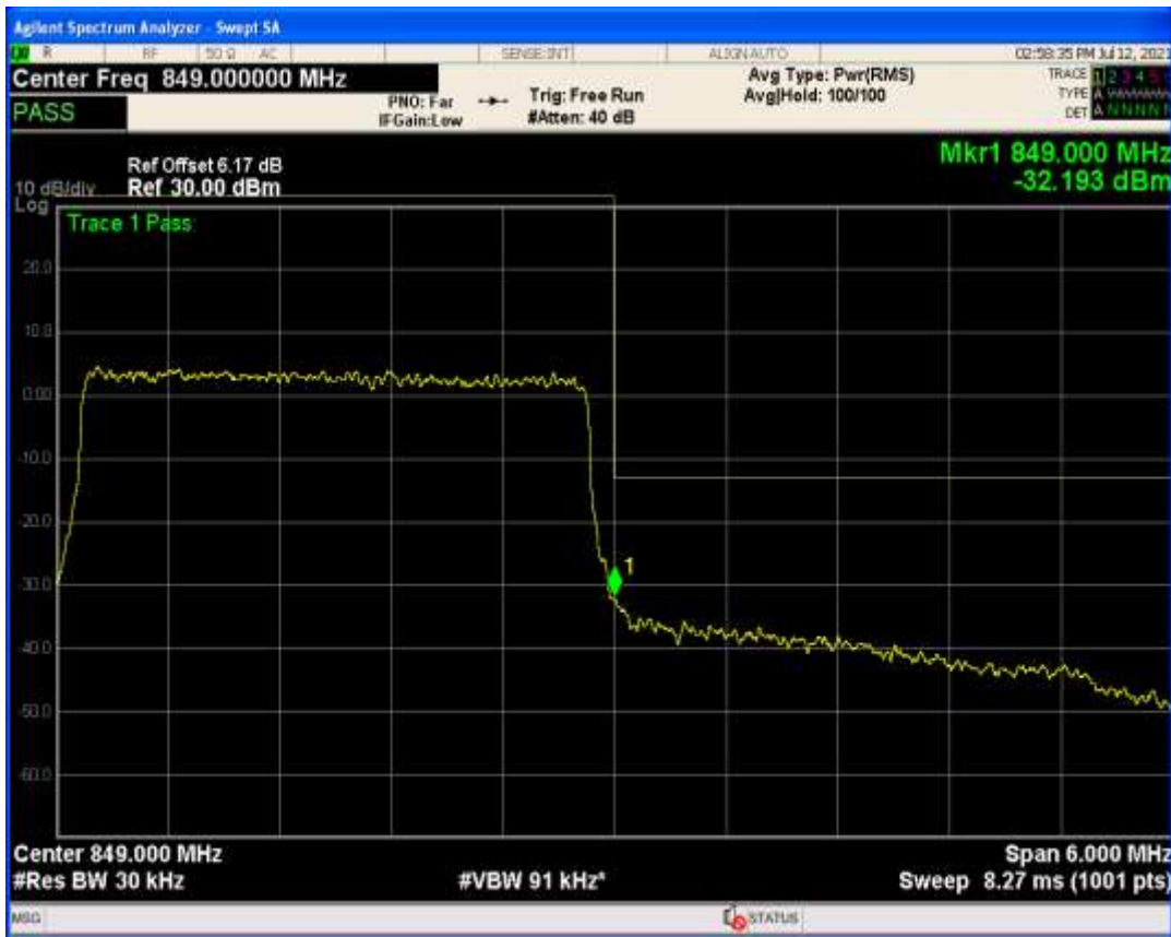
Band26b QPSK BW=5MHz Channel=27015 RB Size=1 Position=#Max
