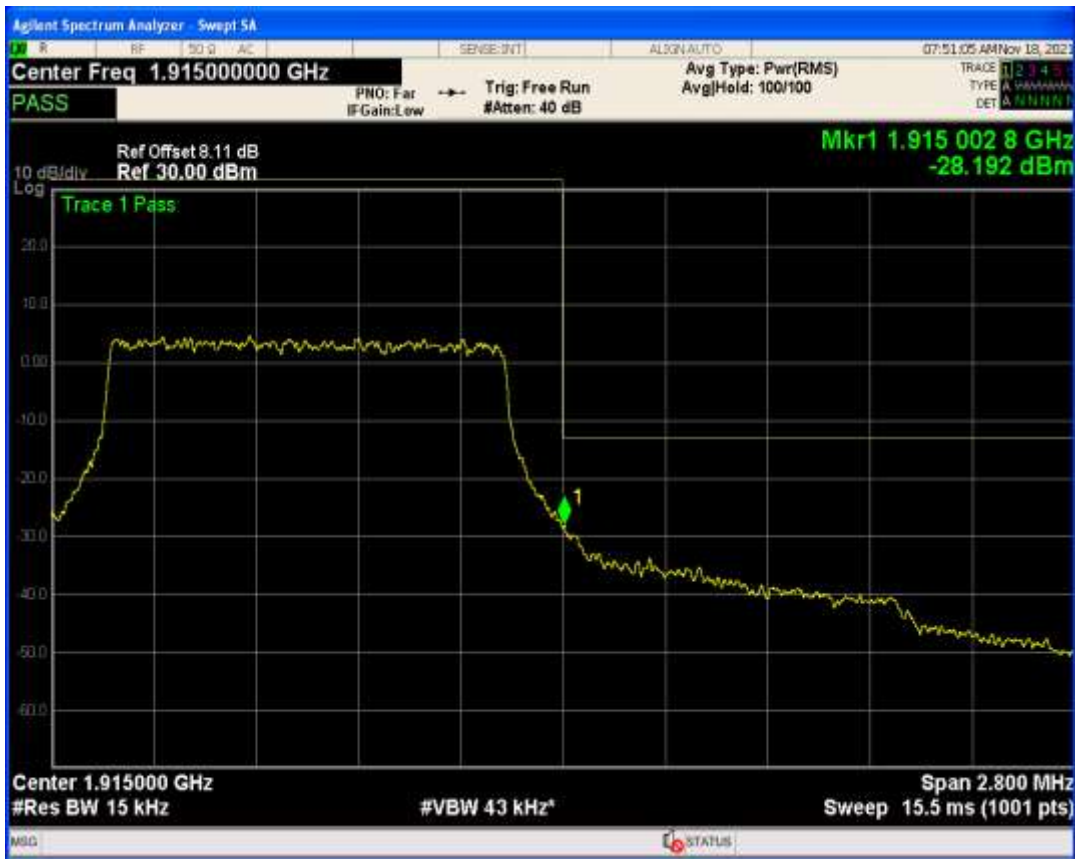
Band25 QPSK BW=1.4MHz Channel=26683 RB Size=1 Position=#Max
