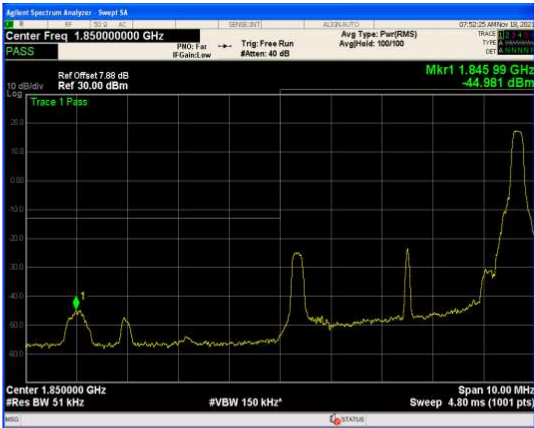
Band25 QPSK BW=5MHz Channel=26065 RB Size=1 Position=#0
