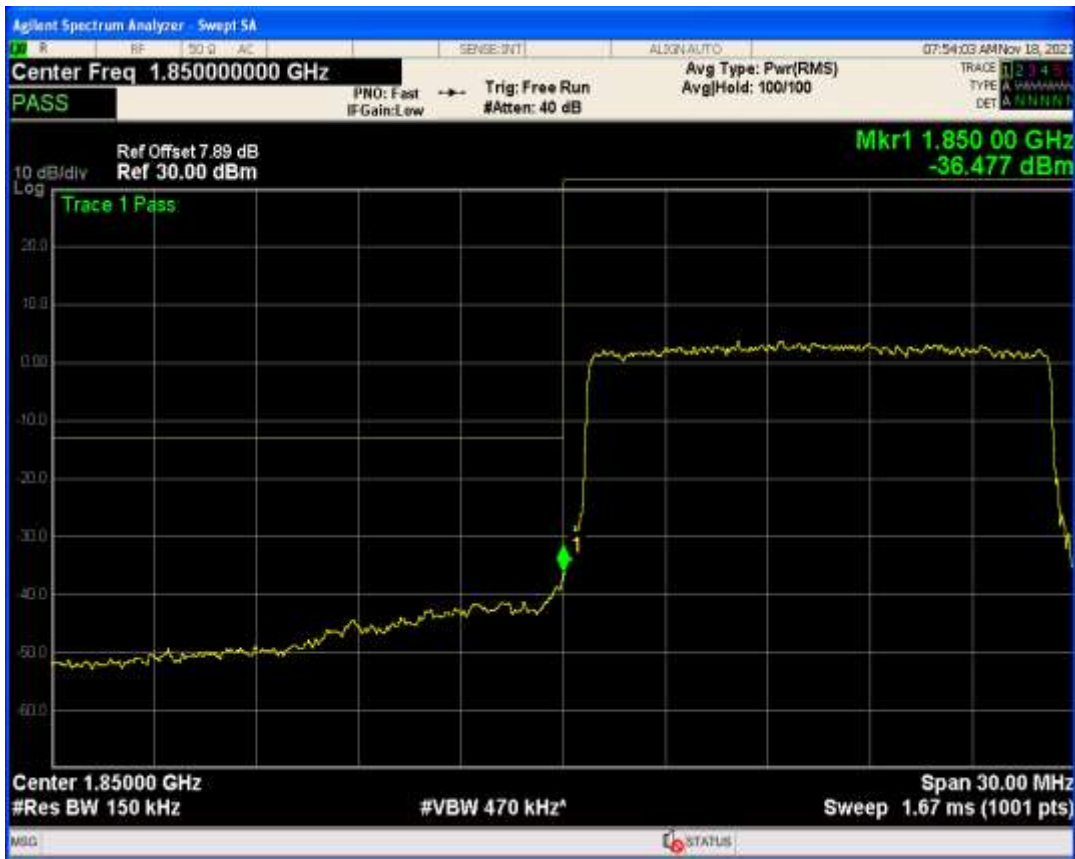
Band25 QPSK BW=15MHz Channel=26115 RB Size=1 Position=#Max
