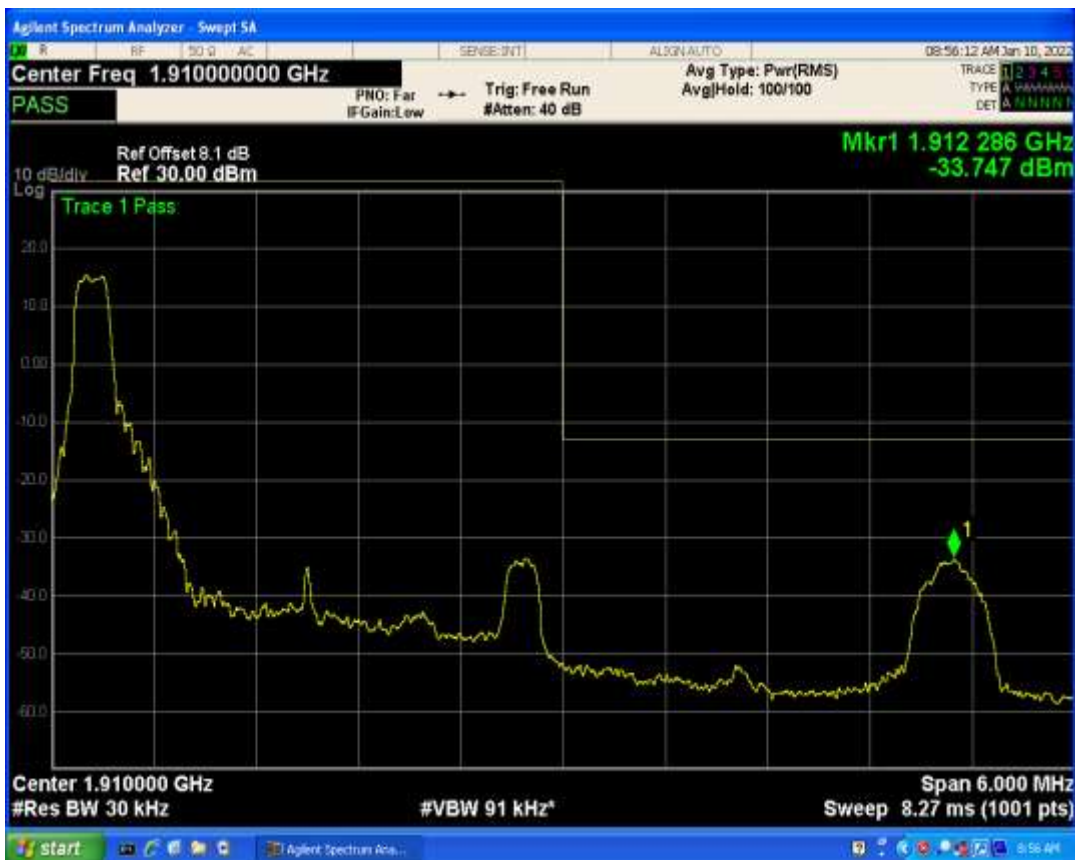
Band2 QPSK BW=3MHz Channel=19185 RB Size=15 Position=#0
