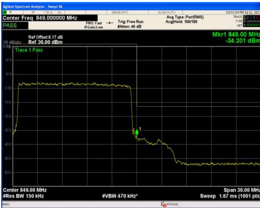
Band26b QPSK BW=15MHz Channel=26865 RB Size=75 Position=#0
