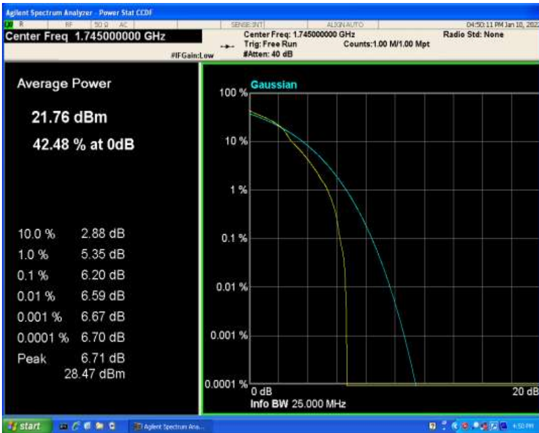
Band66 QAM16 BW=5MHz Channel=132322 RB Size=1 Position=#0
