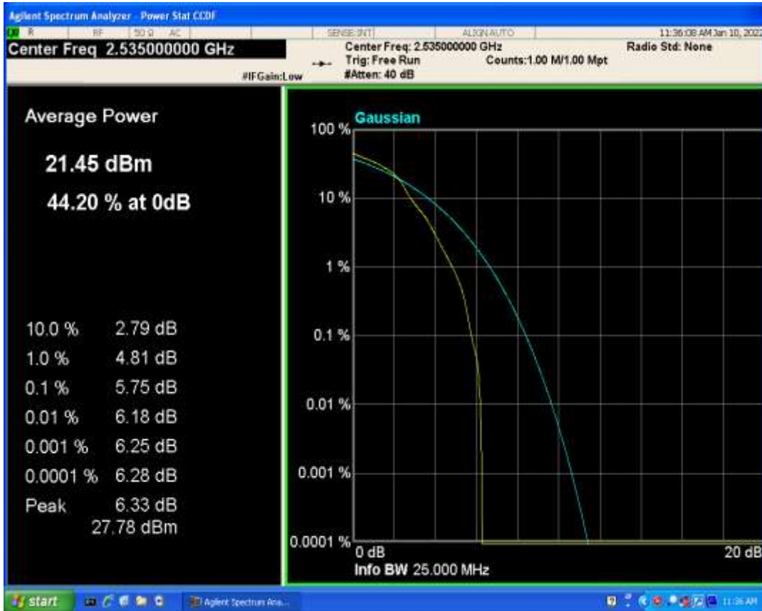
Band7 QAM16 BW=20MHz Channel=21100 RB Size=1 Position=#0
