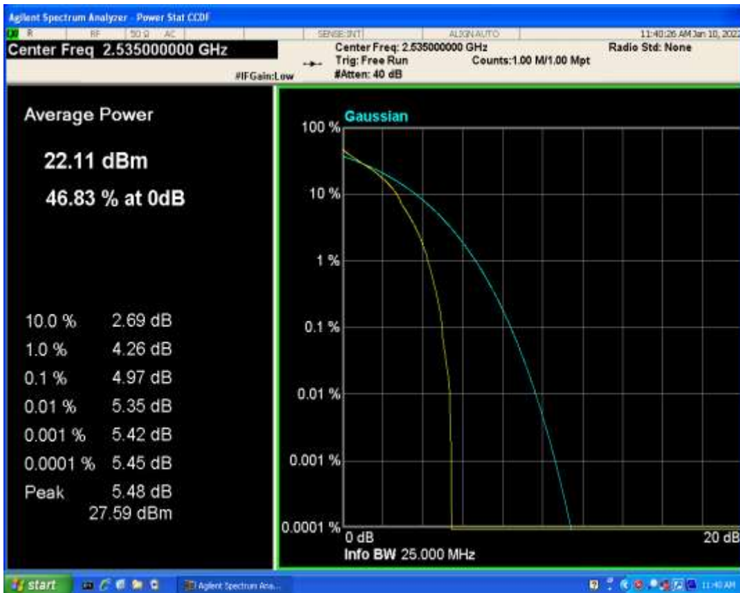
Band7 QPSK BW=15MHz Channel=21100 RB Size=1 Position=#0
