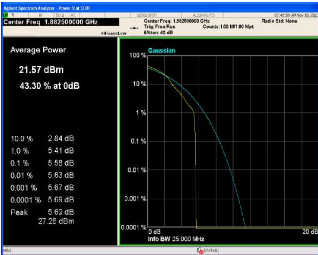
Band25 QAM16 BW=15MHz Channel=26365 RB Size=1 Position=#0
