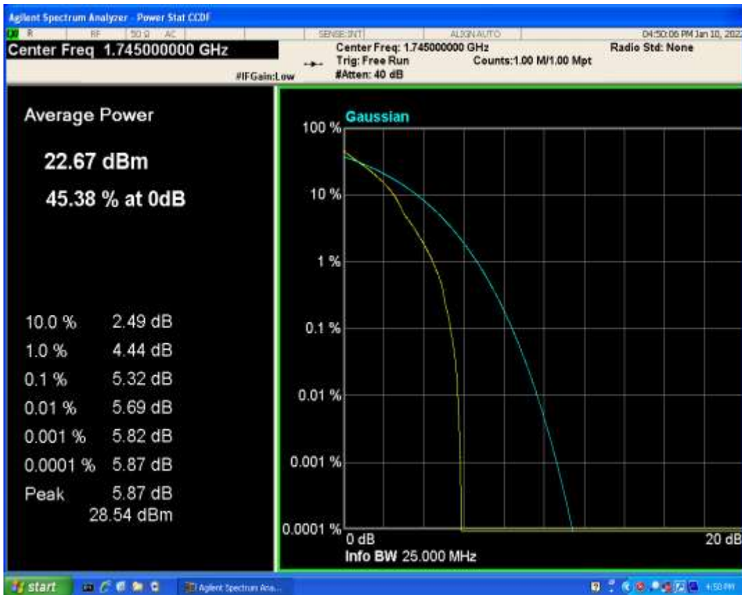
Band66 QPSK BW=10MHz Channel=132322 RB Size=1 Position=#0
