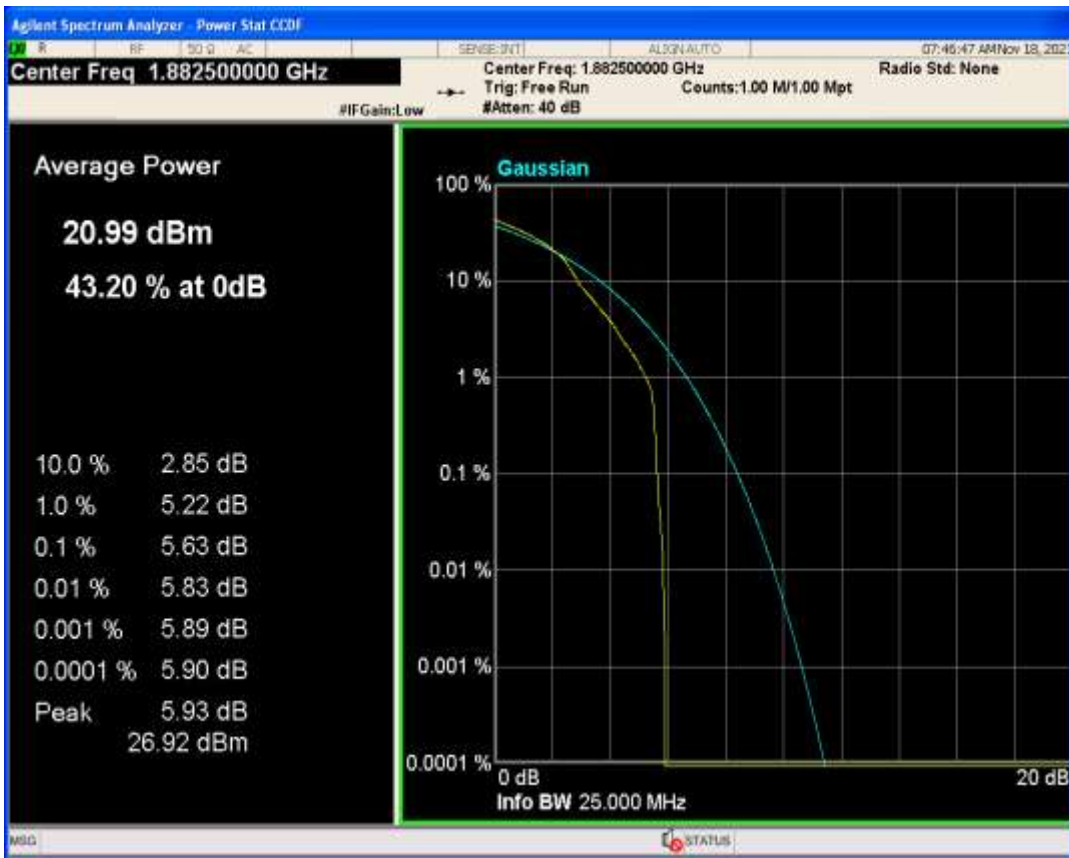
Band25 QAM16 BW=1.4MHz Channel=26365 RB Size=1 Position=#0
