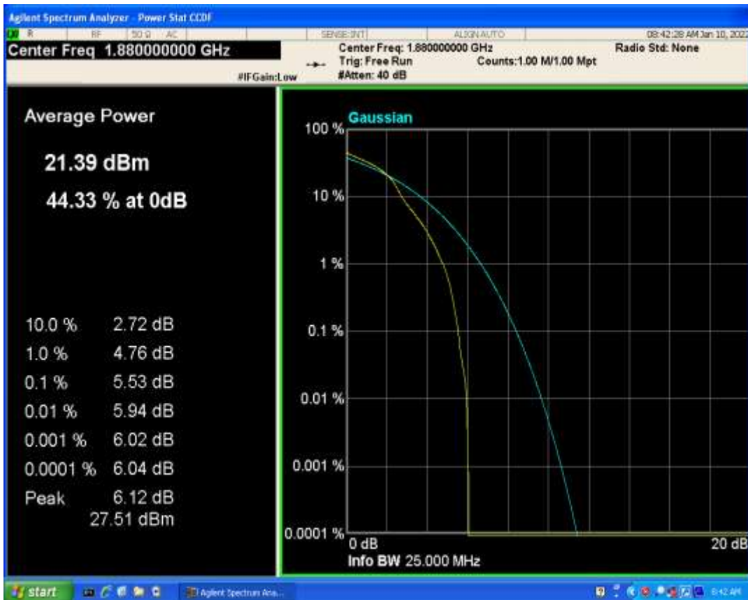
Band2 QAM16 BW=20MHz Channel=18900 RB Size=1 Position=#0
