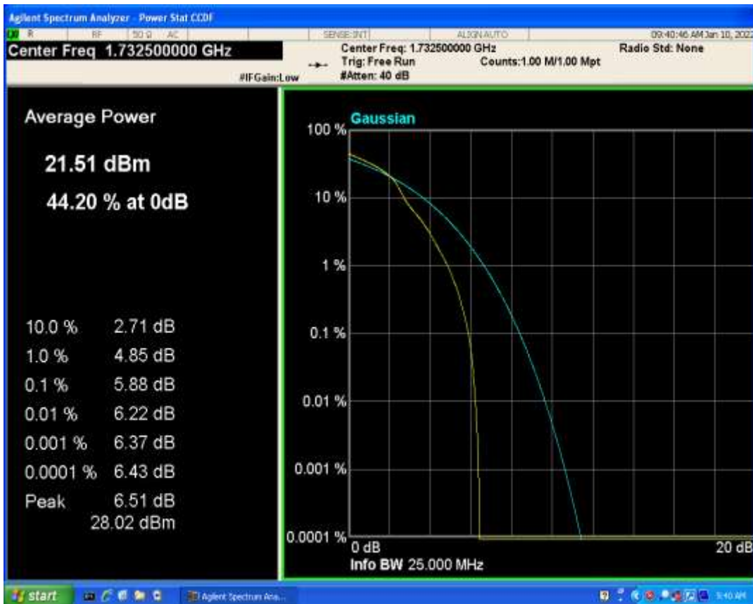
Band4 QPSK BW=5MHz Channel=20175 RB Size=1 Position=#0
