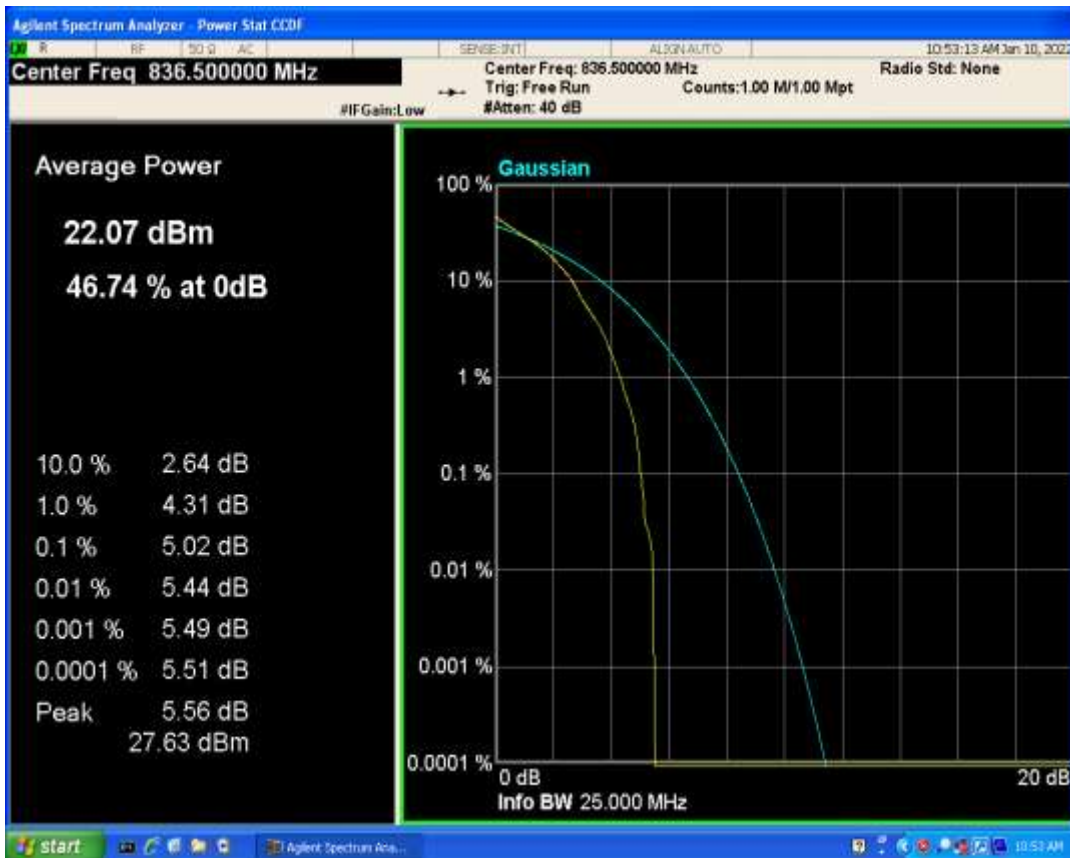
Band5 QAM16 BW=3MHz Channel=20525 RB Size=1 Position=#0
