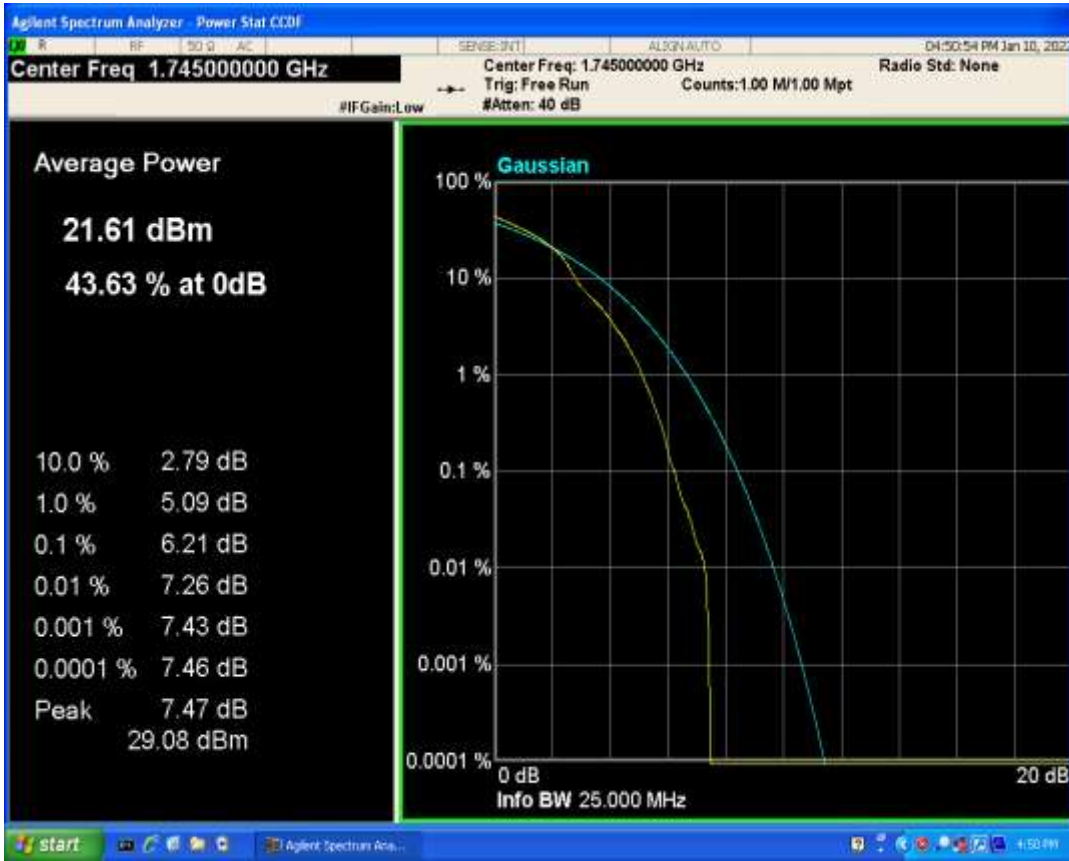
Band66 QAM16 BW=15MHz Channel=132322 RB Size=1 Position=#0
