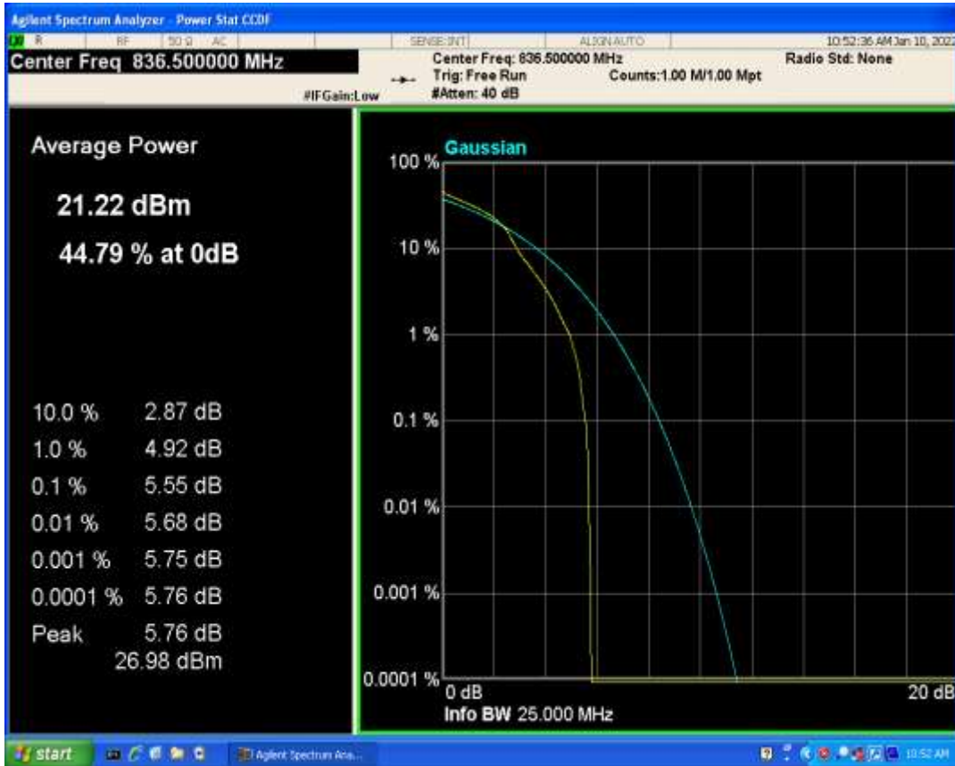
Band5 QAM16 BW=5MHz Channel=20525 RB Size=1 Position=#0
