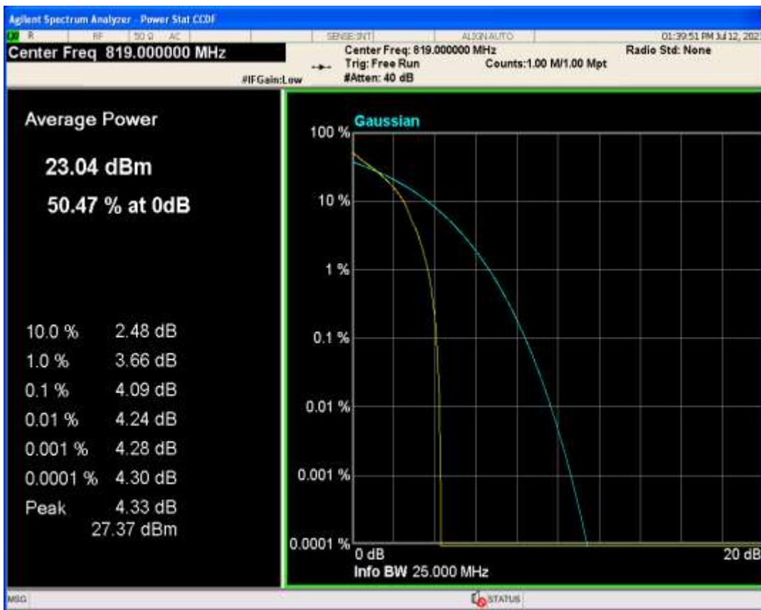
Band26a QPSK BW=10MHz Channel=26740 RB Size=1 Position=#0
