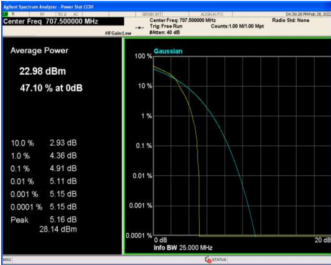
Band13 QPSK BW=10MHz Channel=23230 RB Size=1 Position=#0
