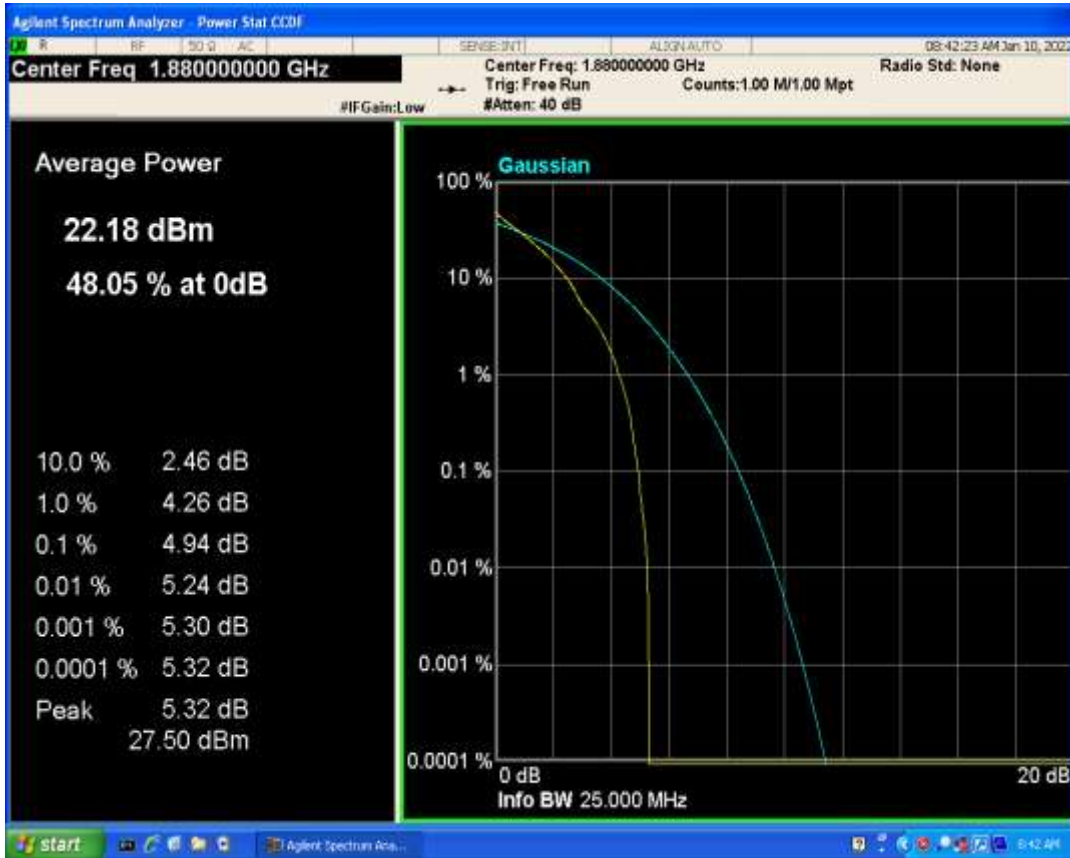
Band2 QPSK BW=5MHz Channel=18900 RB Size=1 Position=#0
