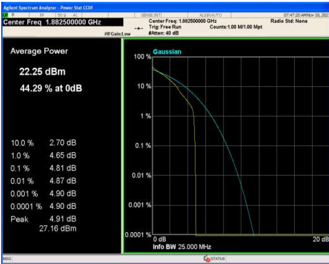
Band25 QPSK BW=3MHz Channel=26365 RB Size=1 Position=#0
