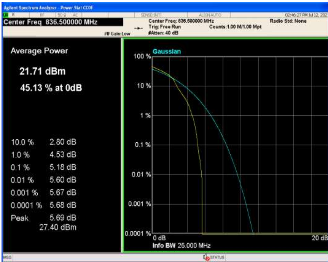
Band26b QAM16 BW=10MHz Channel=26915 RB Size=1 Position=#0
