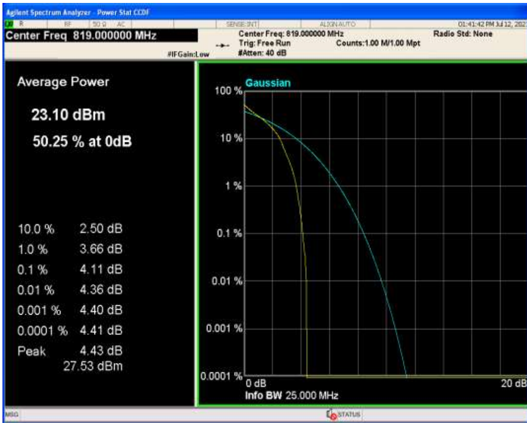
Band26a QPSK BW=3MHz Channel=26740 RB Size=1 Position=#0
