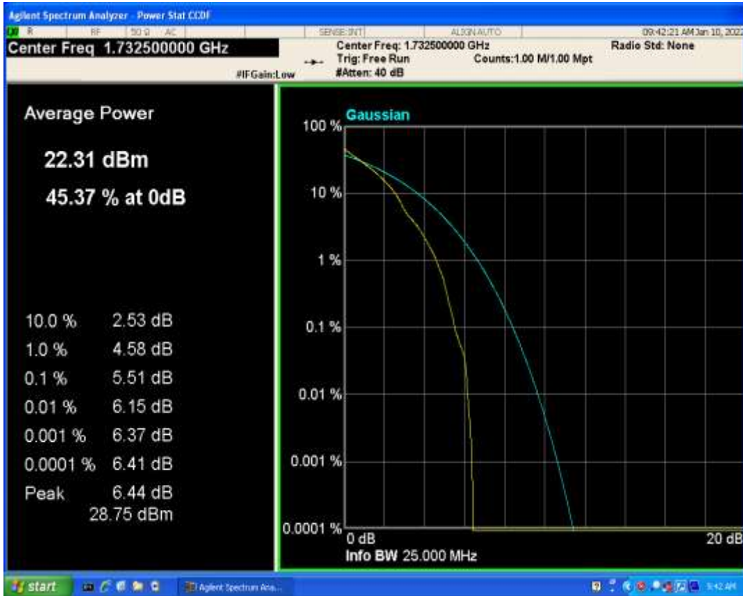
Band4 QPSK BW=10MHz Channel=20175 RB Size=1 Position=#0
