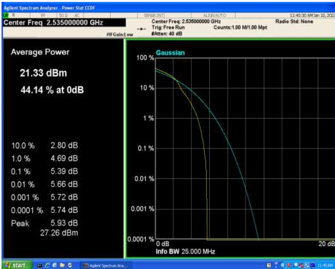
Band7 QAM16 BW=5MHz Channel=21100 RB Size=1 Position=#0
