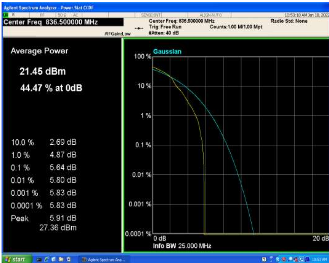
Band5 QPSK BW=1.4MHz Channel=20525 RB Size=1 Position=#0
