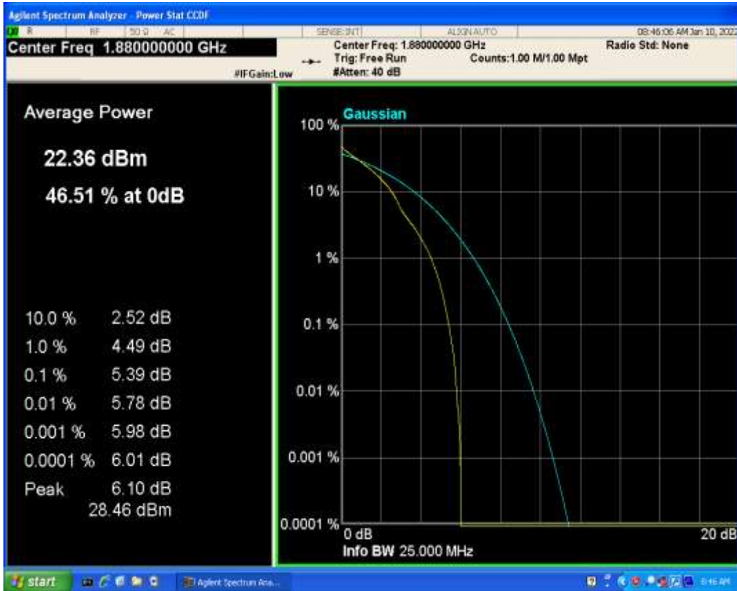
Band2 QPSK BW=20MHz Channel=18900 RB Size=1 Position=#0
