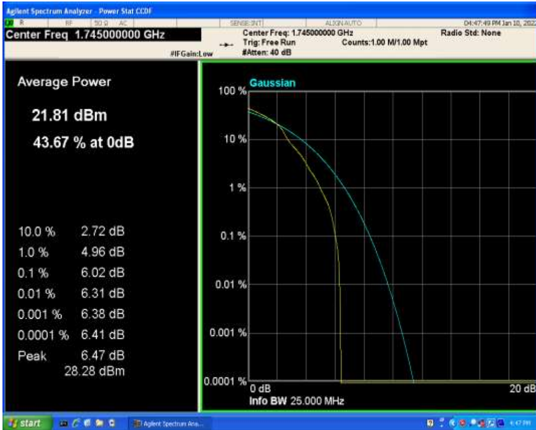
Band66 QAM16 BW=3MHz Channel=132322 RB Size=1 Position=#0
