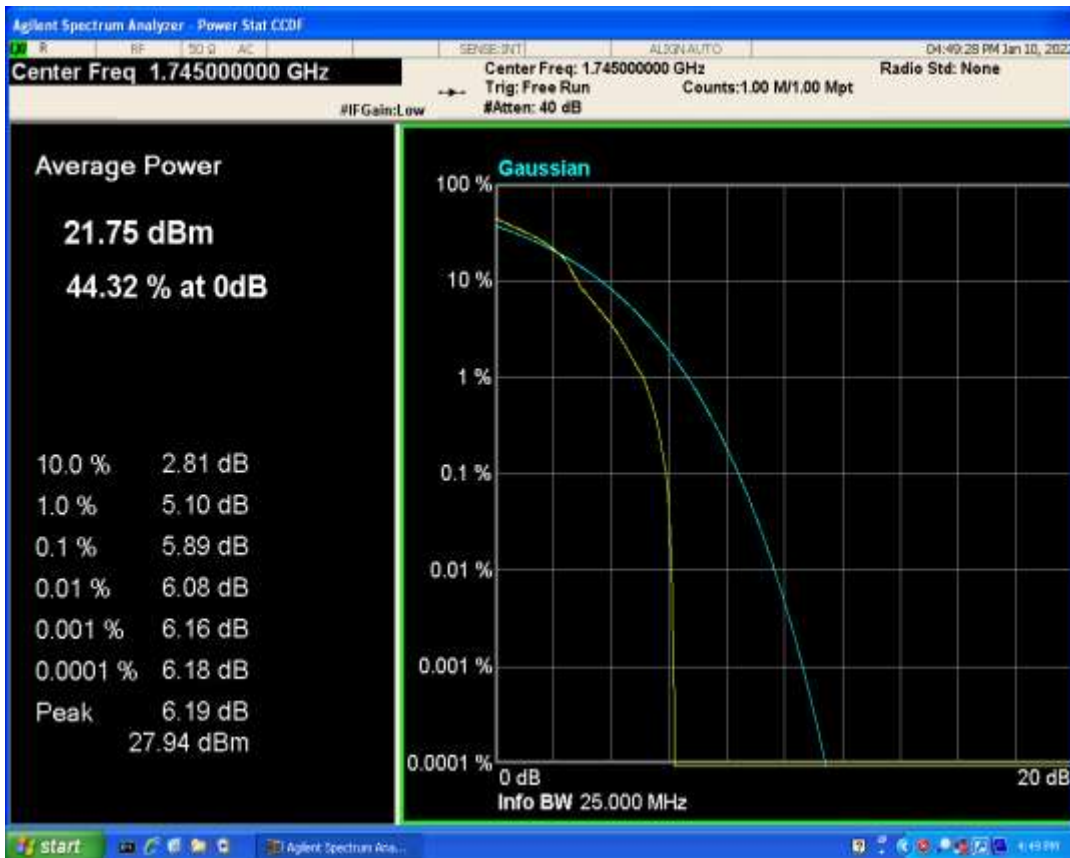
Band66 QAM16 BW=1.4MHz Channel=132322 RB Size=1 Position=#0
