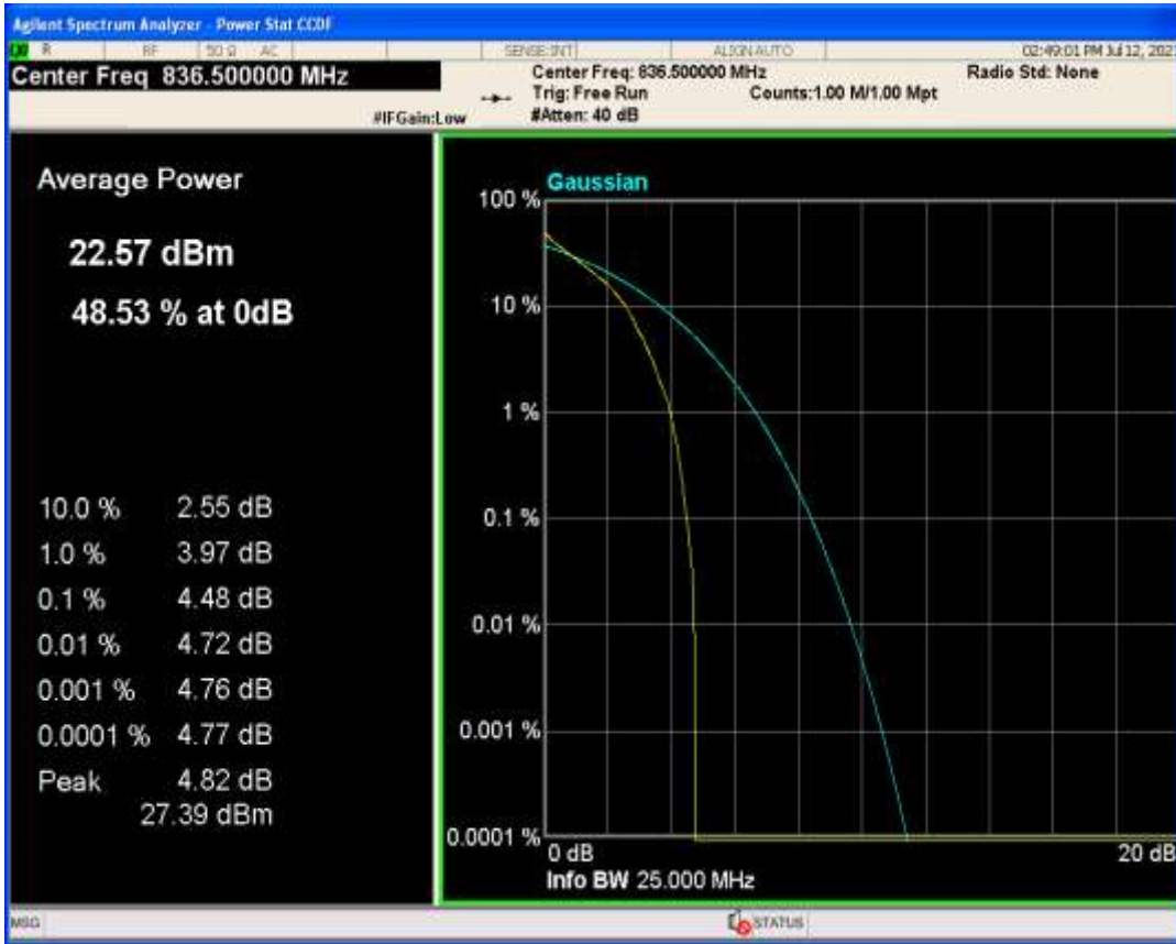
Band4 QAM16 BW=15MHz Channel=20175 RB Size=1 Position=#0
