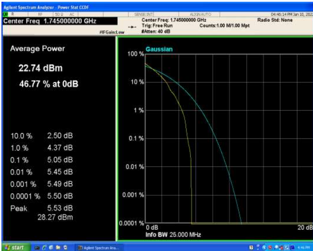
Band66 QAM16 BW=20MHz Channel=132322 RB Size=1 Position=#0
