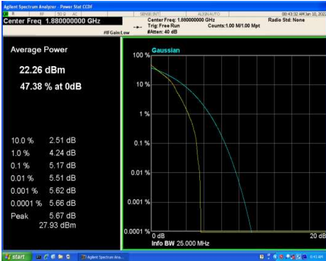
Band25 QAM16 BW=20MHz Channel=26365 RB Size=1 Position=#0
