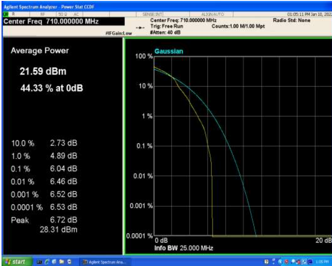
Band2 QAM16 BW=1.4MHz Channel=18900 RB Size=1 Position=#0
