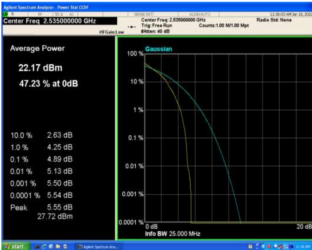
Band7 QPSK BW=5MHz Channel=21100 RB Size=1 Position=#0
