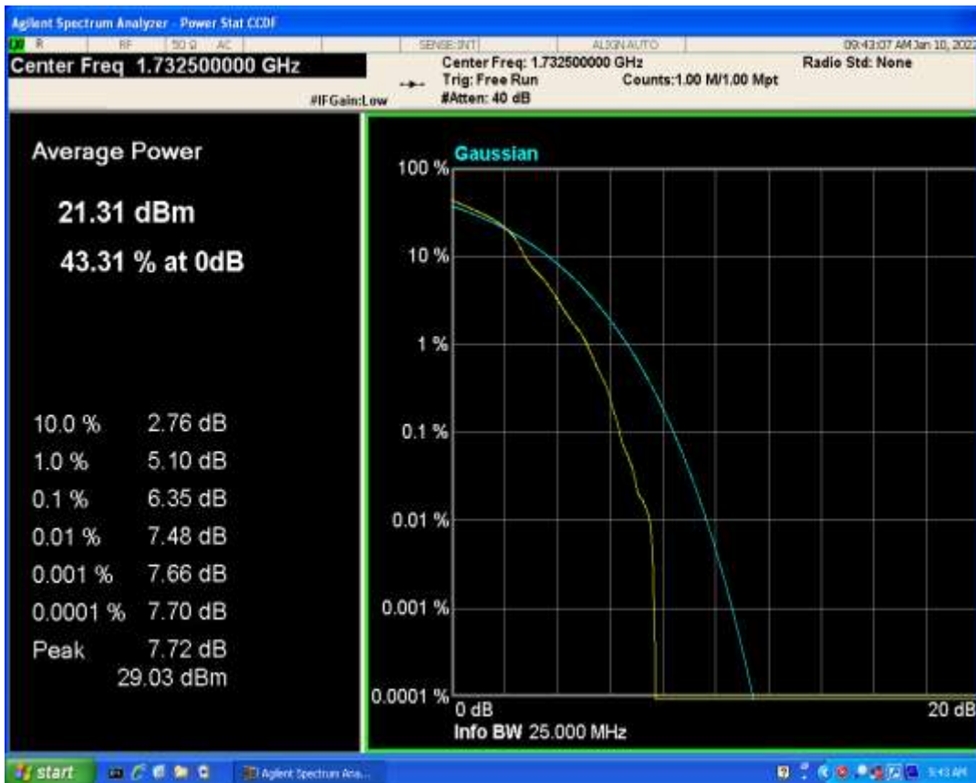
Band4 QPSK BW=1.4MHz Channel=20175 RB Size=1 Position=#0
