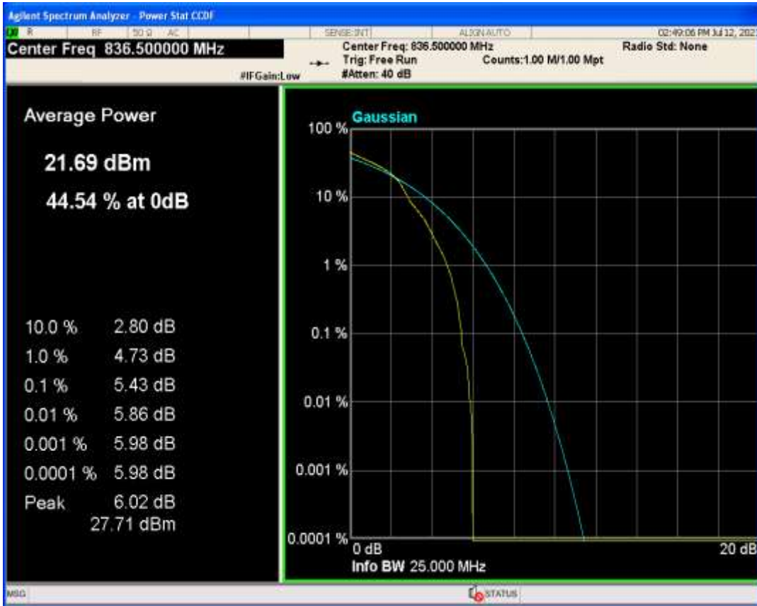
Band26b QPSK BW=15MHz Channel=26915 RB Size=1 Position=#0
