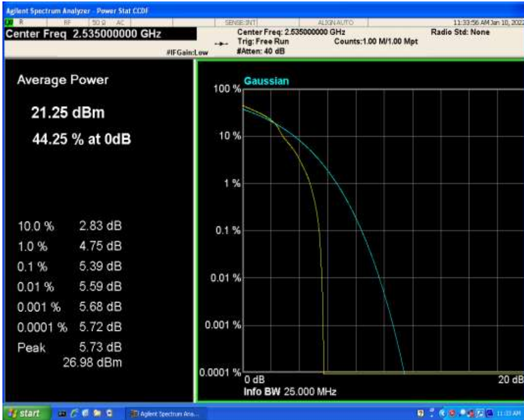
Band7 QPSK BW=10MHz Channel=21100 RB Size=1 Position=#0
