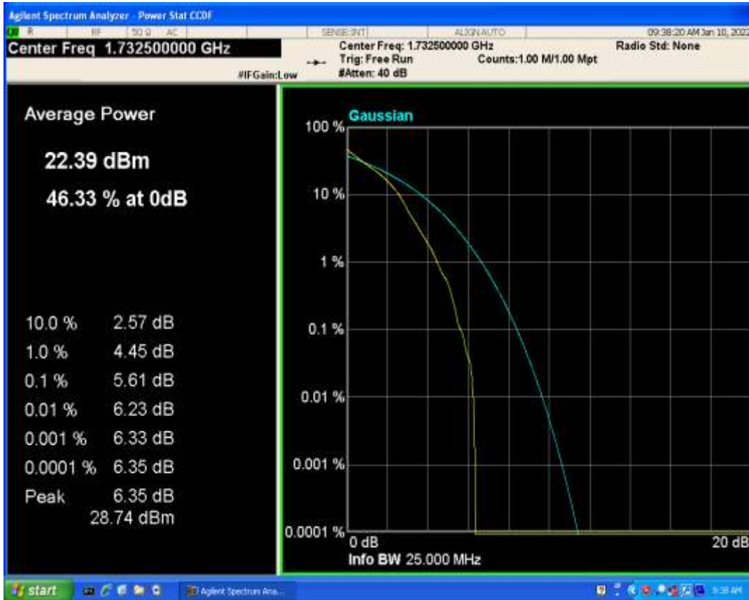
Band4 QAM16 BW=5MHz Channel=20175 RB Size=1 Position=#0
