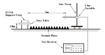
The radiated emission tests were performed at the 3 meters distance in chamber, using the setup accordance with the ANSI C63.4-2014. The specification used was the FCC Part 15.109 Class B limits.
