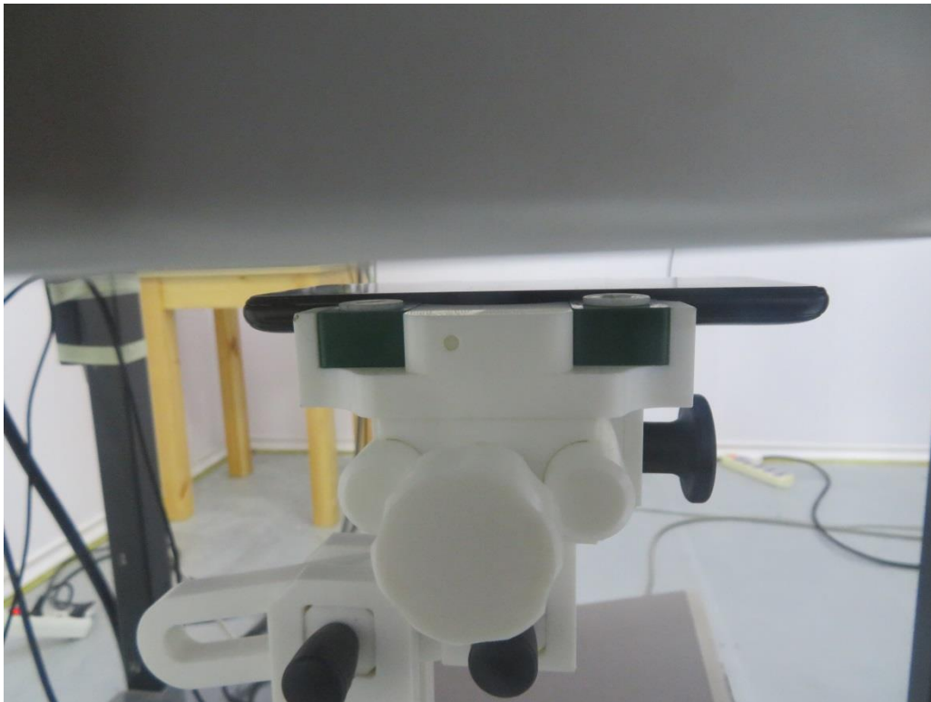
10mm body-worn Front Side Setup Photo (hotspot)
