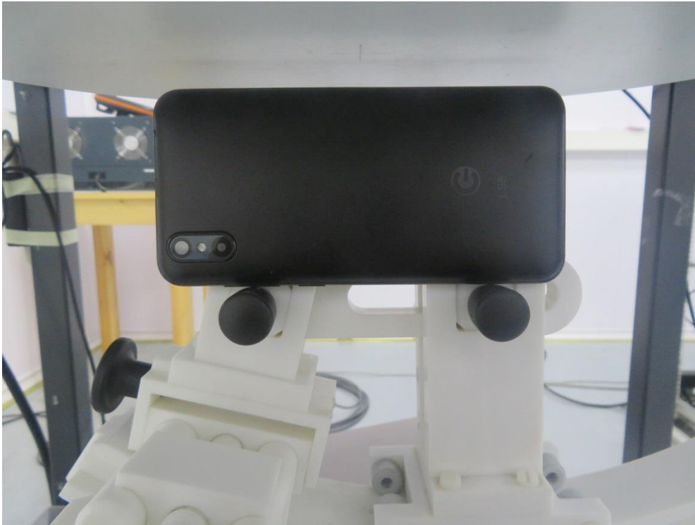
10mm body-worn Left Side Setup Photo (hotspot)
