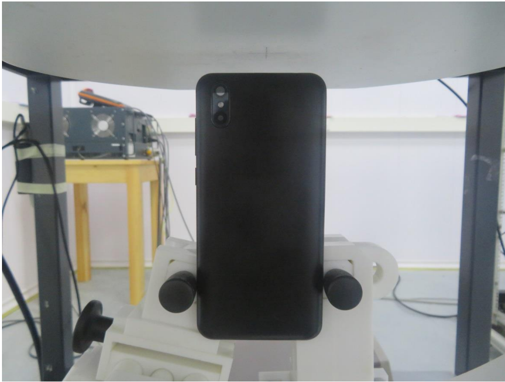
10mm body-worn Bottom Side Setup Photo (hotspot)
