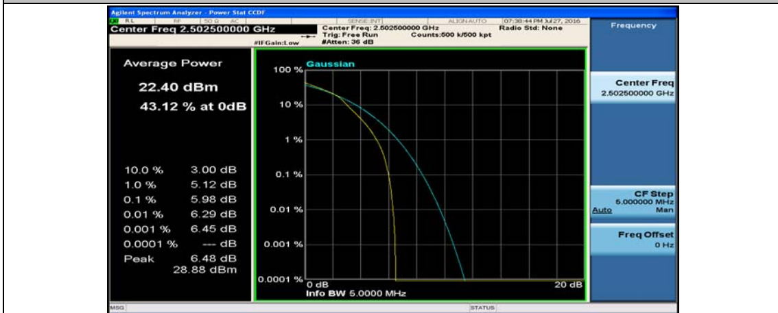
(Channel Bandwidth: 5 MHz)_LCH_16QAM_25RB#0
