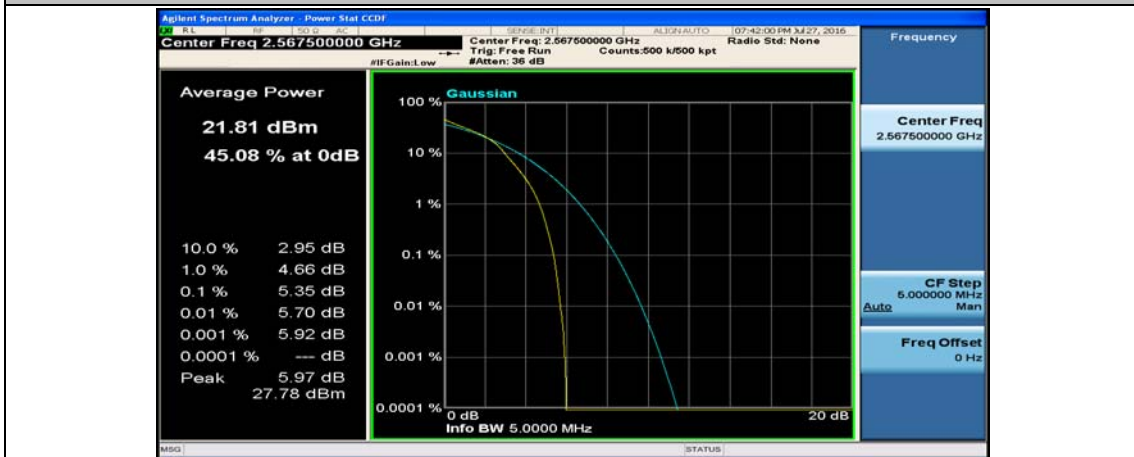
(Channel Bandwidth: 5 MHz)_HCH_16QAM_25RB#0
