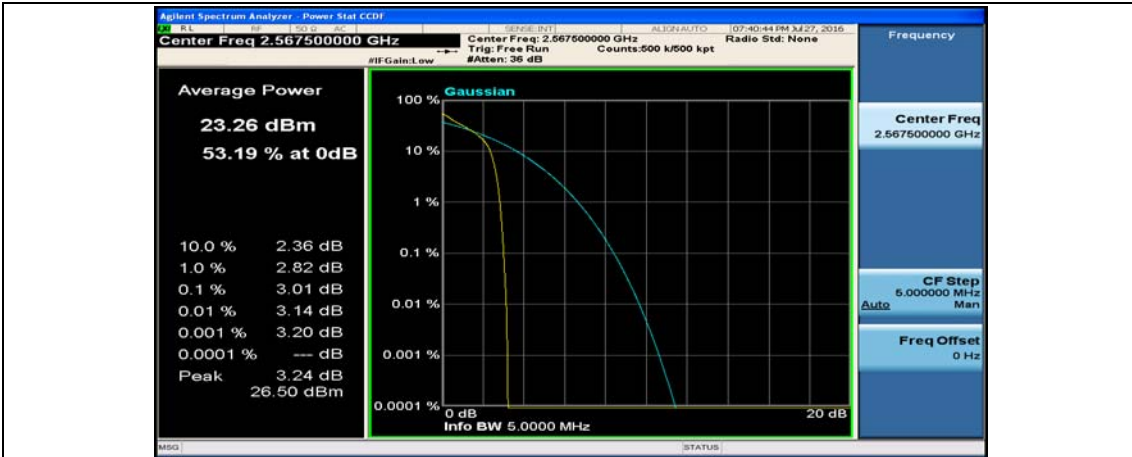
(Channel Bandwidth: 5 MHz)_HCH_QPSK_1RB#24
