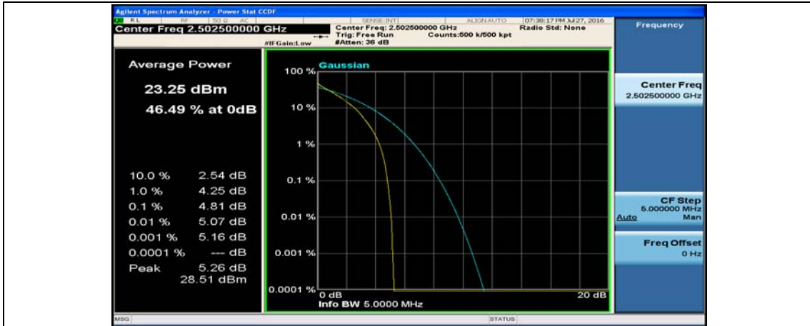
(Channel Bandwidth: 5 MHz)_LCH_QPSK_12RB#6
