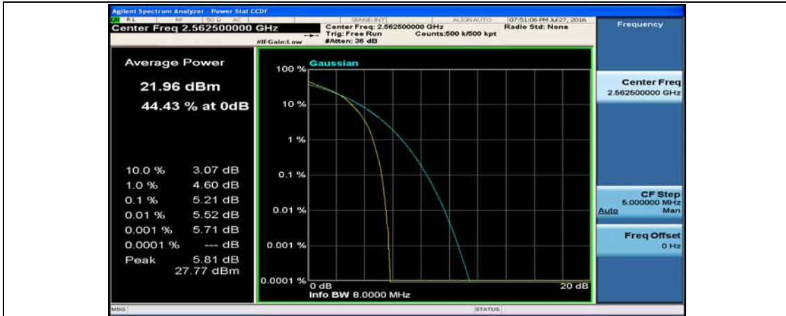
(Channel Bandwidth:15 MHz)_HCH_16QAM_37RB#38
