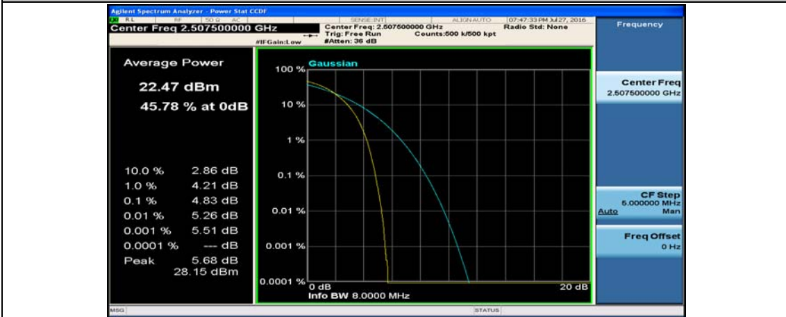
(Channel Bandwidth:15 MHz)_LCH_QPSK_75RB#0
