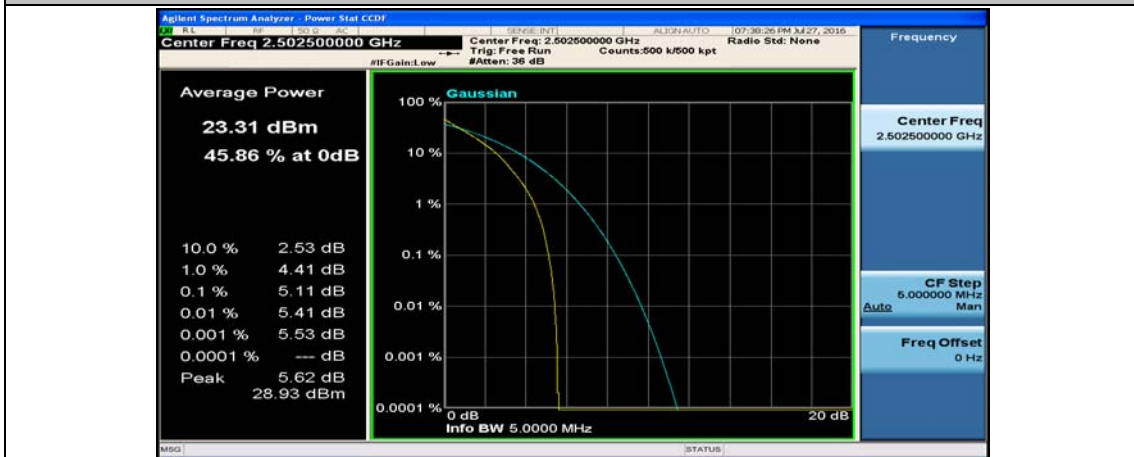
(Channel Bandwidth: 5 MHz)_LCH_QPSK_25RB#0
