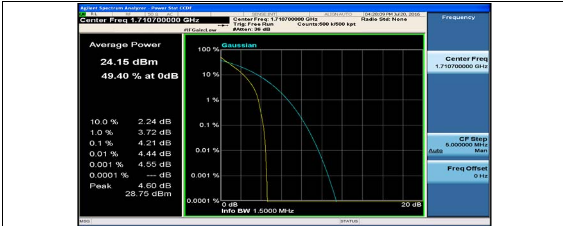
(Channel Bandwidth: 1.4 MHz)_LCH_QPSK_3RB#2
