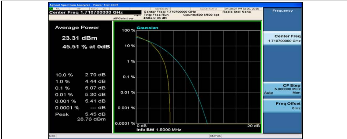
(Channel Bandwidth: 1.4 MHz)_LCH_16QAM_3RB#2
