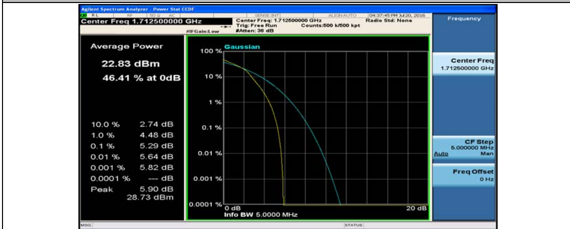
(Channel Bandwidth: 5 MHz)_LCH_16QAM_25RB#0
