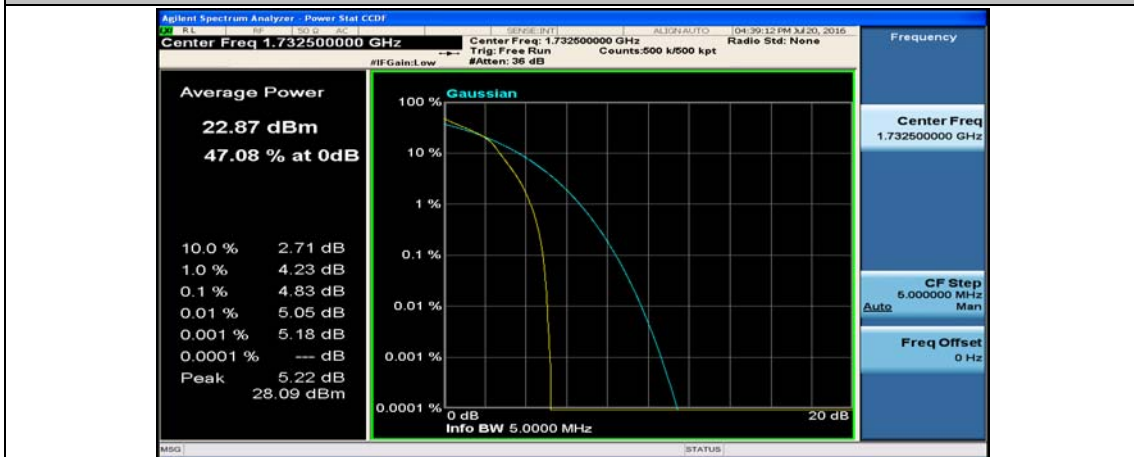
(Channel Bandwidth: 5 MHz)_MCH_16QAM_12RB#13
