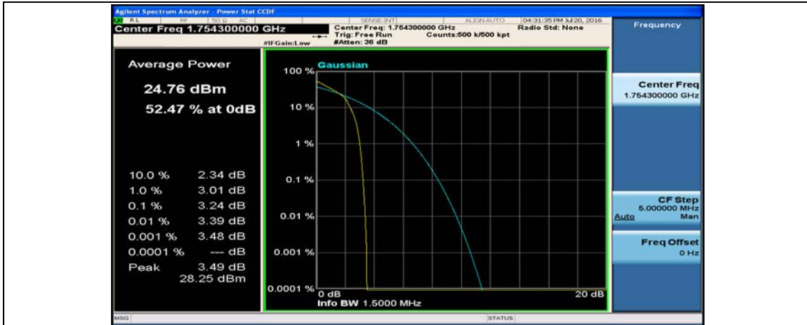
(Channel Bandwidth: 1.4 MHz)_HCH_16QAM_3RB#3
