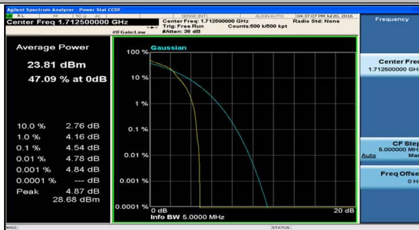
(Channel Bandwidth: 5 MHz)_LCH_16QAM_12RB#0
