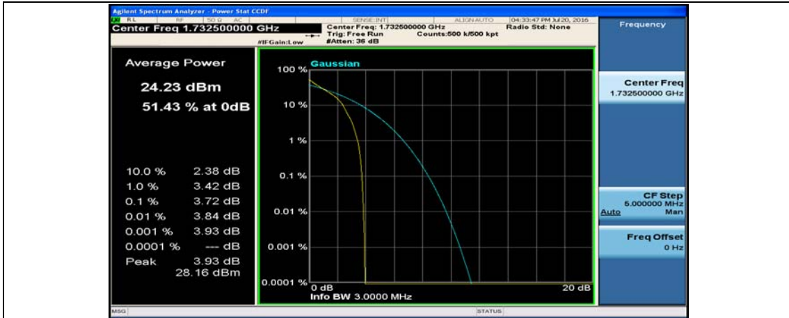
(Channel Bandwidth: 3 MHz)_MCH_QPSK_8RB#0
