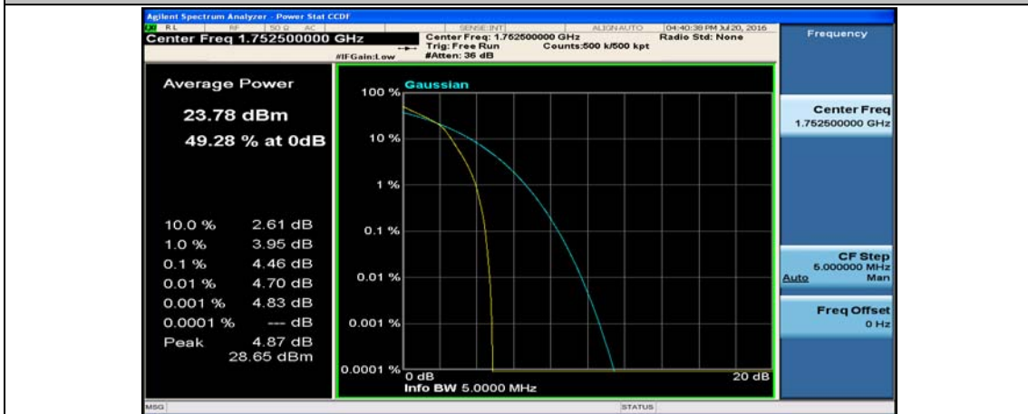
(Channel Bandwidth: 5 MHz)_HCH_16QAM_12RB#6
