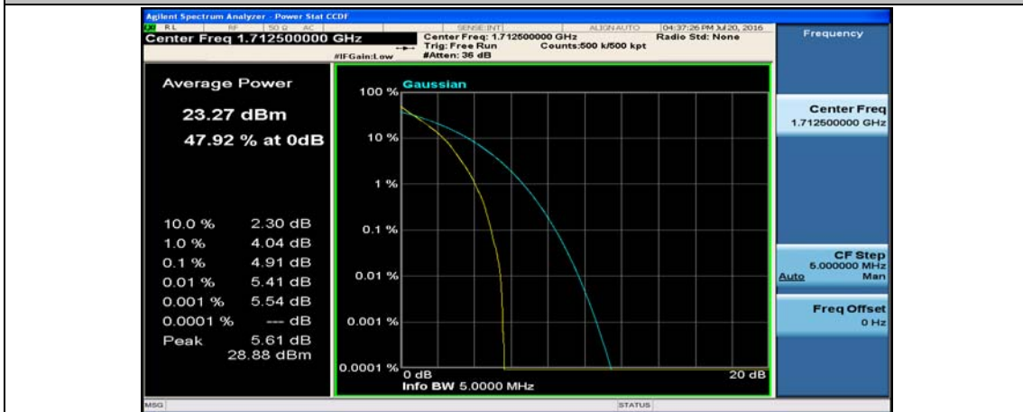
(Channel Bandwidth: 5 MHz)_LCH_QPSK_25RB#0
