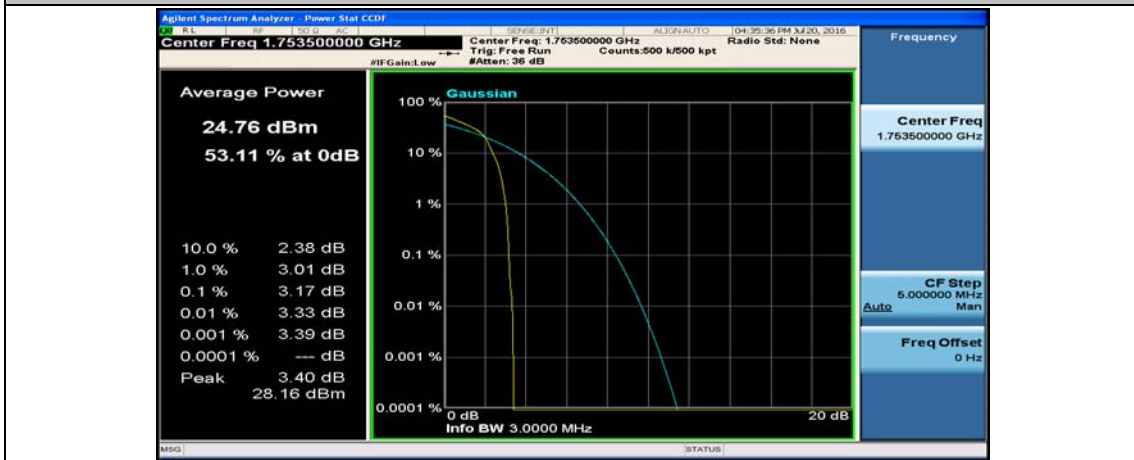
(Channel Bandwidth: 3 MHz)_HCH_16QAM_8RB#0
