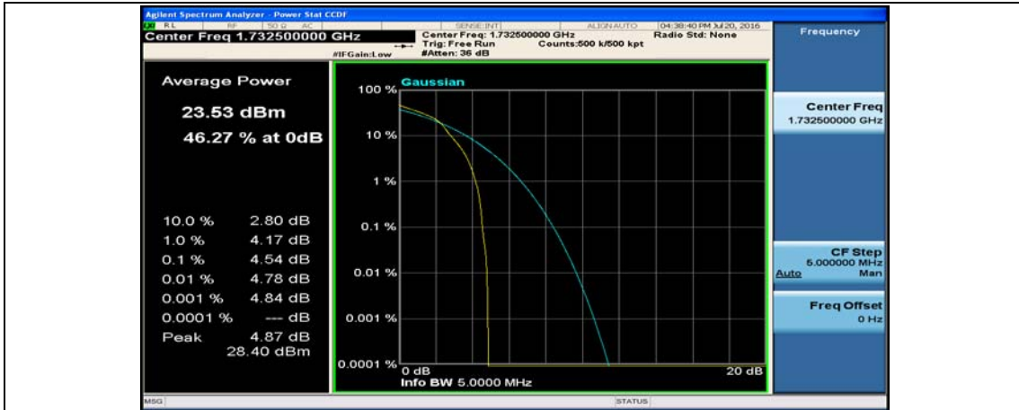
(Channel Bandwidth: 5 MHz)_MCH_16QAM_12RB#0
