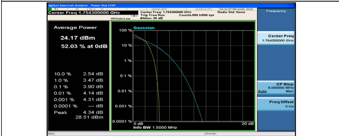
(Channel Bandwidth: 1.4 MHz)_HCH_16QAM_6RB#0
