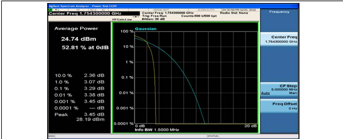
(Channel Bandwidth: 1.4 MHz)_HCH_16QAM_1RB#5
