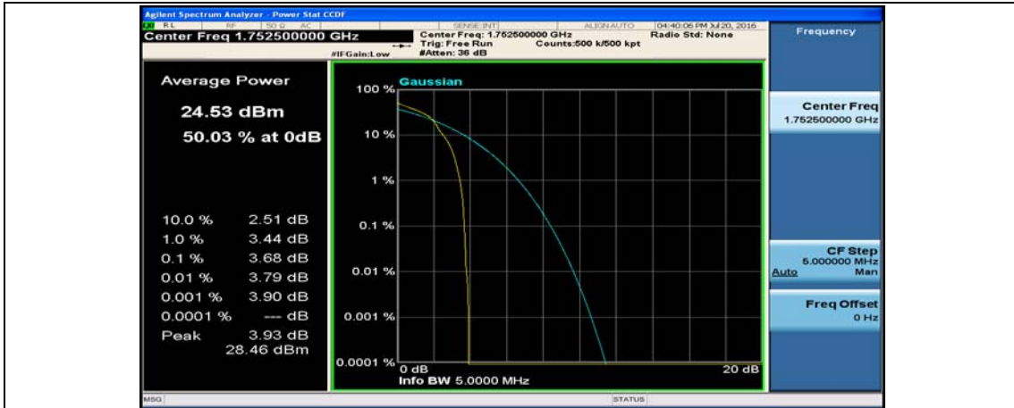
(Channel Bandwidth: 5 MHz)_HCH_16QAM_1RB#24
