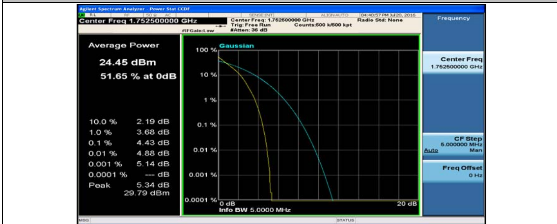
(Channel Bandwidth: 5 MHz)_HCH_QPSK_25RB#0
