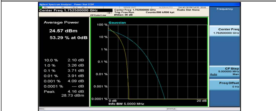
(Channel Bandwidth: 5 MHz)_HCH_QPSK_25RB#0
