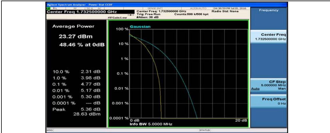
(Channel Bandwidth: 5 MHz)_MCH_QPSK_25RB#0
