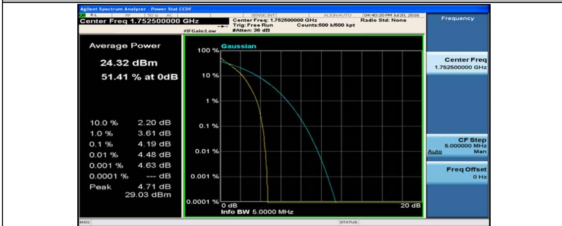
(Channel Bandwidth: 5 MHz)_HCH_QPSK_12RB#6
