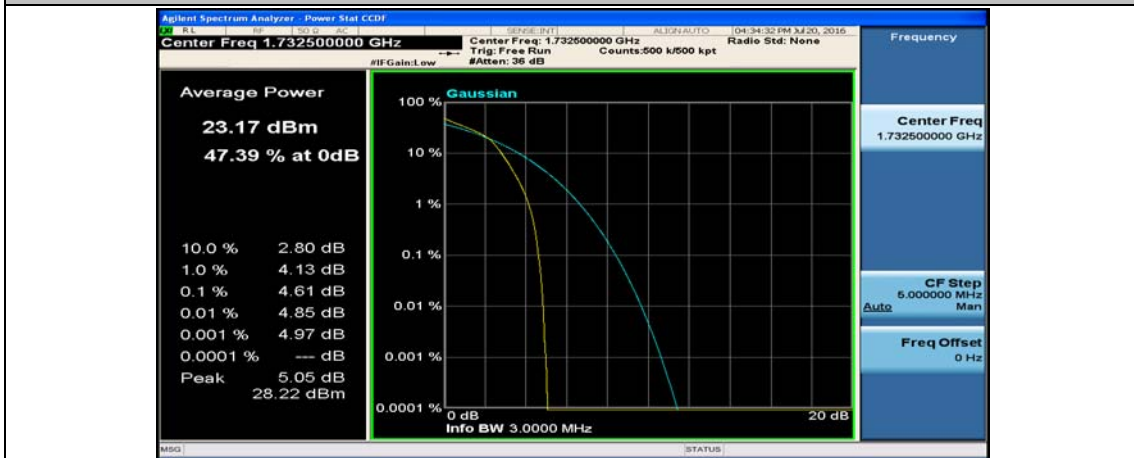
(Channel Bandwidth: 3 MHz)_MCH_16QAM_8RB#4
