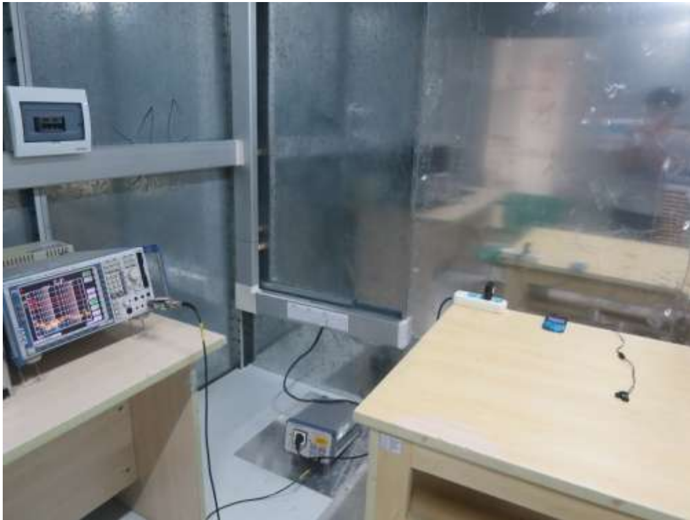
FCC RADIATED EMISSION TEST SETUP
