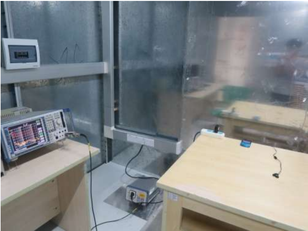
FCC RADIATED EMISSION TEST SETUP
