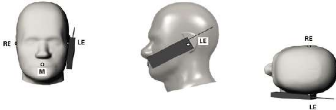
Fig. 11.3 Illustration for Cheek Position
