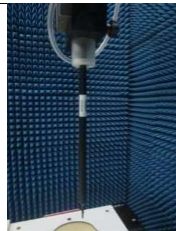
Fig. 8.2 Photo of E-Field Probe
