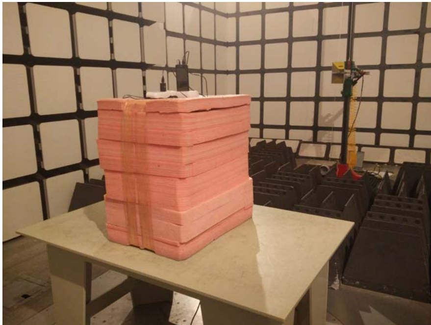
Radiated Emissions View (Above 1 GHz)
