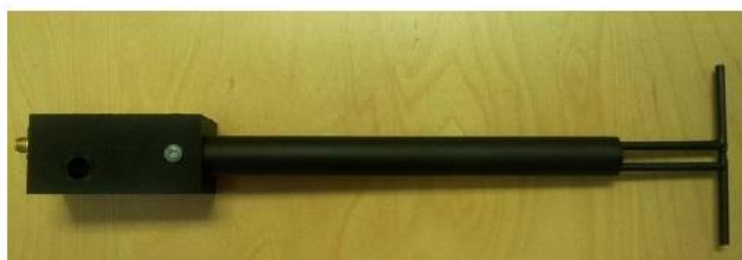
Figure 1 – MVG COMOSAR Validation Dipole
