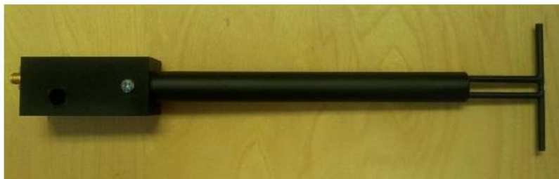
Figure 1 – MVG COMOSAR Validation Dipole
