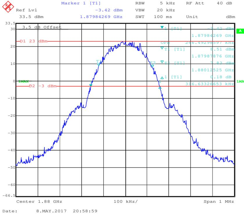
**99% Occupied Bandwidth & 26 dB Emissions Bandwidth for RMC (BPSK) Mode**
