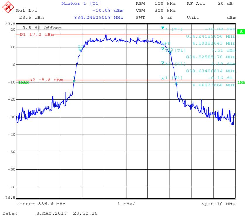
**99% Occupied Bandwidth & 26 dB Emissions Bandwidth for HSDPA (16QAM) Mode**
