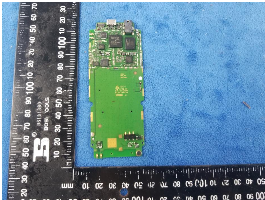
Mainboard without Shielding - Front View
