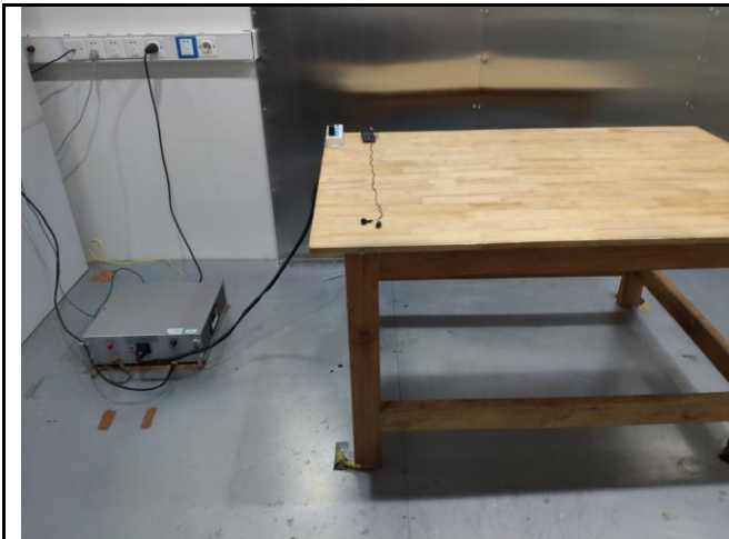
Conducted Emissions Test Setup Front View
