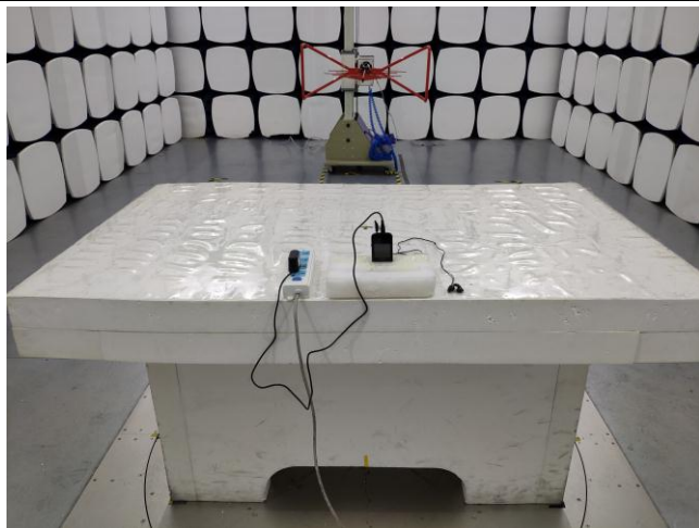
Radiated Spurious Emissions Test Setup Below 1GHz
