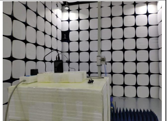
Radiated Spurious Emissions Test Setup Above 1GHz
