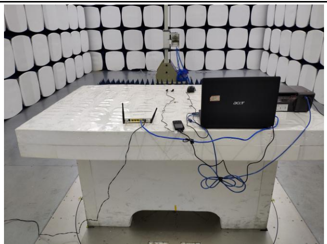
Radiated Emissions Test Setup Above 1GHz
