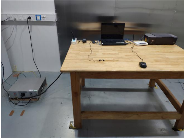
Conducted Emissions Test Setup – Front View
