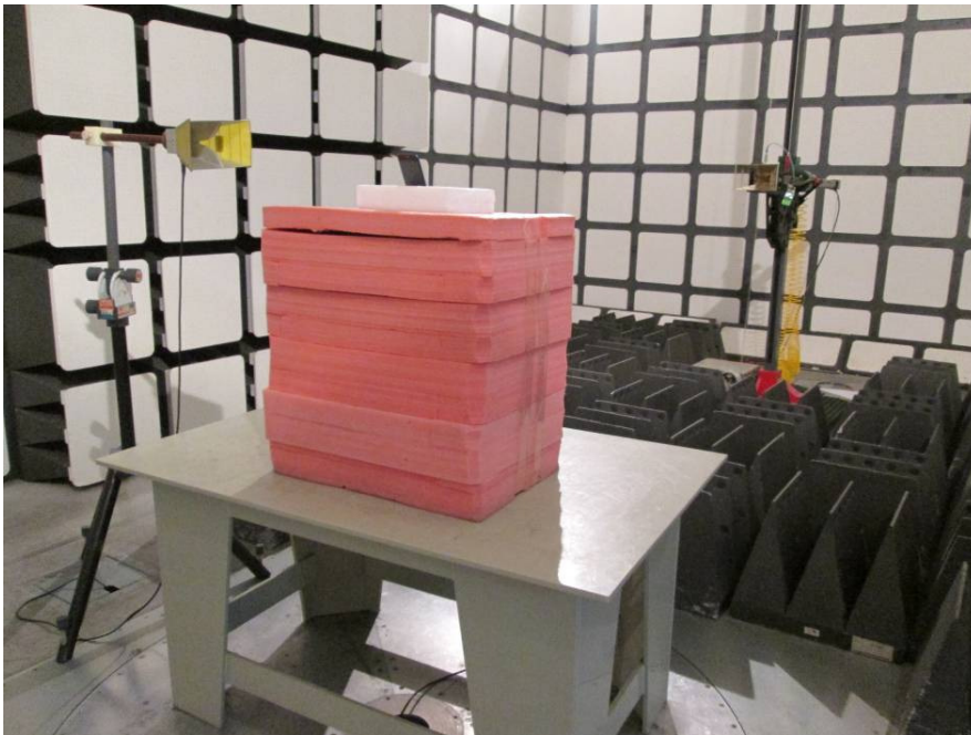
Radiated Emissions Test View (Above 1 GHz)
