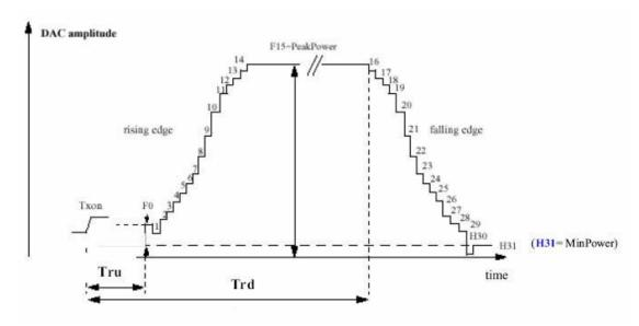
$Tru = TxTRUDefault + \Delta TRU_P + \Delta TRU_T$  $Trd = TxTRD_NBDefault + \Delta TRD_P \text{ (for a normal burst).}$  $Trd = TxTRD_ABDefault + \Delta TRD_P \text{ (for an access burst).}$ 3 Parameters
