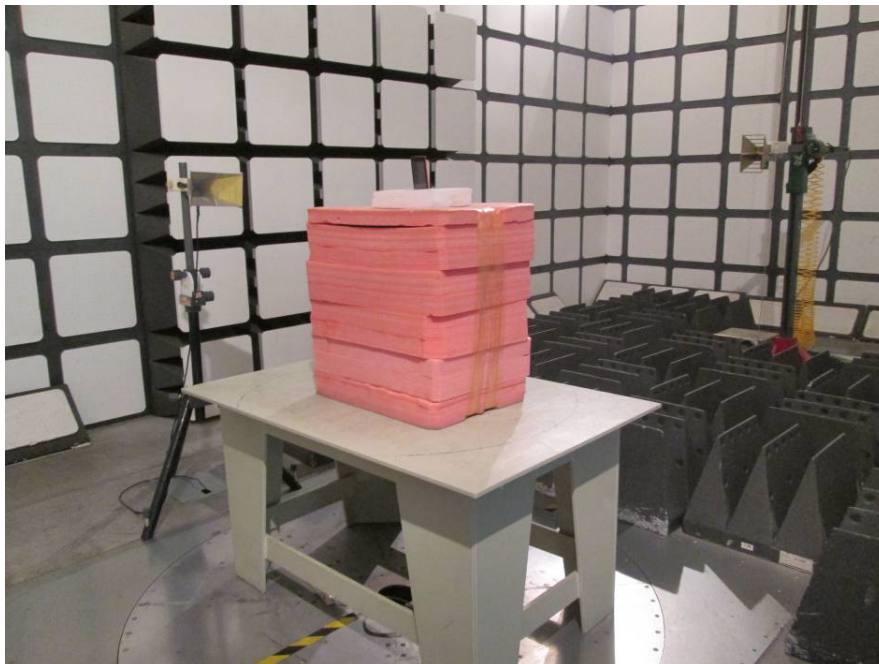
Radiated Emissions Test View (Above 1 GHz)
