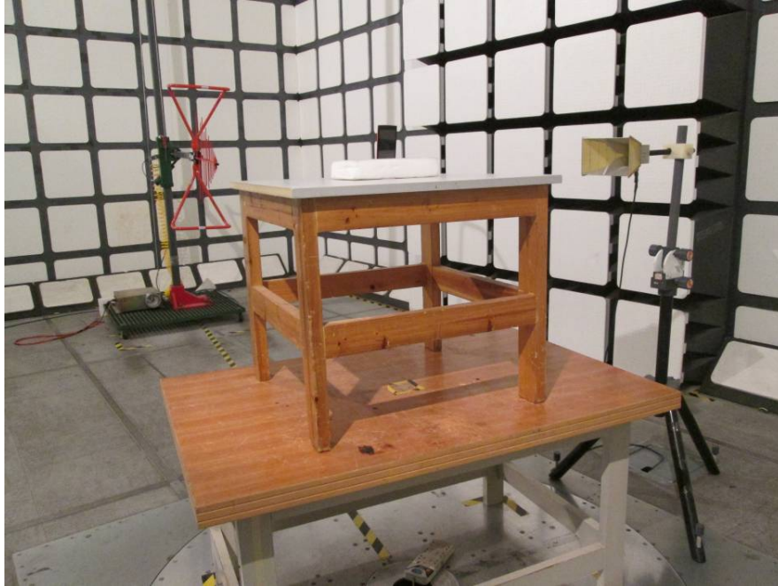
Radiated Emissions Test View (Below 1 GHz)
