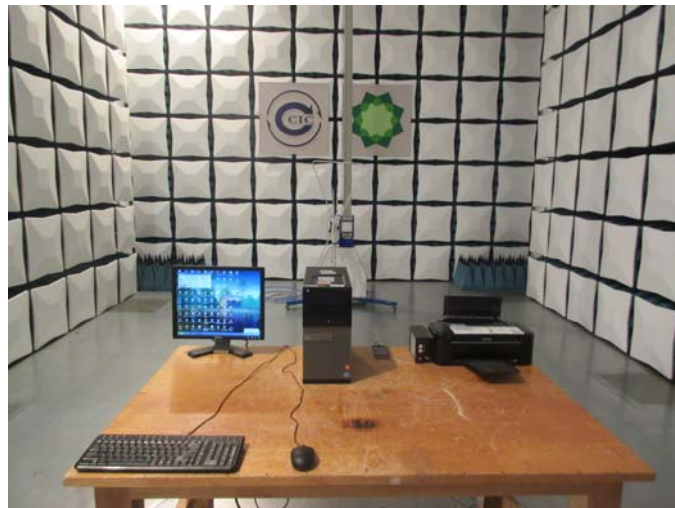
Radiated Emission (above 1GHz) PC Data Transfer
