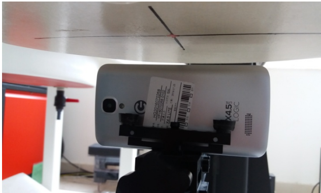
Hotspot mode - Left Side (10mm)
