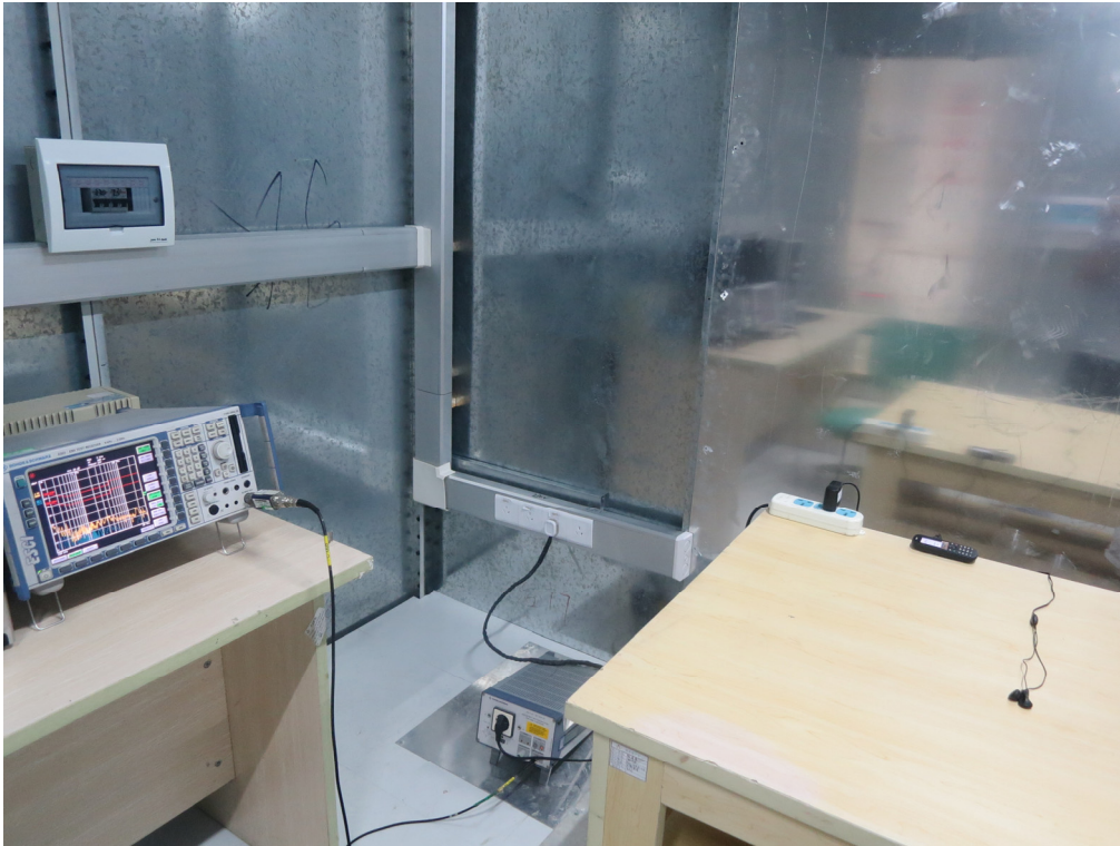
FCC LINE CONDUCTED EMISSION TEST SETUP
