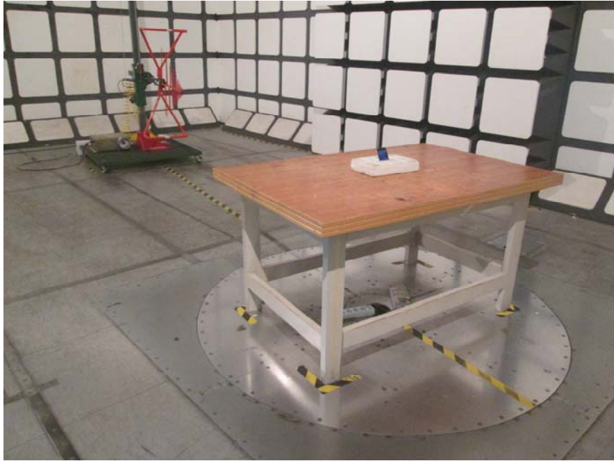
Radiated Emissions View (Below 1 GHz)
