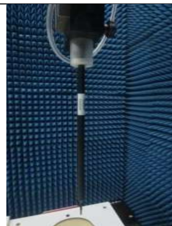
Fig.8.2 Photo of E-Field Probe
