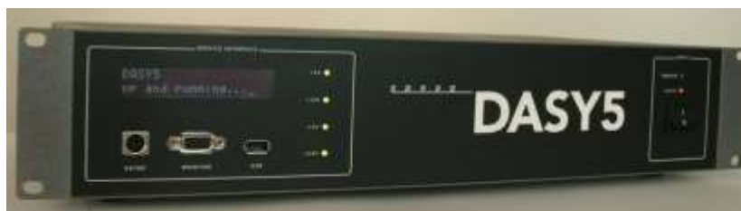
Fig. 8.5 Photo of Server for DASY5
