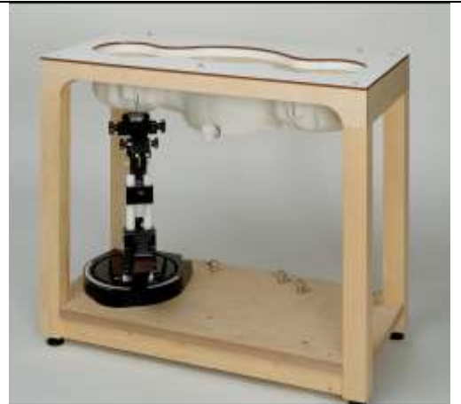
Fig. 8.7 Photo of SAM Twin Phantom
