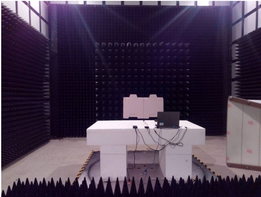
Radiated Emissions – Rear View (Above 1 GHz)
