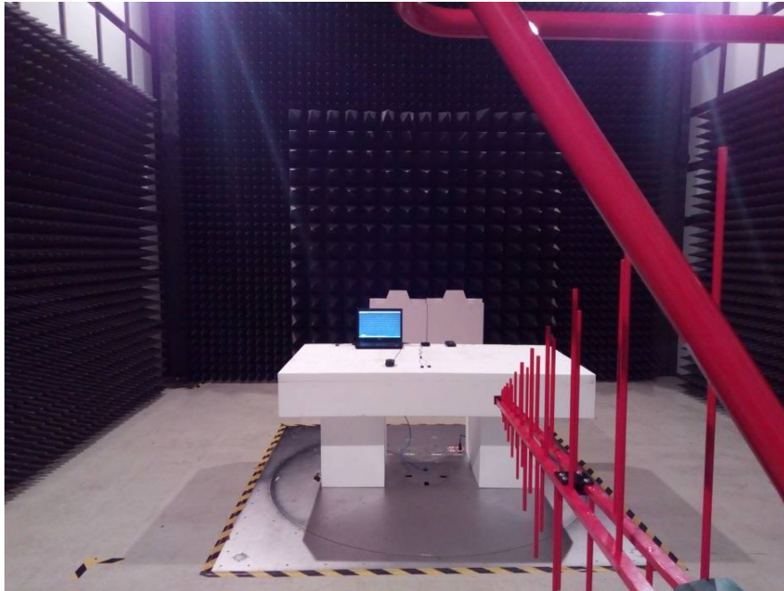
Radiated Emissions – Front View (Below 1 GHz)
