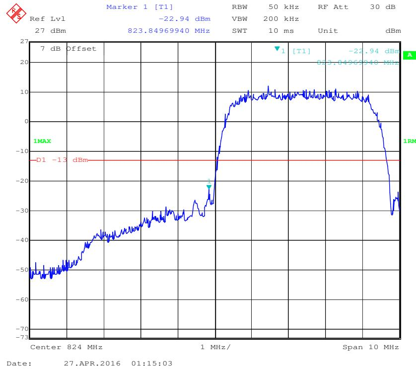
**Cellular Band, Right Band Edge for WCDMA (BPSK) Mode**
