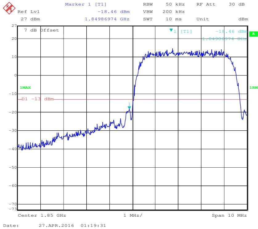
**PCS Band, Right Band Edge for WCDMA (BPSK) Mode**
