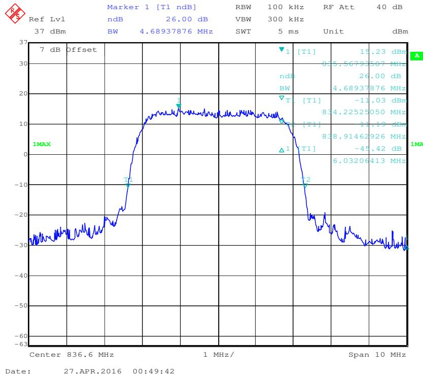
**PCS Band (Part 24E)****99% Occupied Bandwidth for GSM (GMSK) Mode**
