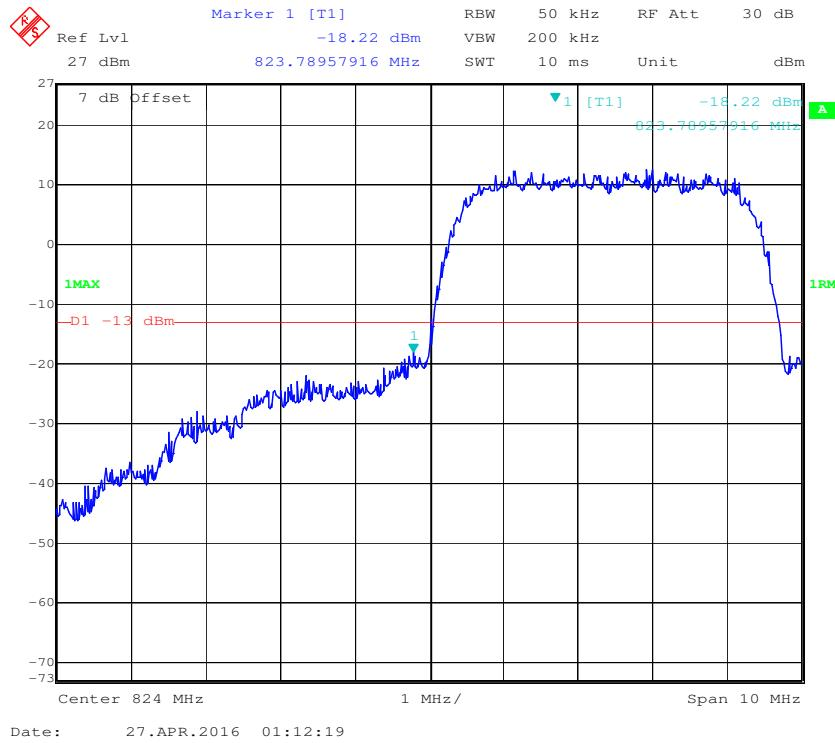
**Cellular Band, Right Band Edge for HSDPA (16QAM) Mode**
