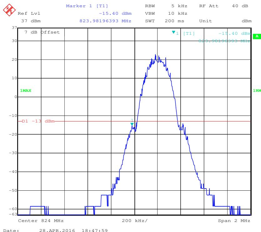
**Cellular Band, Right Band Edge for GSM (GMSK) Mode**
