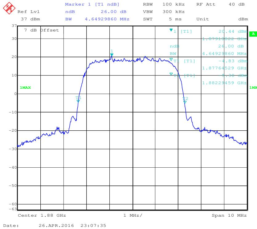
**99% Occupied Bandwidth for HSUPA (BPSK) Mode**
