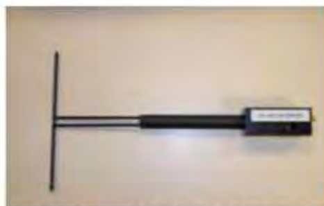
Figure 1 – Satimo COMOSAR Validation Dipole
