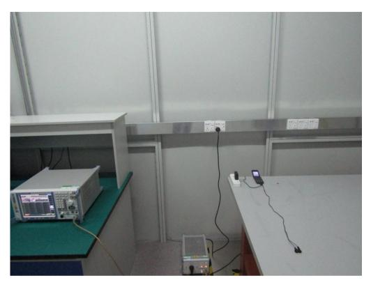
RADIATED EMISSION TEST SETUP
