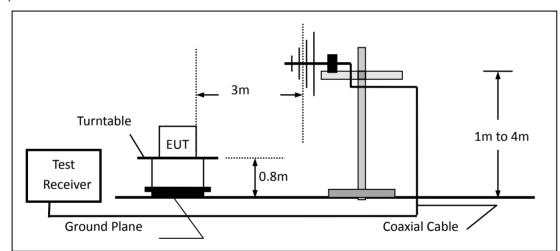
(c) For radiated emissions above 1000MHz
