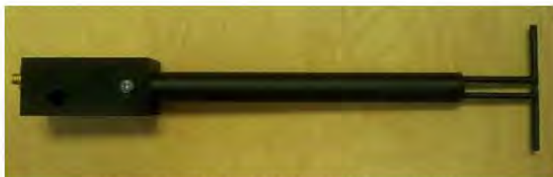
Figure 1 – MVG COMOSAR Validation Dipole
