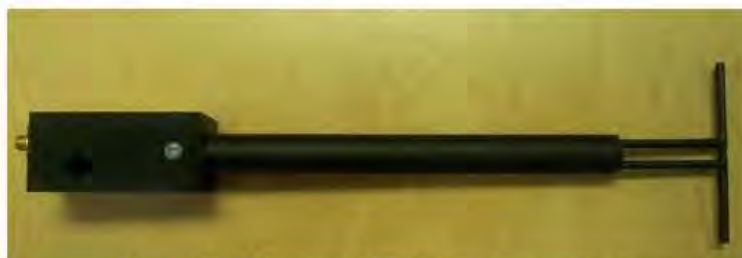
Figure 1 – MVG COMOSAR Validation Dipole
