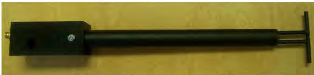
Figure 1 – MVG COMOSAR Validation Dipole
