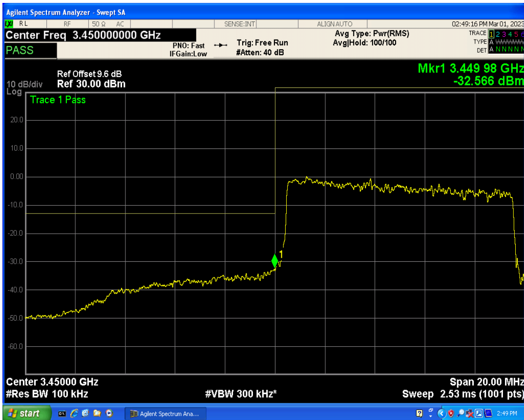
Band42 QPSK BW=10MHz Channel=43040 RB Size=1 Position=#0
