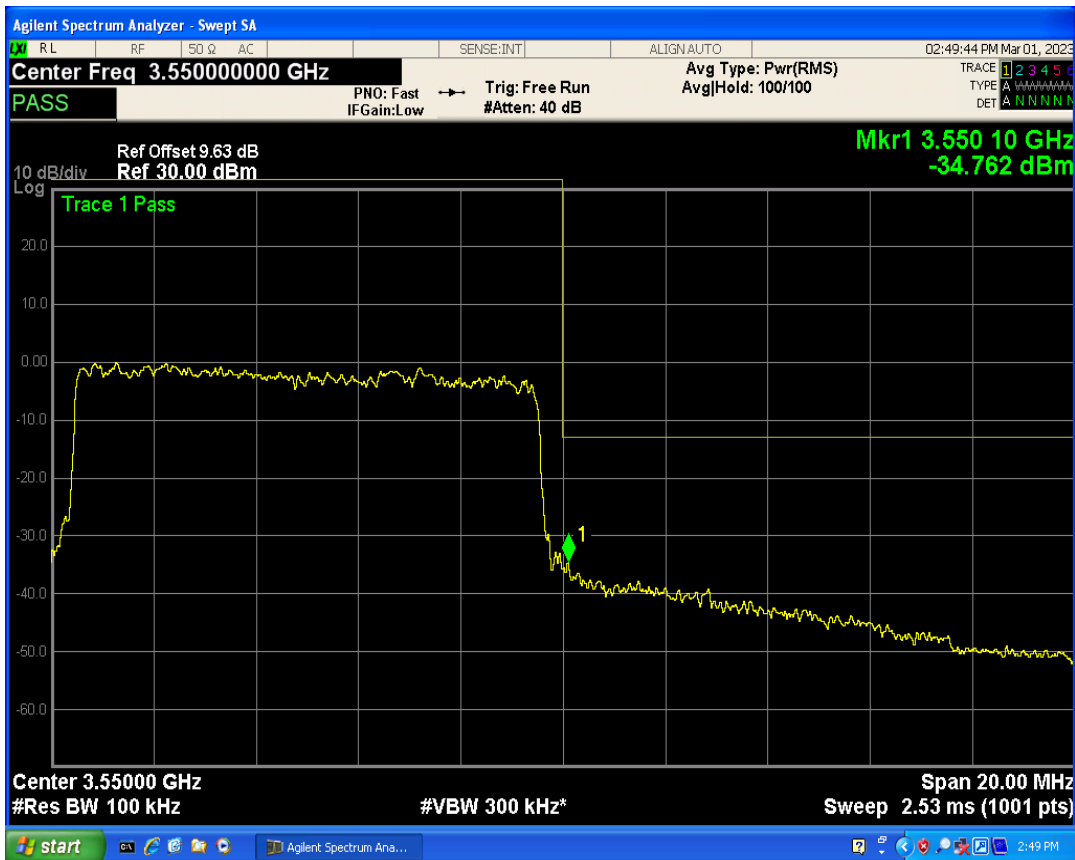
Band42 QPSK BW=15MHz Channel=42165 RB Size=1 Position=#0
