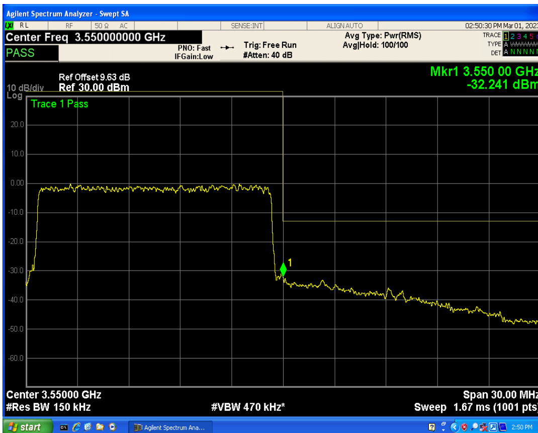
Band42 QAM16 BW=15MHz Channel=43015 RB Size=1 Position=#0
