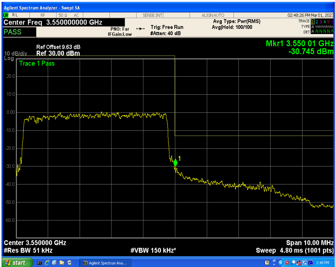
Band42 QAM16 BW=5MHz Channel=43065 RB Size=1 Position=#Max
