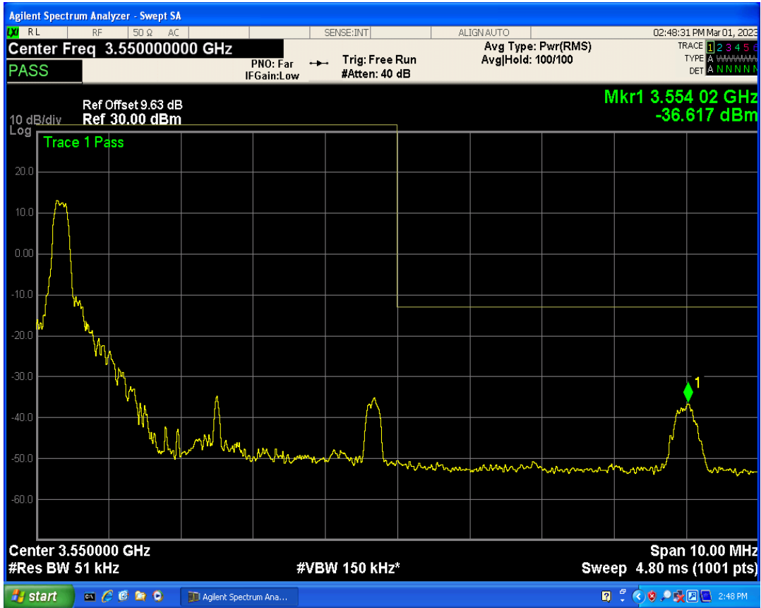
Band42 QPSK BW=5MHz Channel=43065 RB Size=25 Position=#0
