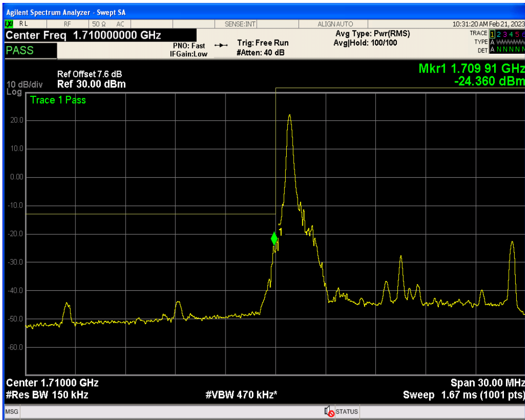
Band4 QPSK BW=15MHz Channel=20025 RB Size=75 Position=#0
