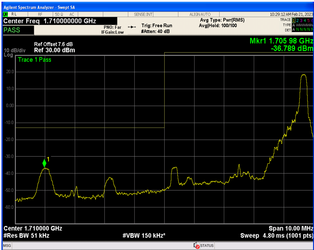
Band4 QPSK BW=5MHz Channel=19975 RB Size=25 Position=#0
