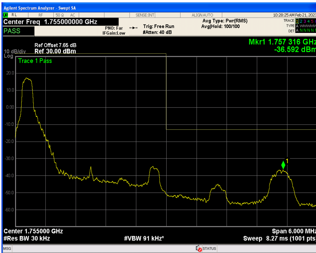
Band4 QPSK BW=3MHz Channel=20385 RB Size=1 Position=#Max
