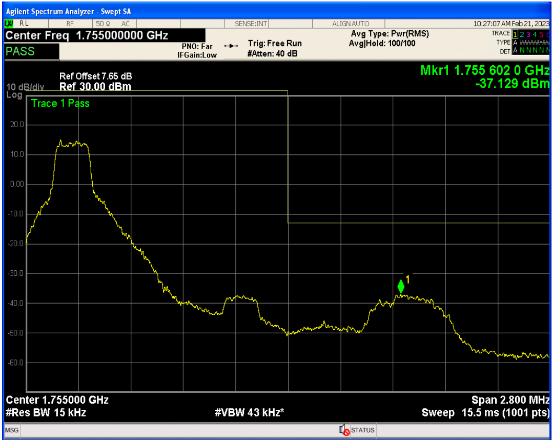
Band4 QPSK BW=1.4MHz Channel=20393 RB Size=1 Position=#Max
