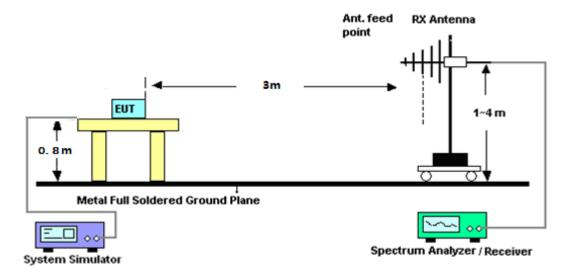
For radiated test from above 1GHz
