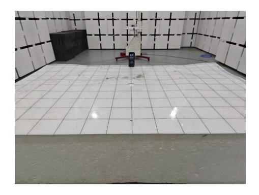
Set-up for Radiated Spurious Emission, Above 1GHz
