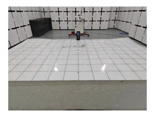
Set-up for Radiated Spurious Emission, Above 1GHz
