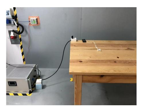
Set-up for Radiated Emission (RE), Below 1GHz
