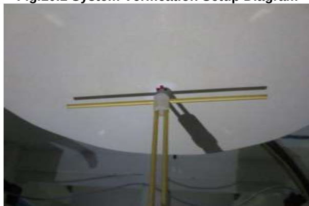
Fig.10.2 Photo of Dipole setup
