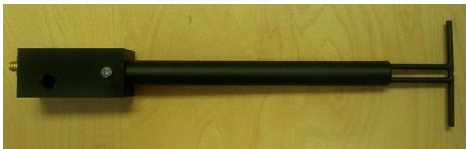
Figure 1 – MVG COMOSAR Validation Dipole
