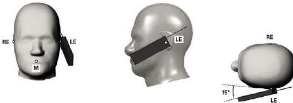
Fig.11.4 Illustration for Tilted Position
