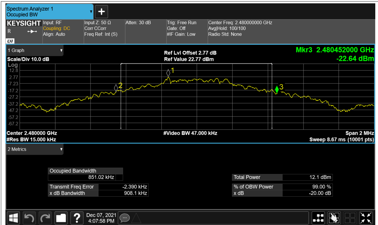
-20dB Bandwidth NVNT 2-DH1 2402MHz Ant1
