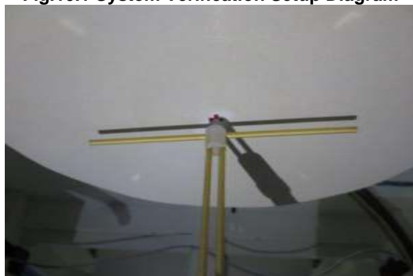
Fig.10.2 Photo of Dipole setup
